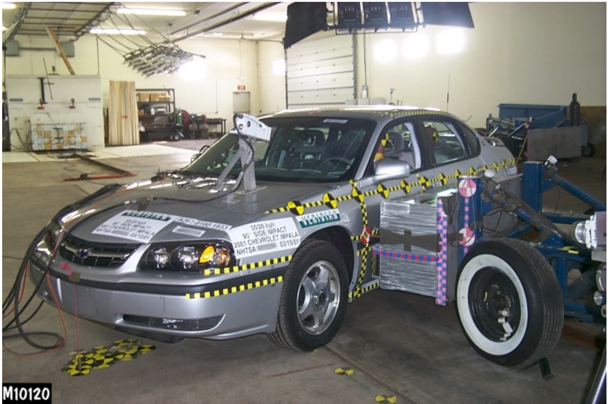
Figure A-29: PRE-TEST LEFT SIDE VIEW OF MDB WITH IMPACTOR FACE IN POSITION
