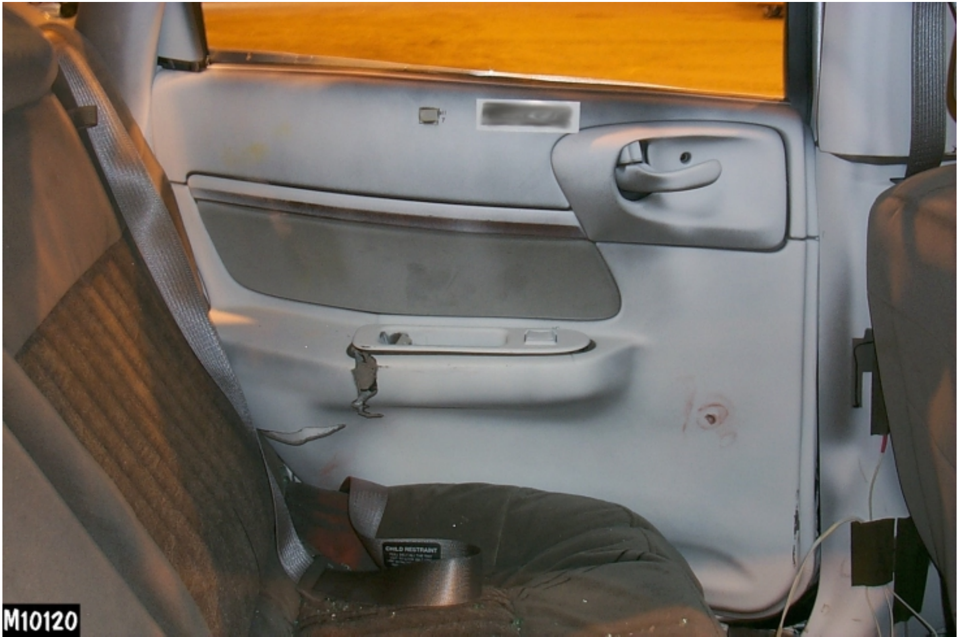
Figure A-28: POST-TEST REAR INTERIOR TRIM SHOWING SID IMPACT LOCATIONS
