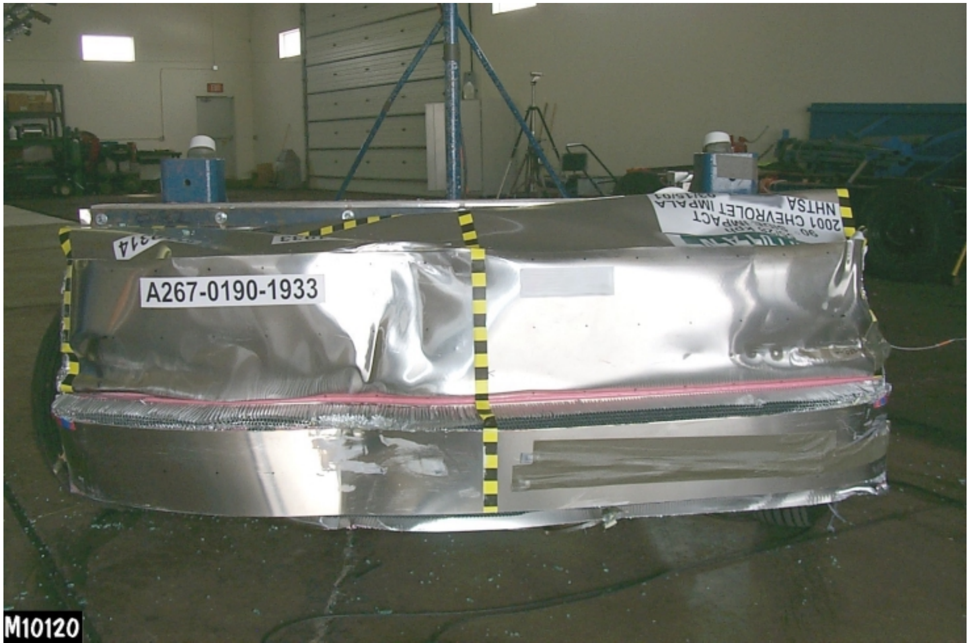
Figure A-8: POST-TEST FRONTAL VIEW OF IMPACTOR FACE
