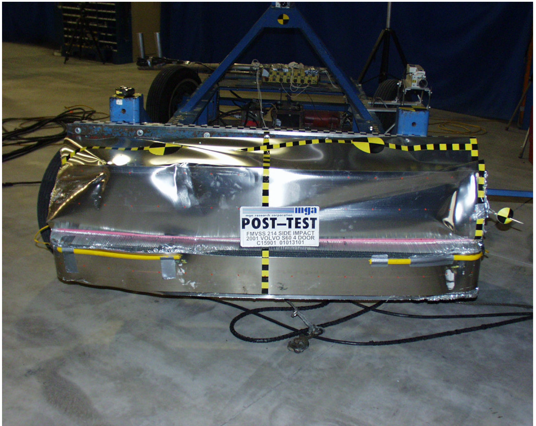
Photo No. A-16 - Post-Test MDB Front View
