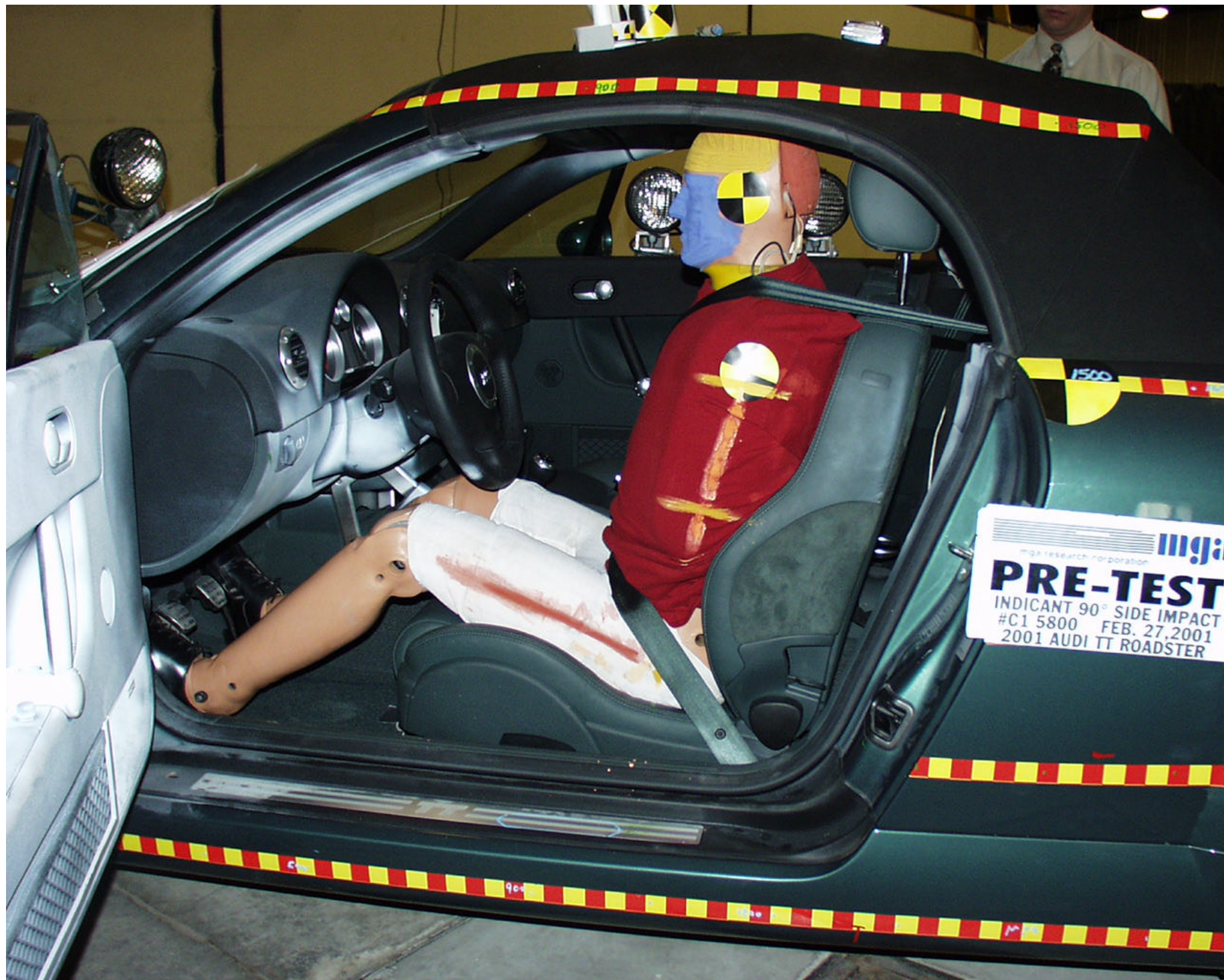
Photo No. A-25 - Pre-Test Driver Dummy Left Side View (Door Open)
