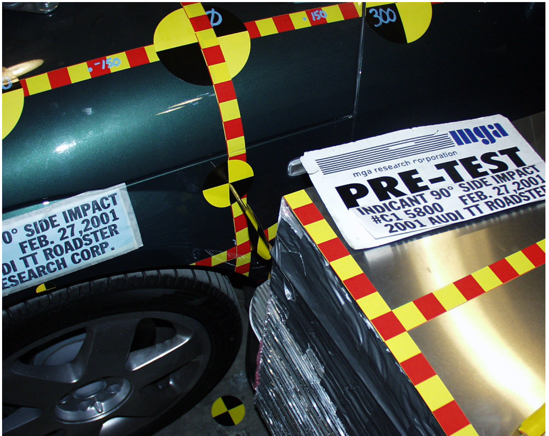
Photo No. A-30 - Pre-Test Left Front Impact Point on Vehicle
