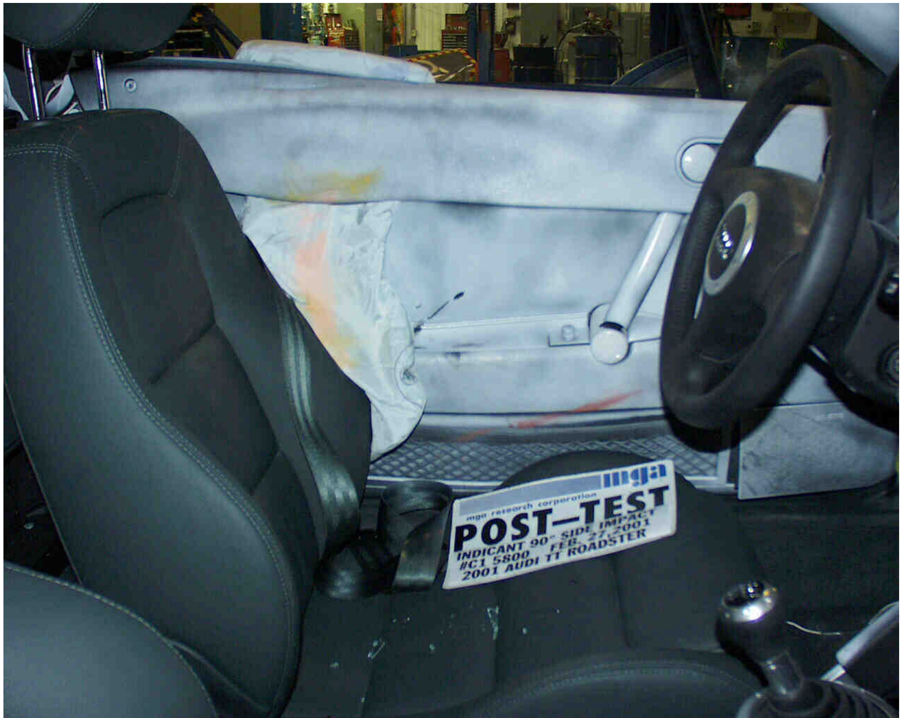
Photo No. A-28 - Post-Test Driver Dummy Contact
