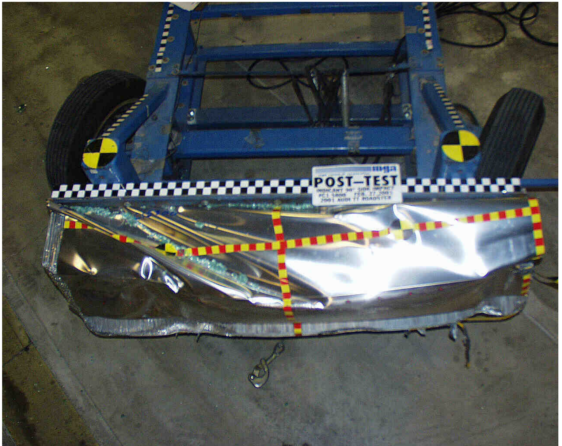
Photo No. A-14 - Post-Test MDB Top View
