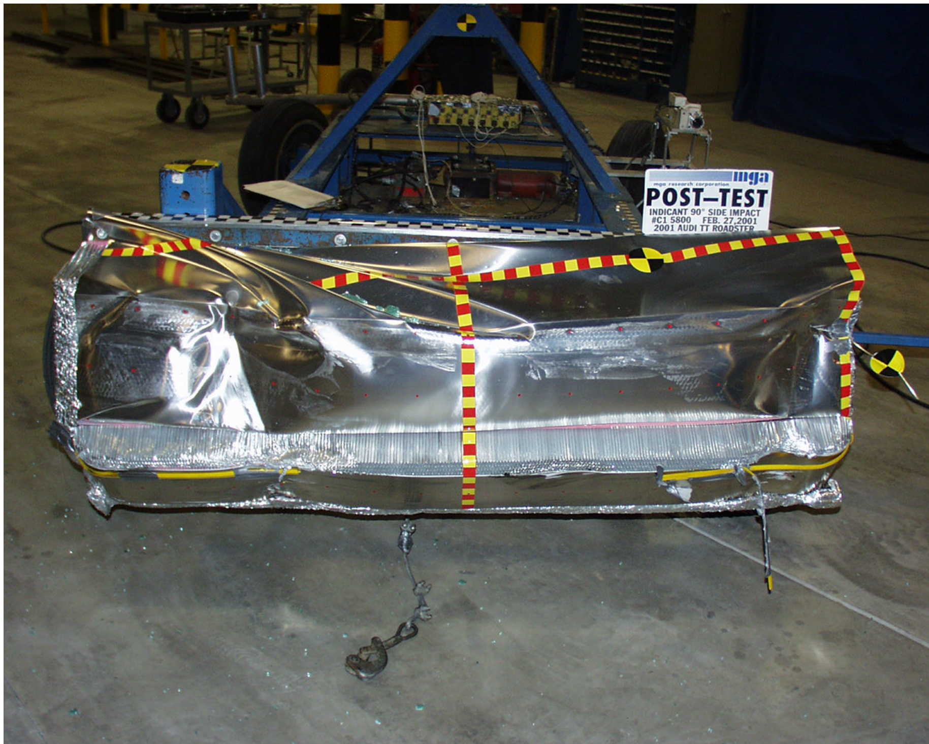
Photo No. A-16 - Post-Test MDB Front View
