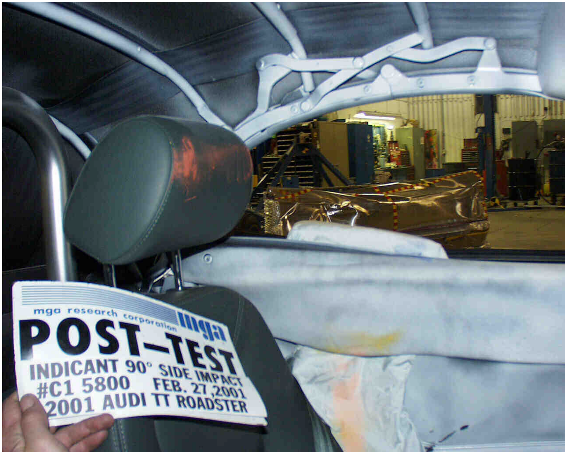
Photo No. A-29 - Post-Test Driver Dummy Head Contact
