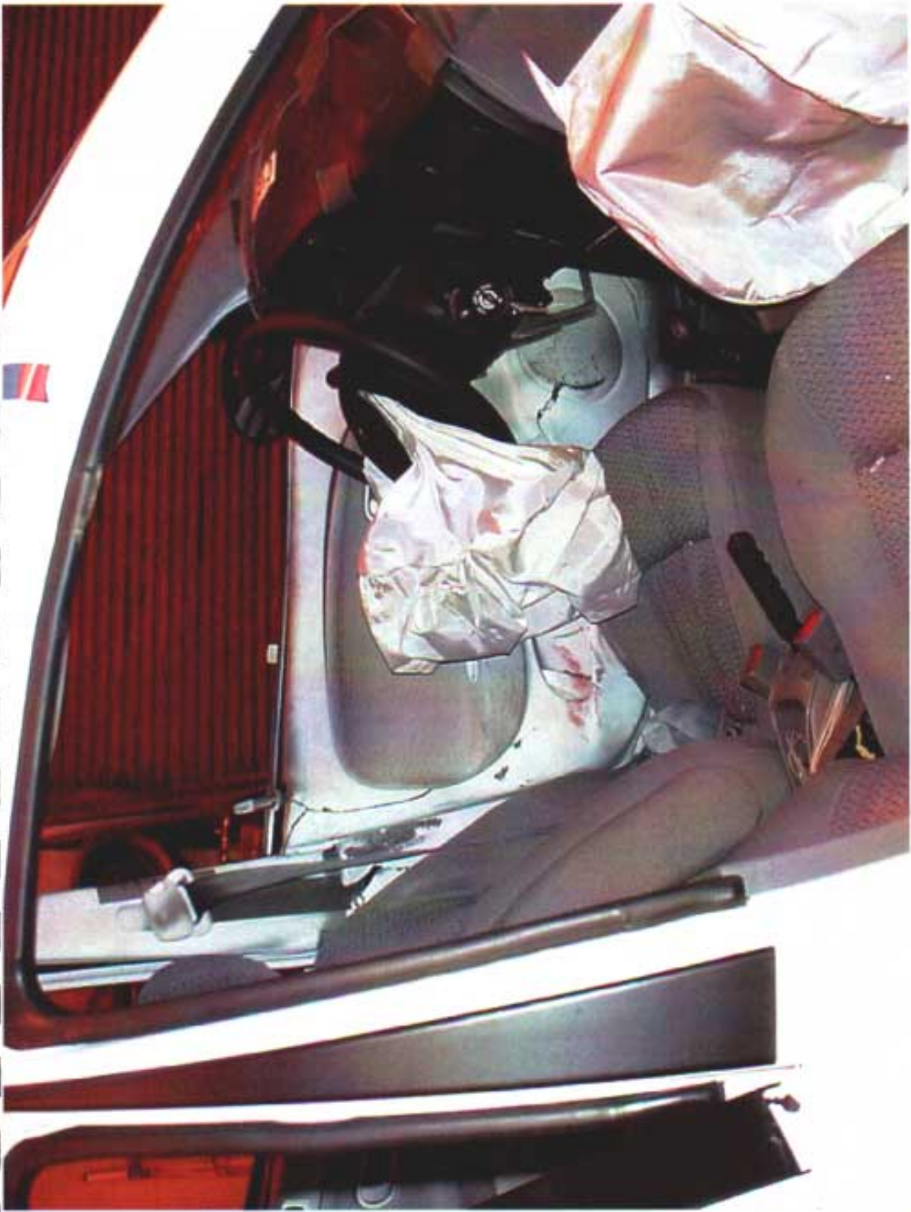
Figure A-26 POST-TEST INTERIOR OF FRONT DOOR SHOWING SID IMPACT LOCATIONS
