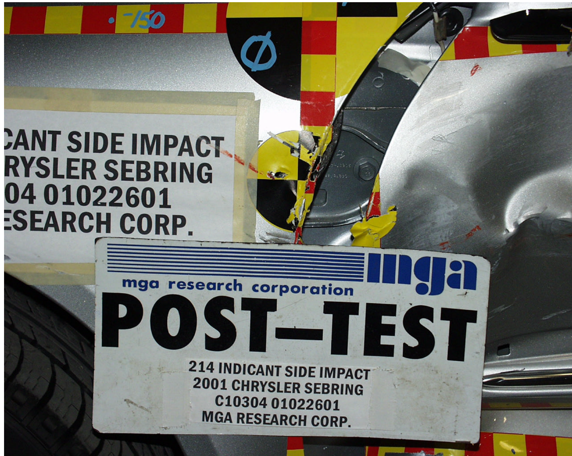
Photo No. A-38 - Post-Test Left Front Impact Point on Vehicle
