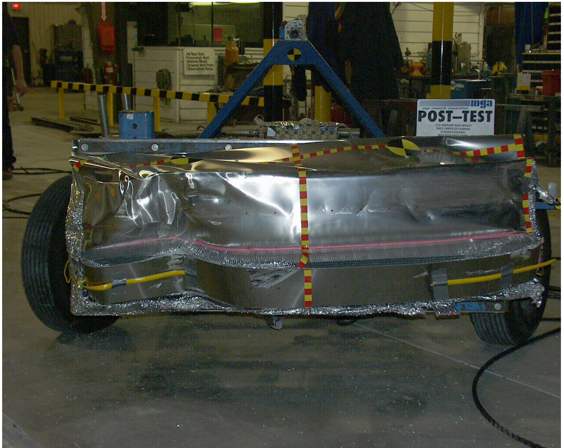
Photo No. A-16 - Post-Test MDB Front View
