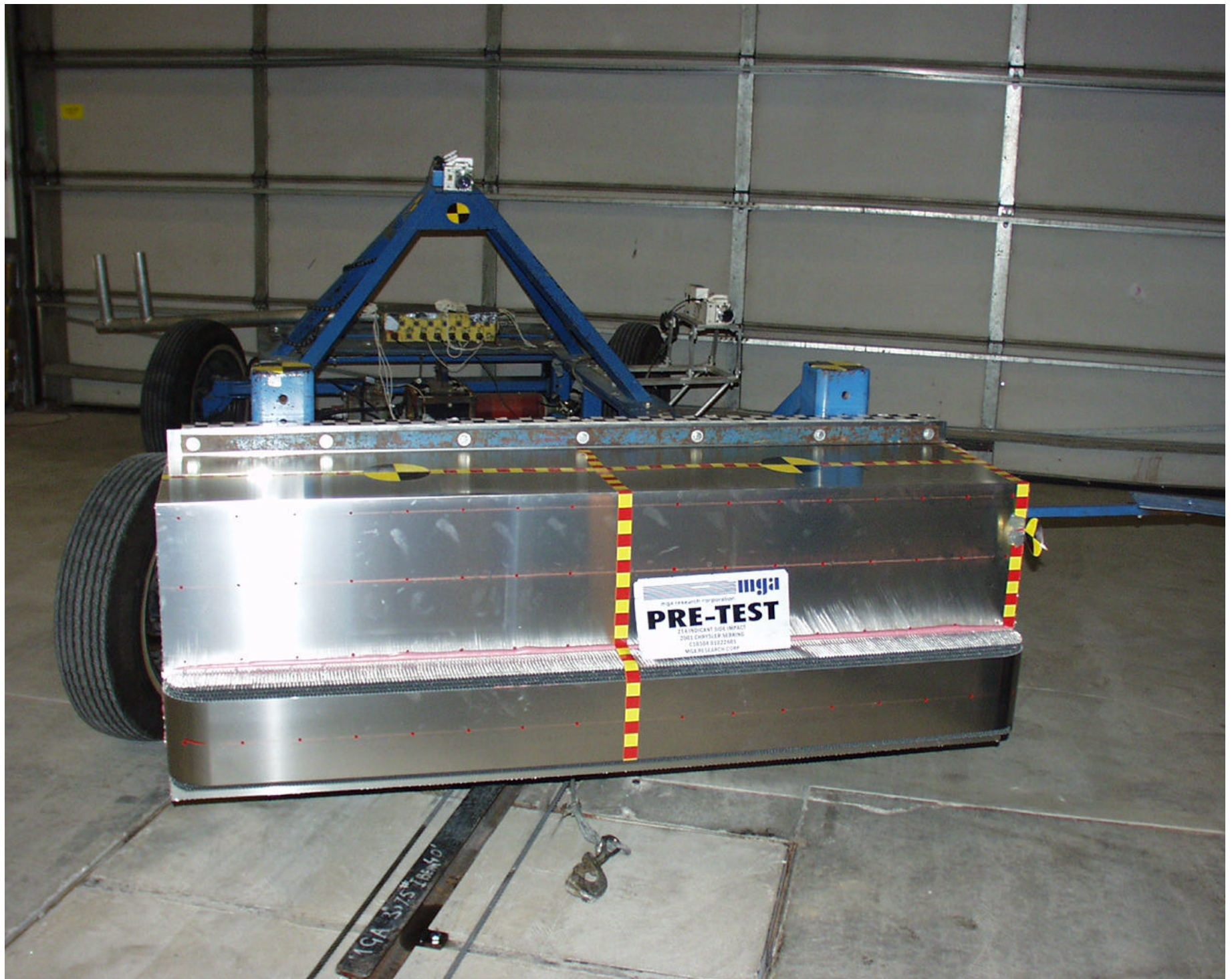
Photo No. A-15 - Pre-Test MDB Front View
