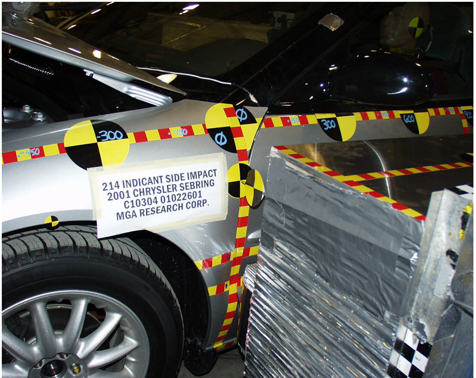
Photo No. A-37 - Pre-Test Left Front Impact Point on Vehicle
