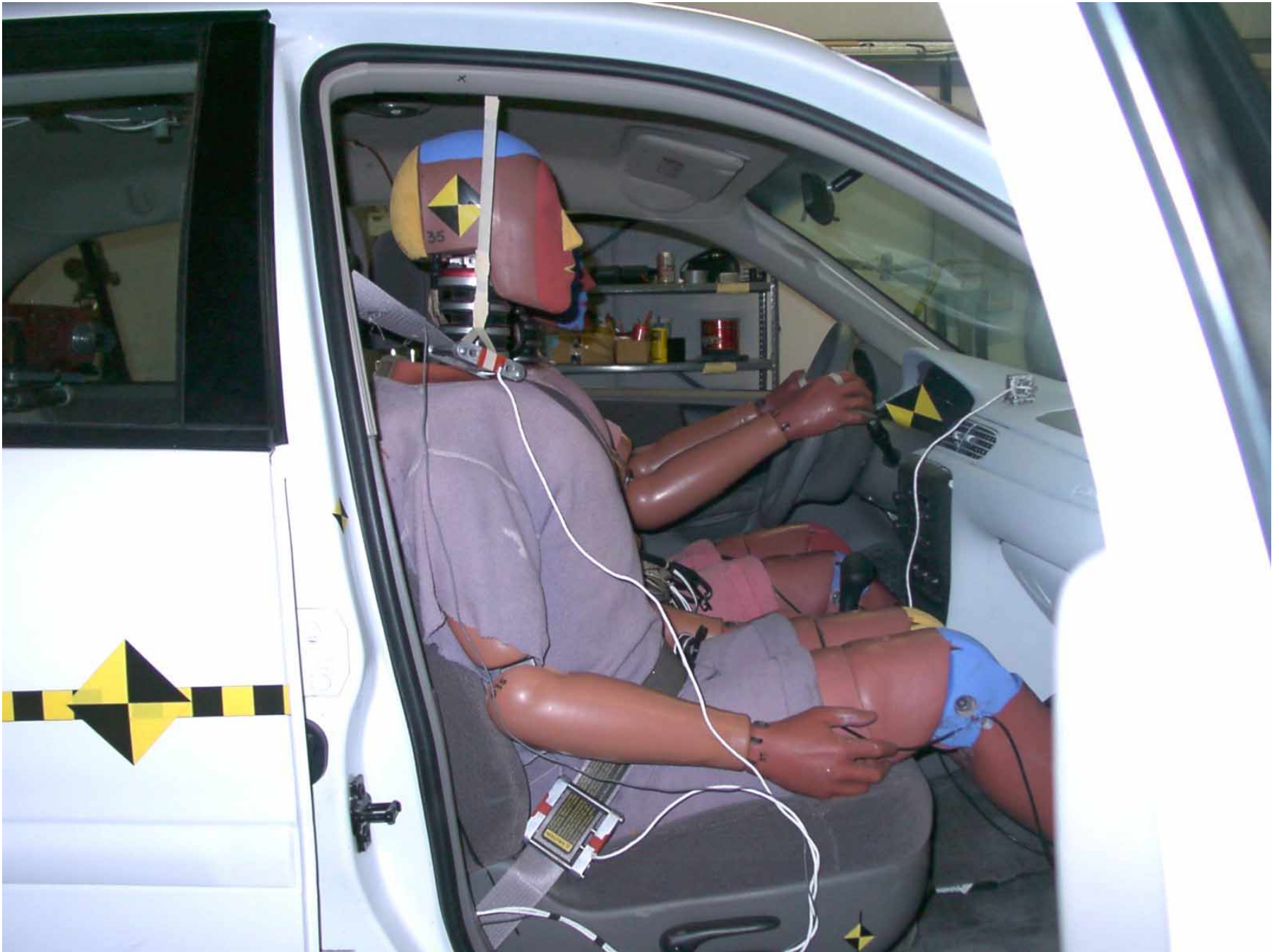
Figure A-47: Passenger Dummy 90° To Vehicle, Pre-Test
