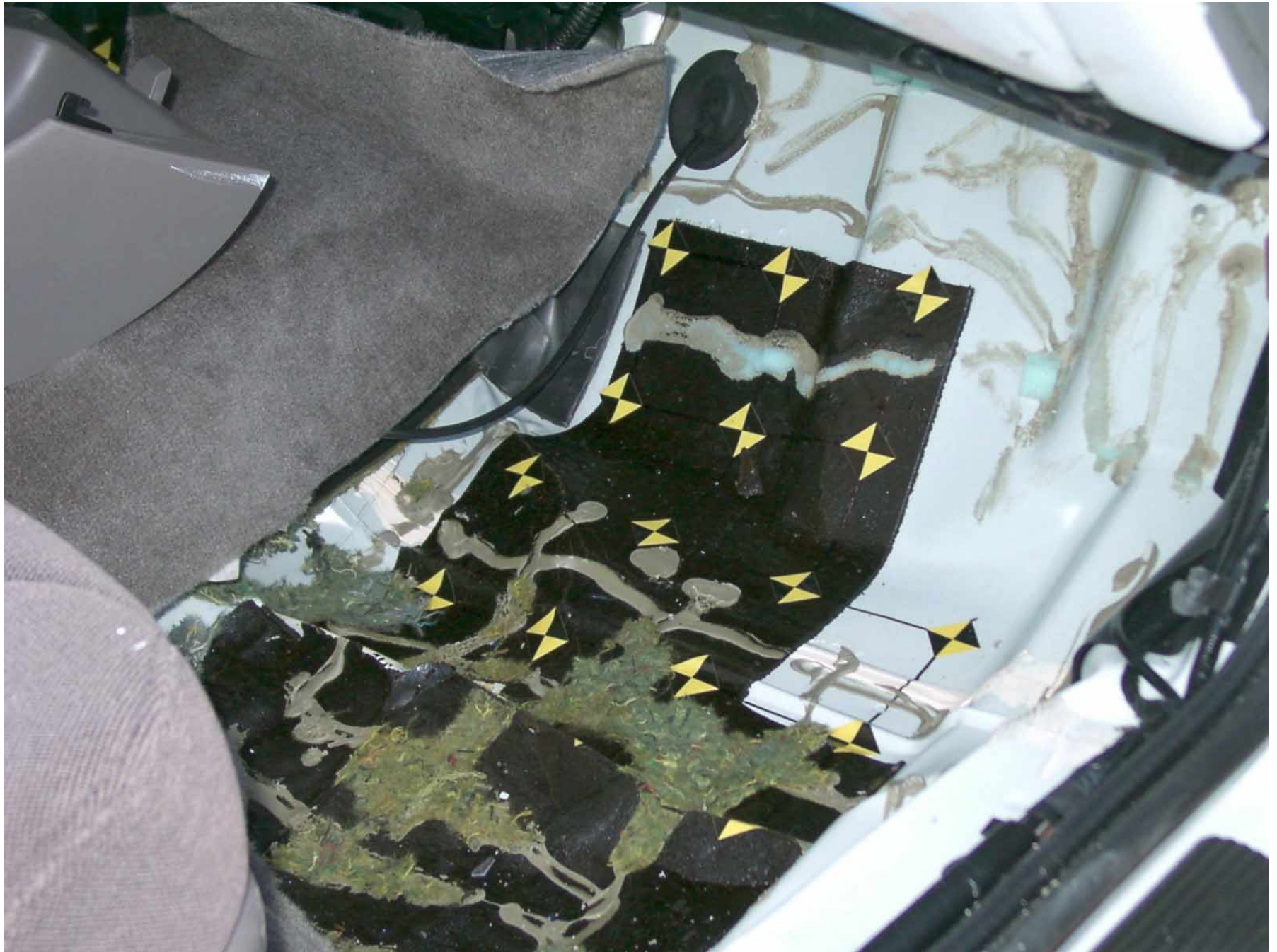
Figure A-52: Passenger Side Floor Pan, Post-Test
