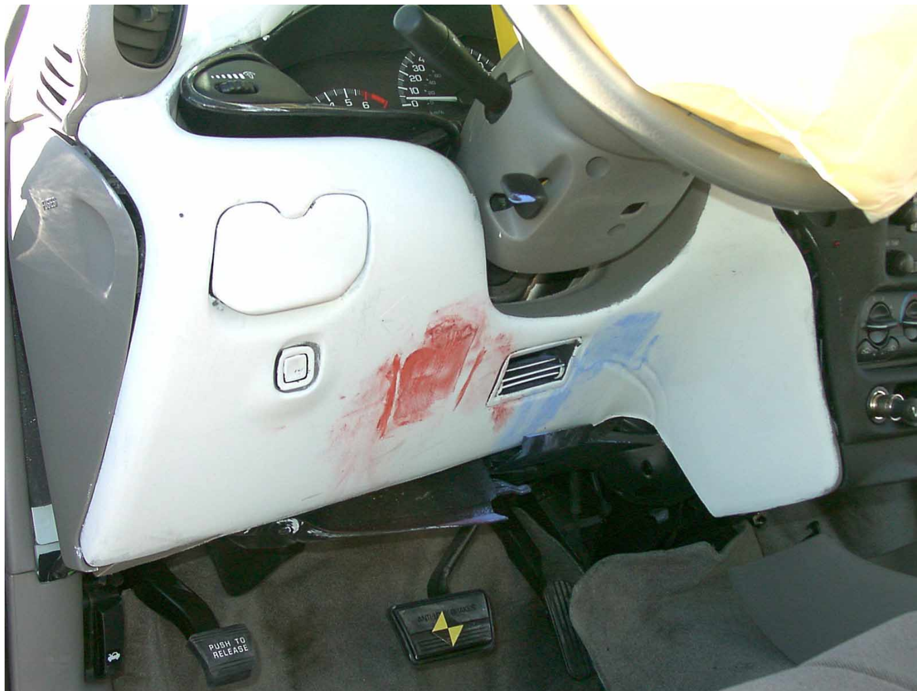
Figure A-36: Driver Side Knee Bolster, Post-Test
