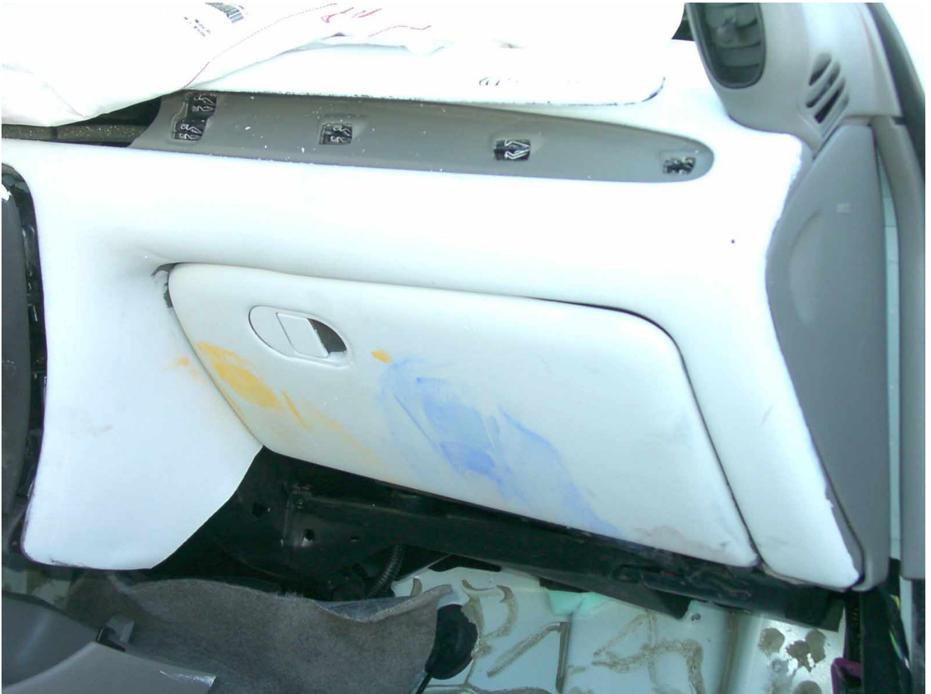
Figure A-54: Passenger Side Knee Bolster, Post-Test
