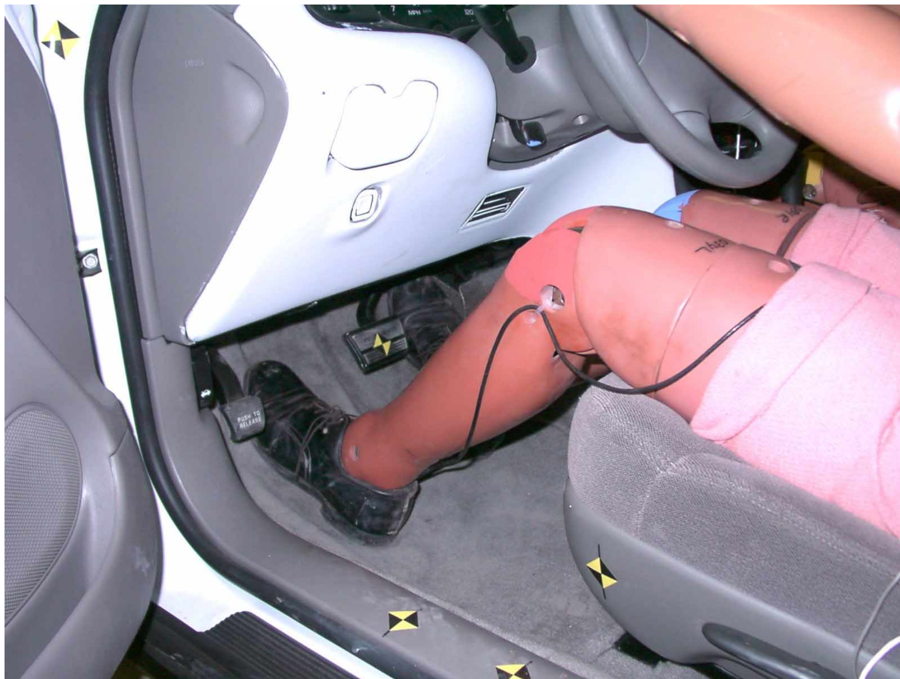
Figure A-33: Driver Dummy Feet, Pre-Test
