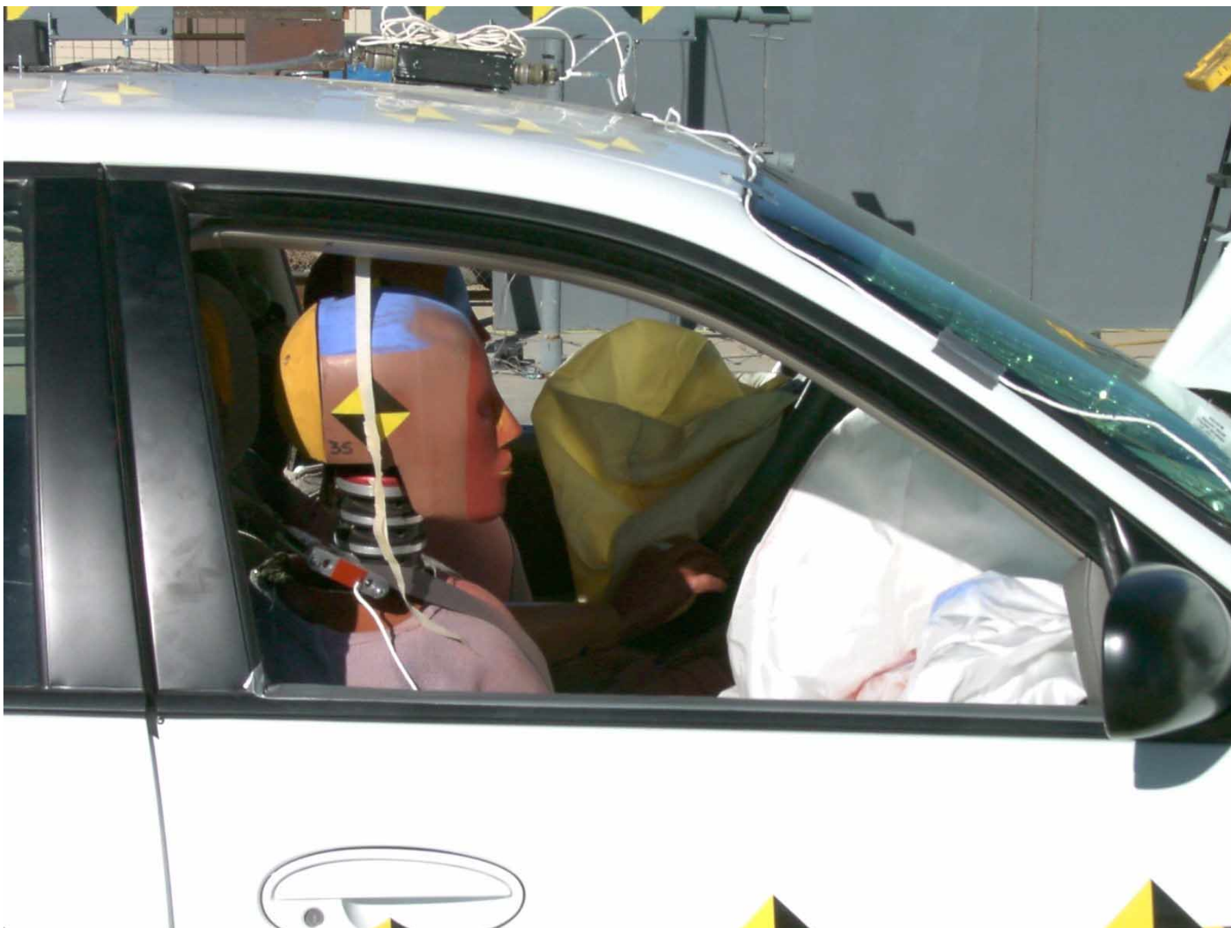
Figure A-44: Passenger Dummy Through Window, Post-Test
