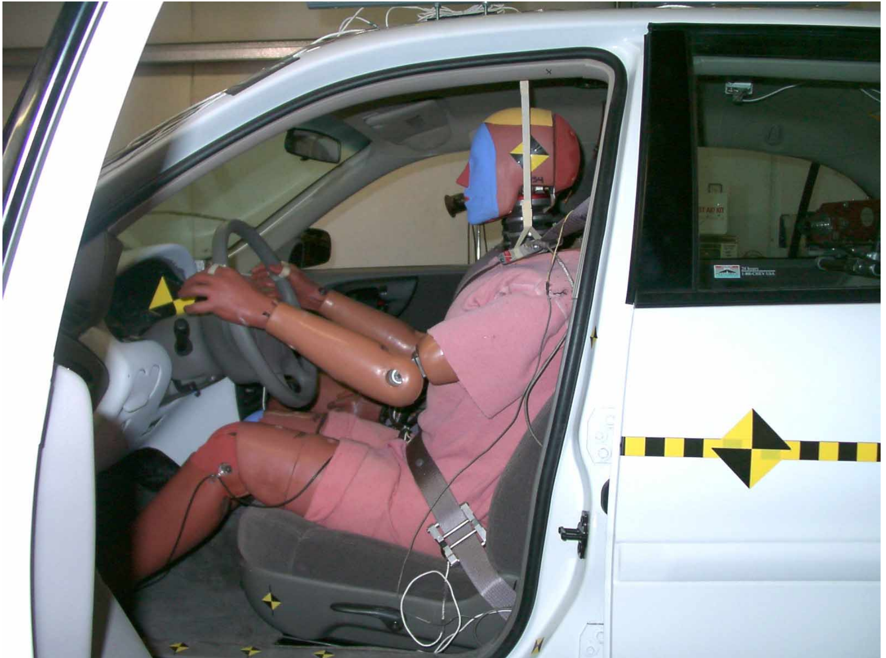
Figure A-31: Driver Dummy 90° To Vehicle, Pre-Test
