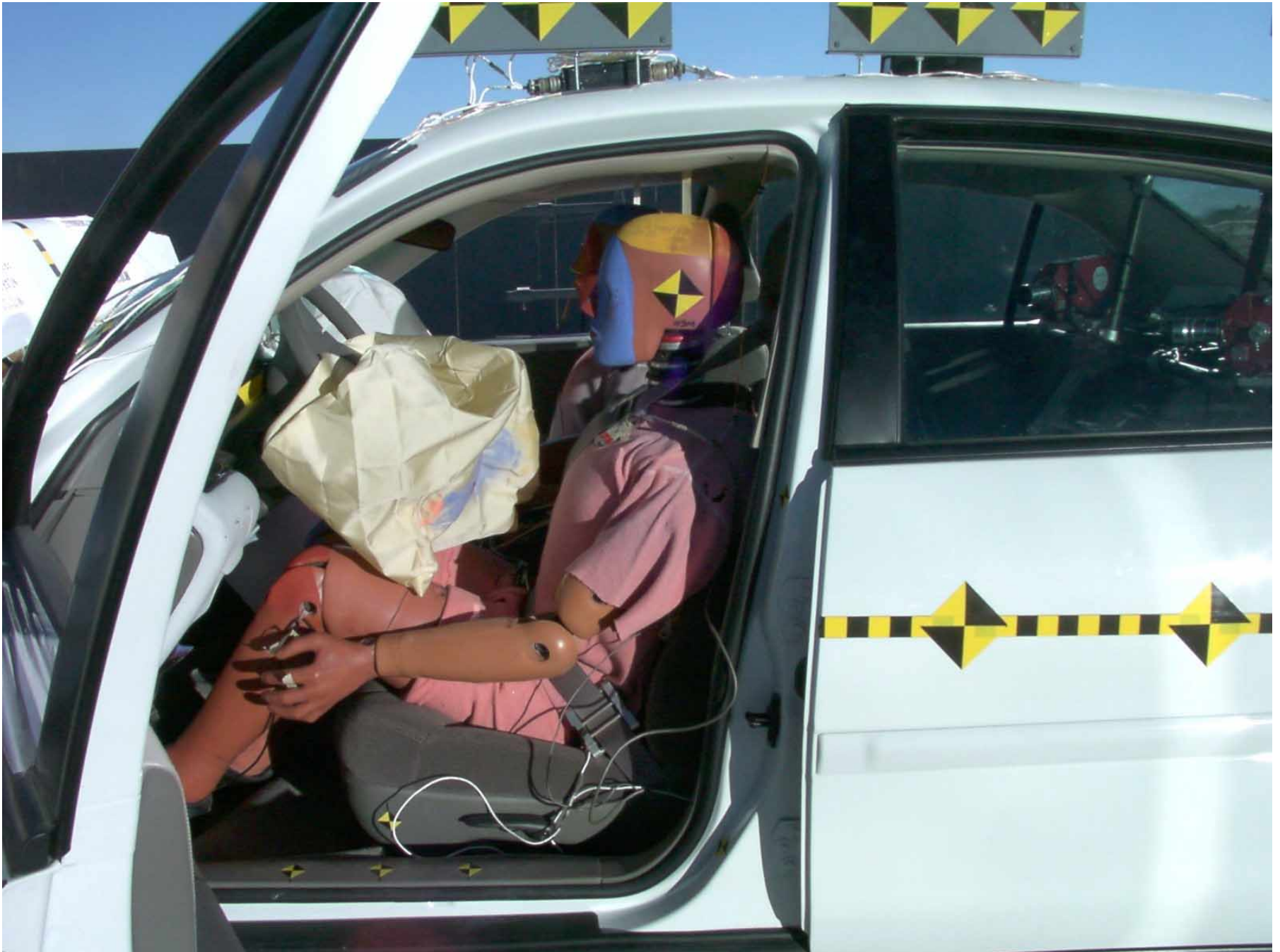
Figure A-32: Driver Dummy 90° To Vehicle, Post-Test
