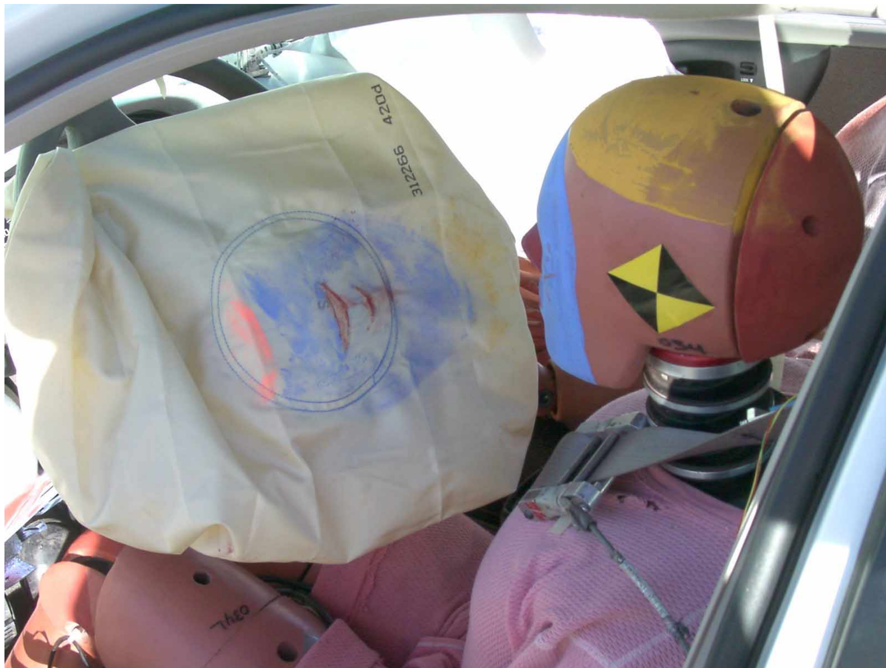
Figure A-40: Driver Dummy Contact, Post-Test
