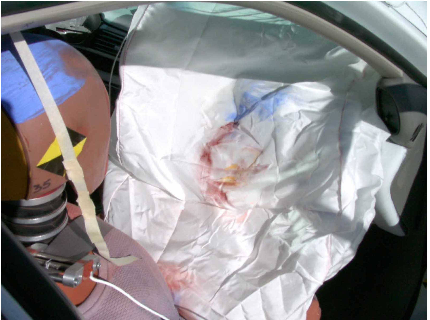
Figure A-56: Passenger Dummy Contact, Post-Test
