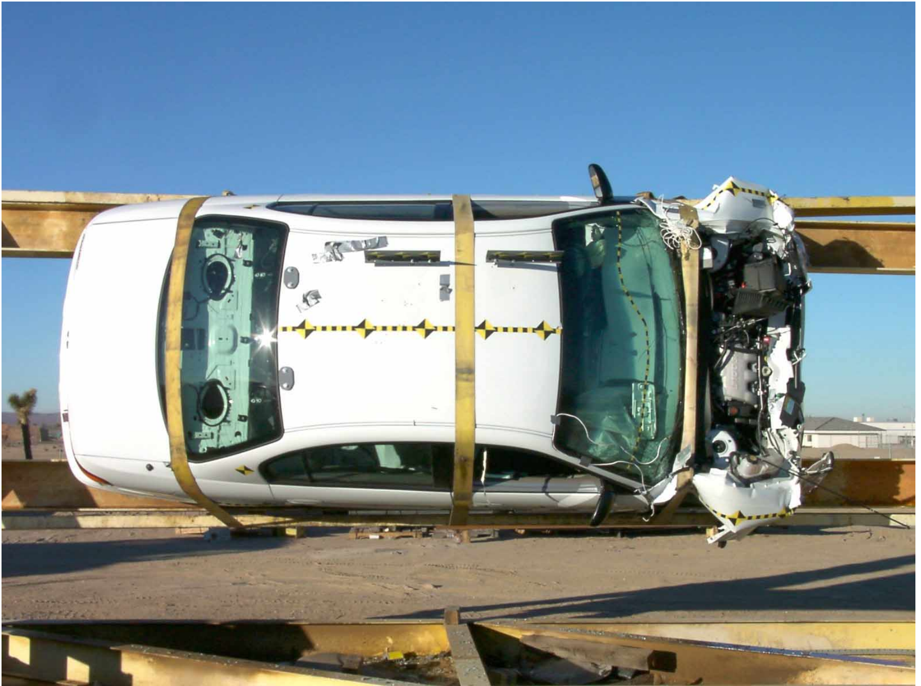
Figure A-57: Vehicle on Rollover Device
