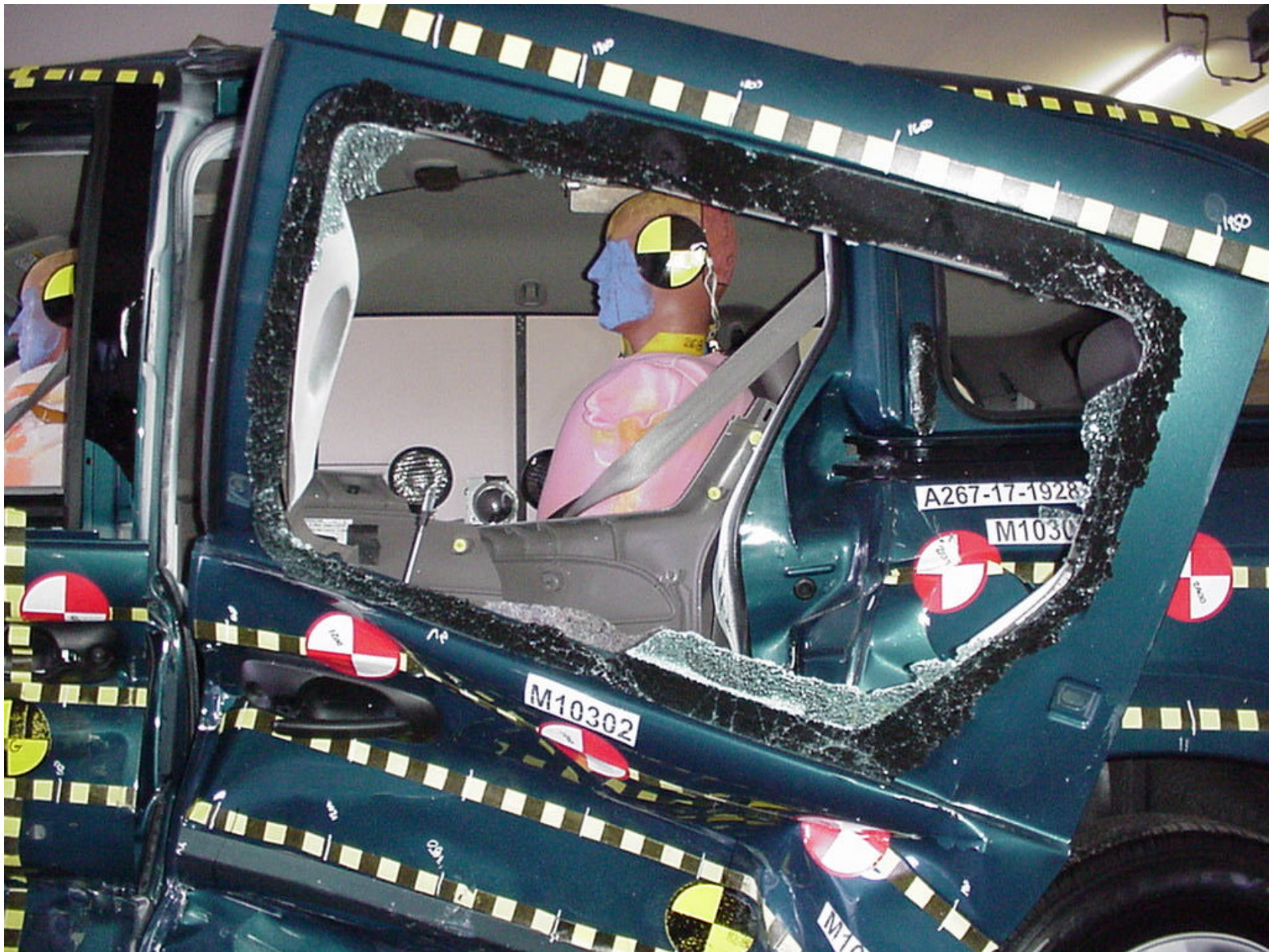
Figure A-24 POST-TEST LEFT OCCUPANT COMPARTMENT VIEW OF REAR SID
