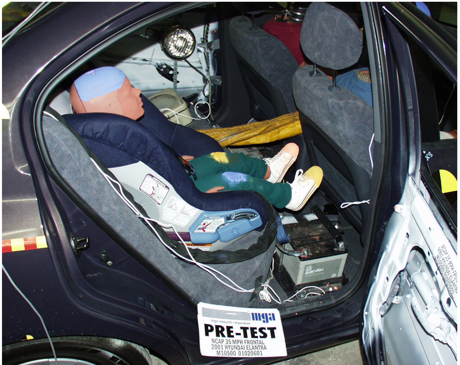
Photo 3 - Pre-Test RRS 3 Year Old Left Side View (Door Open)
