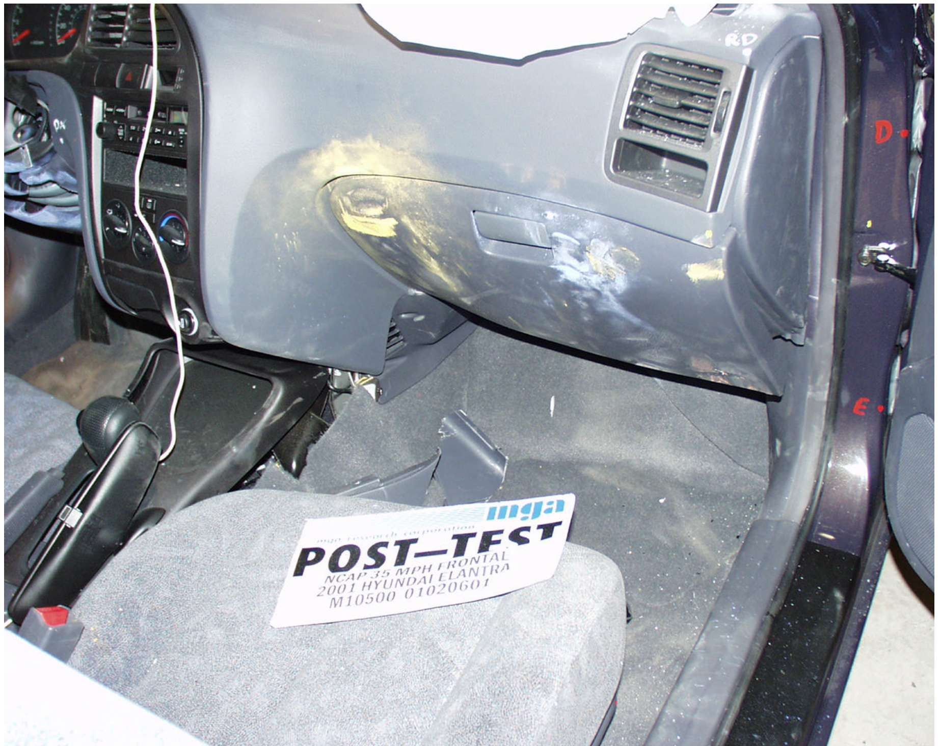
Photo No. A-45 - Post-Test Passenger Knee Contact View
