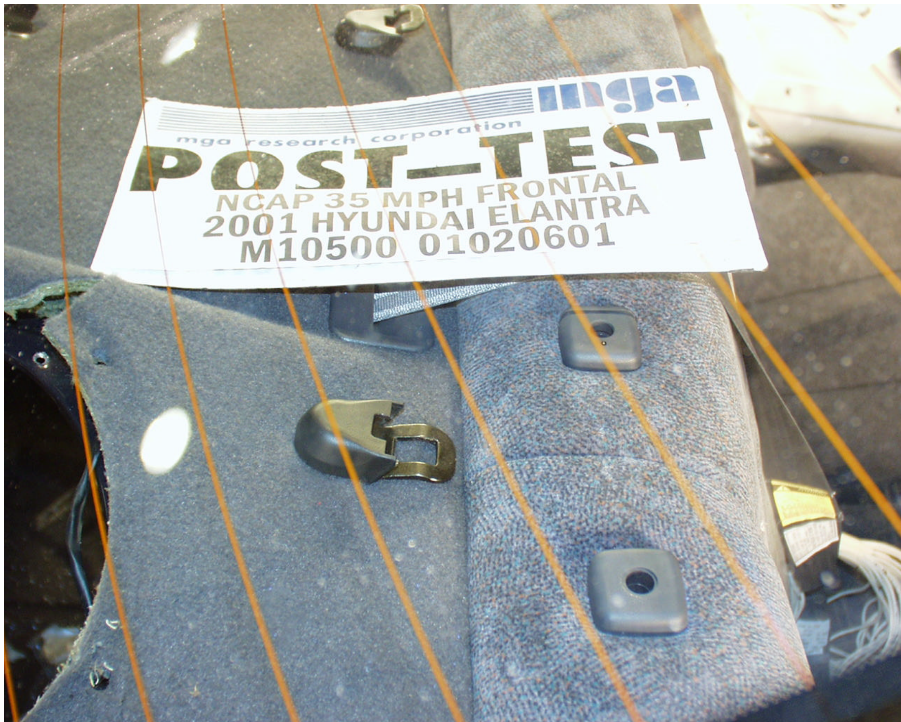
Photo 7 - Post-Test RRS Top Tether View
