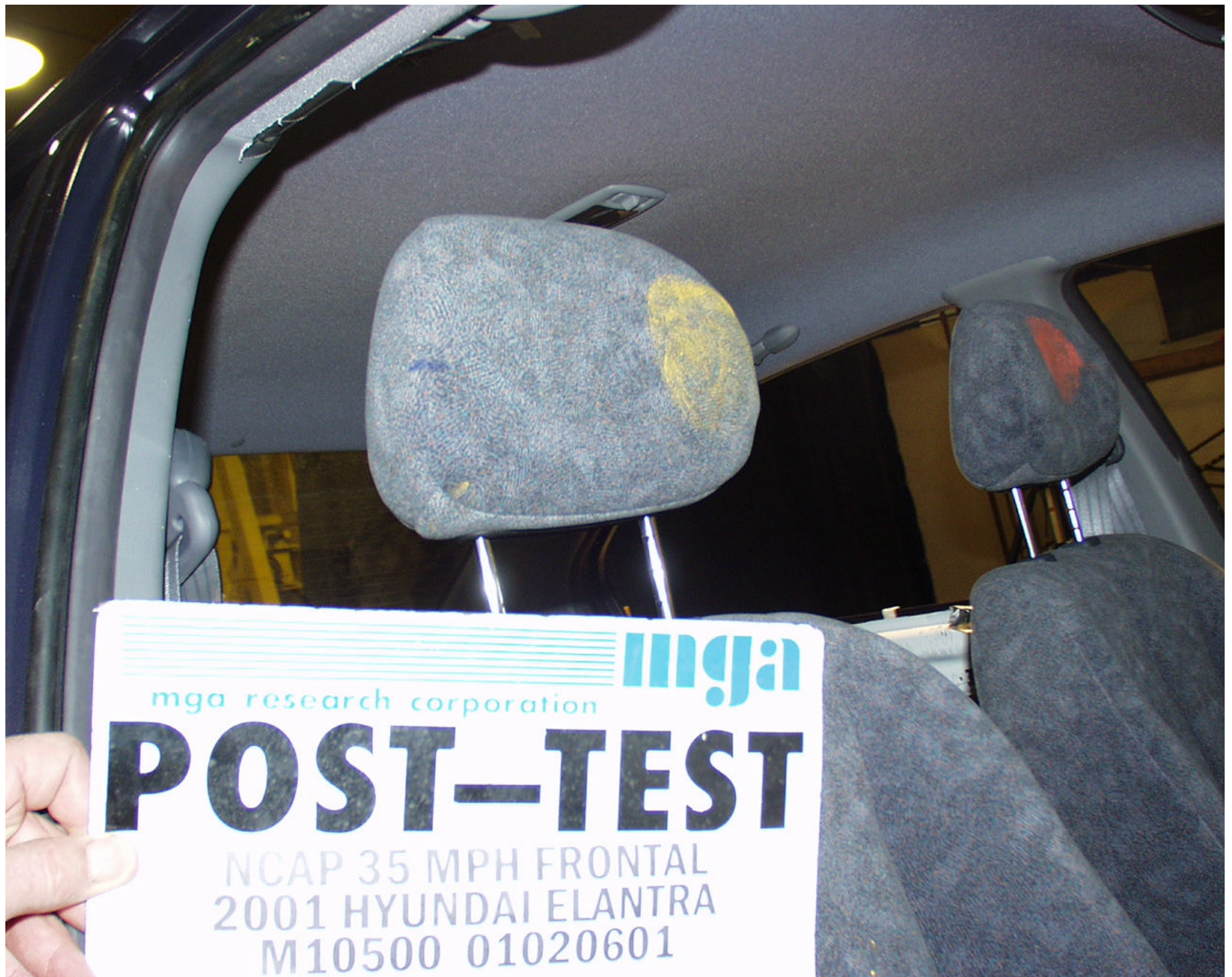
Photo No. A-46 - Post-Test Passenger Head Contact View
