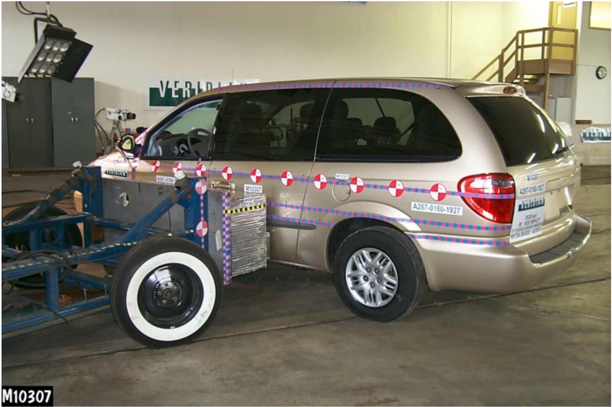
Figure A-30: PRE-TEST RIGHT SIDE VIEW OF MDB WITH IMPACTOR FACE IN POSITION
