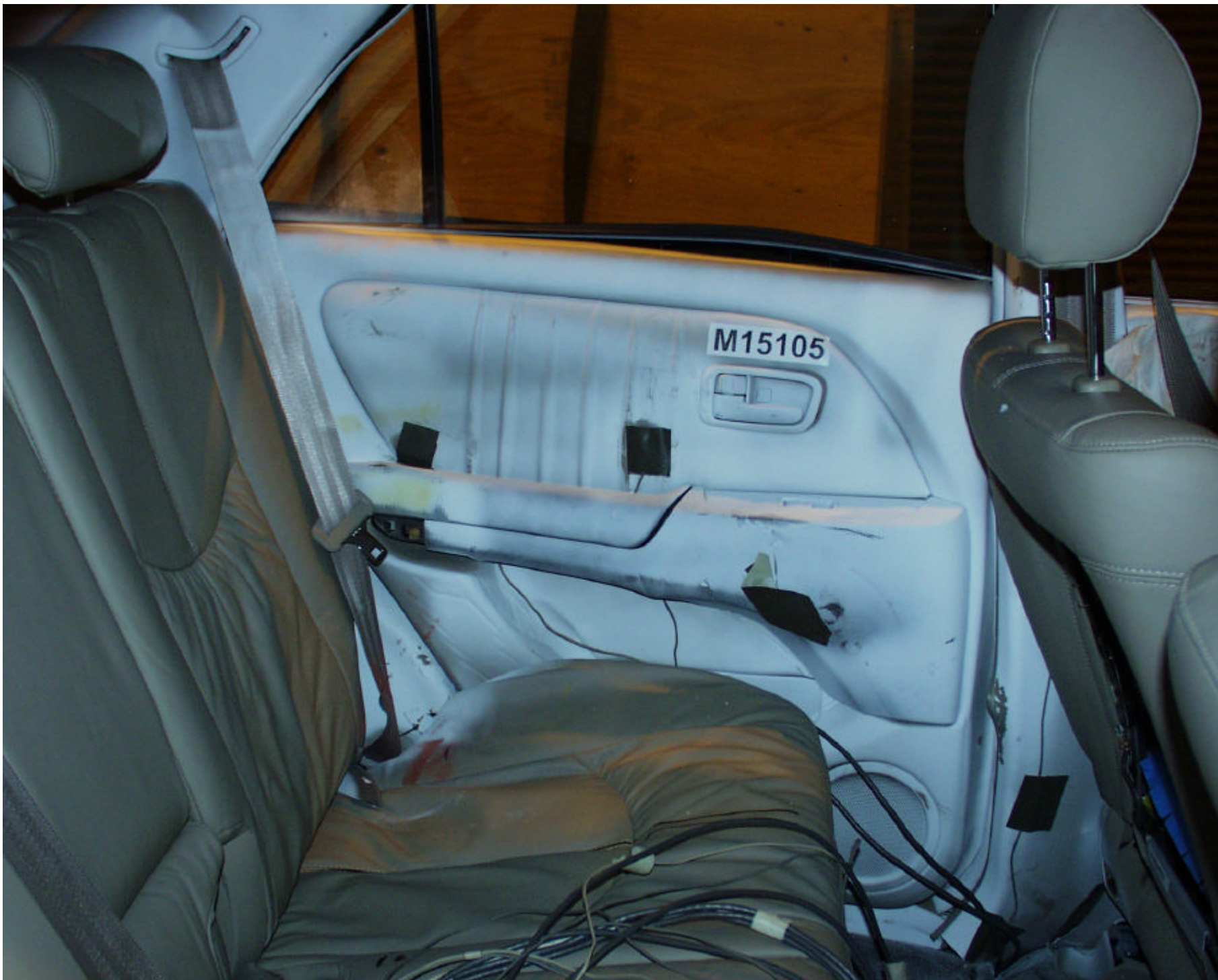
Figure A-28 POST-TEST INTERIOR OF REAR DOOR SHOWING SID IMPACT LOCATIONS
