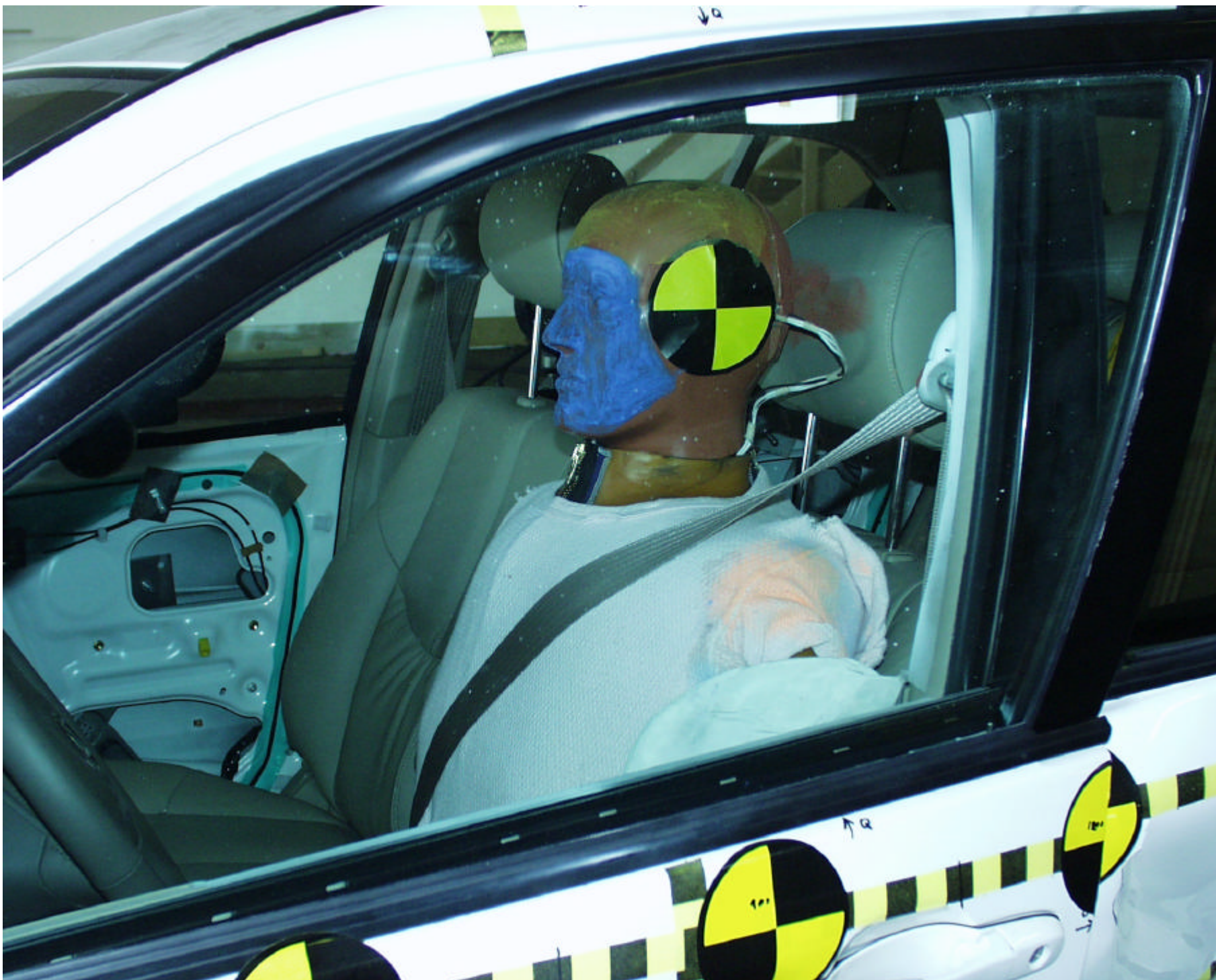
Figure A-22 POST-TEST LEFT OCCUPANT COMPARTMENT VIEW OF FRONT SID
