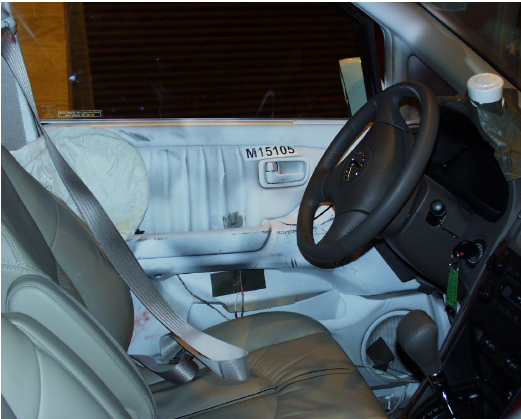
Figure A-26 POST-TEST INTERIOR OF FRONT DOOR SHOWING SID IMPACT LOCATIONS
