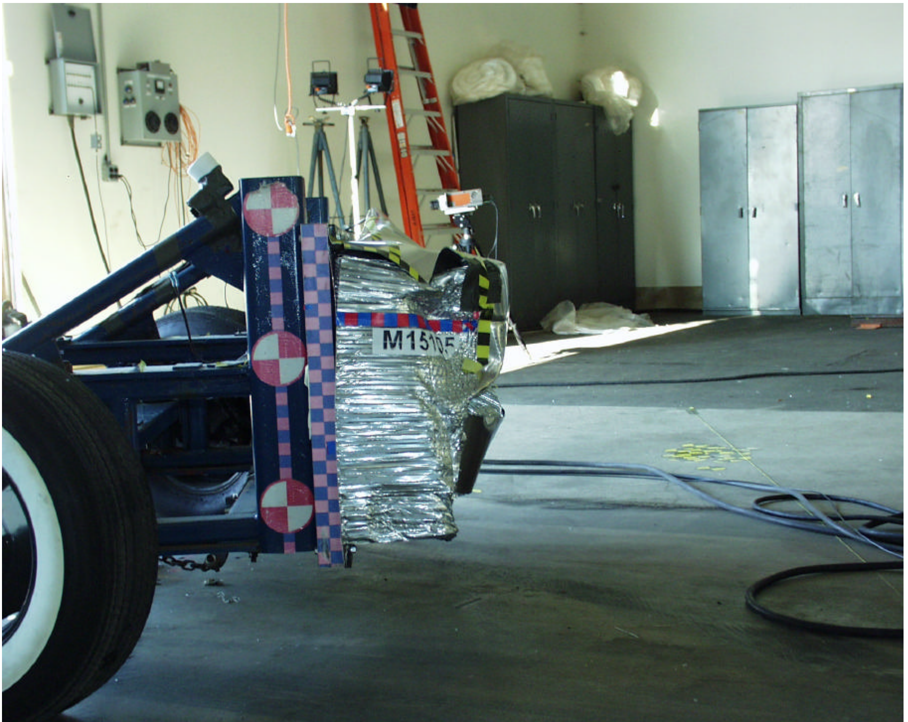
Figure A-12 POST-TEST RIGHT SIDE VIEW OF IMPACTOR FACE
