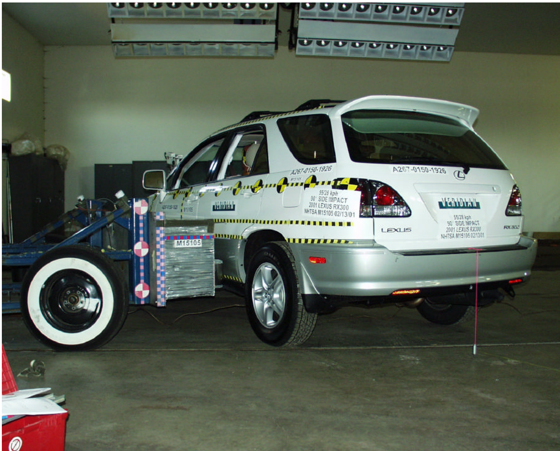
Figure A-30 PRE-TEST RIGHT SIDE VIEW OF MDB WITH IMPACTOR FACE IN POSITION
