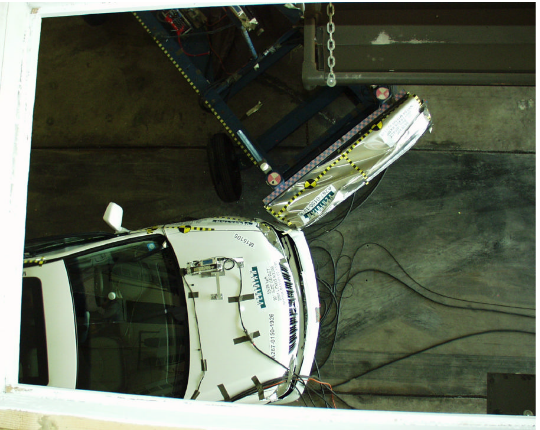
Figure A-16 POST-TEST OVERHEAD VIEW OF MDB AND VEHICLE
