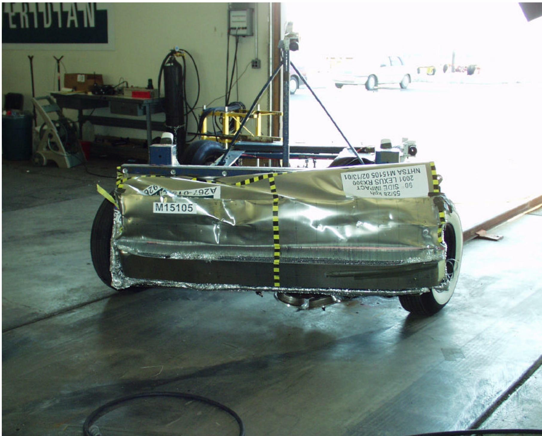
Figure A-8 POST-TEST FRONTAL VIEW OF IMPACTOR FACE
