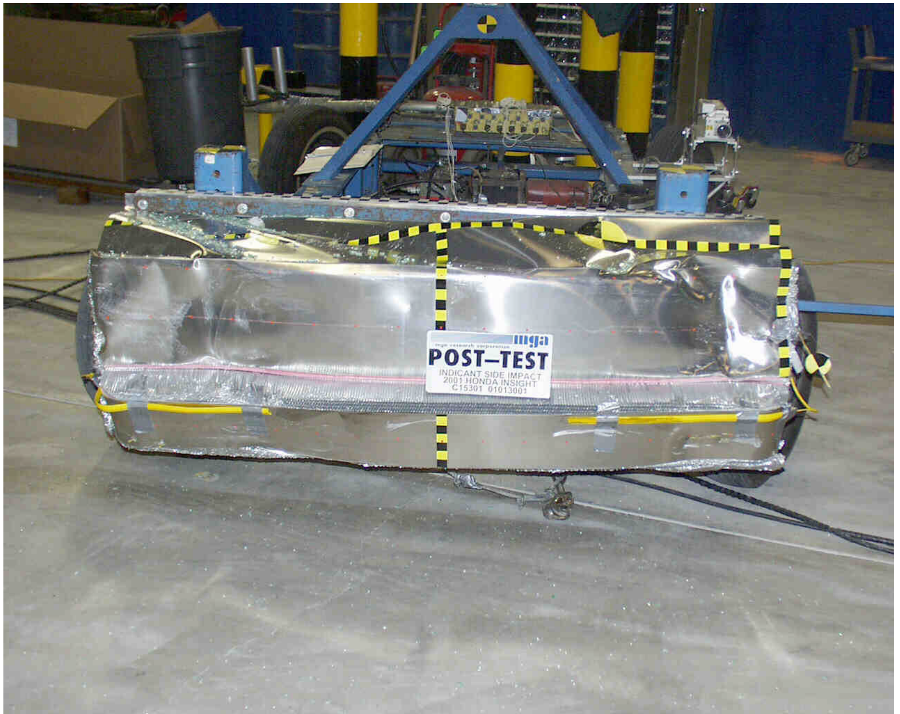
Photo No. A-16 - Post-Test MDB Front View
