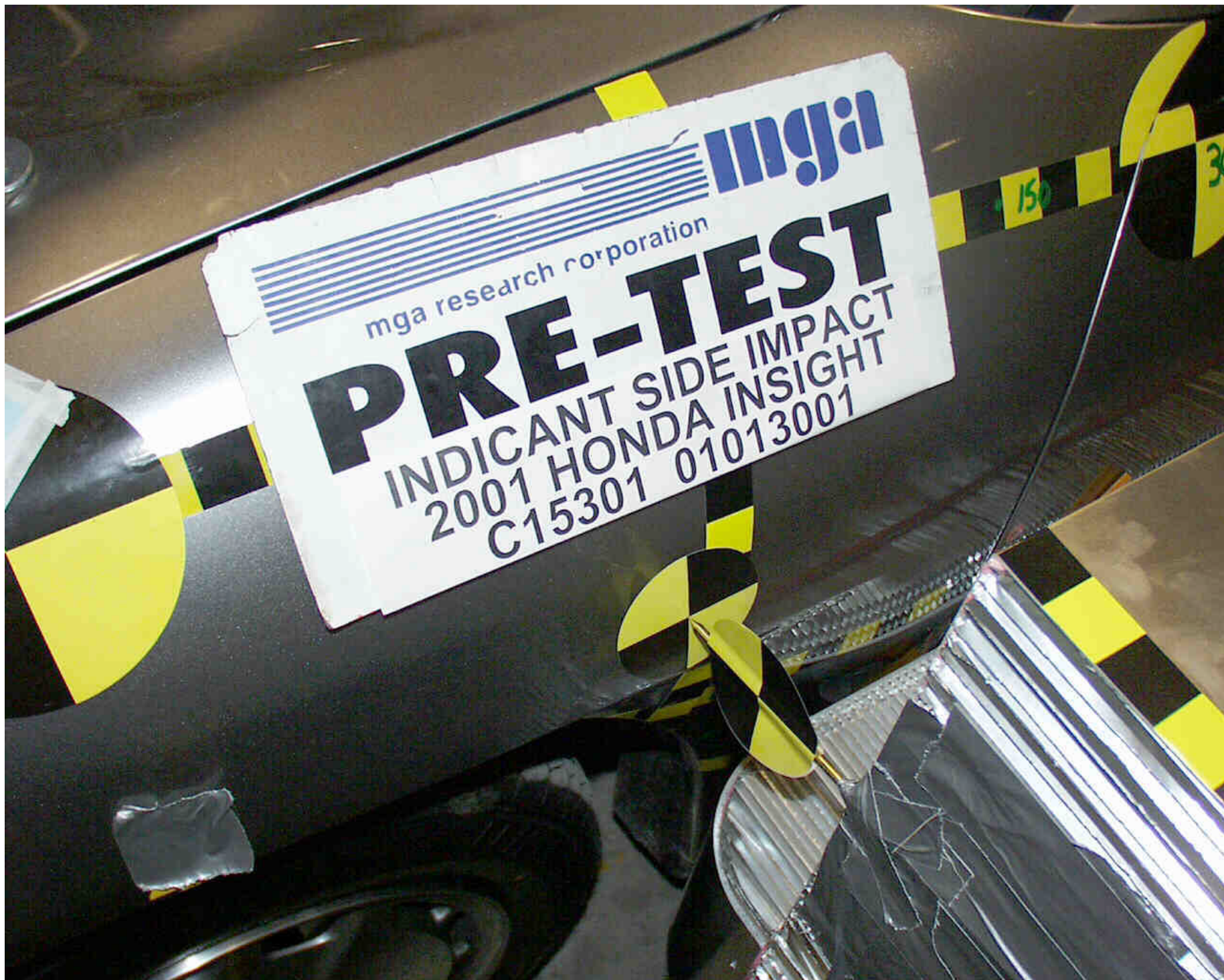
Photo No. A-31 - Pre-Test Left Front Impact Point on Vehicle
