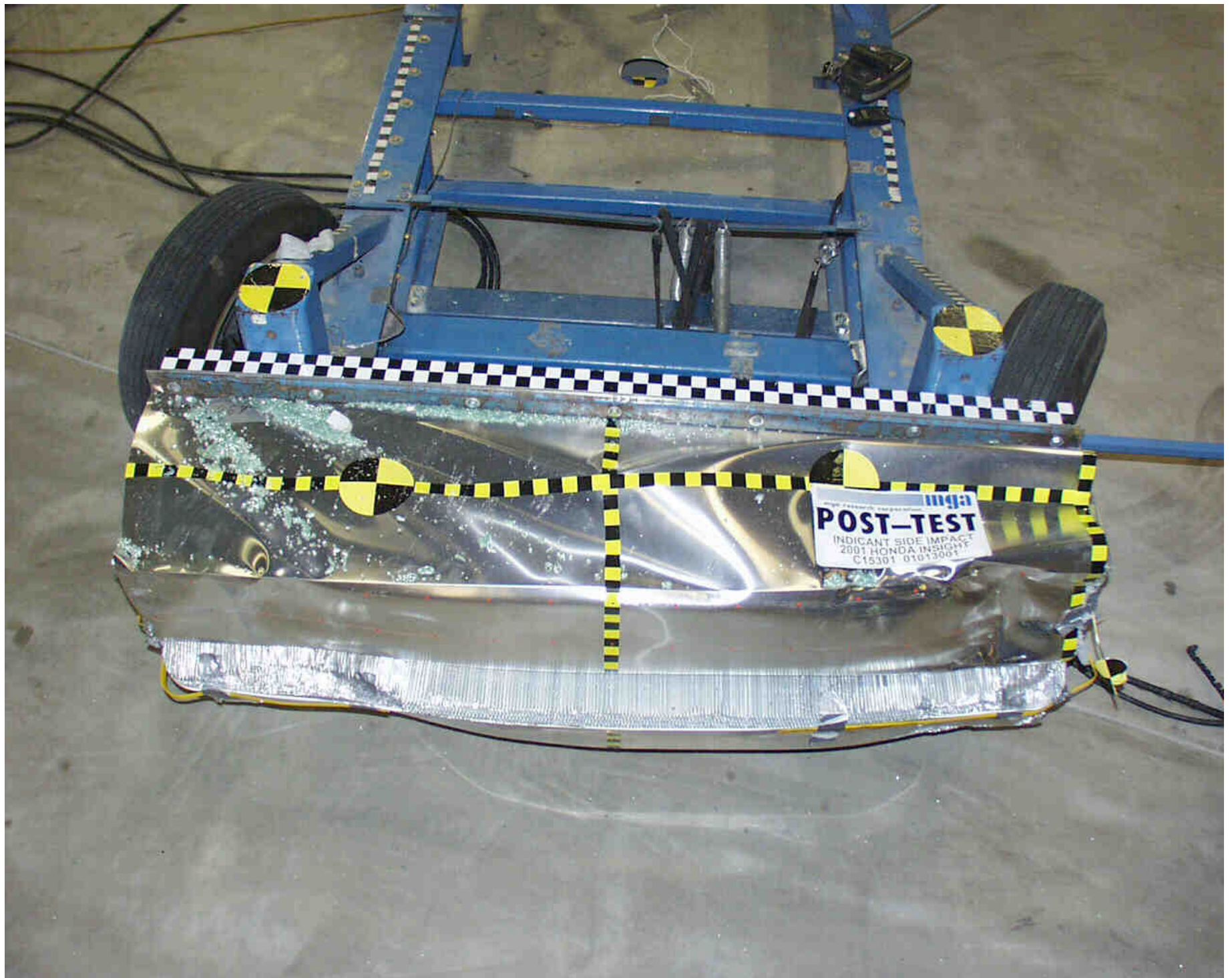
Photo No. A-14 - Post-Test MDB Top View
