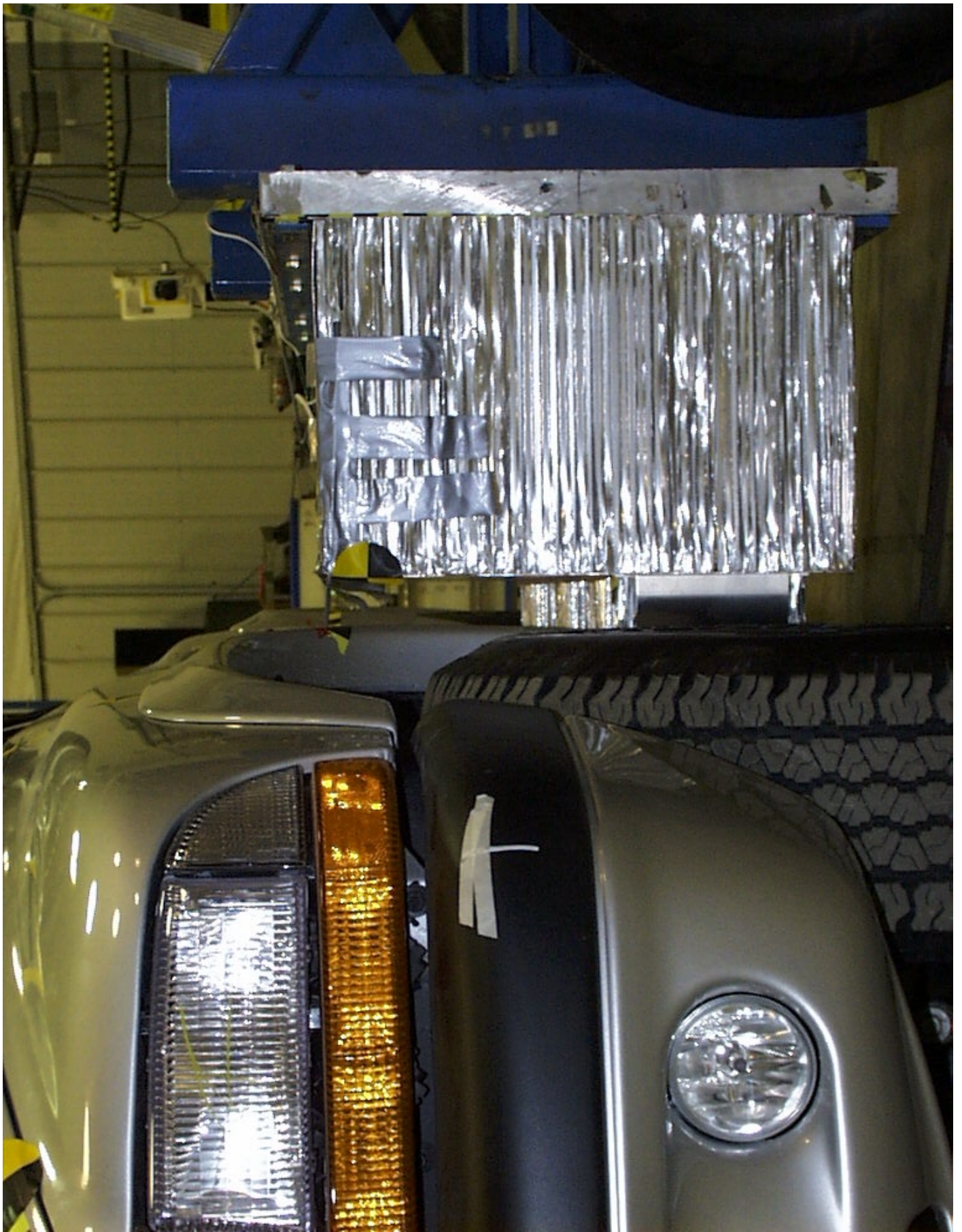
Figure A-27 PRE-TEST LEFT SIDE VIEW OF MDB WITH IMPACTOR FACE IN POSITION
