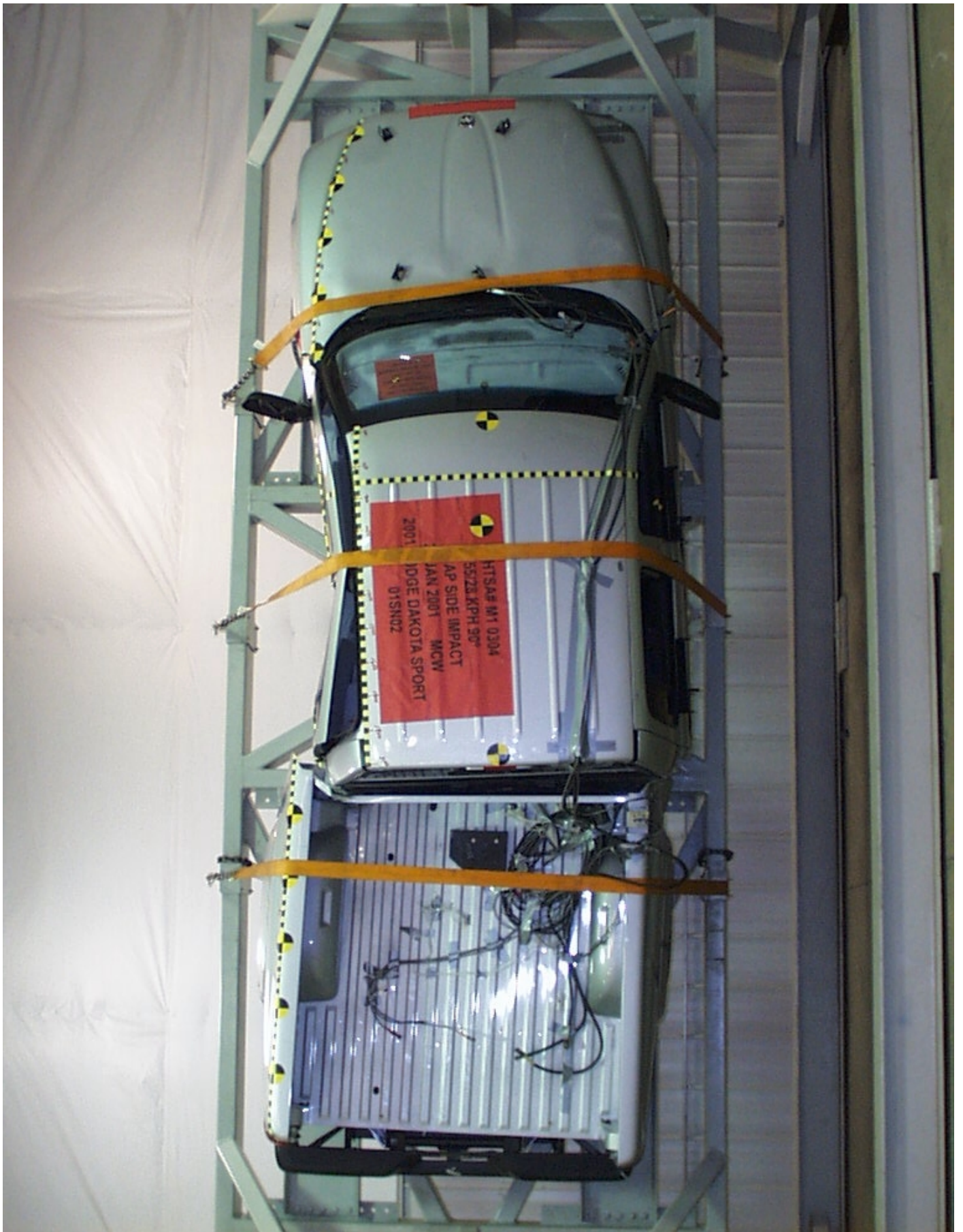
Figure A-34 ROLLOVER 270 DEGREES
