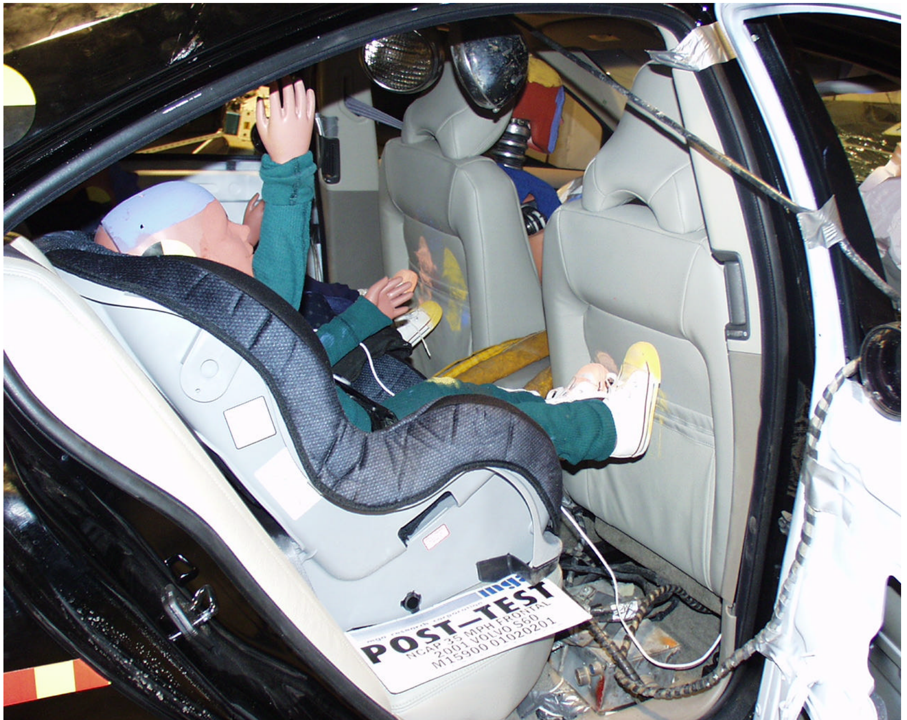
Photo 7 - Post-Test RRS 3 Year Old Right Side View (Door Open)
