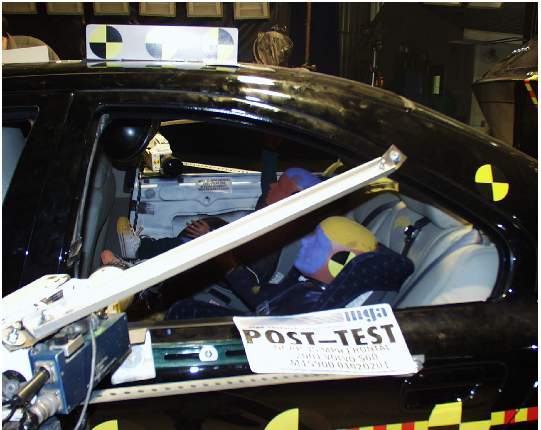
Photo 2 - Post-Test LRS 3 Year Old Left Side View
