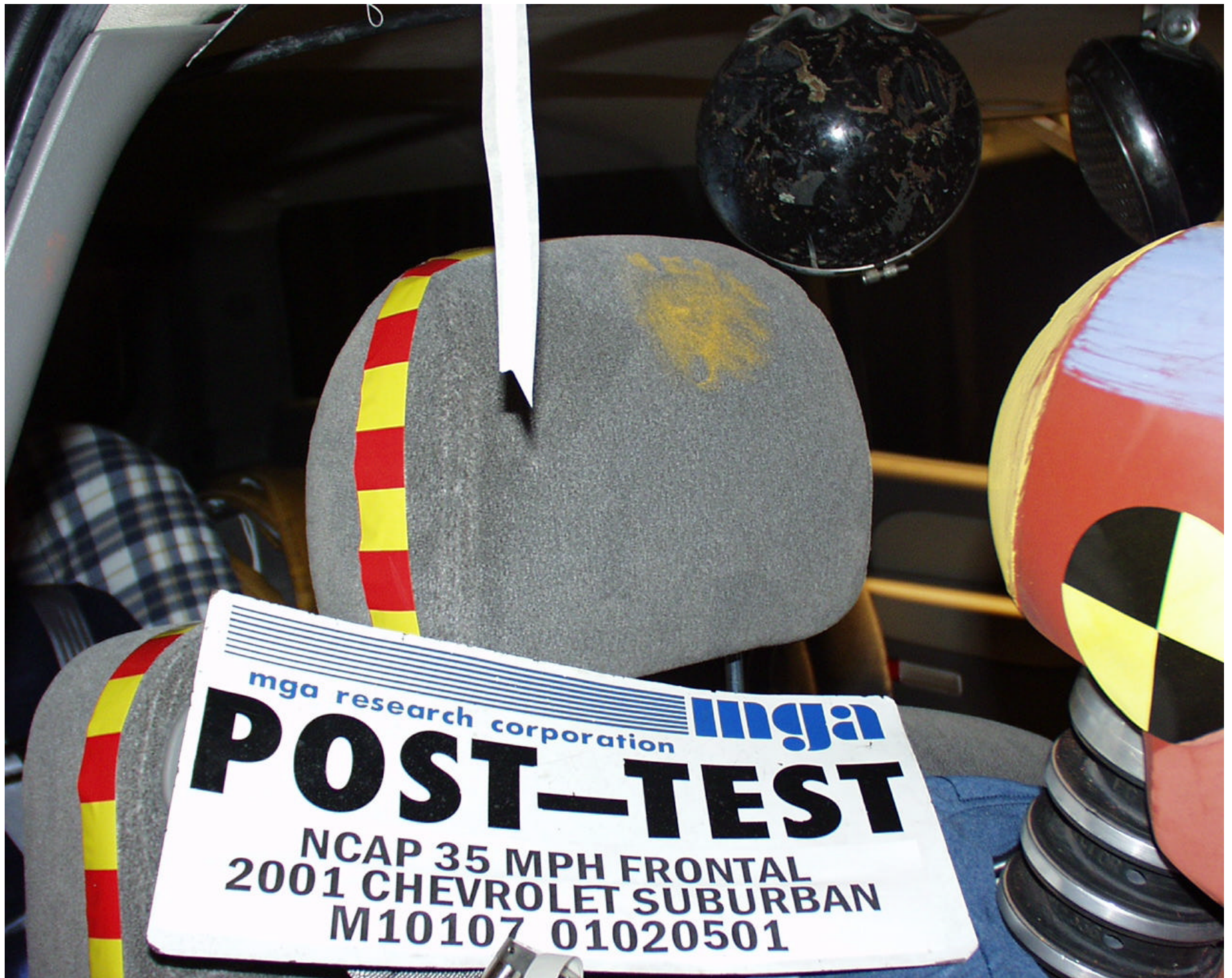
Photo No. A-40 - Post-Test Passenger Head Contact View (headrest)
