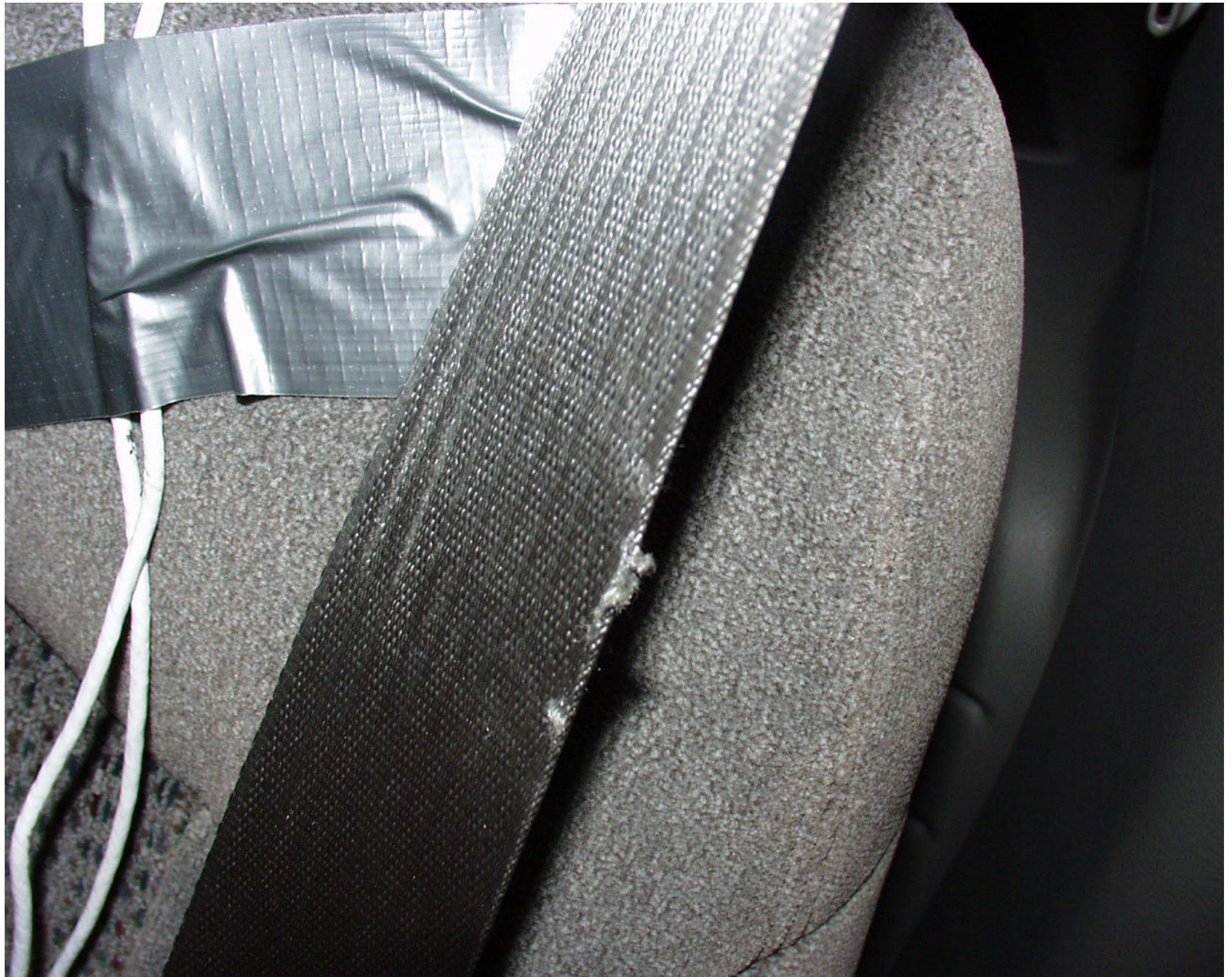
Photo 6 - LRS Vehicle Seat Belt Damage
