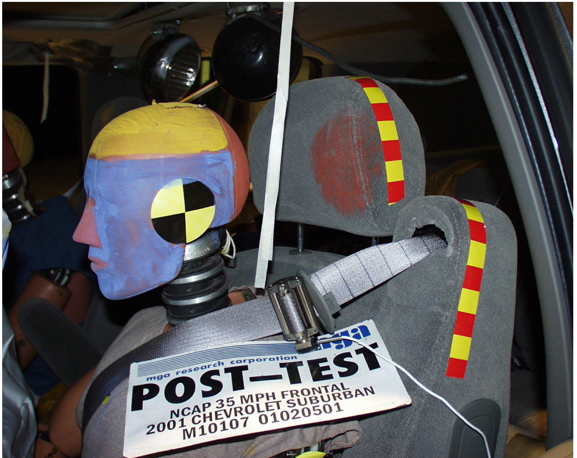
Photo No. A-28 - Post-Test Driver Head Contact View (headrest)
