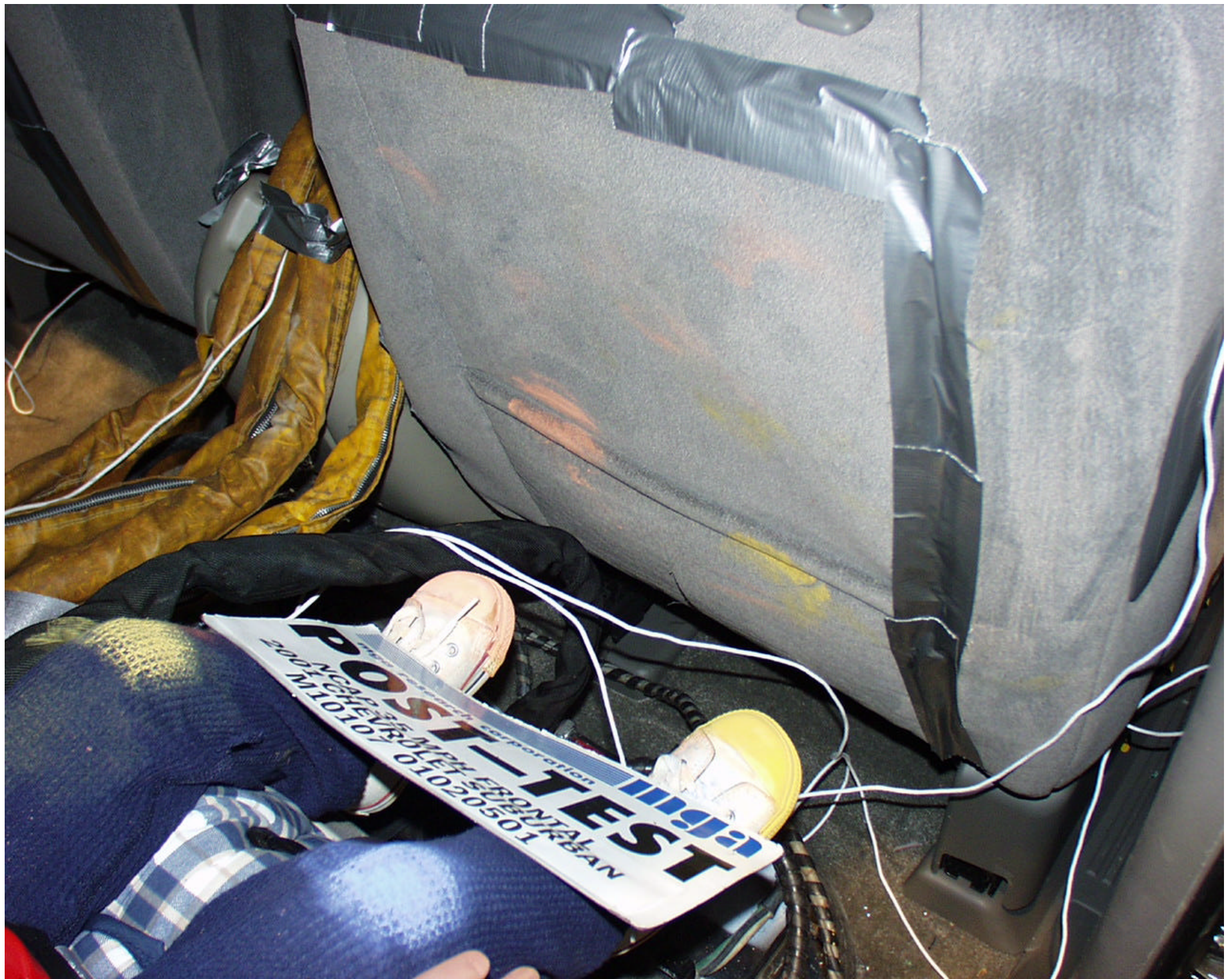
Photo 5 - Post-Test RRS 3 Year Old Right Side View Foot Contact
