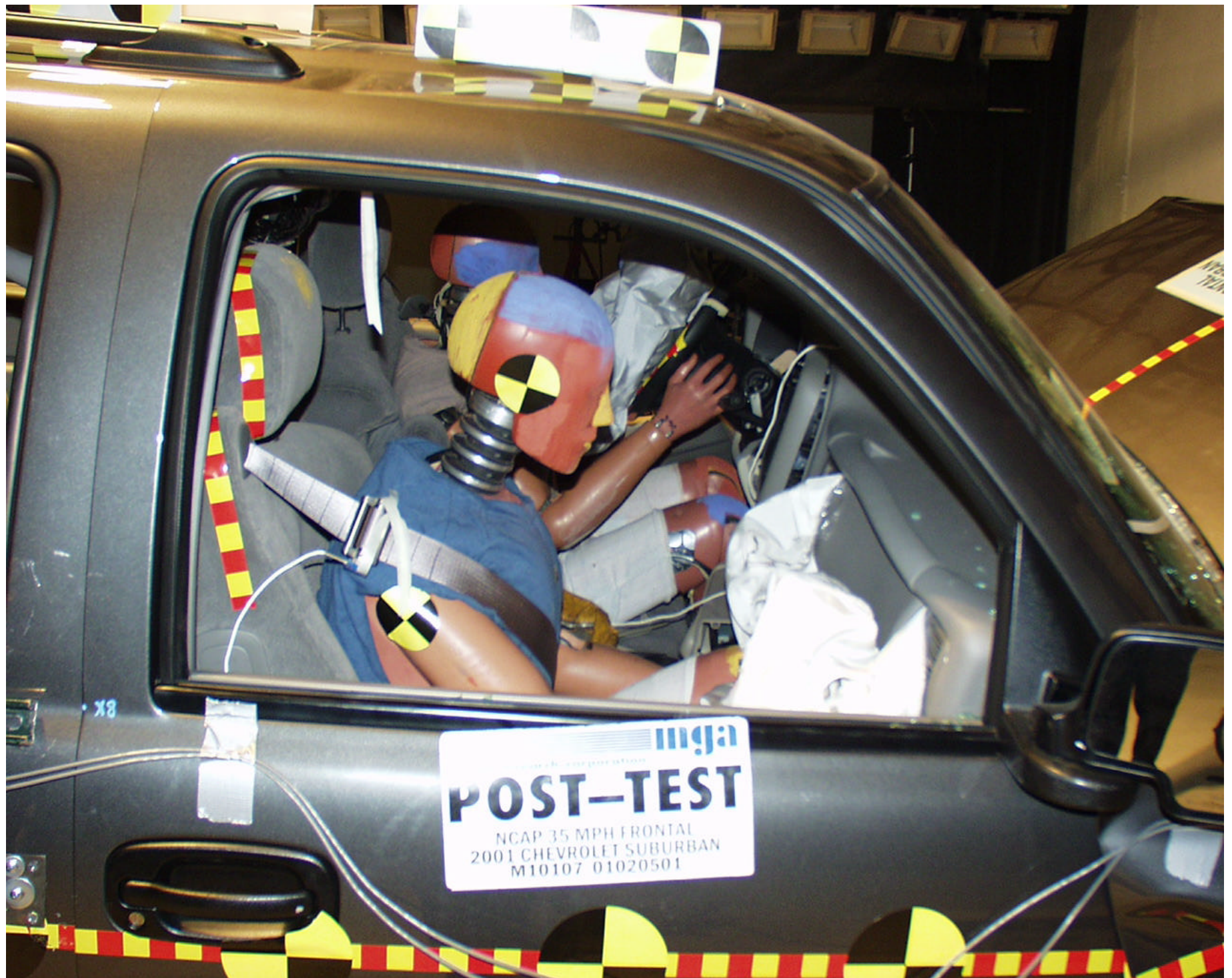
Photo No. A-32 - Post-Test Passenger Dummy Position Right Side View
