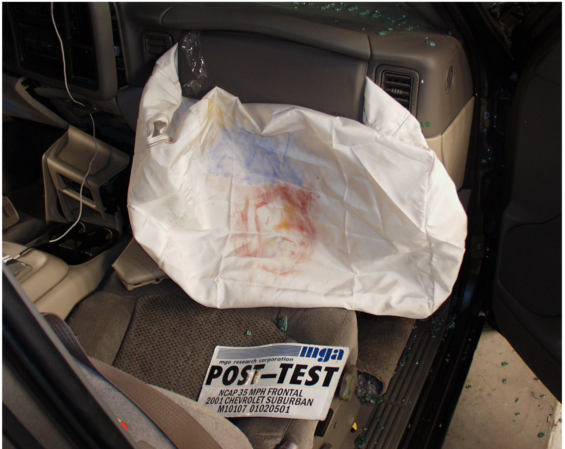
Photo No. A-39 - Post-Test Passenger Airbag Contact
