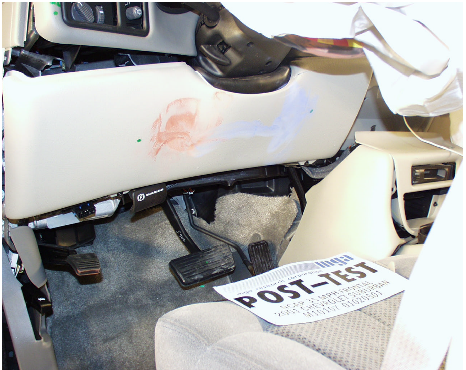
Photo No. A-29 - Post-Test Driver Knee Contact View
