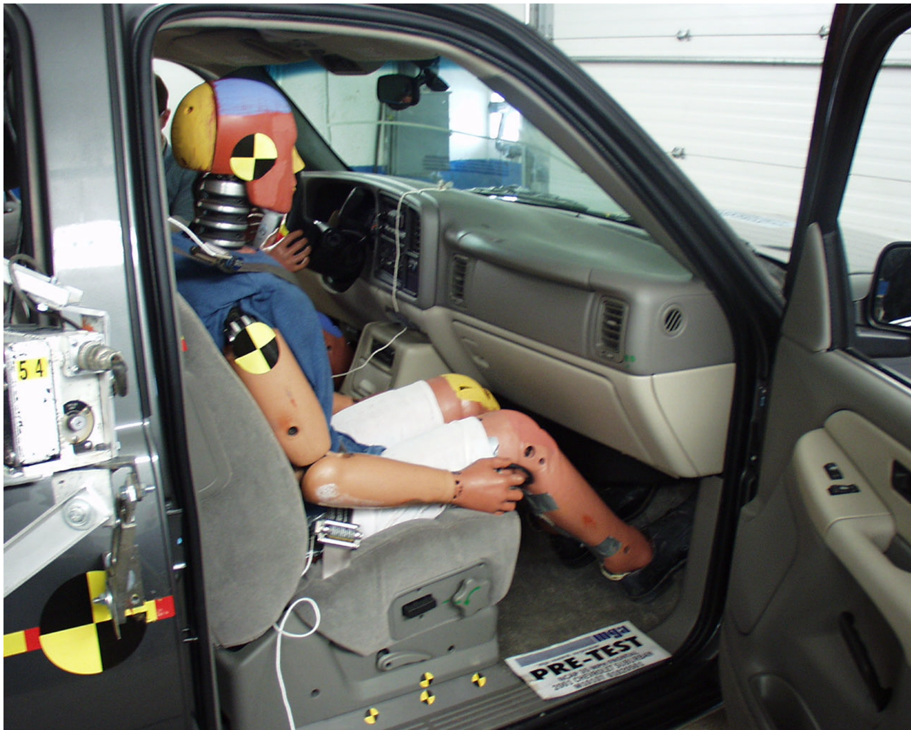
Photo No. A-33 - Pre-Test Passenger Dummy Position Right Side View (Door Open)
