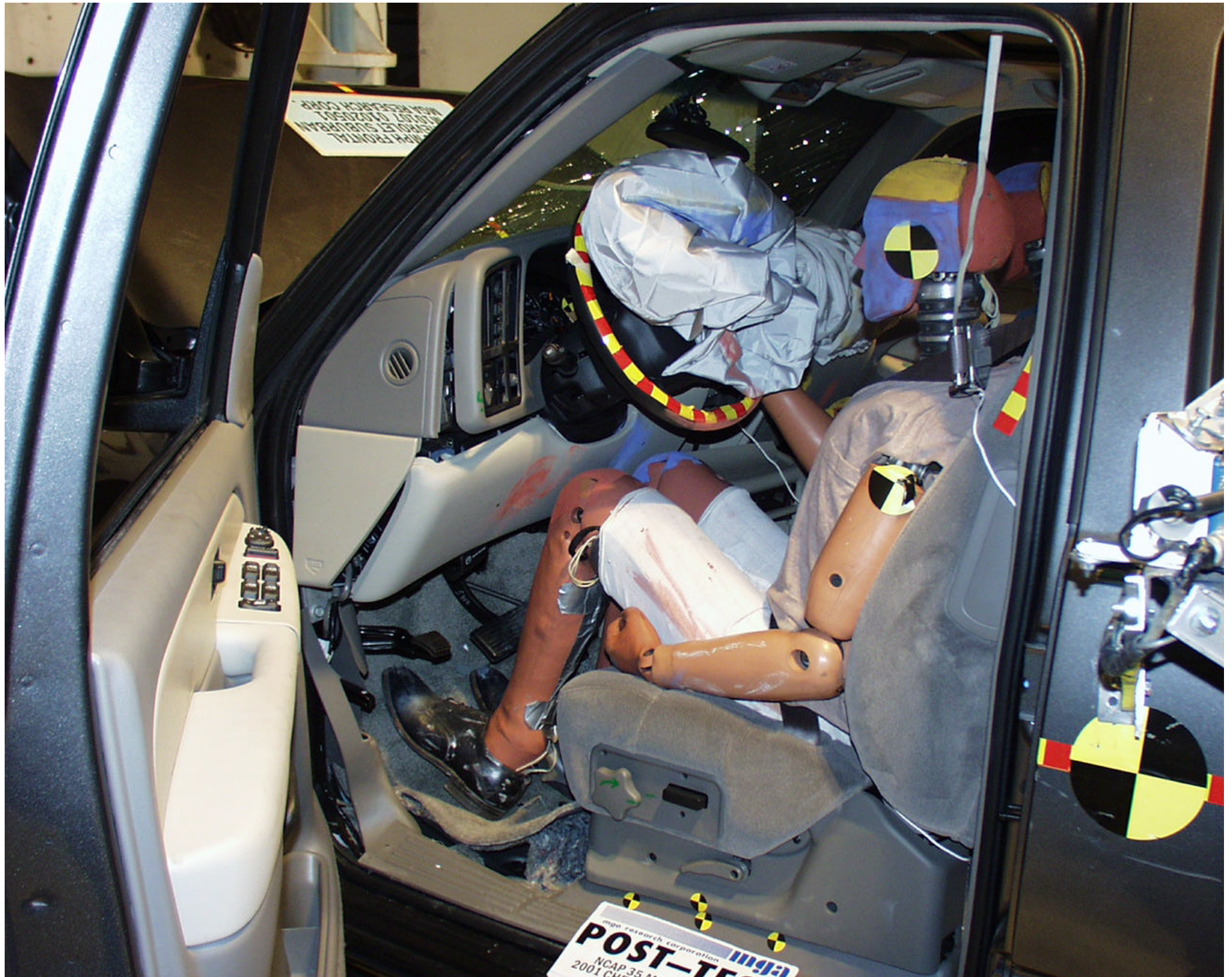
Photo No. A-22 - Post-Test Driver Dummy Position Left Side View (Door Open)
