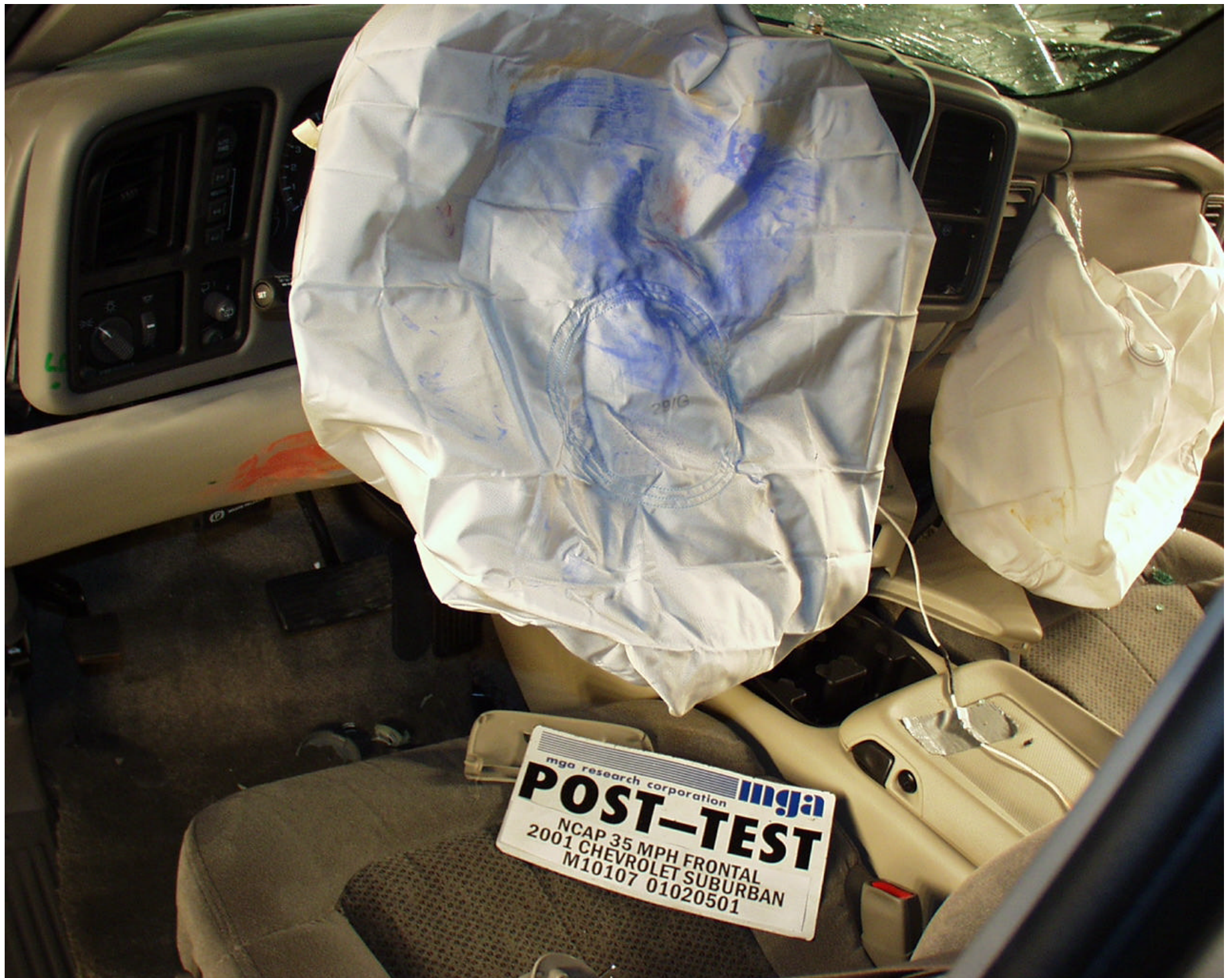
Photo No. A-27 - Post-Test Driver Airbag Contact
