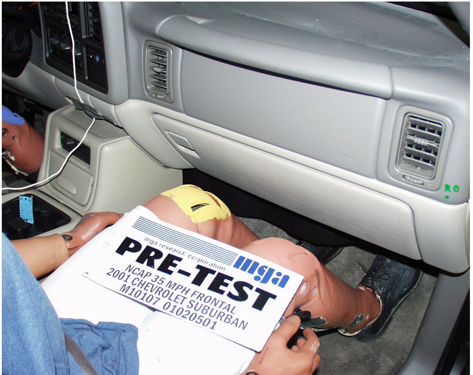
Photo No. A-37 - Pre-Test Passenger Dummy Knee Position
