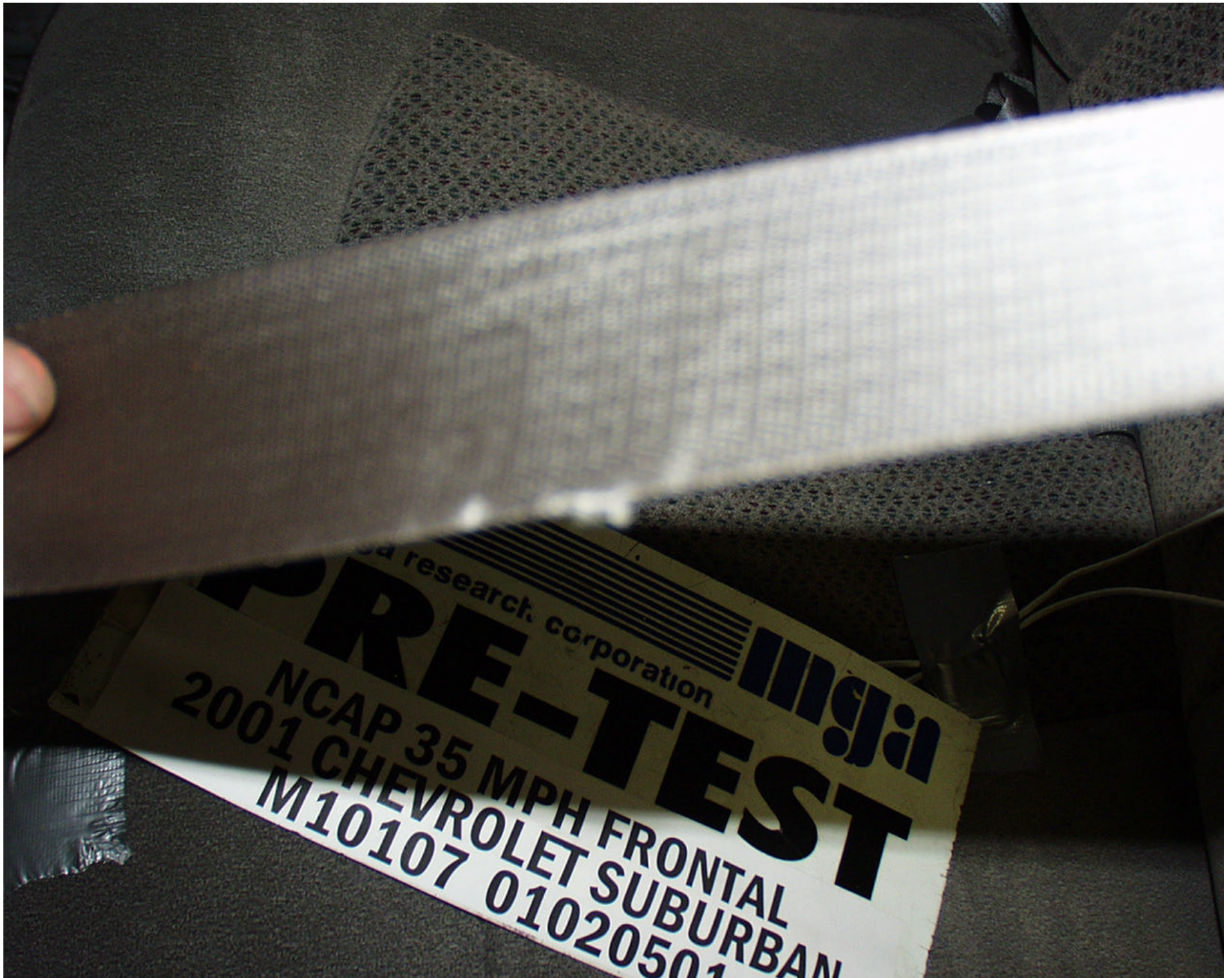
Photo 7 - LRS Vehicle Seat Belt Damage
