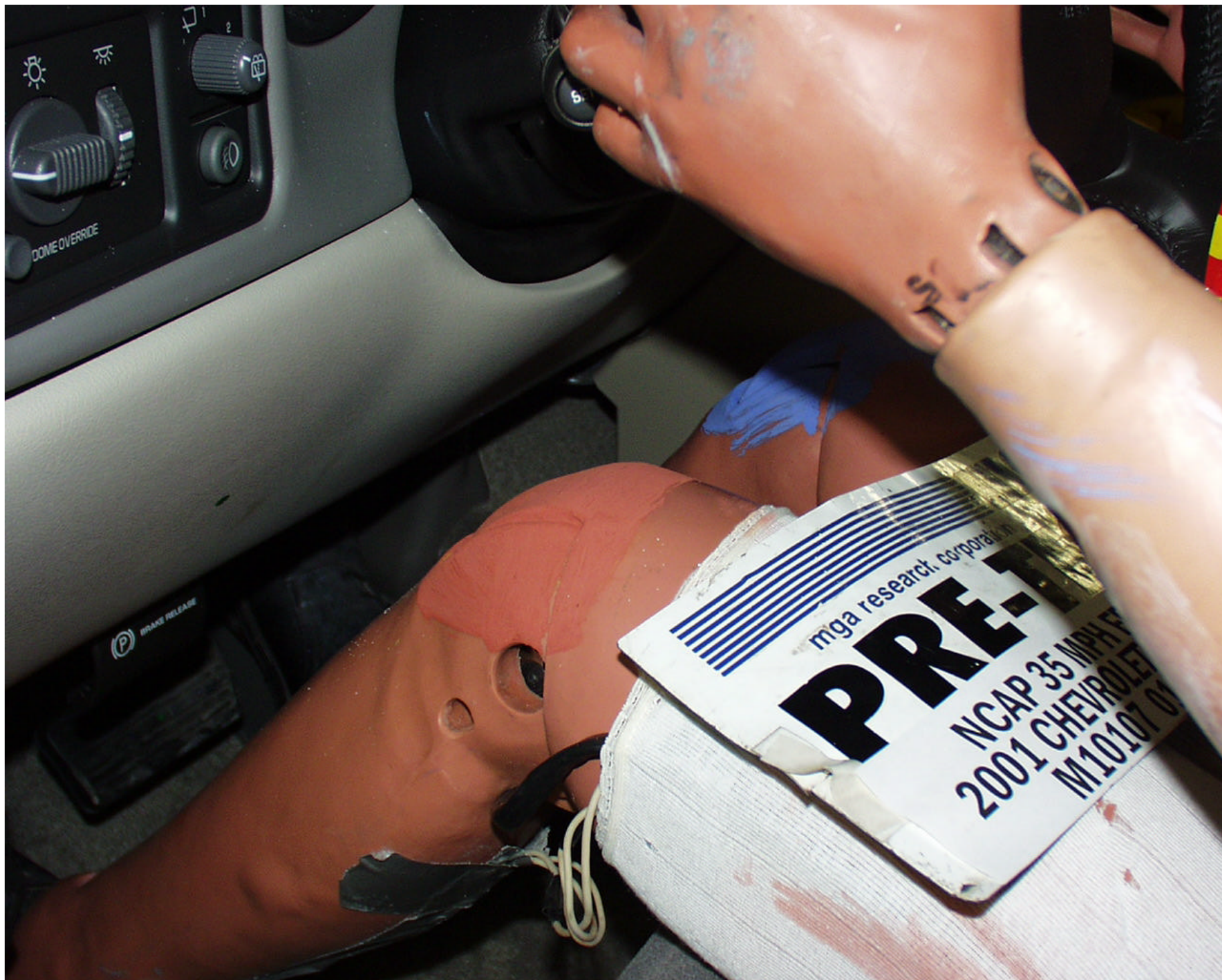
Photo No. A-25 - Pre-Test Driver Dummy Knee Position
