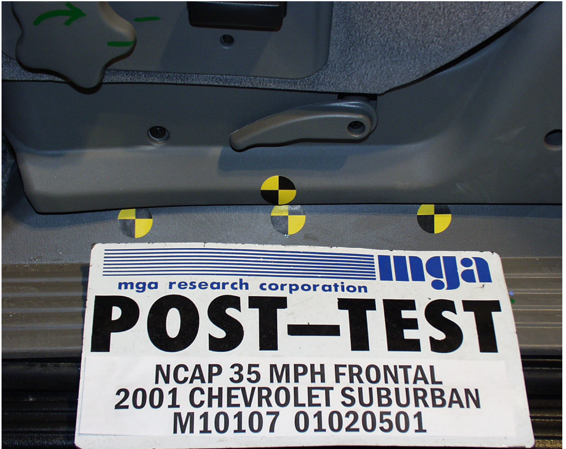
Photo No. A-24 - Post-Test Driver Seat Position View
