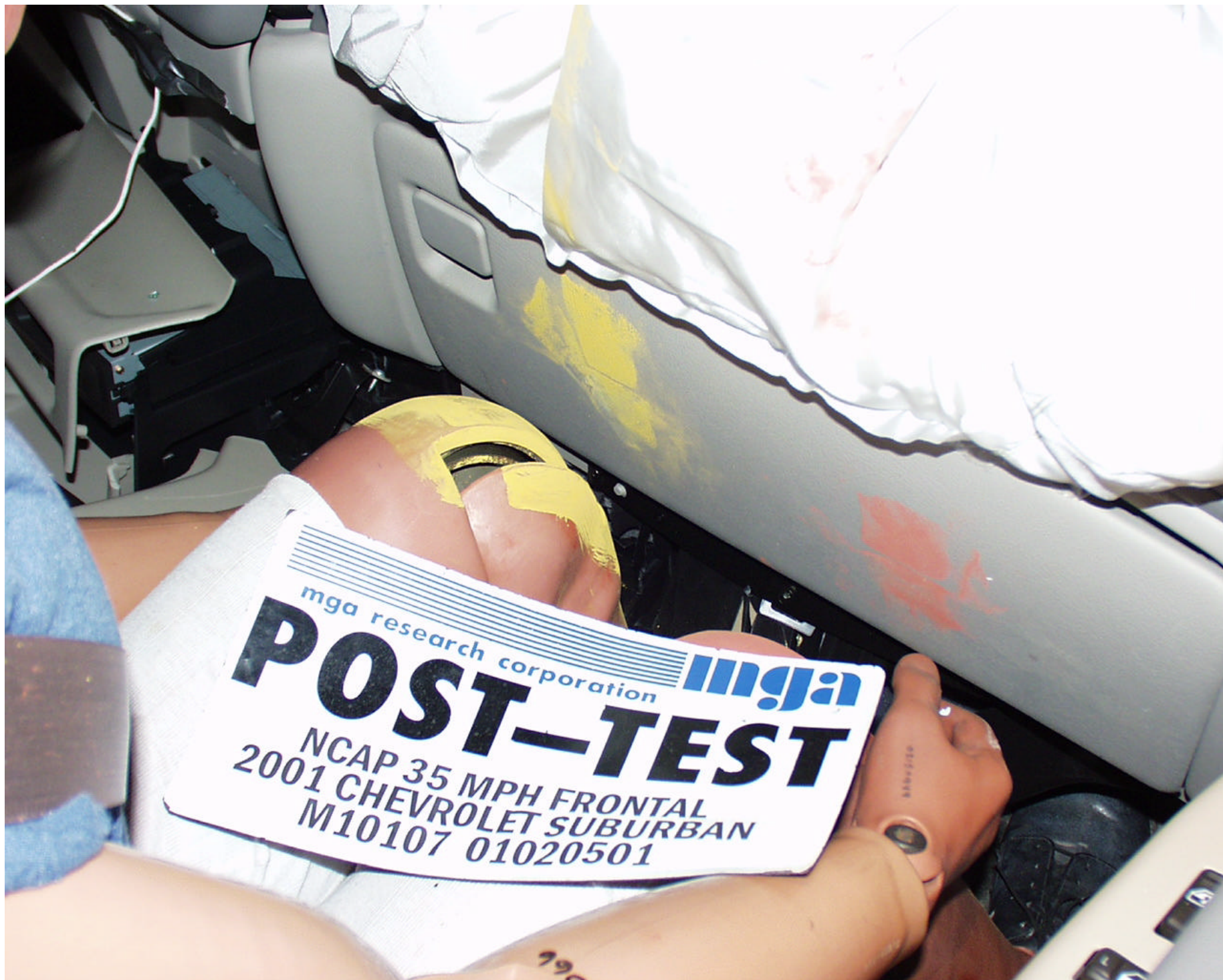
Photo No. A-38 - Post-Test Passenger Dummy Knee Position
