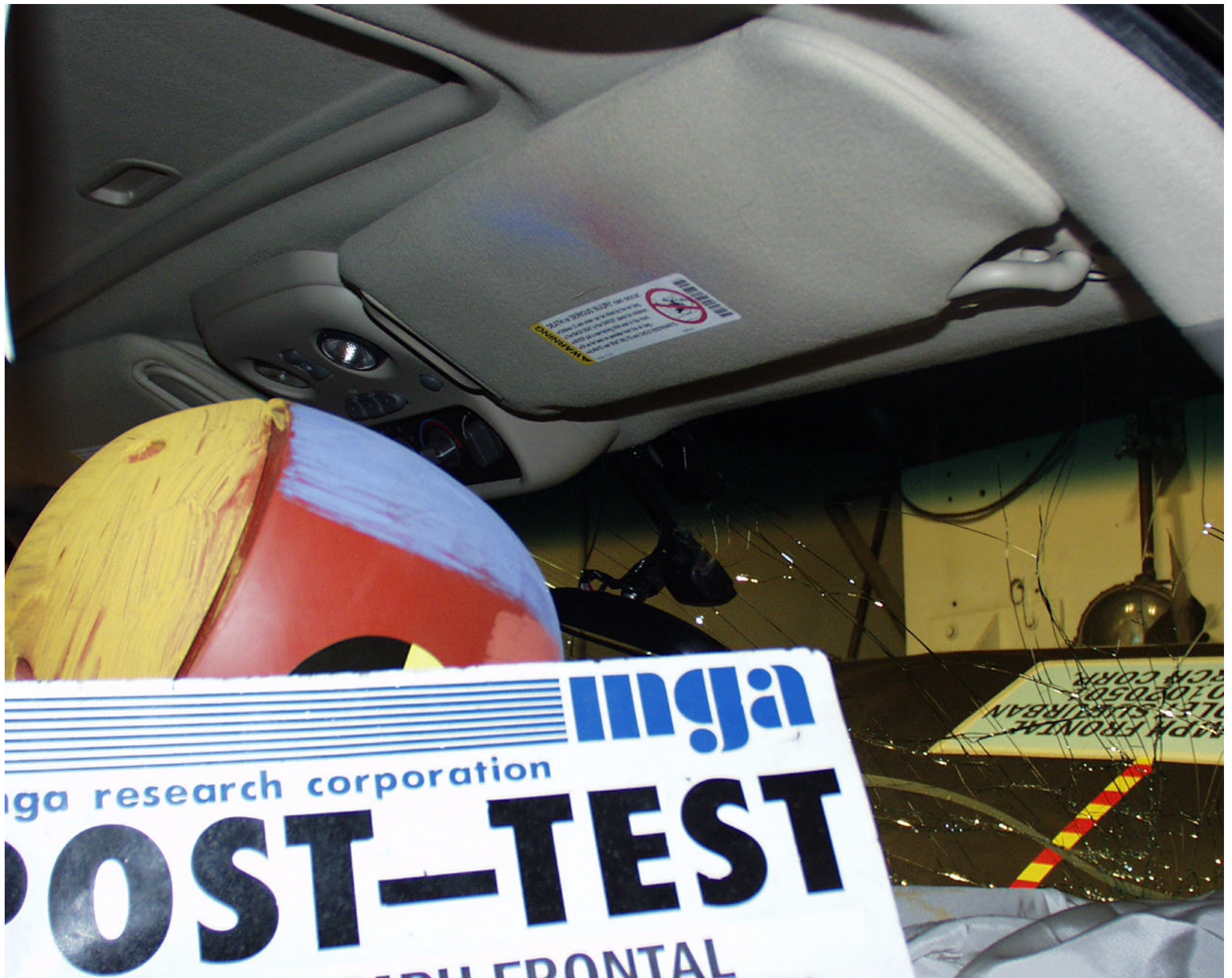
Photo No. A-41 - Post-Test Passenger Head Contact View (visor)
