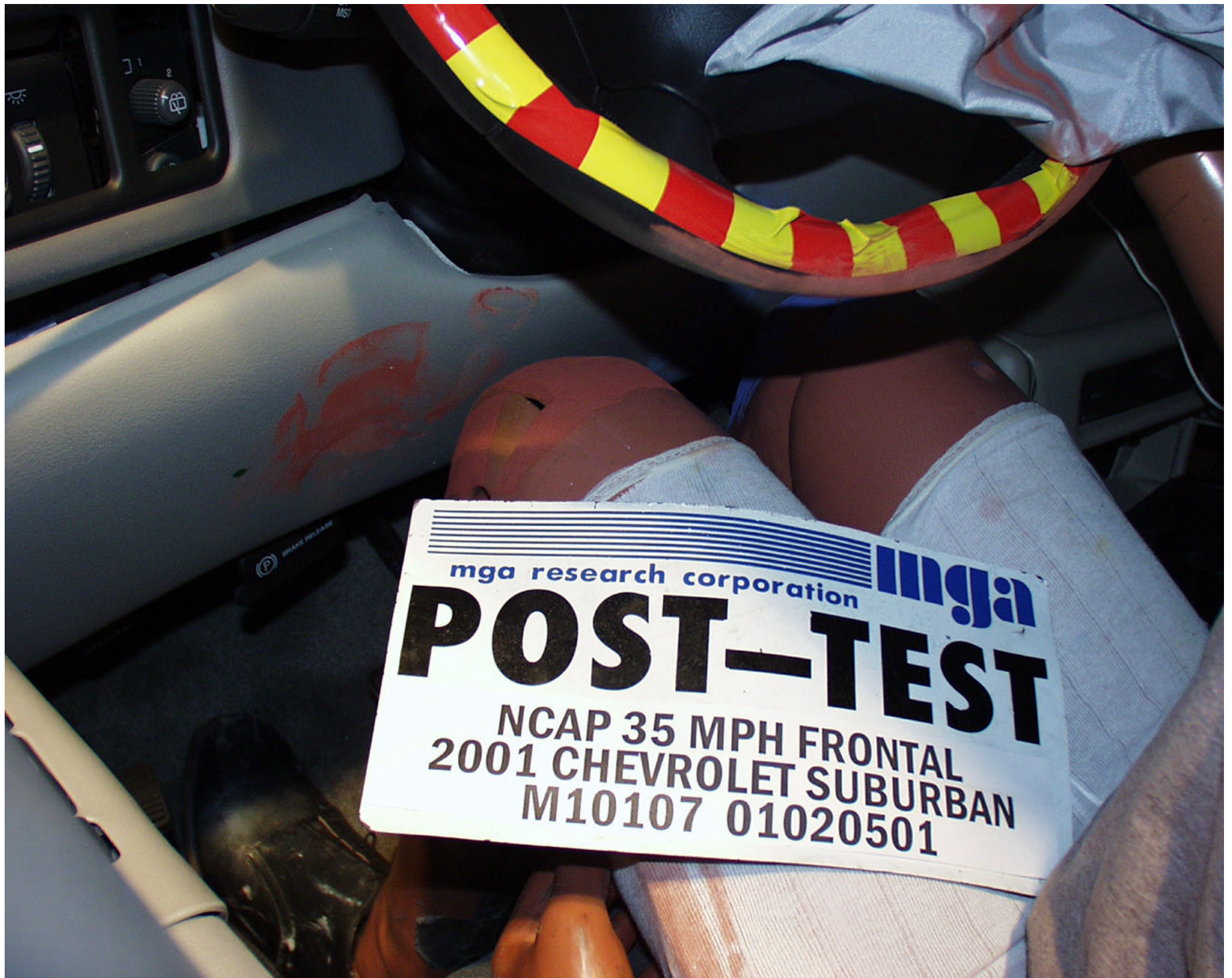
Photo No. A-26 - Post-Test Driver Dummy Knee Position
