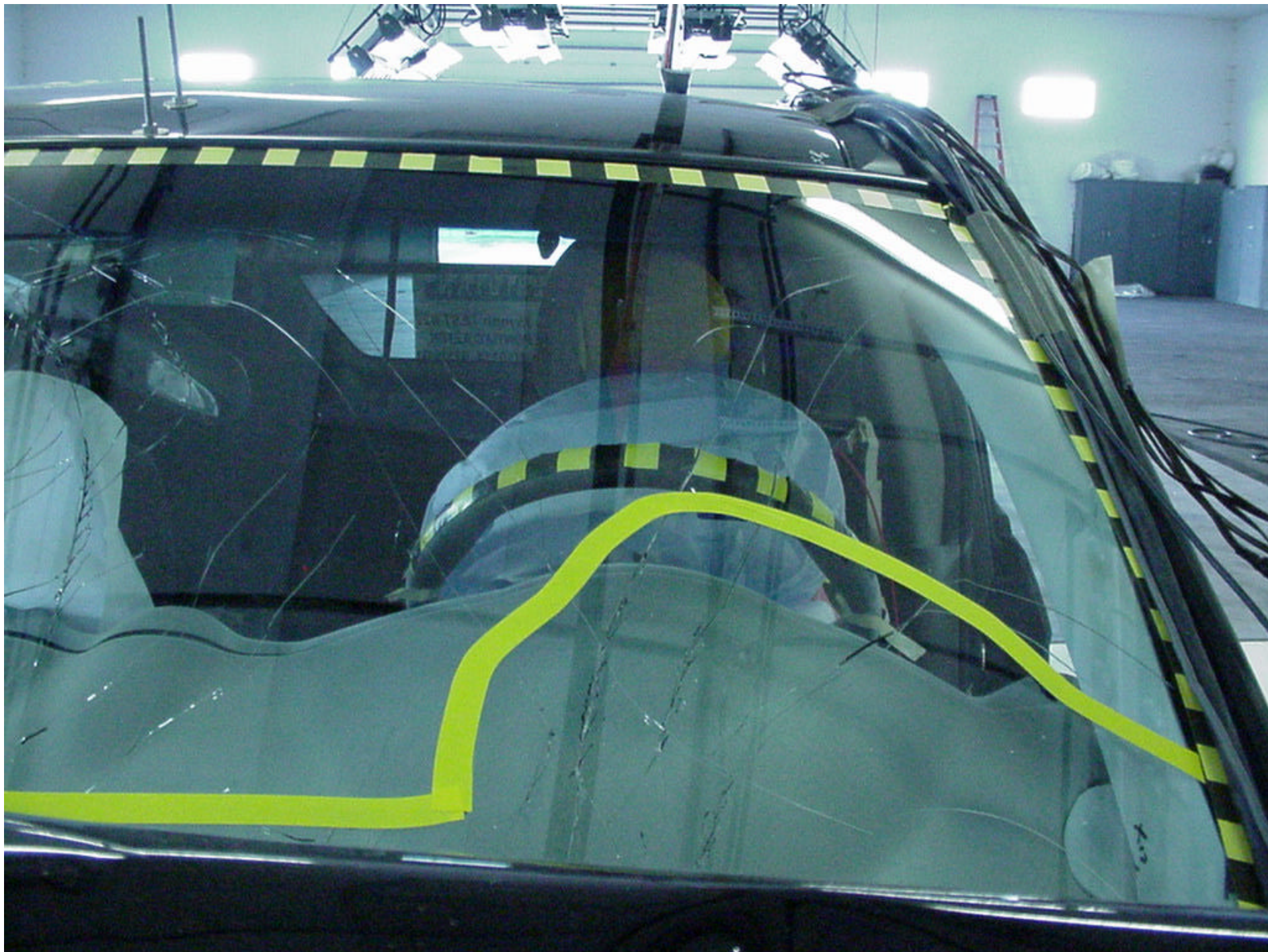
Figure A-31 POST-TEST DRIVER HEAD LOCATION
