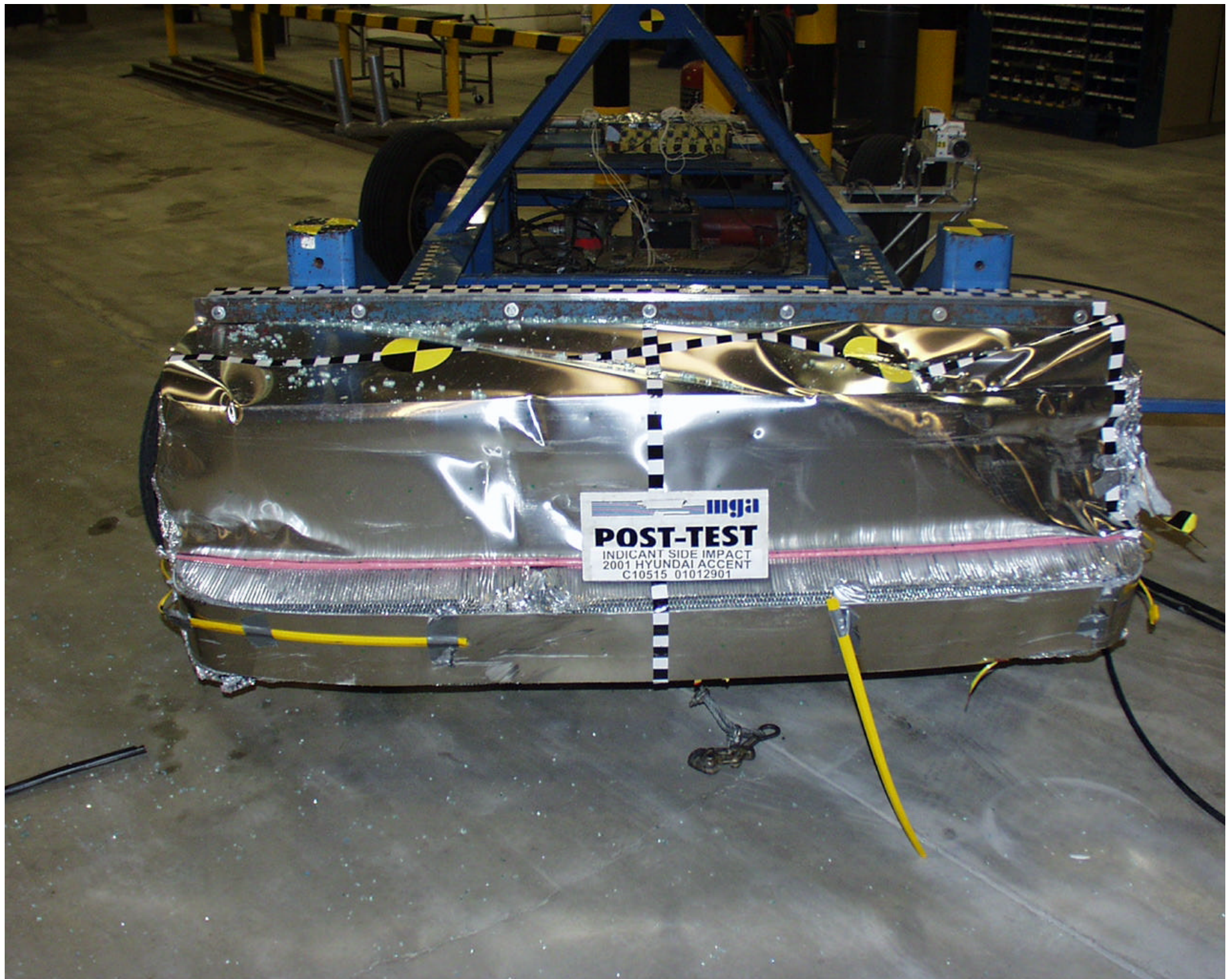
Photo No. A-15 - Post-Test MDB Front View
