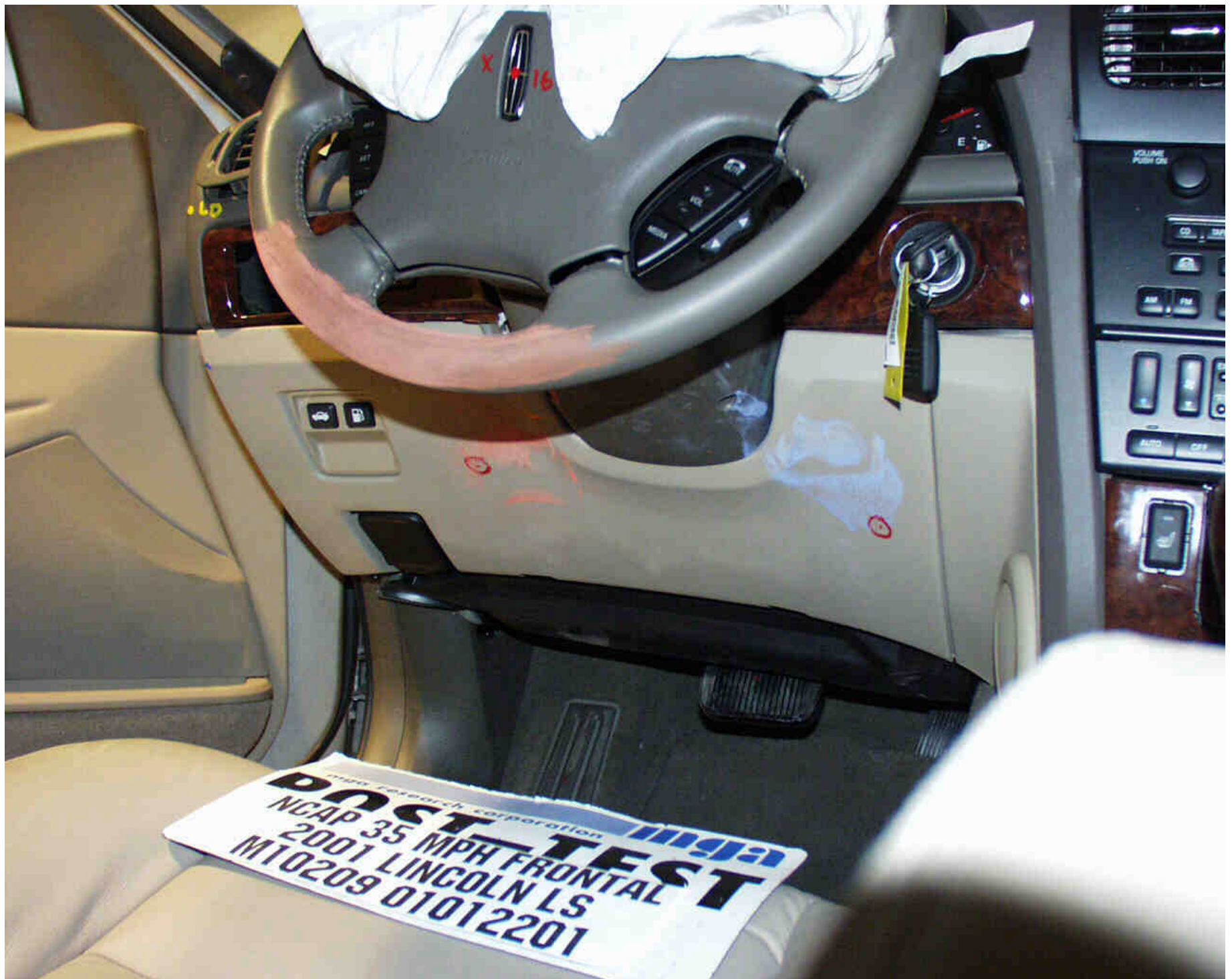
Photo No. A-30 - Post-Test Driver Knee Contact View
