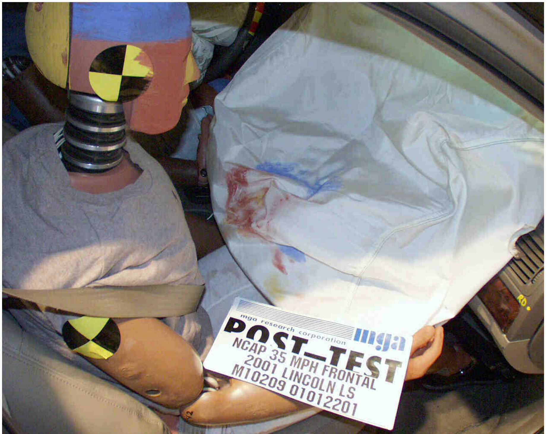
Photo No. A-41 - Post-Test Passenger Airbag Contact
