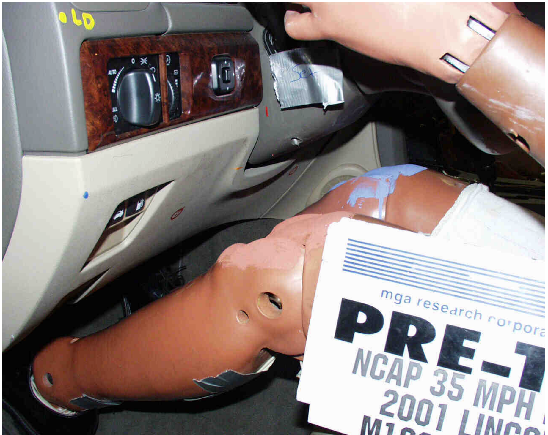
Photo No. A-27 - Pre-Test Driver Dummy Knee Position
