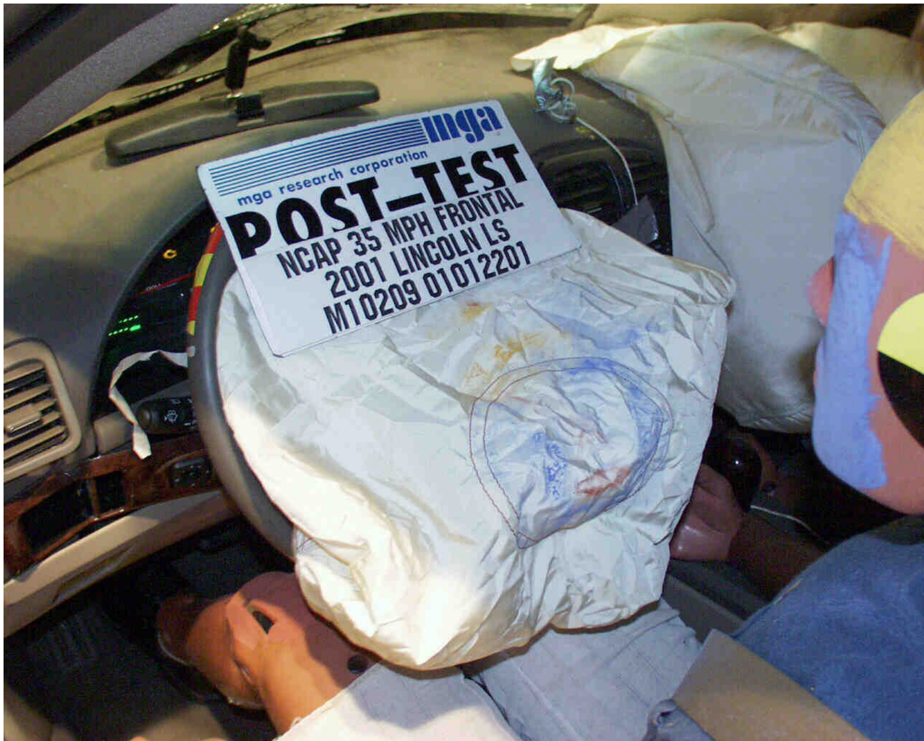
Photo No. A-29 - Post-Test Driver Airbag Contact
