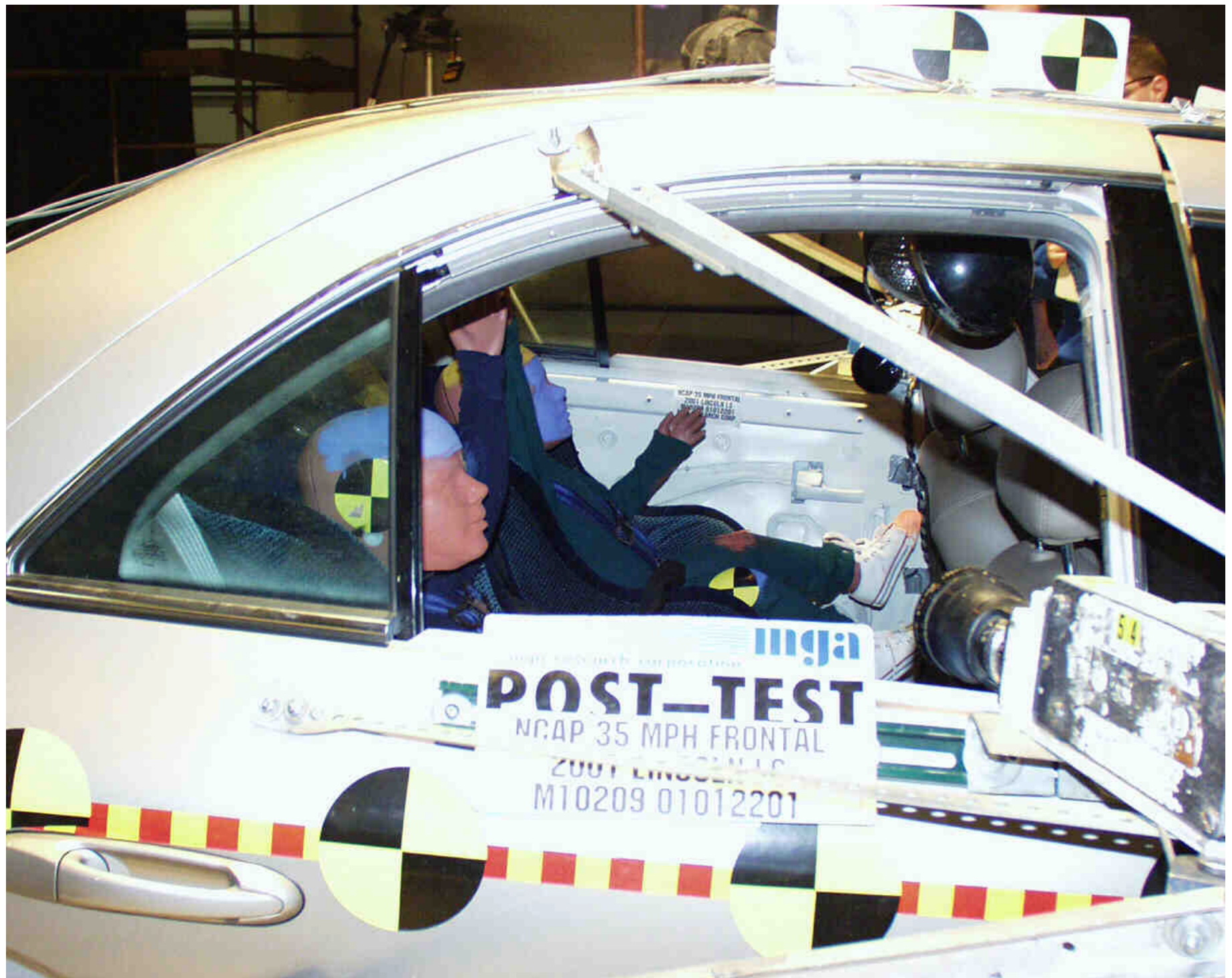
Photo 6 - Post-Test RRS 3 Year Old Right Side View
