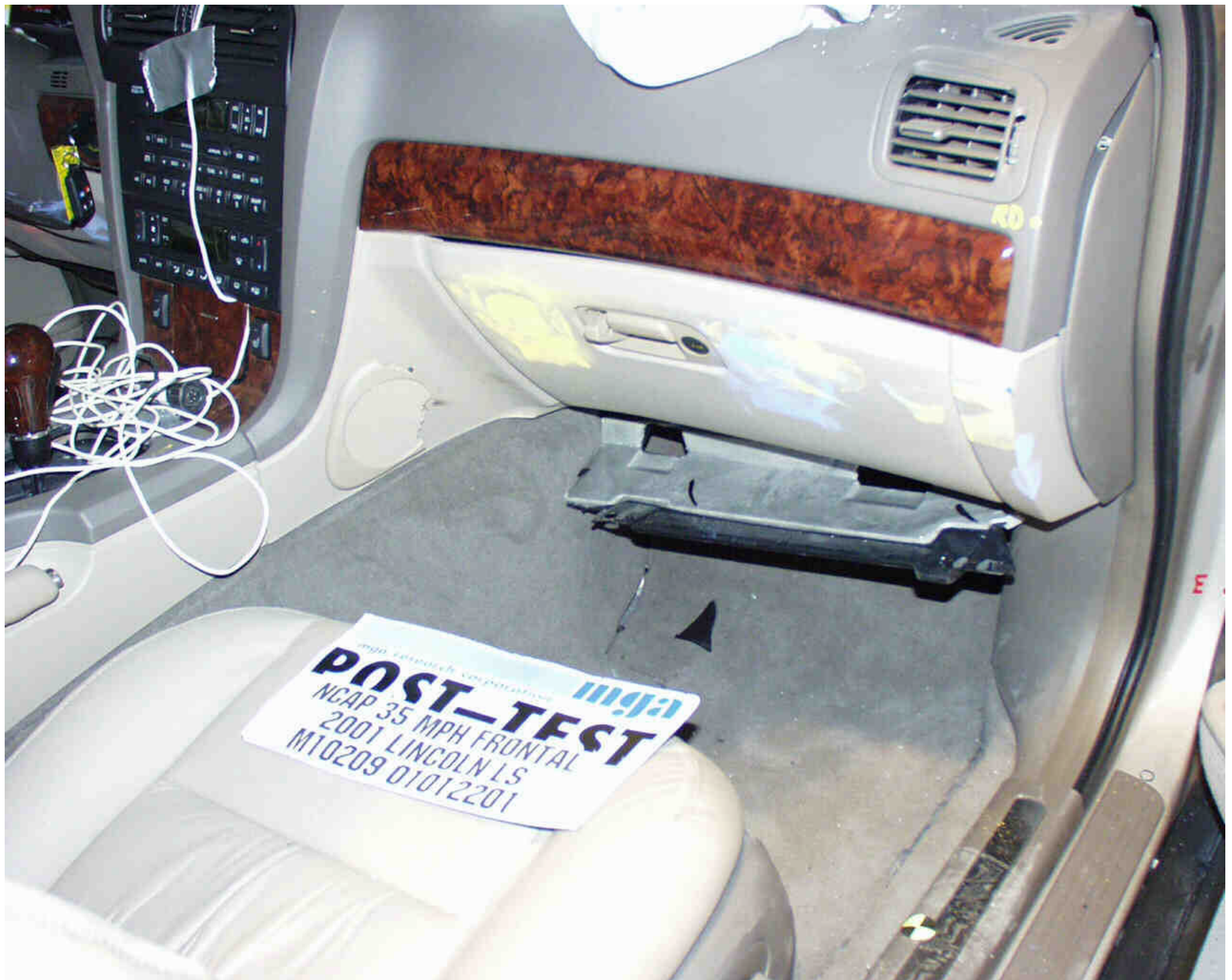
Photo No. A-42 - Post-Test Passenger Knee Contact View
