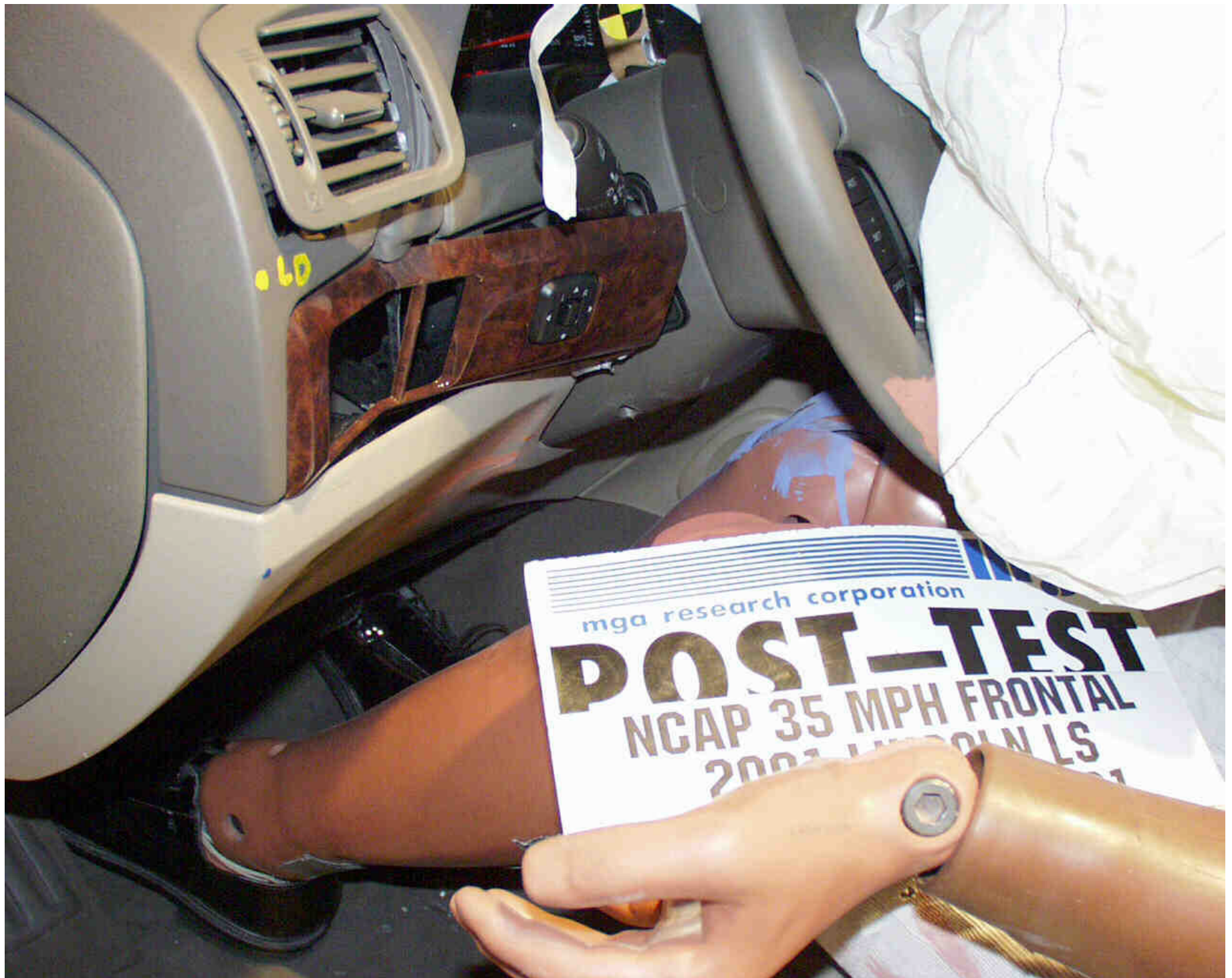
Photo No. A-28 - Post-Test Driver Dummy Knee Position
