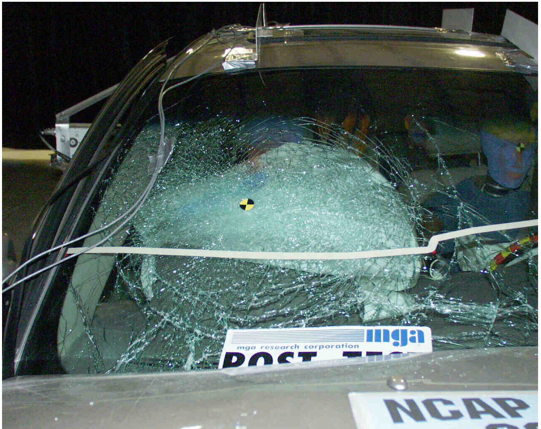
Photo No. A-44 - Post-Test Passenger Windshield View
