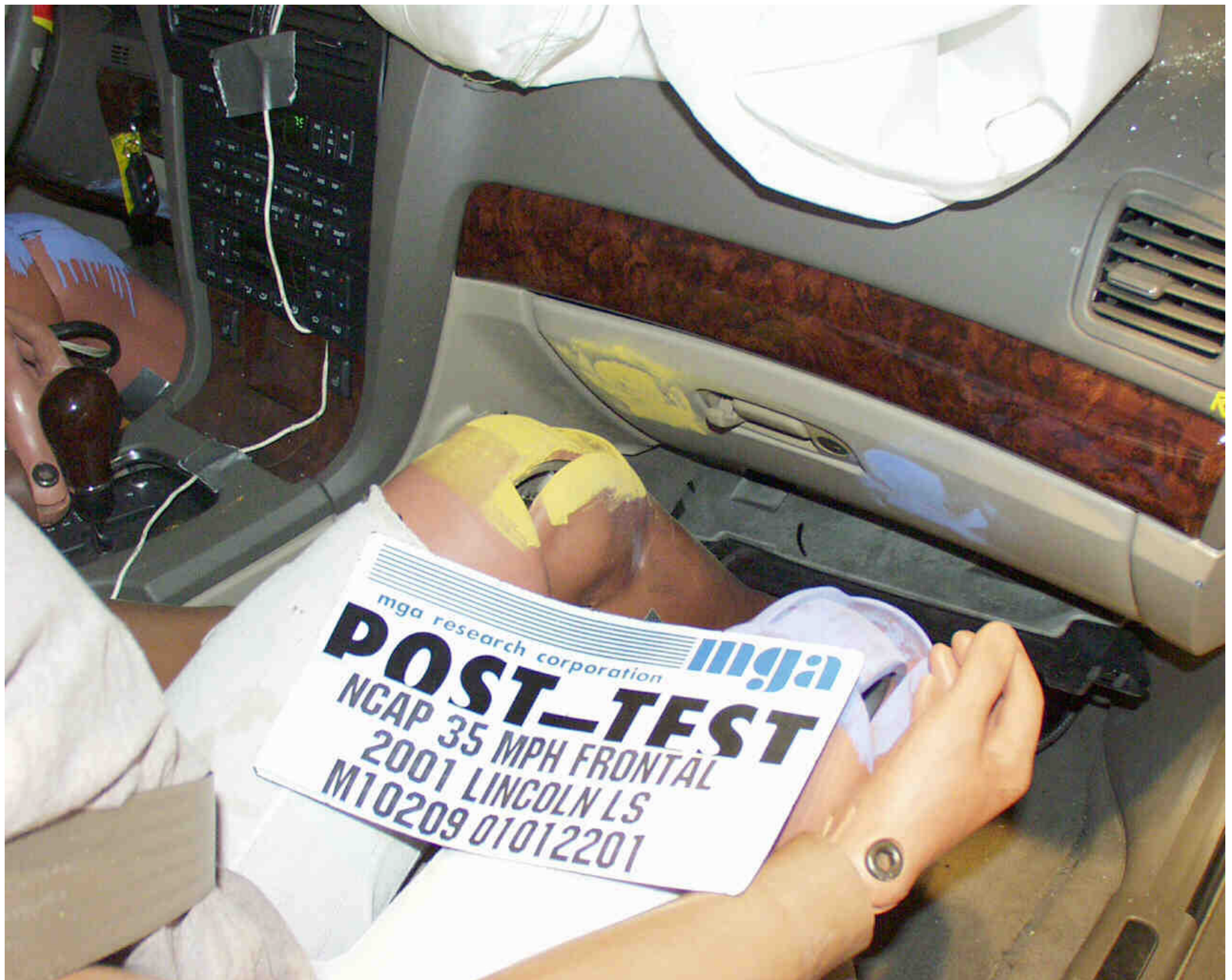
Photo No. A-40 - Post-Test Passenger Dummy Knee Position
