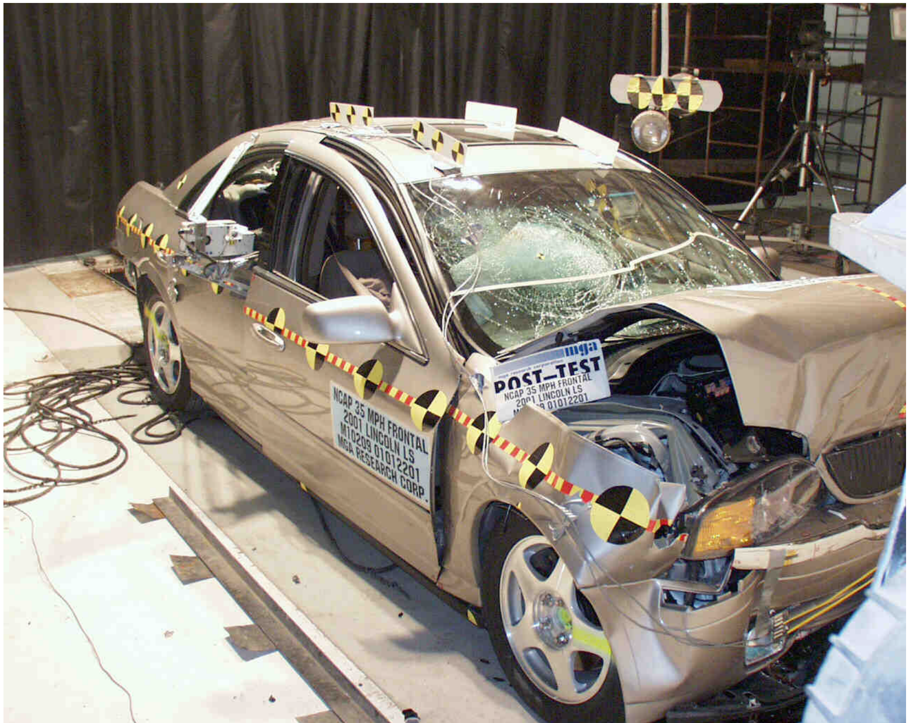
Photo No. A-11 - Post-Test Right Front Three-Quarter View of Test Vehicle
