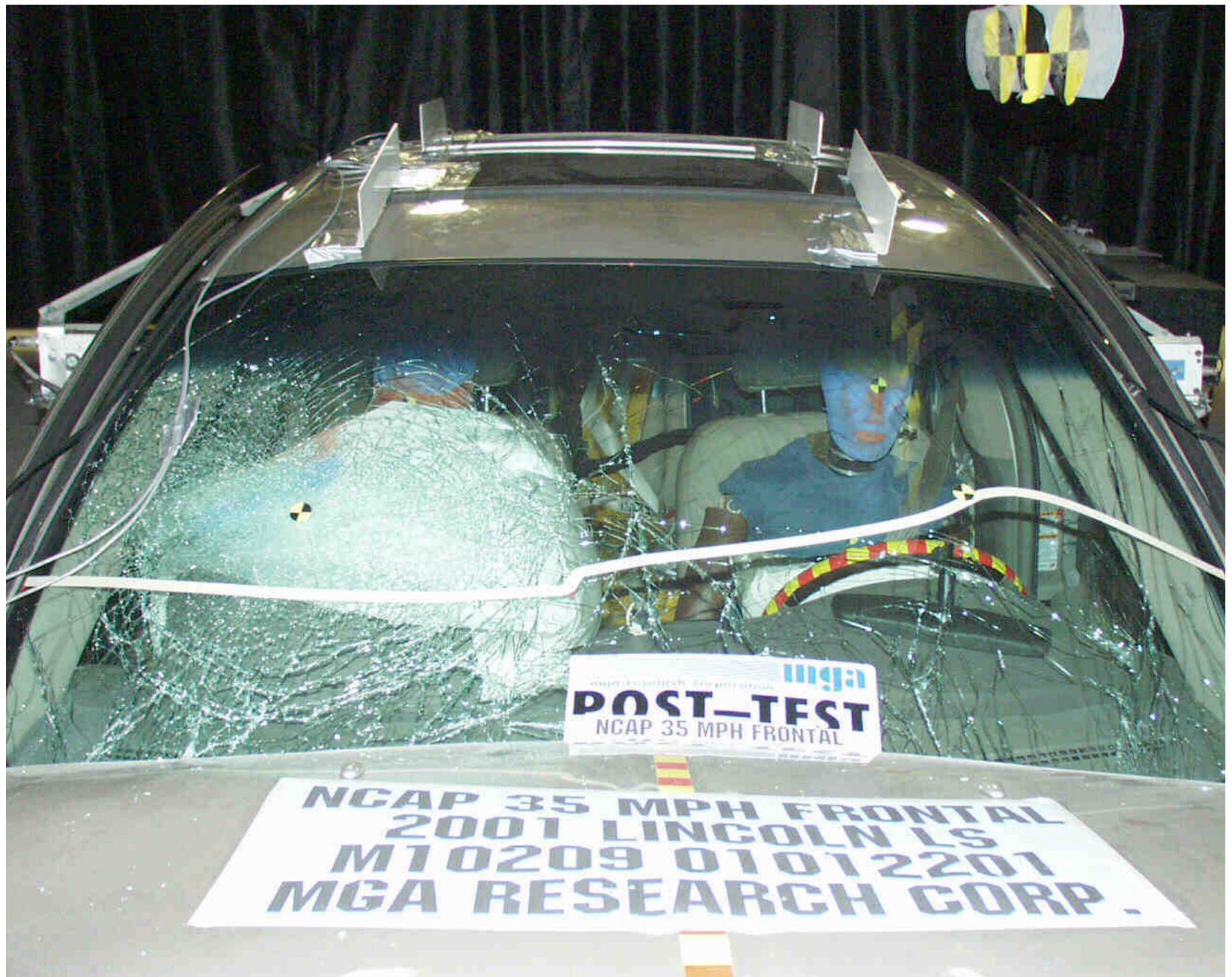
Photo No. A-20 - Post-Test Windshield View
