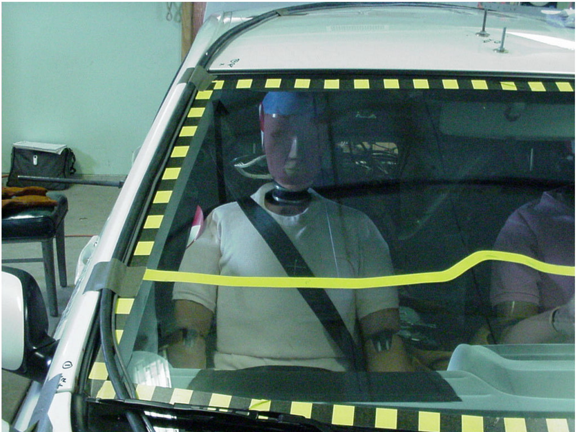
Figure A-32 PRE-TEST PASSENGER HEAD LOCATION
