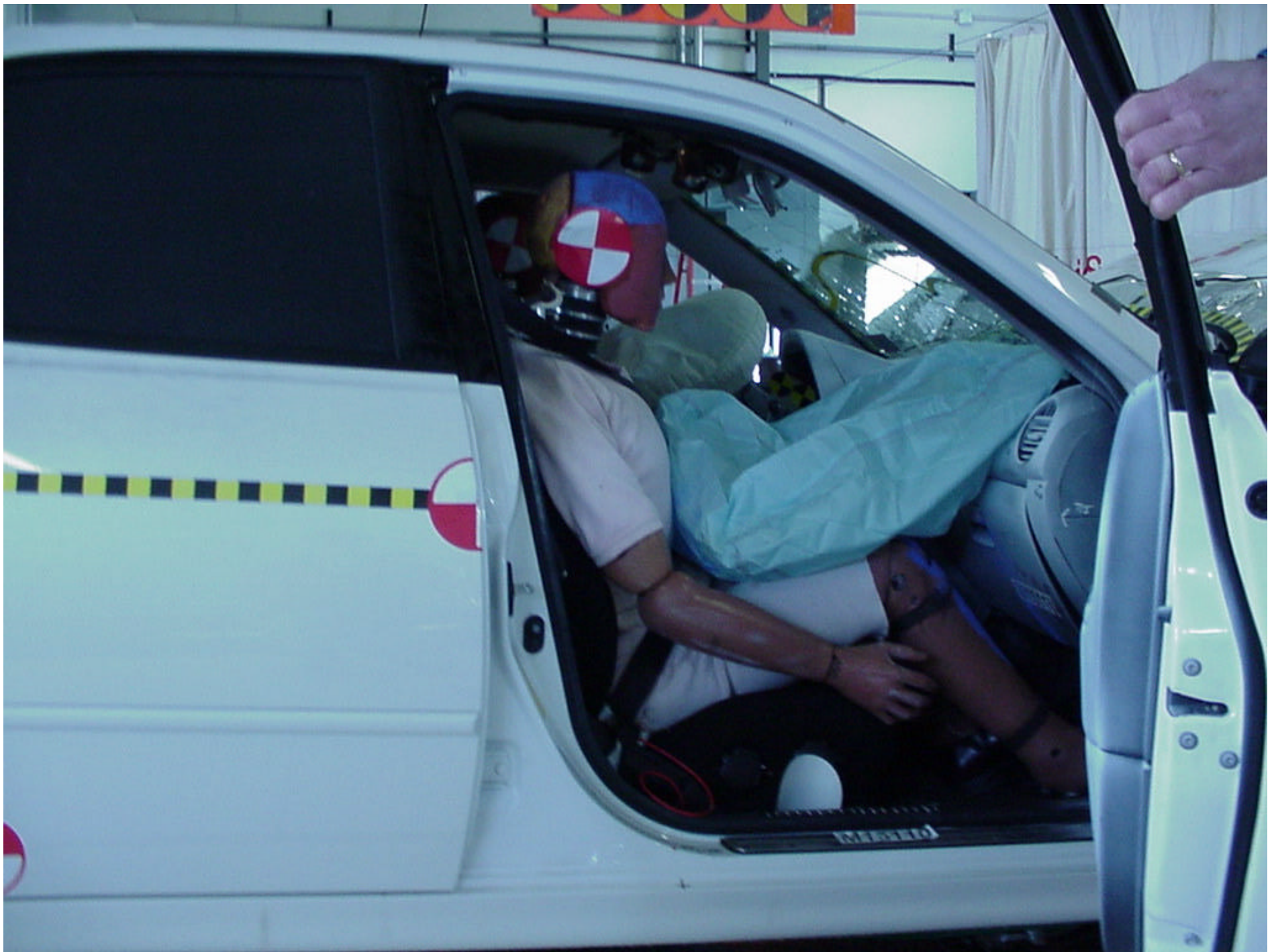
Figure A-25 POST-TEST PASSENGER POSITION VIEW
