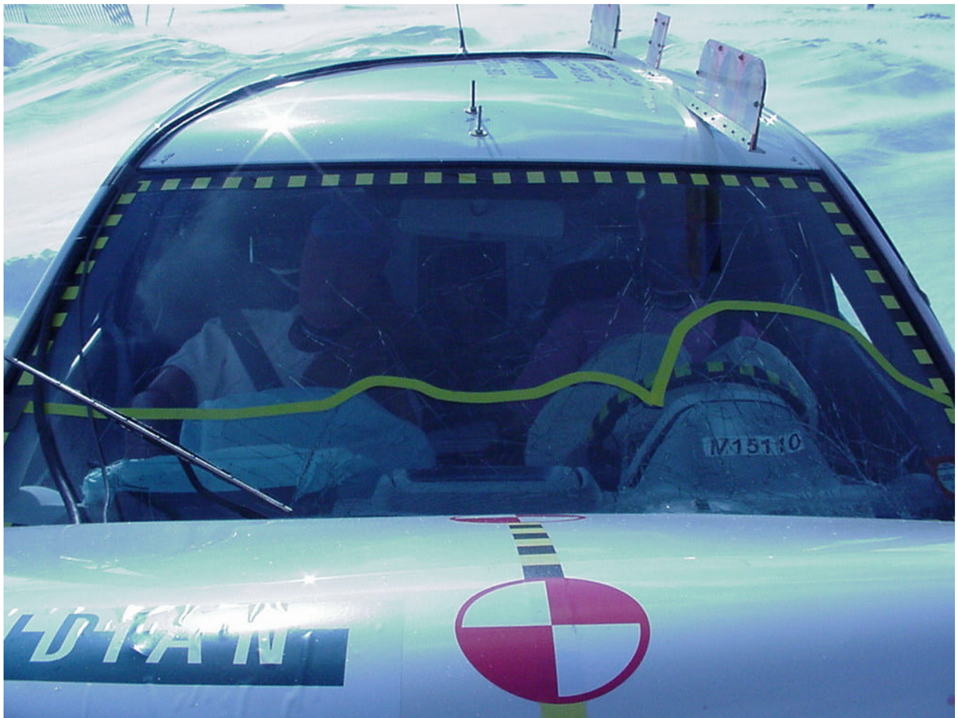
Figure A-13 POST-TEST WINDSHIELD VIEW
