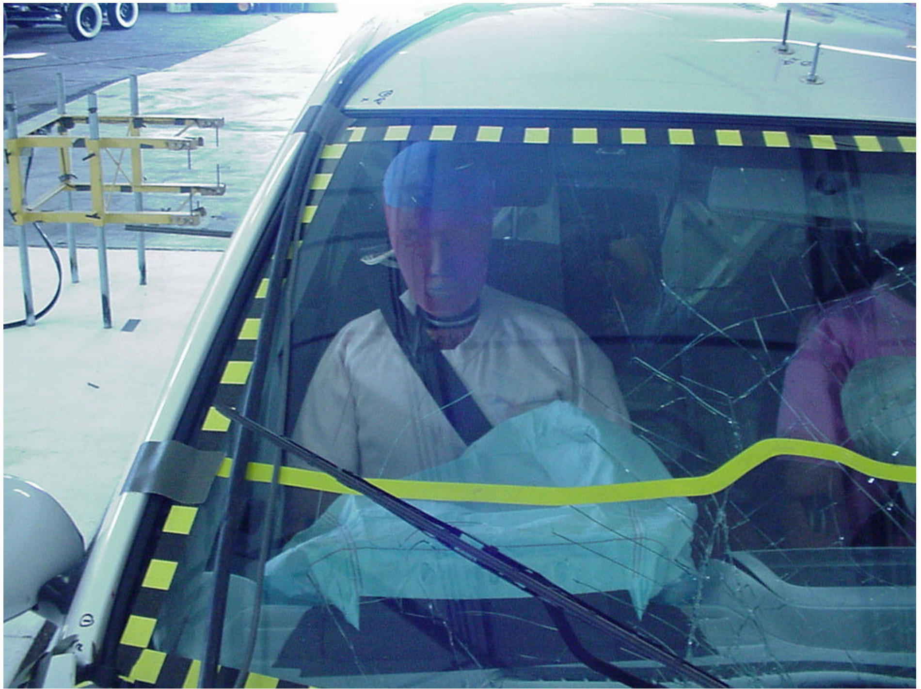
Figure A-33 POST-TEST PASSENGER HEAD LOCATION
