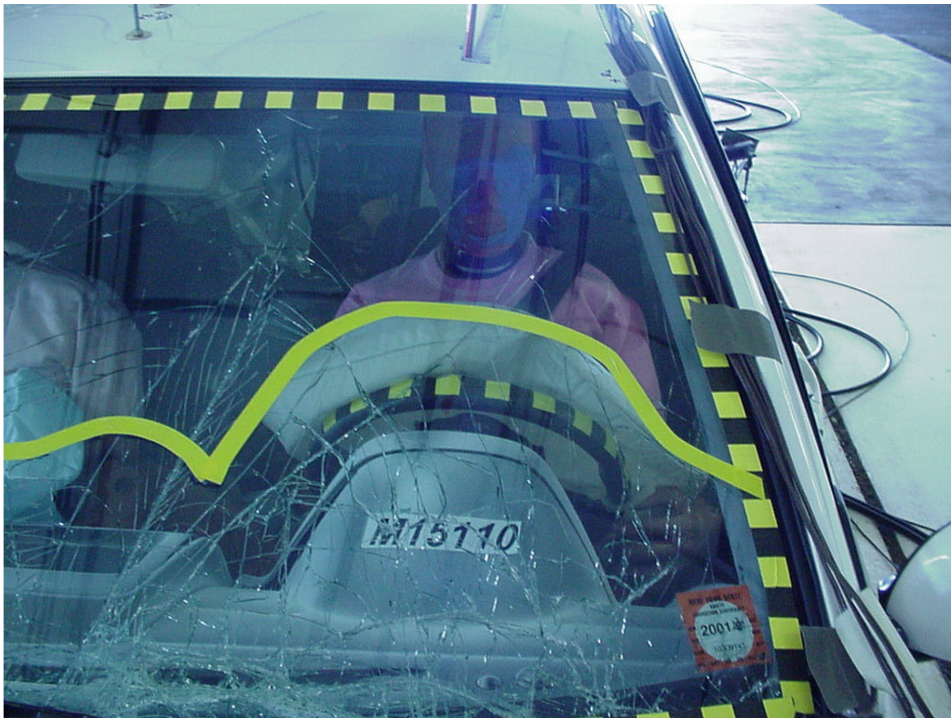
Figure A-31 POST-TEST DRIVER HEAD LOCATION
