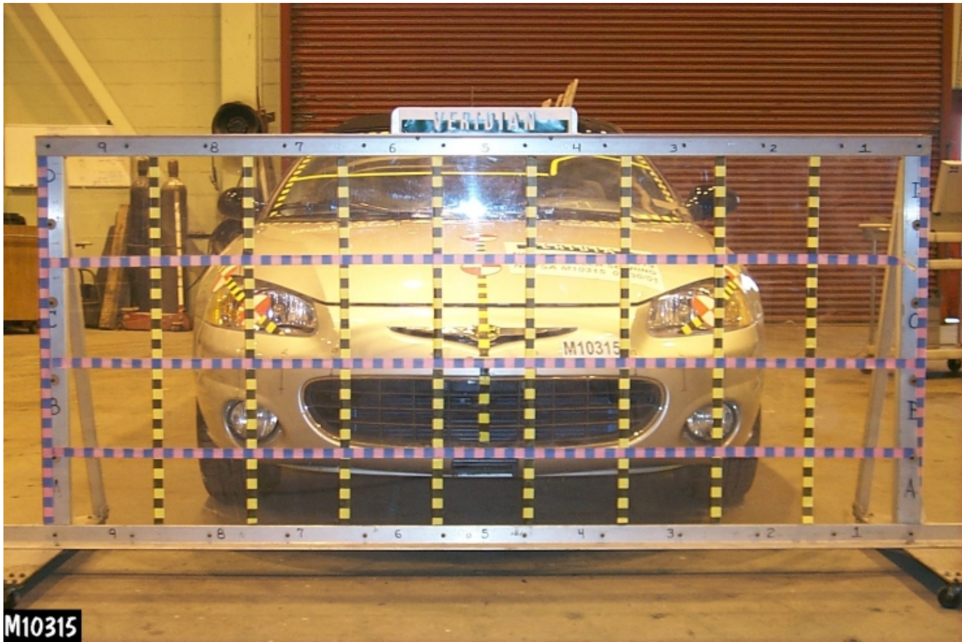
Figure A-1: LOAD CELL LOCATIONS.
