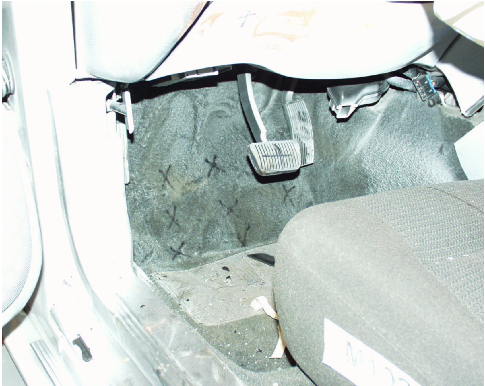
Figure A-35: POST-TEST DRIVER FLOOR PAN VIEW
