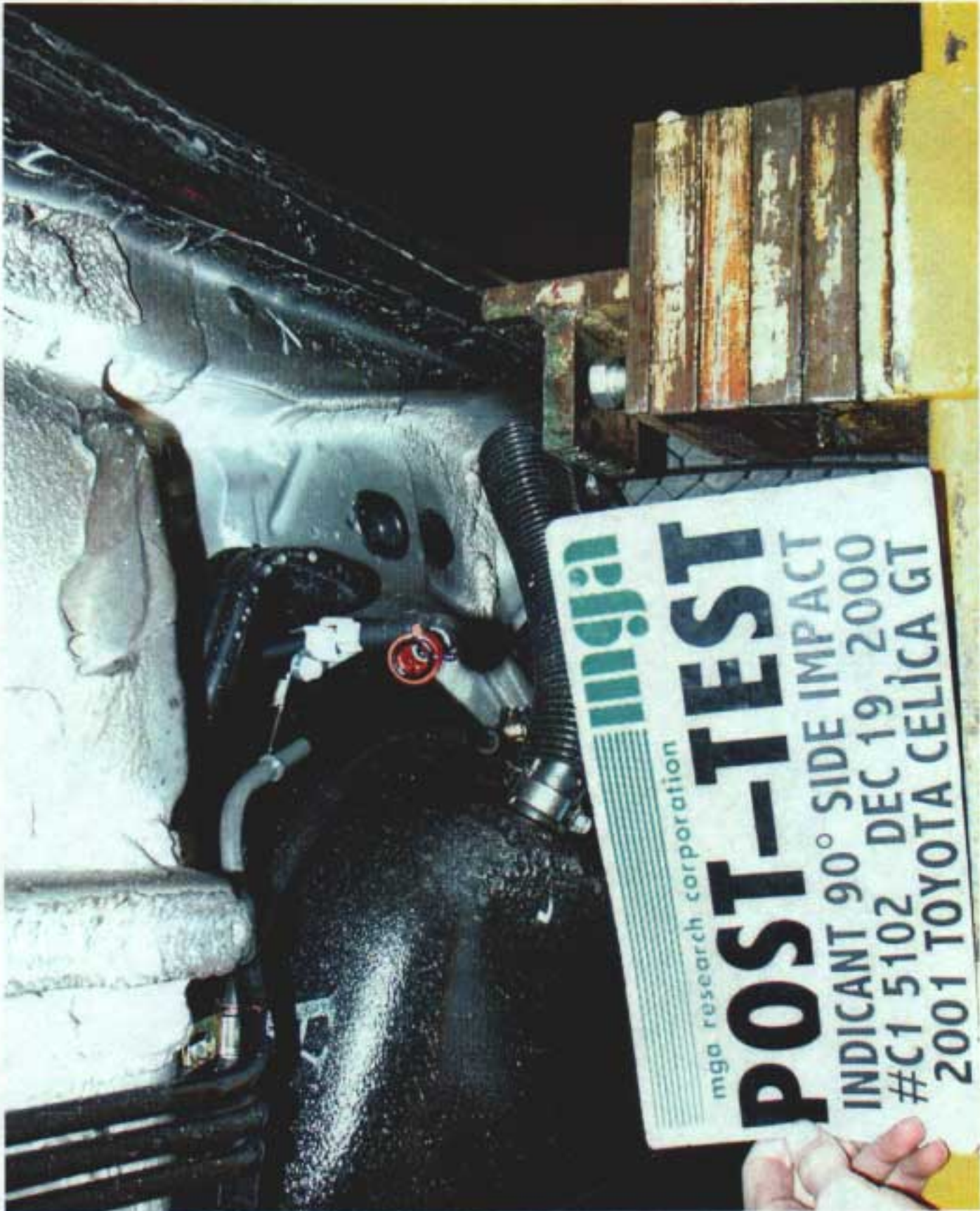
Photo No. A-51 - Post-Test Fuel Leakage Location
