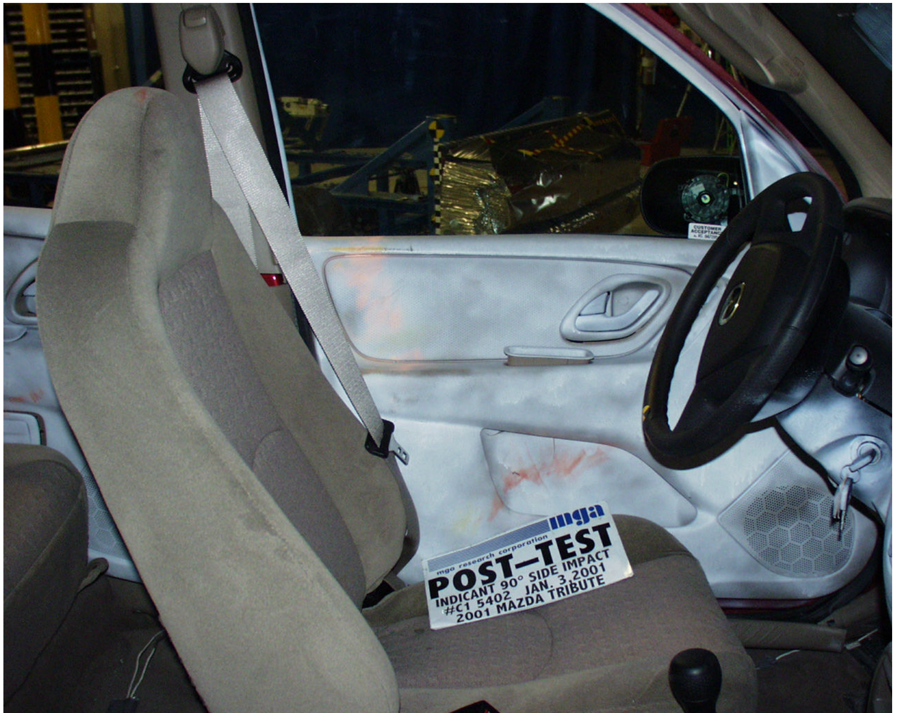
Photo No. A-27 - Post-Test Driver Dummy Contact
