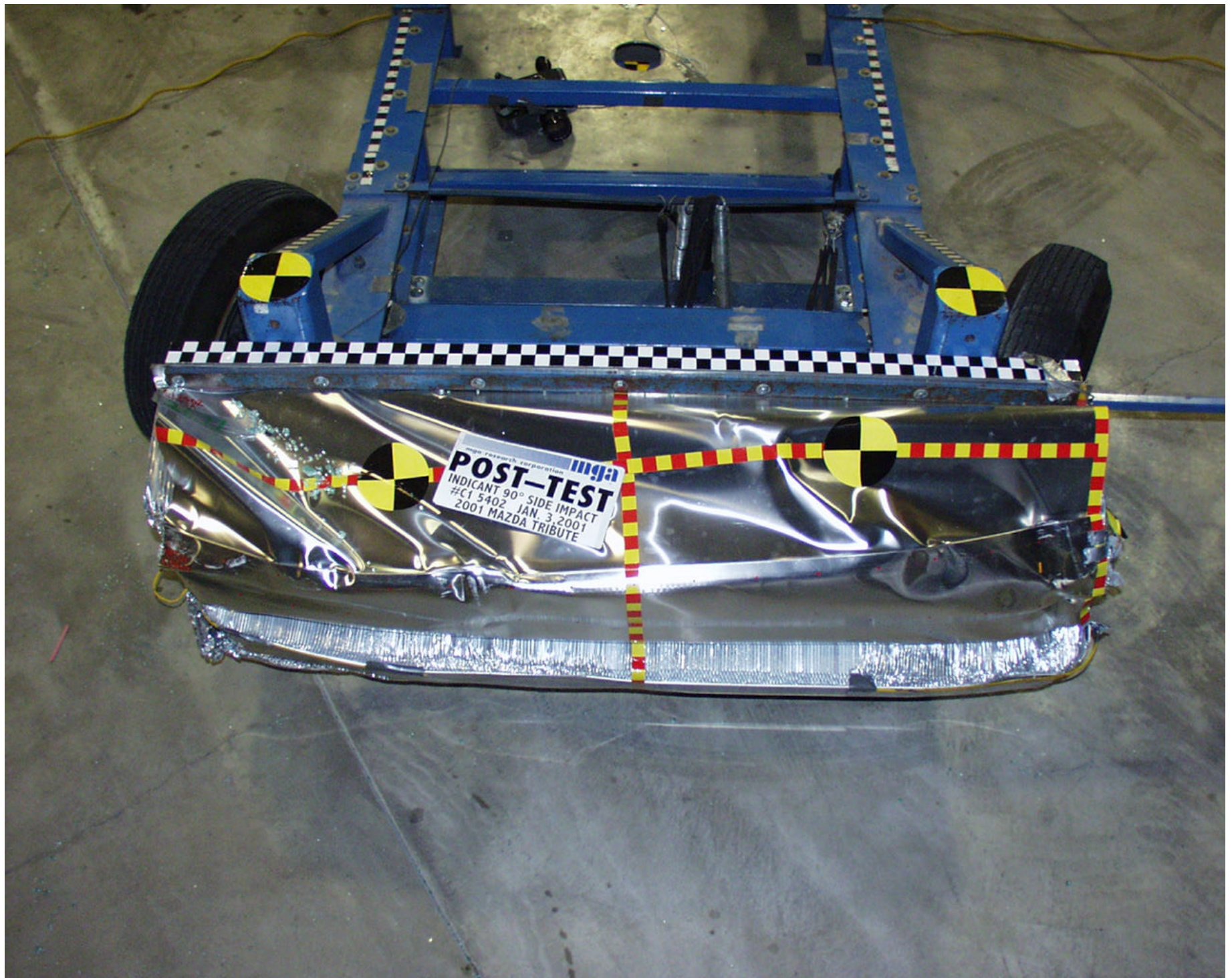
Photo No. A-13 - Post-Test MDB Top View
