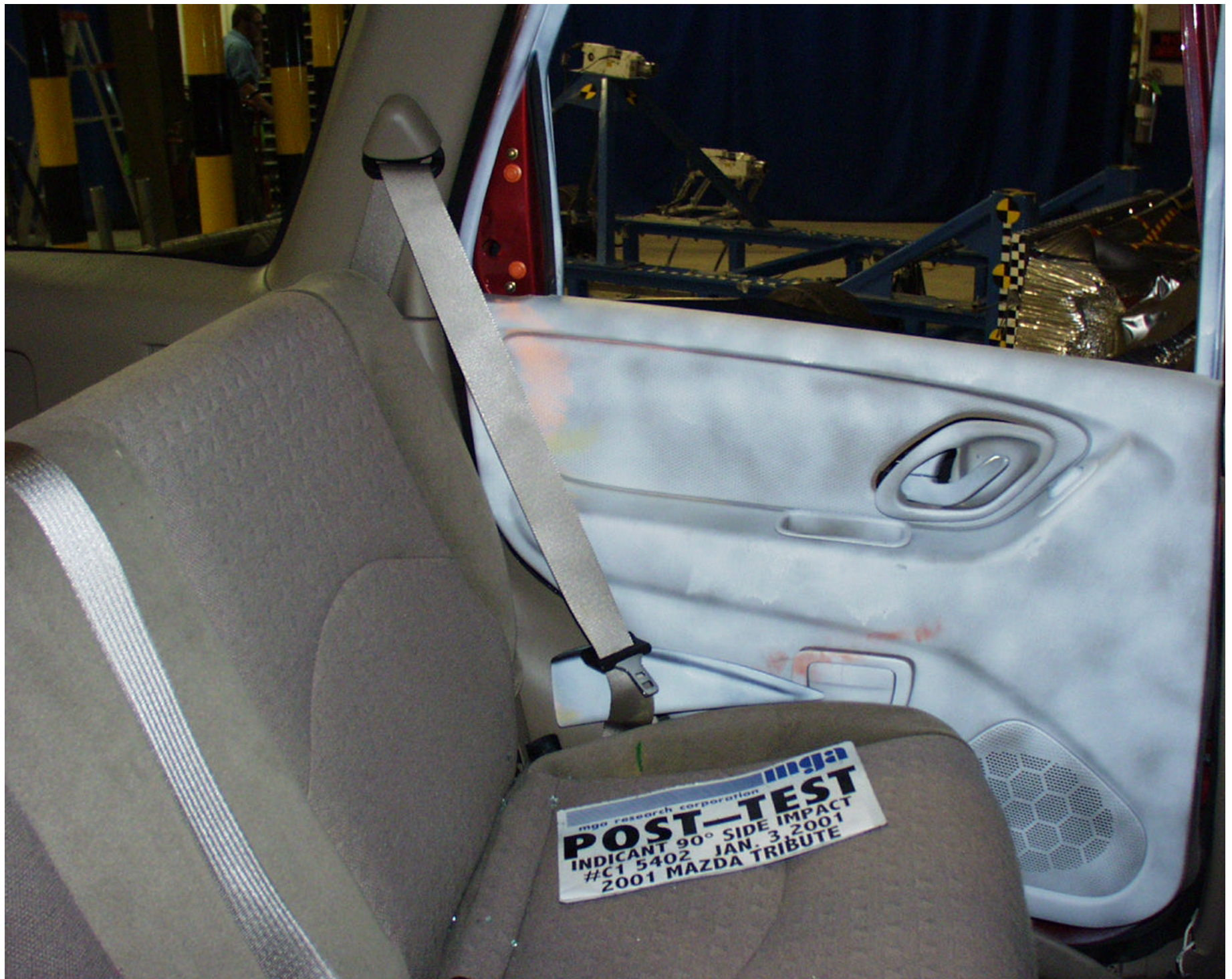
Photo No. A-36 - Post-Test Passenger Dummy Contact
