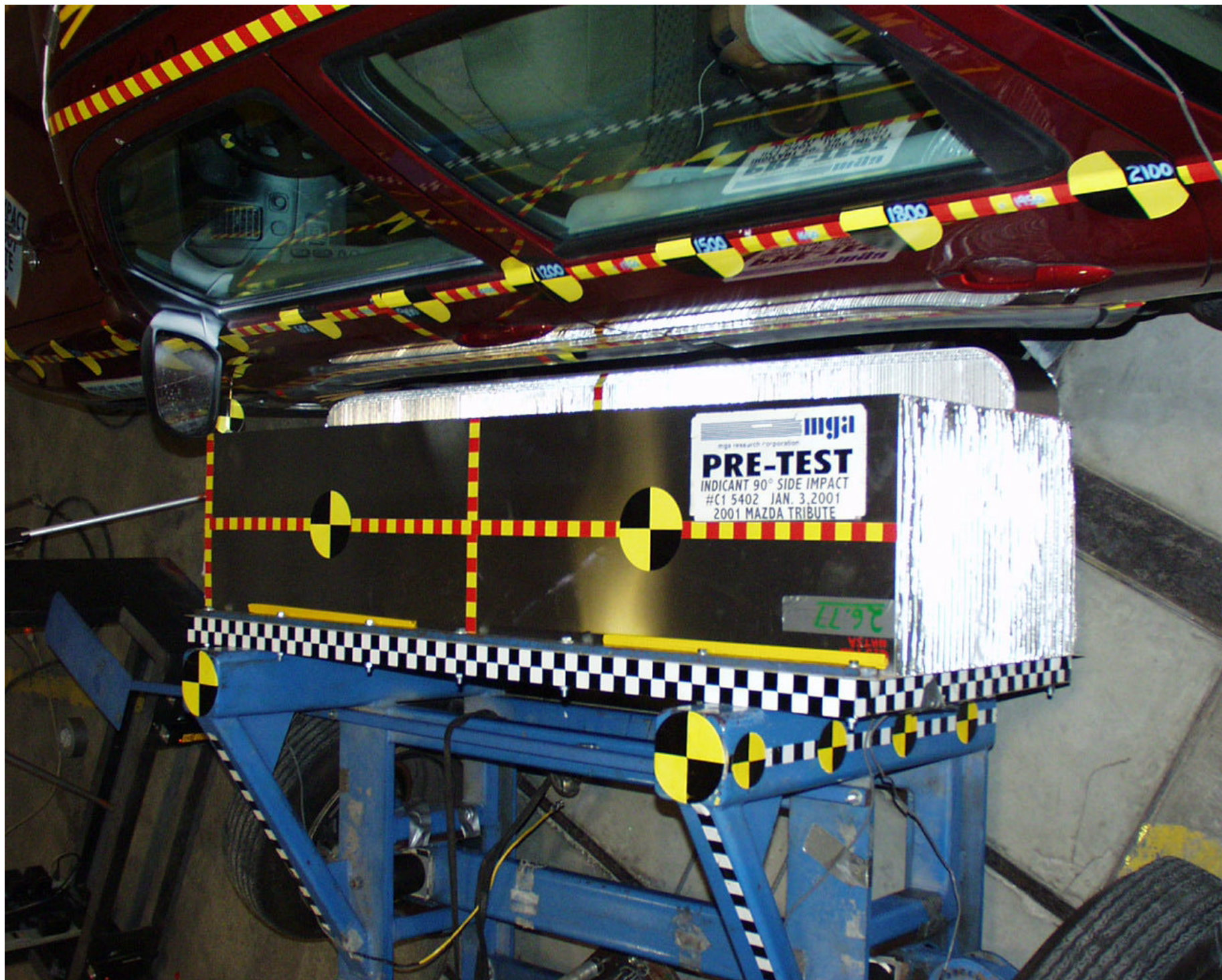
Photo No. A-9 - Pre-Test MDB Positioned Against Vehicle Overhead View
