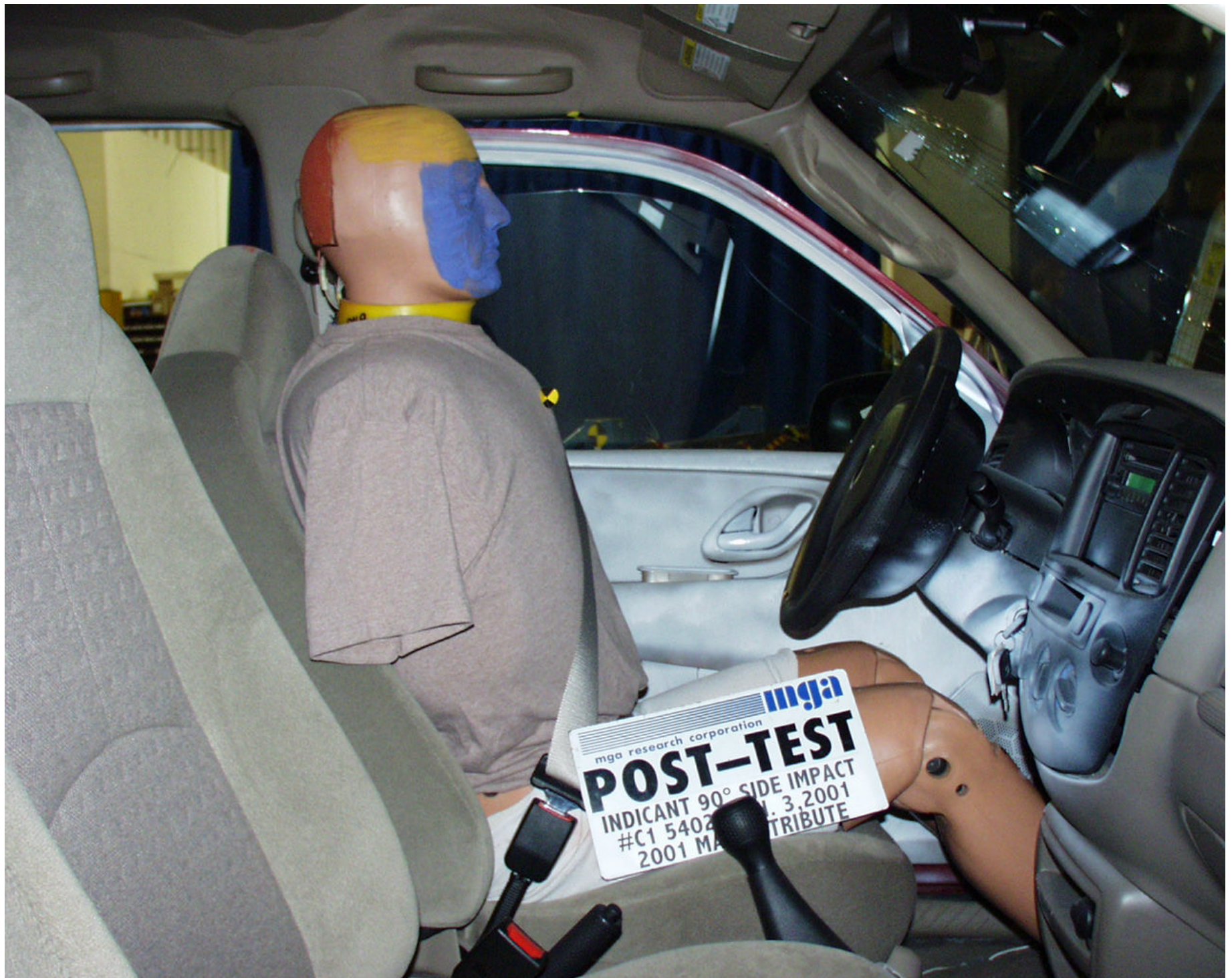
Photo No. A-21 - Post-Test Driver Dummy Right Side View
