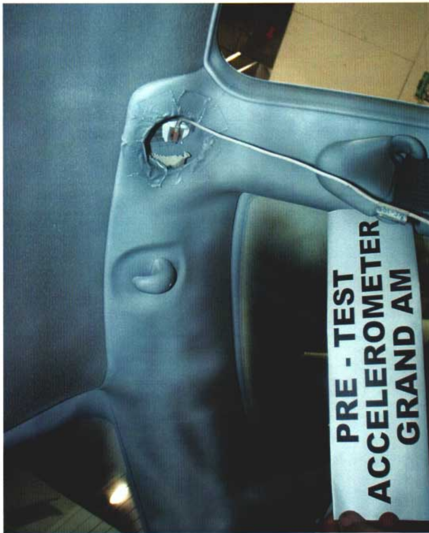
Photo No. A-51 - Left Upper B Post Accelerometer
