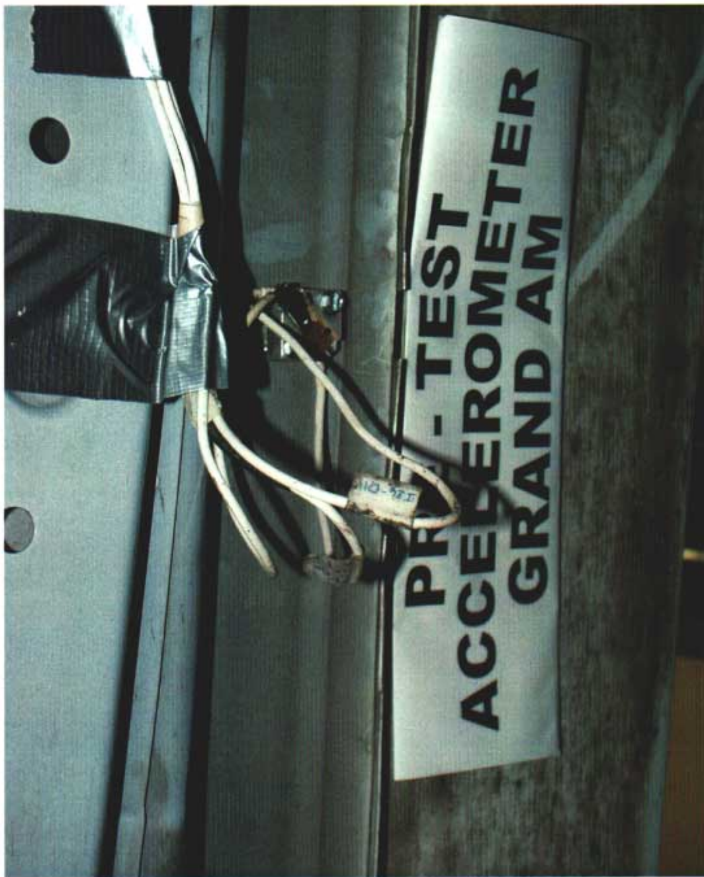
Photo No. A-46 - Right Front Sill Accelerometer
