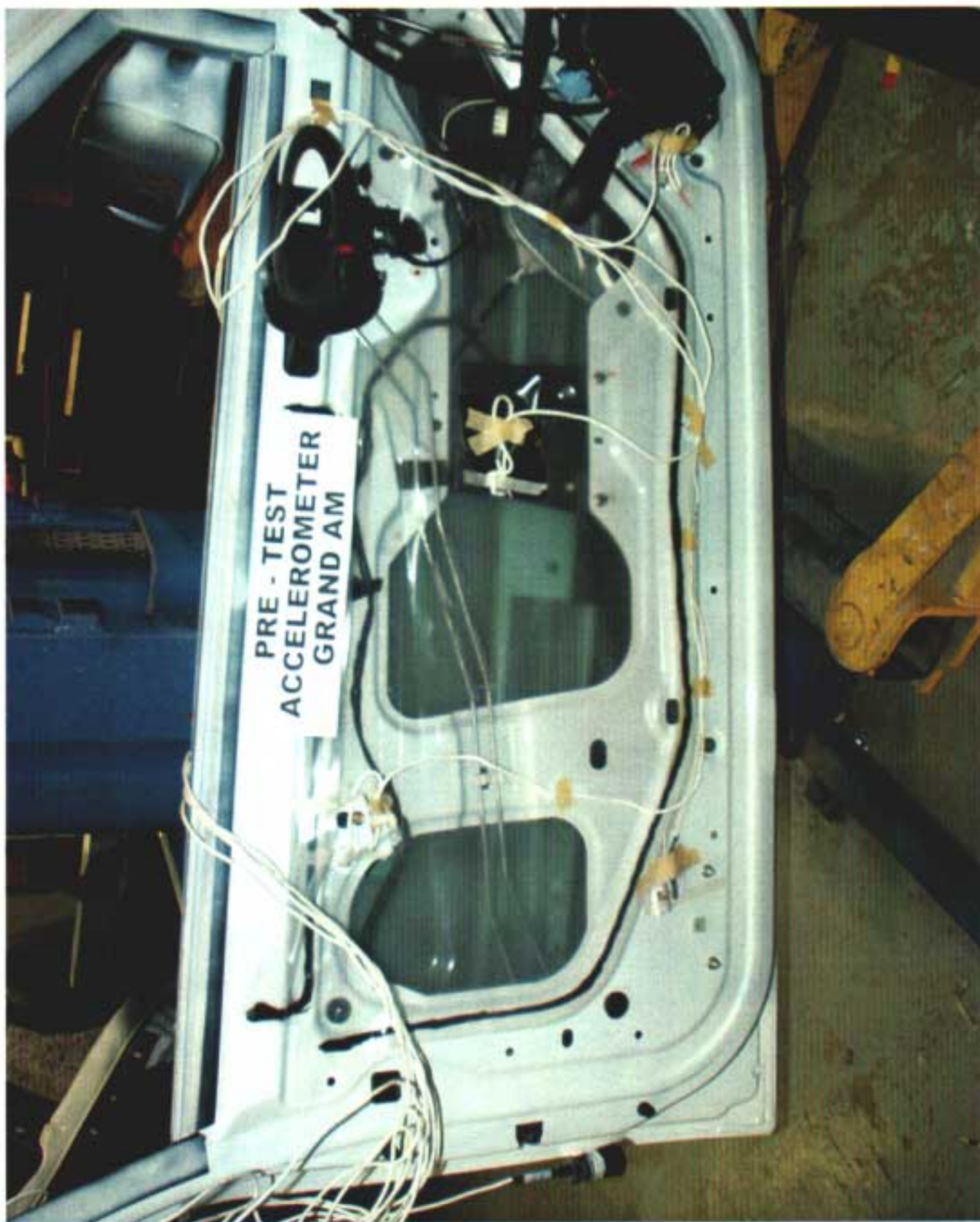
Photo No. A-50 - Left Front Door Accelerometer
