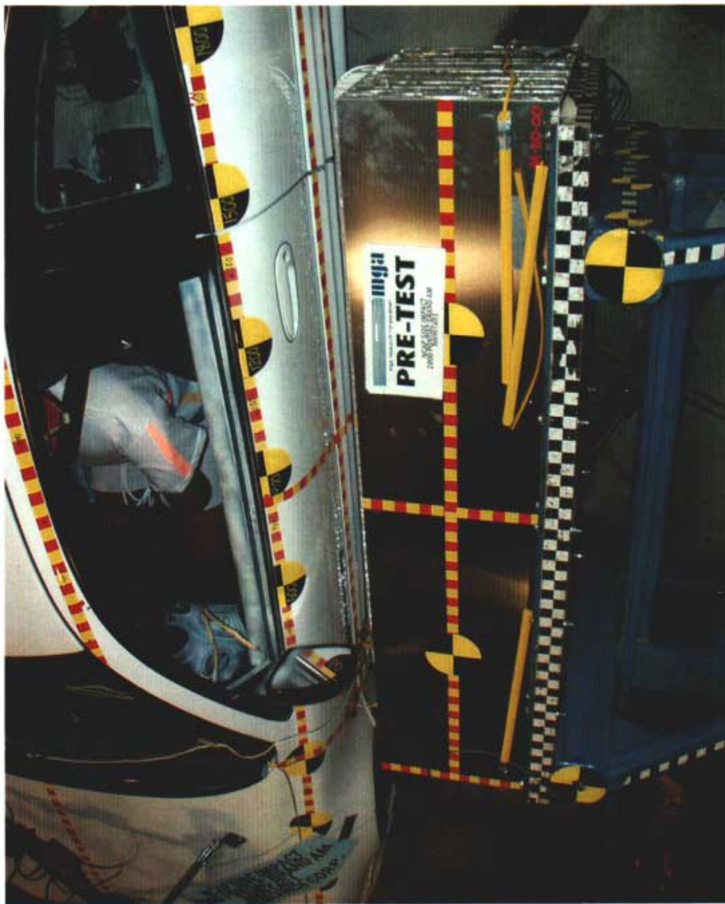
Photo No. A-9 - Pre-Test MDB Positioned Against Vehicle Overhead View
