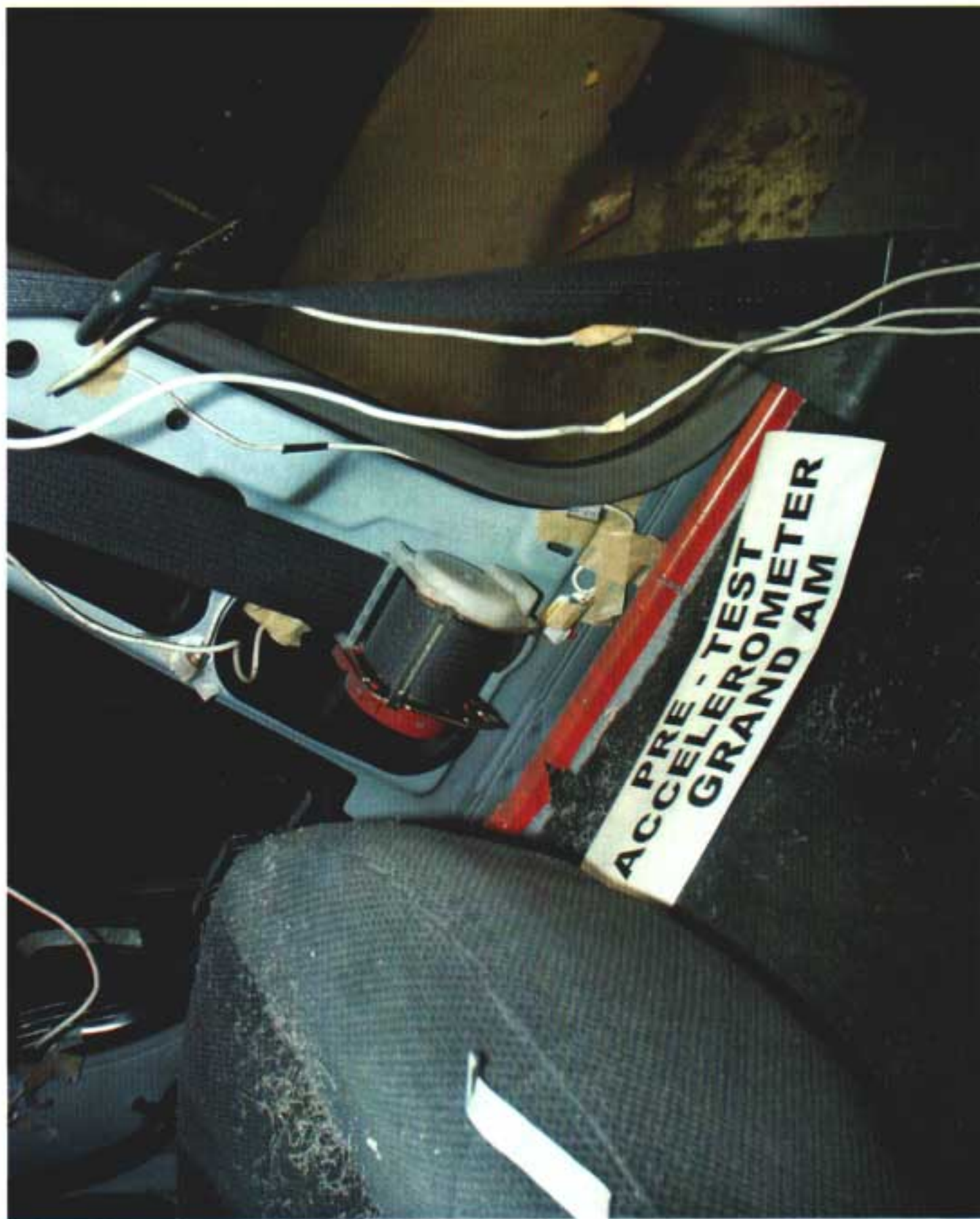
Photo No. A-52 - Left Lower B Post Accelerometer
