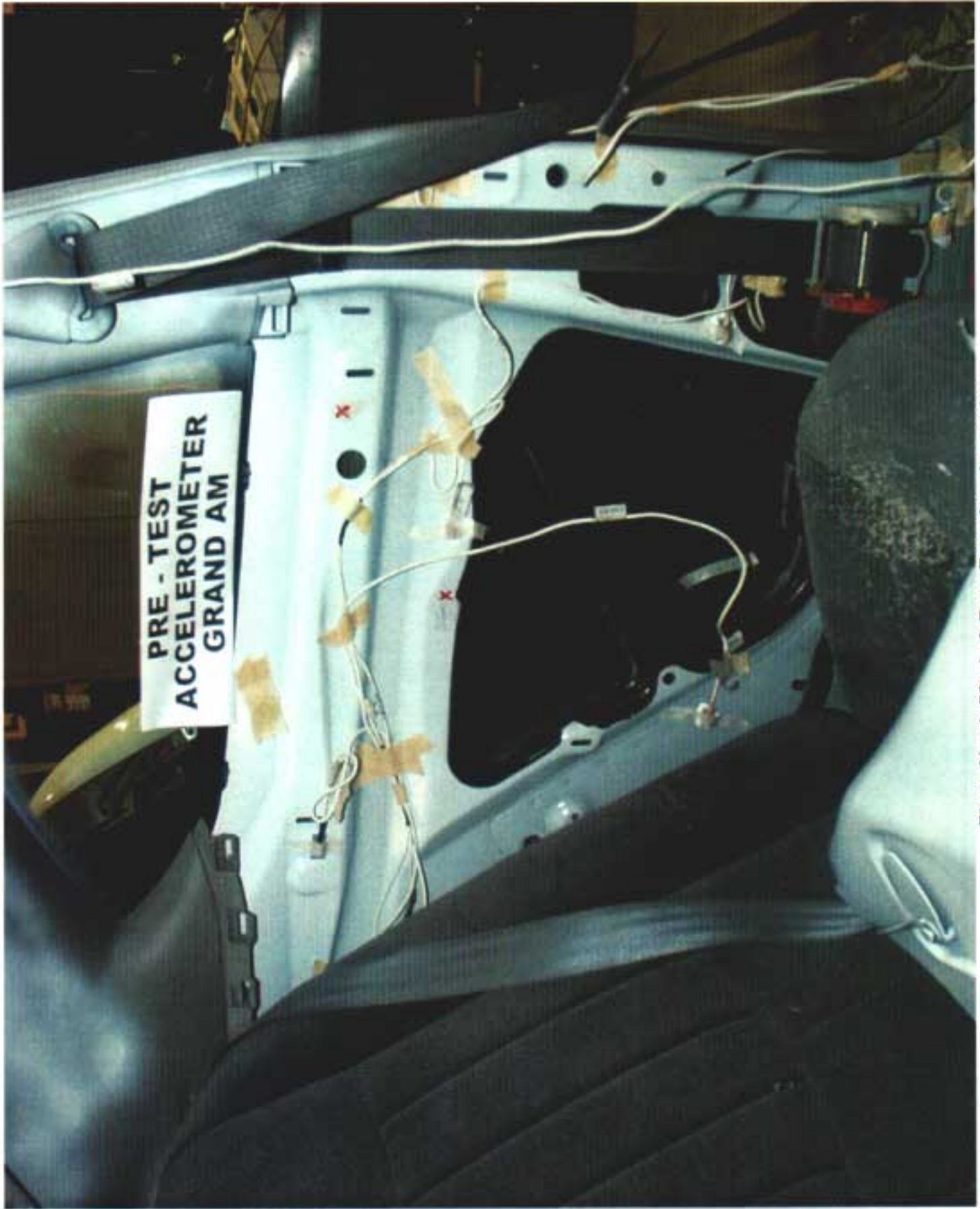
Photo No. A-53 - Left Rear Door Accelerometer
