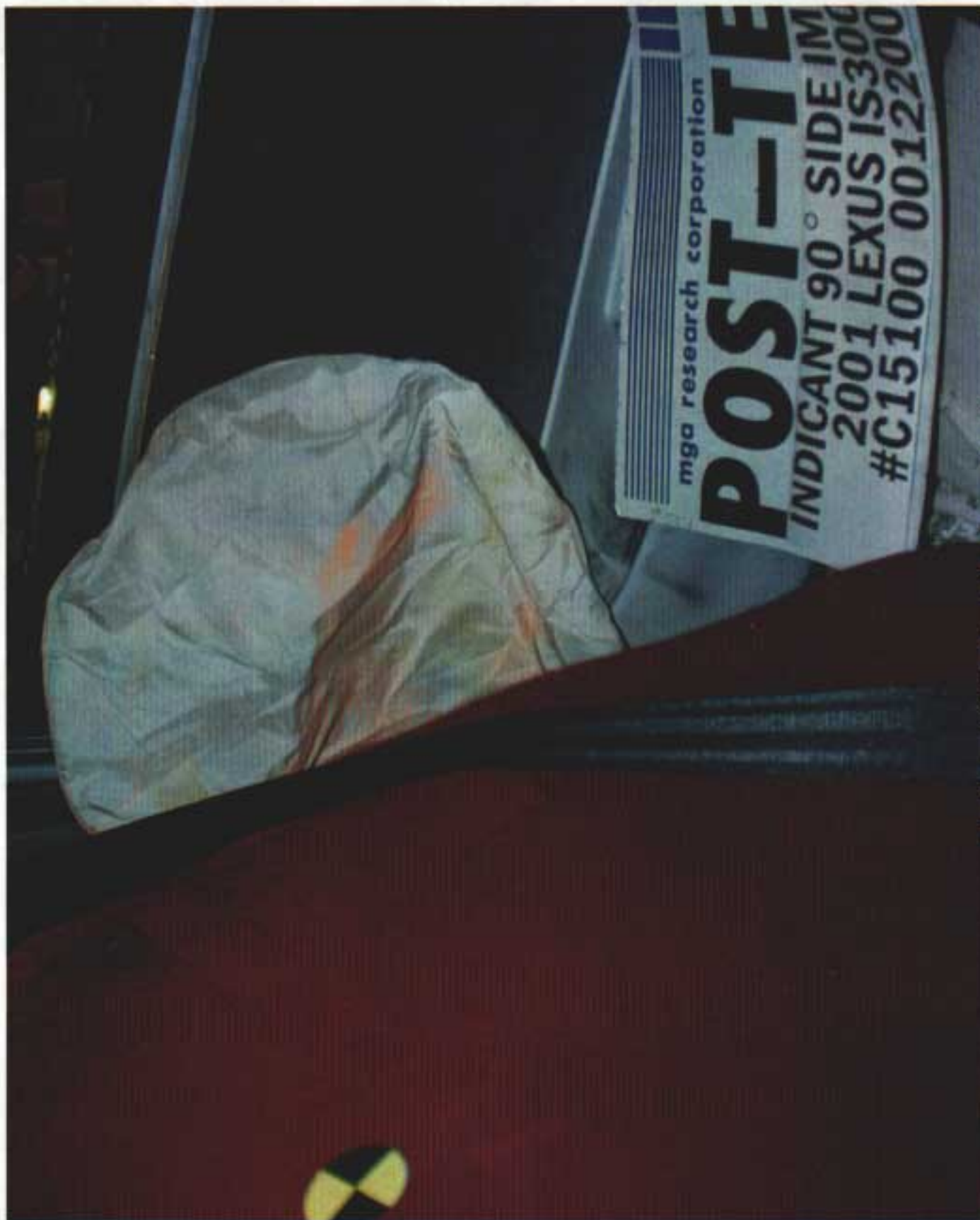
Photo No. A-28 - Post-Test Driver Dummy Contact
