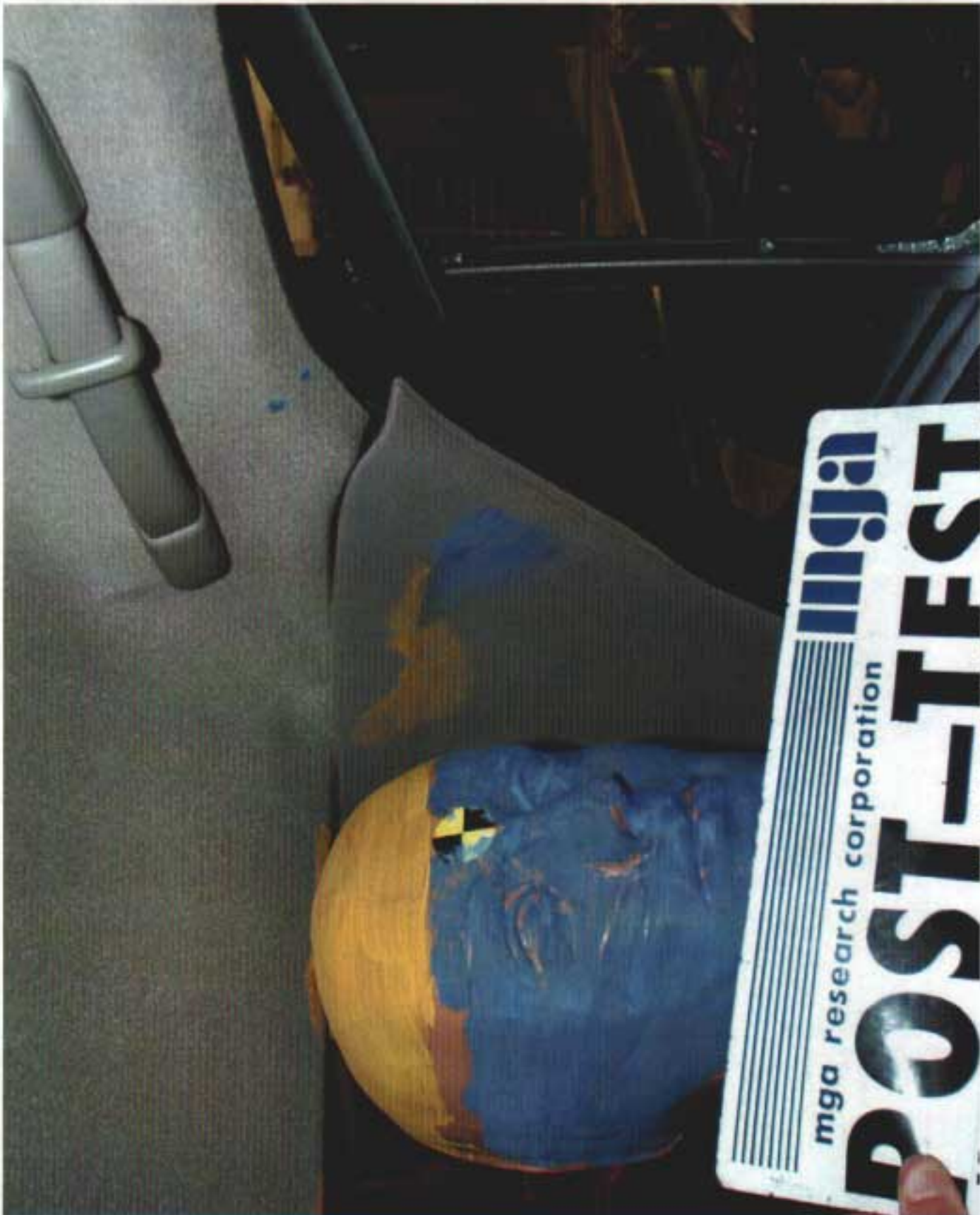
Photo No. A-38 - Post-Test Passenger Dummy Head Contact
