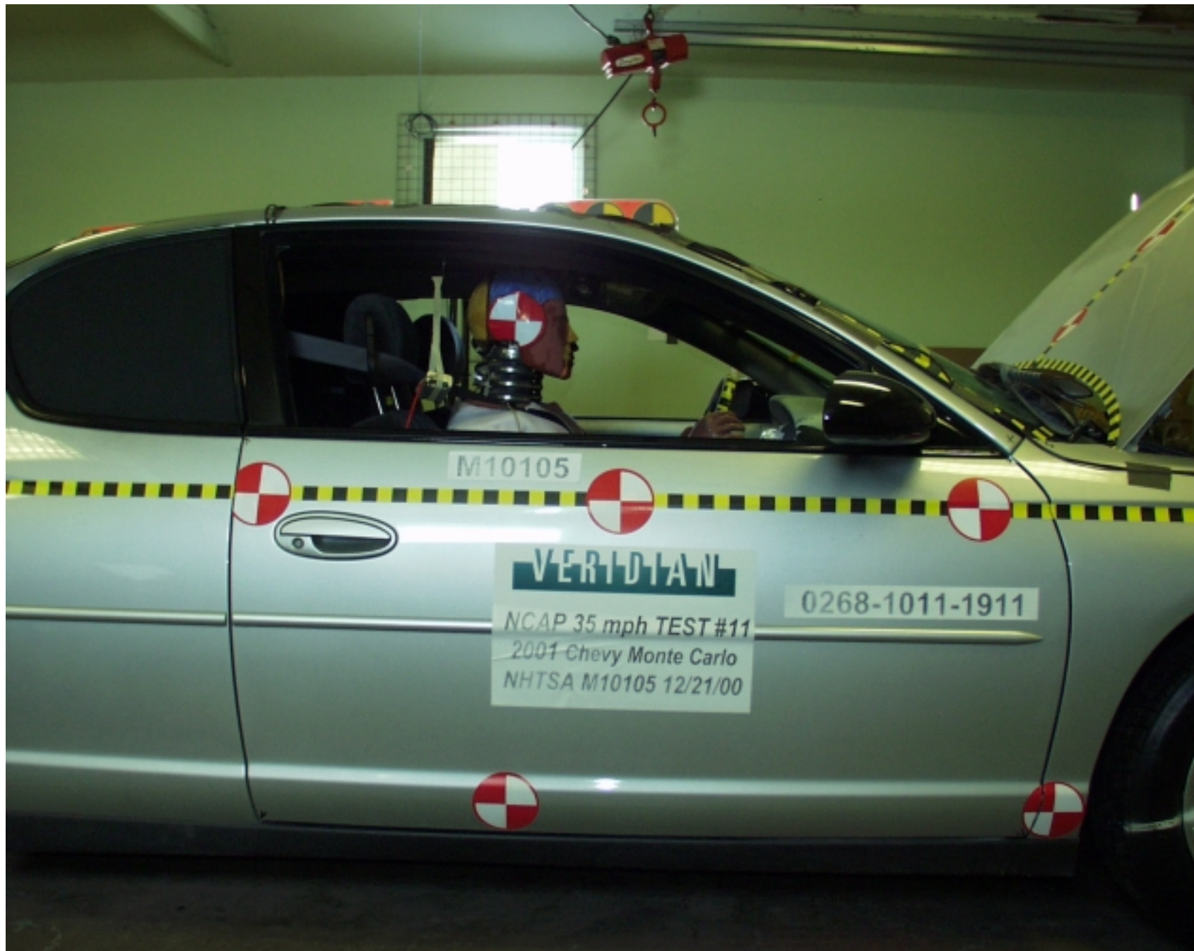
Figure A-24: PRE-TEST PASSENGER POSITION VIEW
