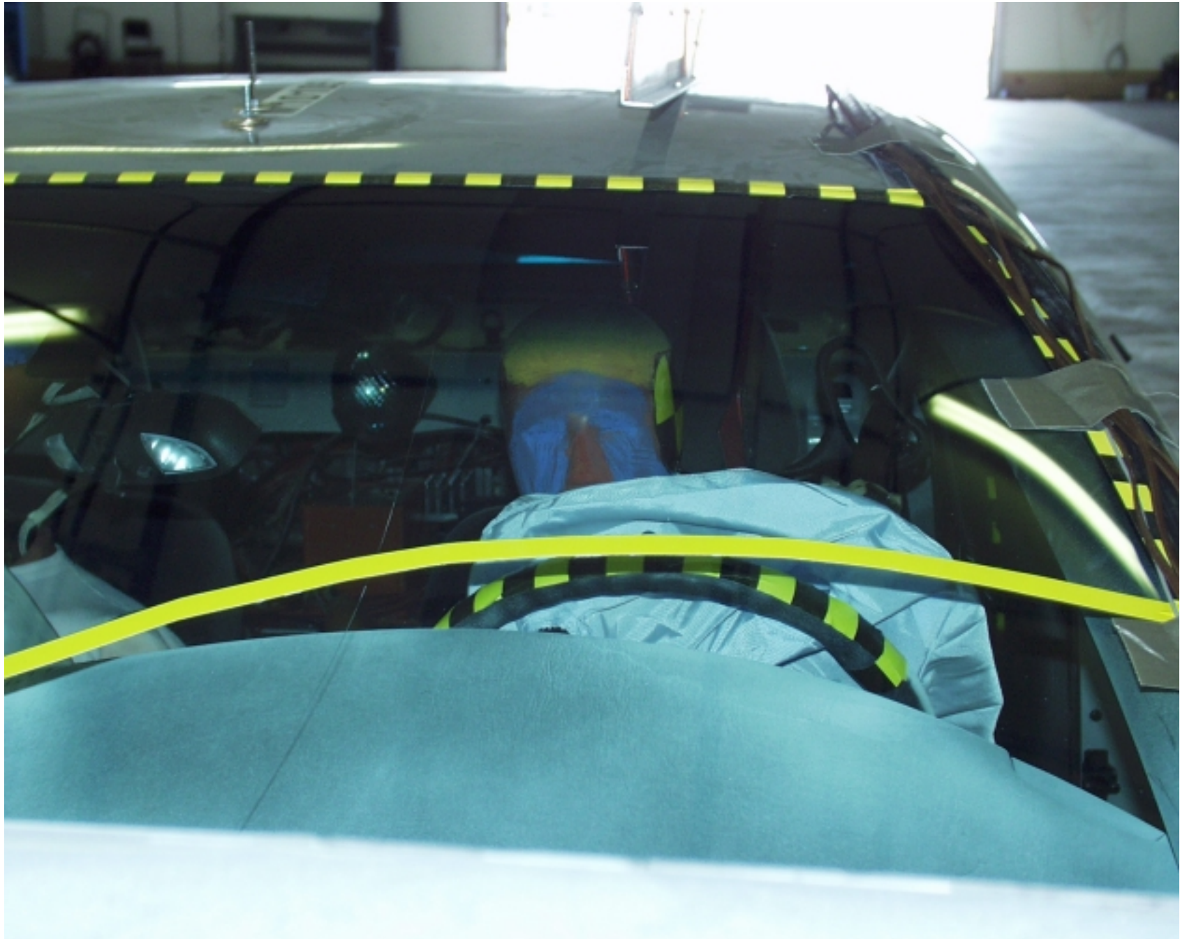
Figure A-31: POST-TEST DRIVER HEAD LOCATION
