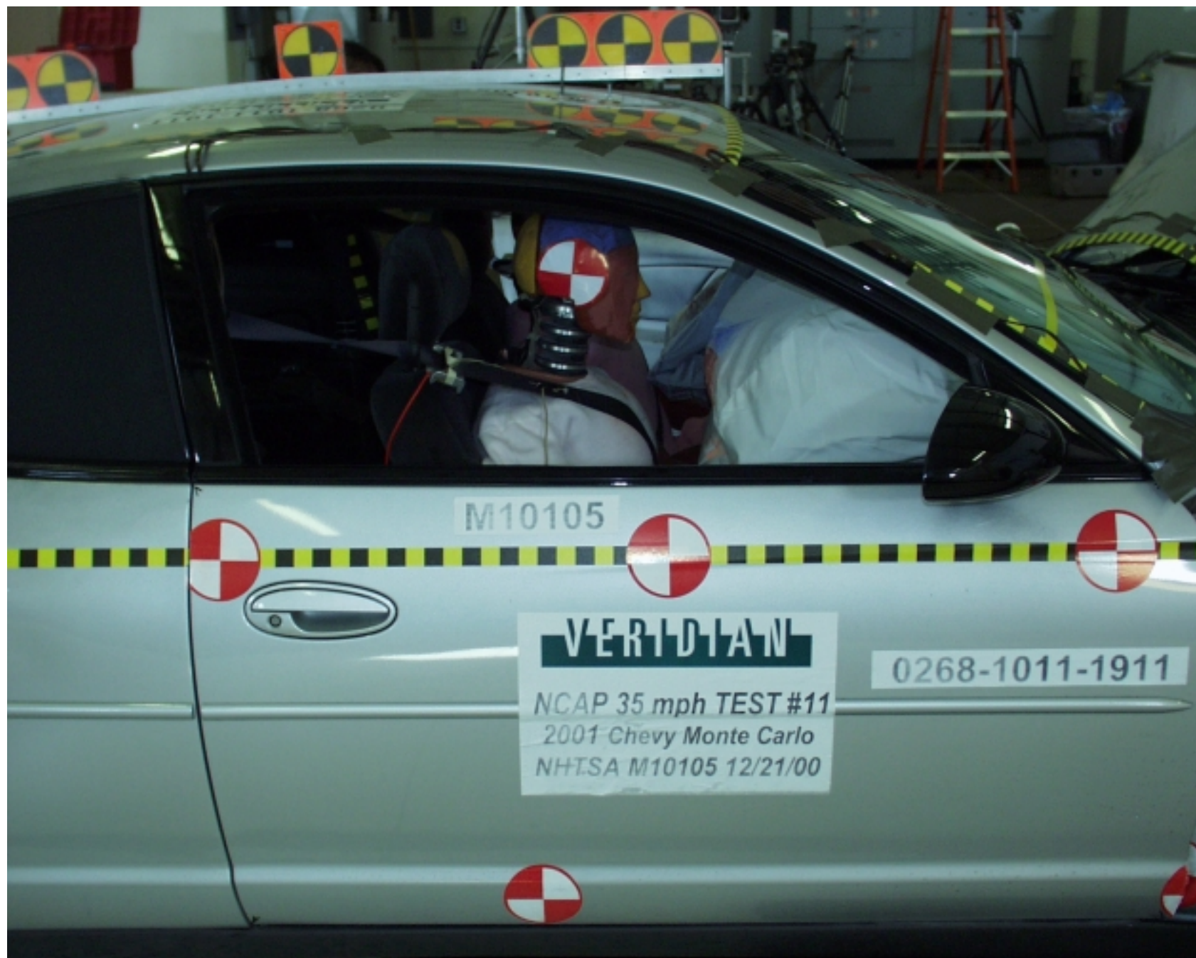
Figure A-25: POST-TEST PASSENGER POSITION VIEW
