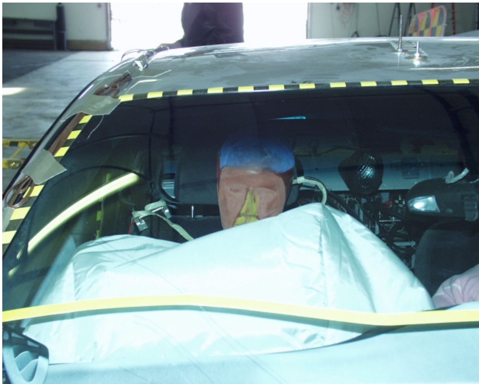
Figure A-33: POST-TEST PASSENGER HEAD LOCATION
