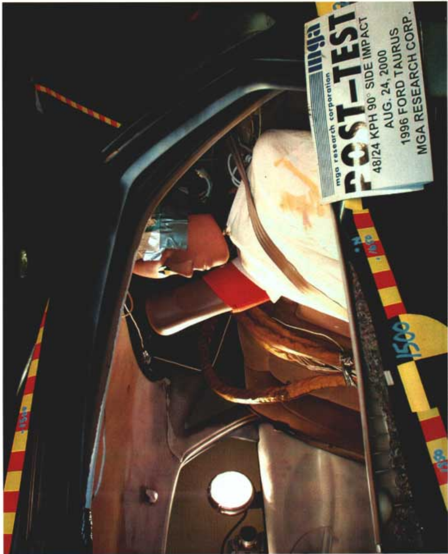
Photo No. A-30 – Post-Test Left Rear Passenger Dummy Left Side View
