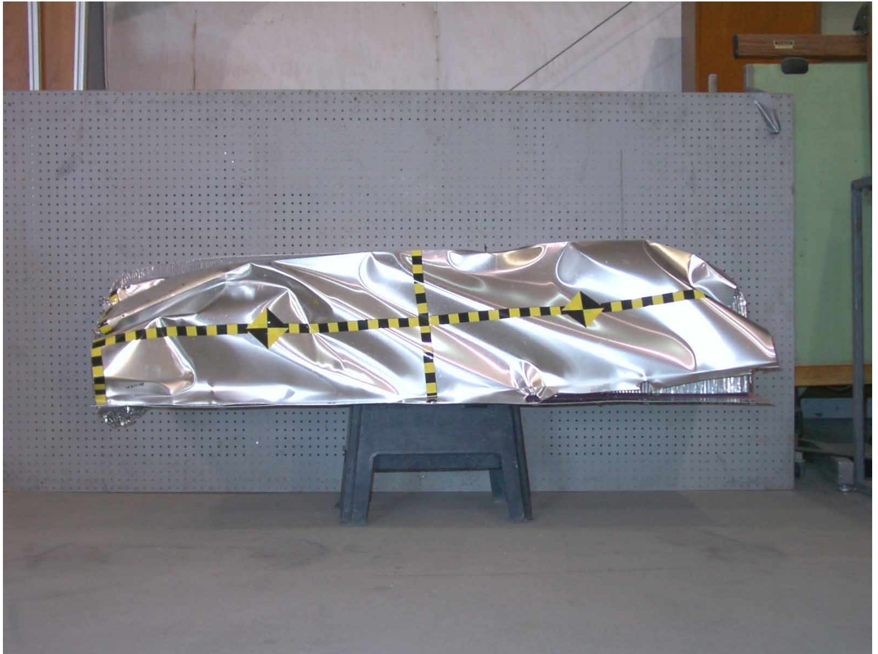
Figure A-39: Top View of Deformable Barrier, Post-Test
