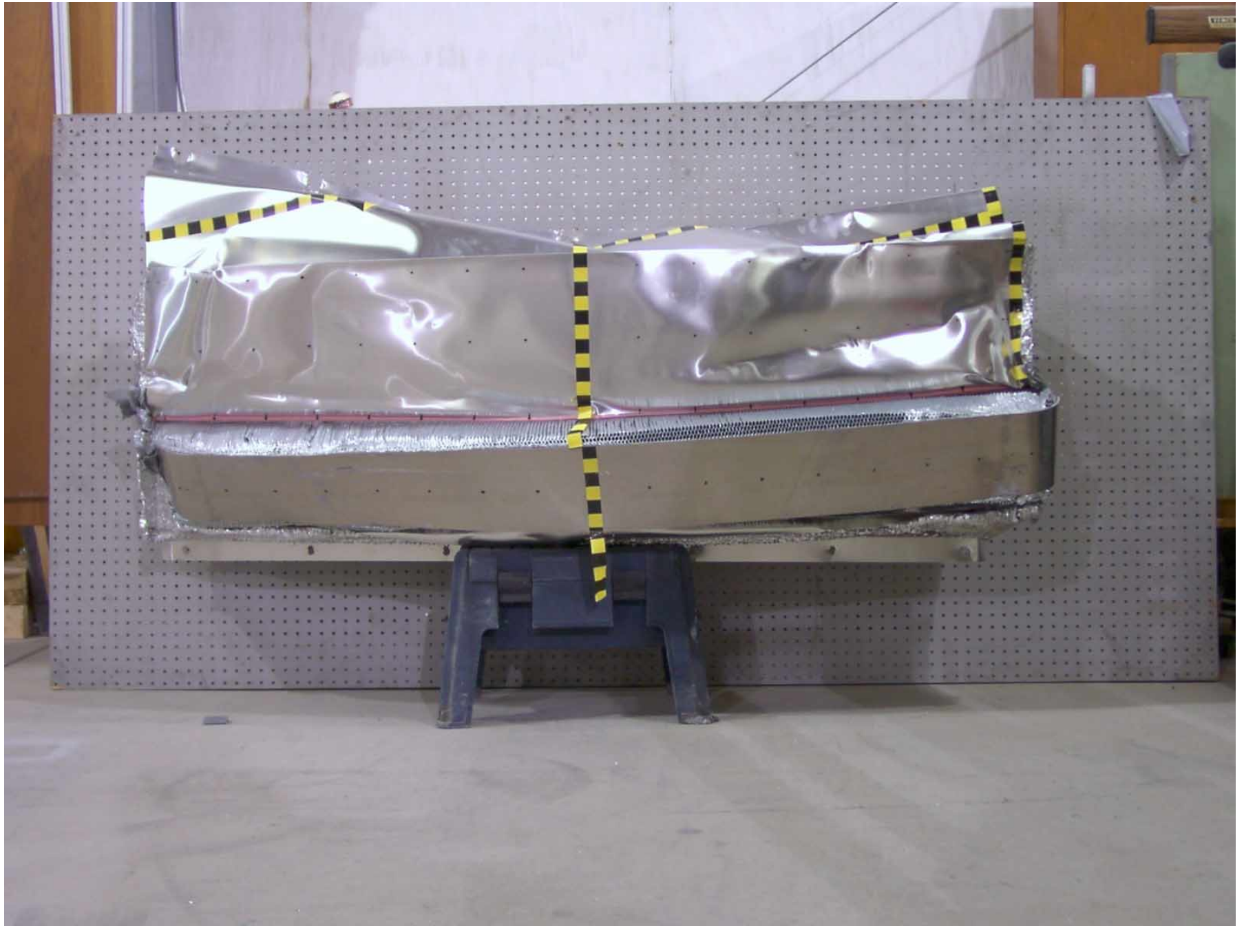
Figure A-37: Front View of Deformable Barrier, Post-Test
