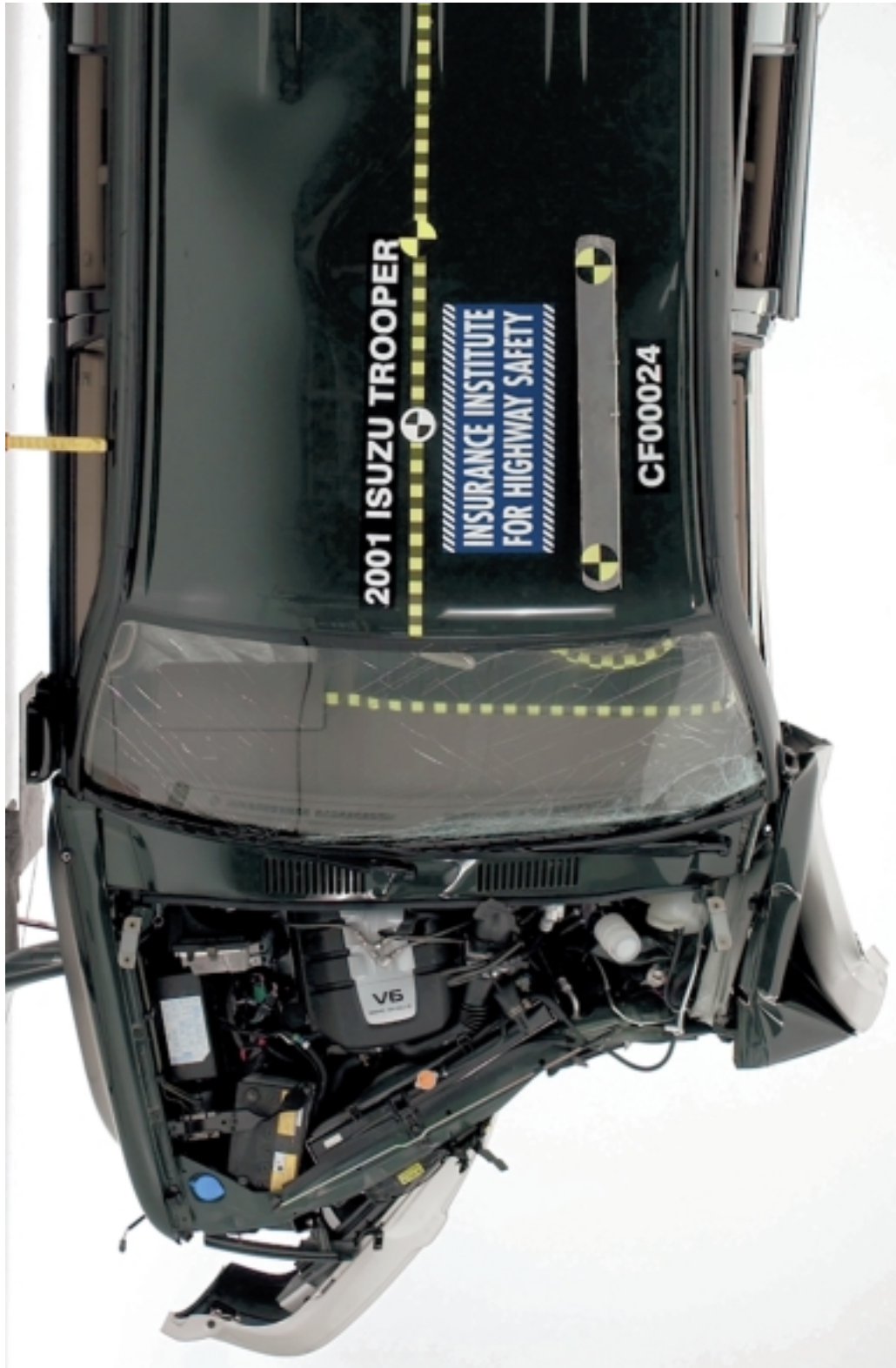
Figure 2 Overhead View of Crash Deformation — 2001 Isuzu Trooper
