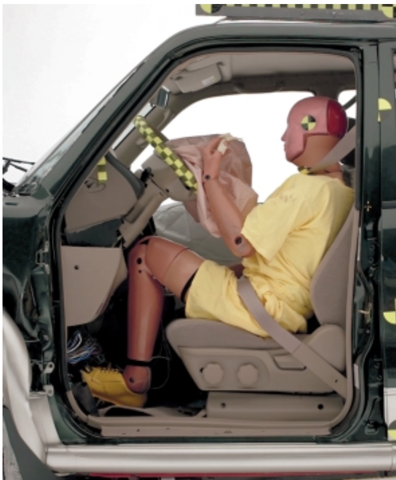
Figure 8 Dummy and Vehicle Interior, Postcrash — 2001 Isuzu Trooper
