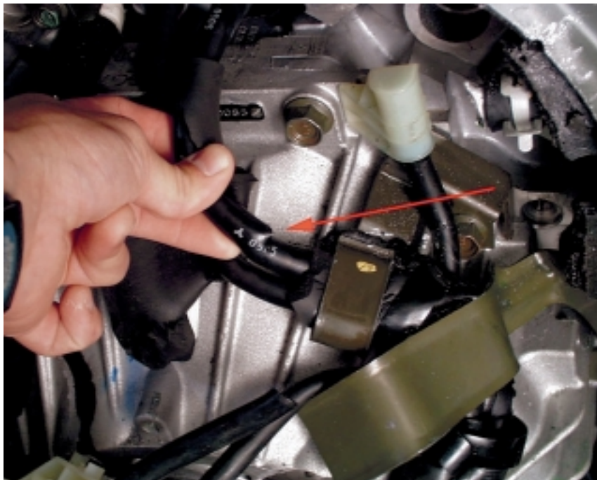
Figure 6 Close-up View of Torn Fuel Hose — 2001 Isuzu Trooper
