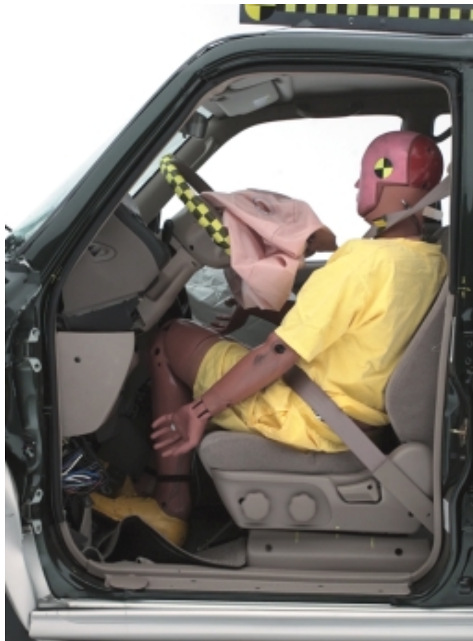
Figure 6 Dummy and Vehicle Interior, Postcrash — 2001 Isuzu Trooper
