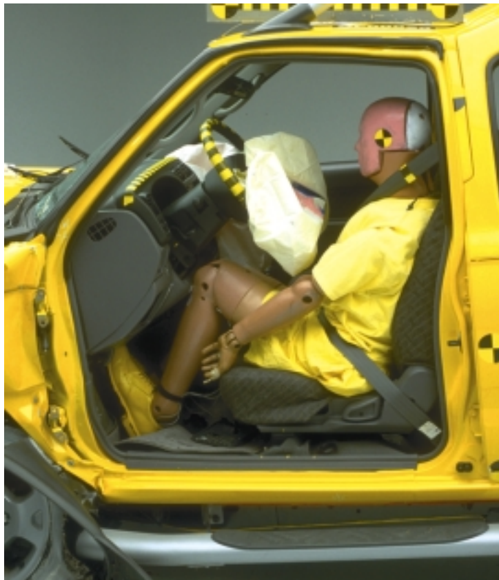
Figure 6 Dummy and Vehicle Interior, Postcrash — 2000 Nissan Xterra
