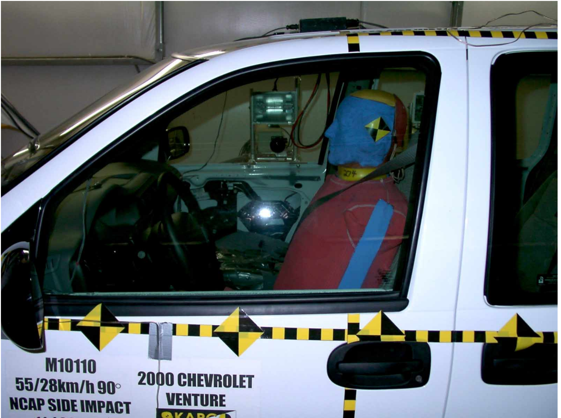
Figure A-19: Driver Dummy Left Side, Pre-test
