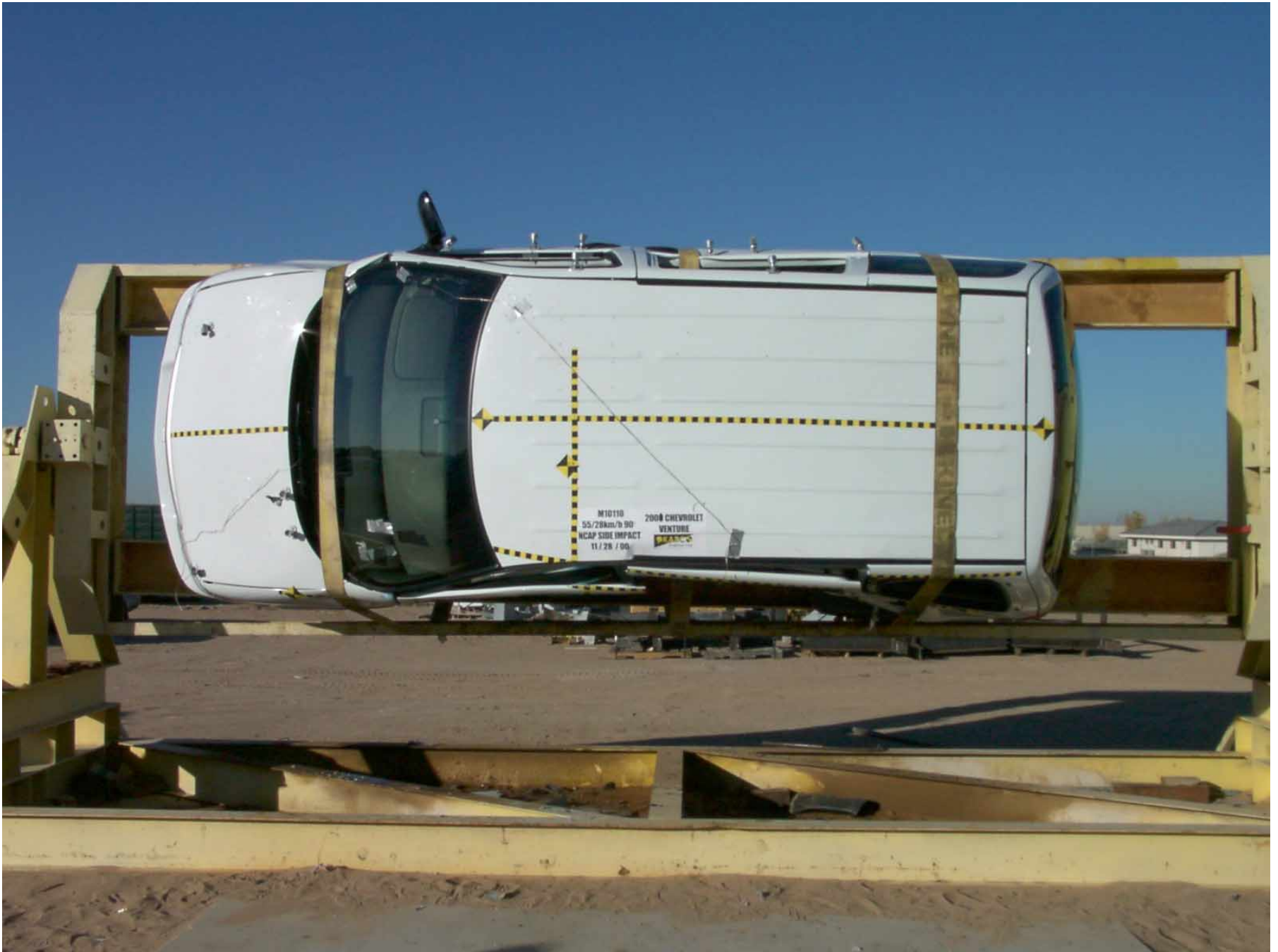
Figure A-44: Vehicle on Rollover Device, Top View
