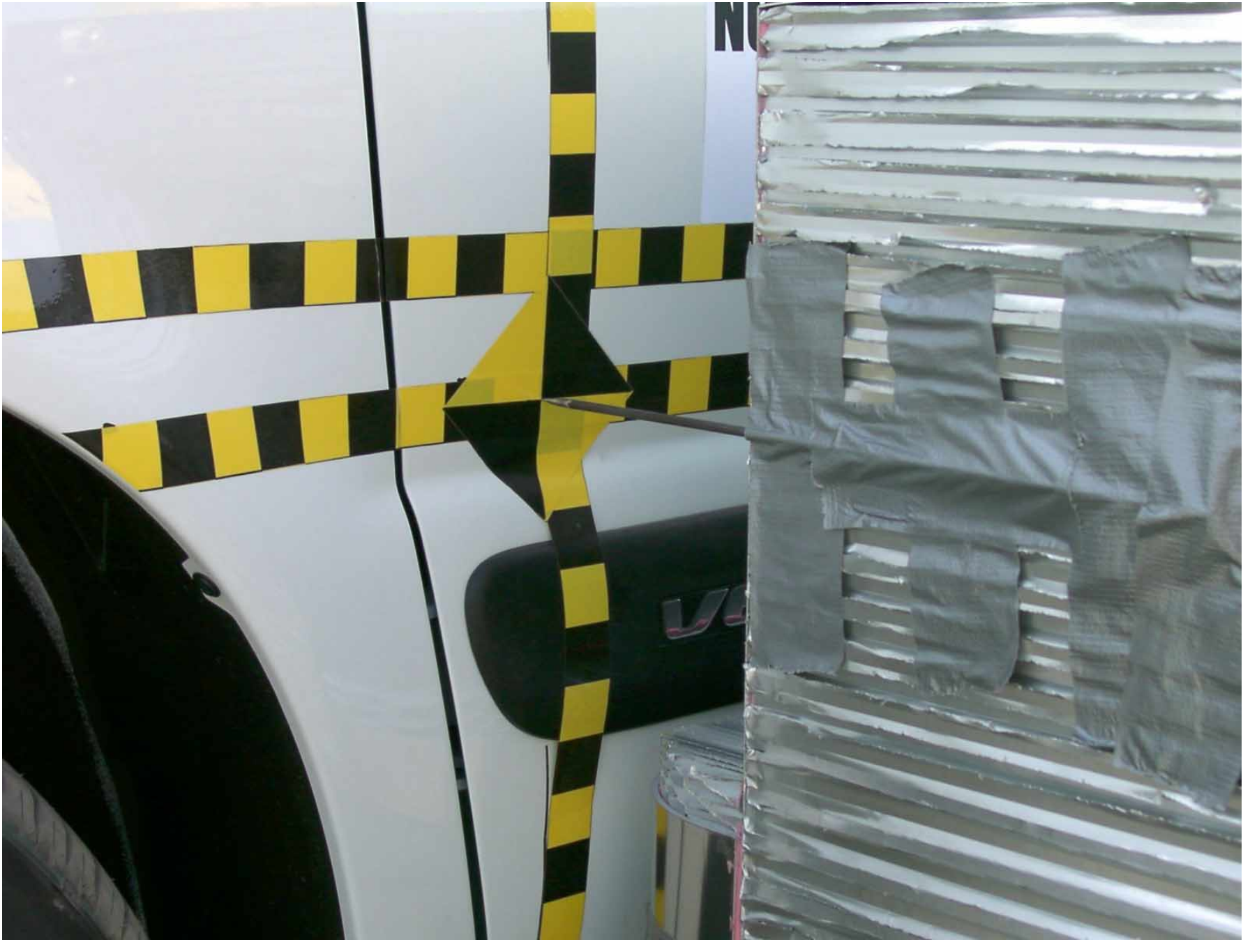
Figure A-16: Impact Point Target Close-up, Pre-Test
