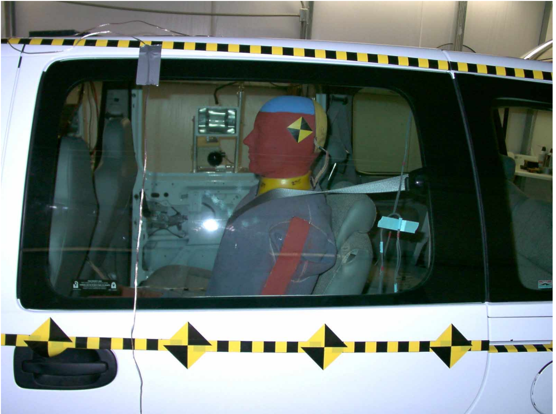
Figure A-28: Passenger Dummy Left Side, Pre-Test
