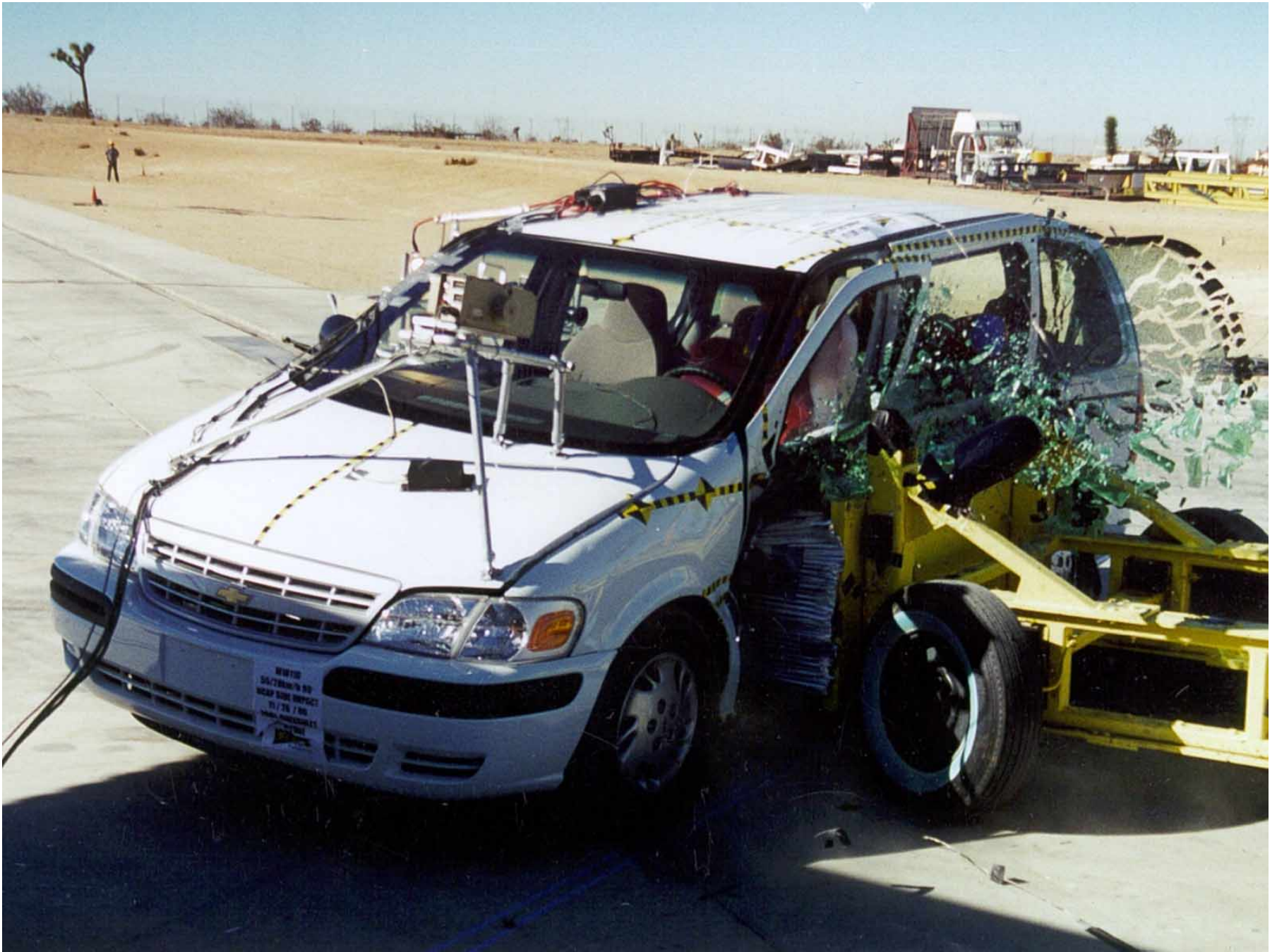
Figure A-45: Vehicle During Impact
