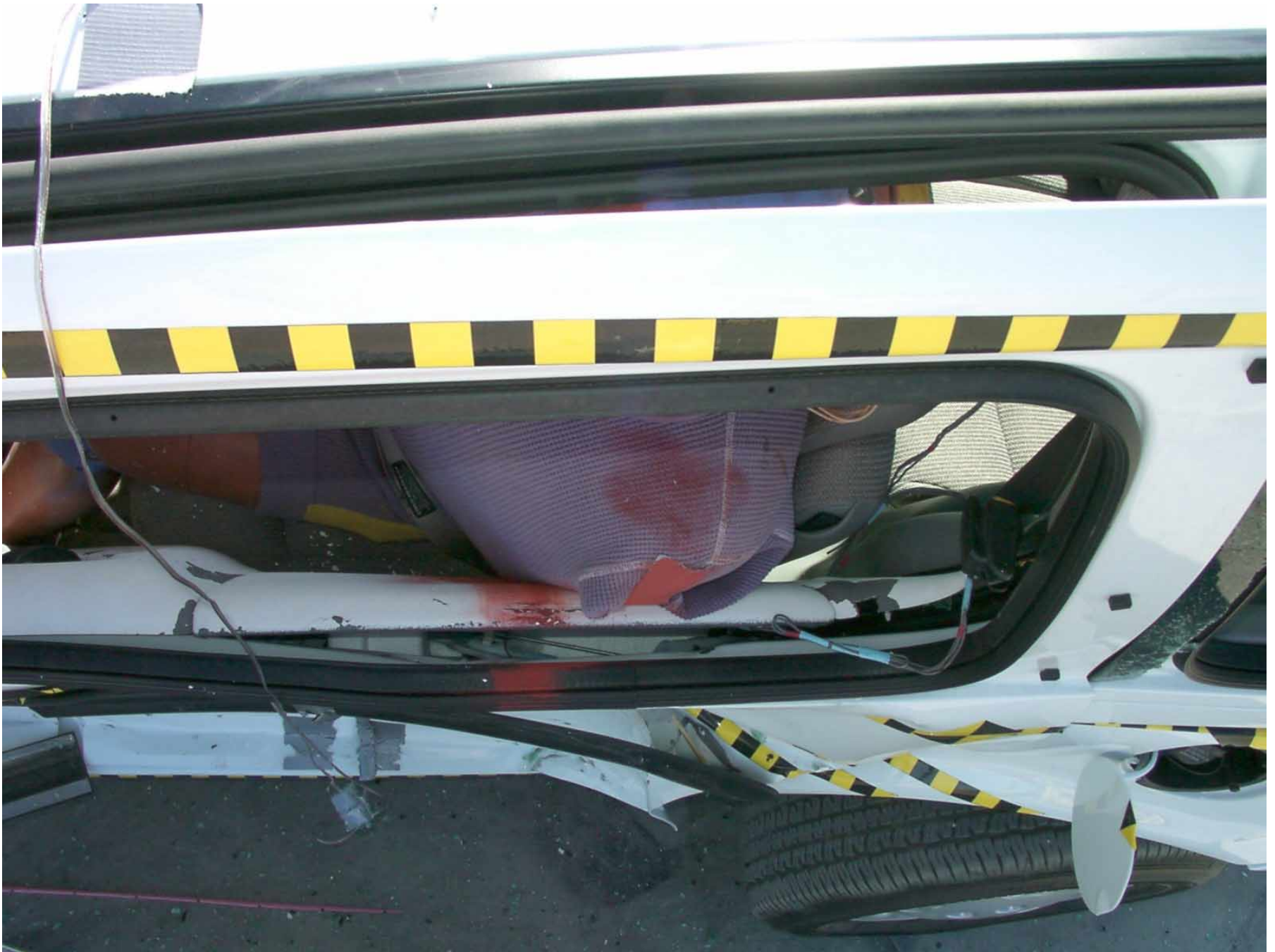
Figure A-31: Passenger Dummy Clearance, Post-Test
