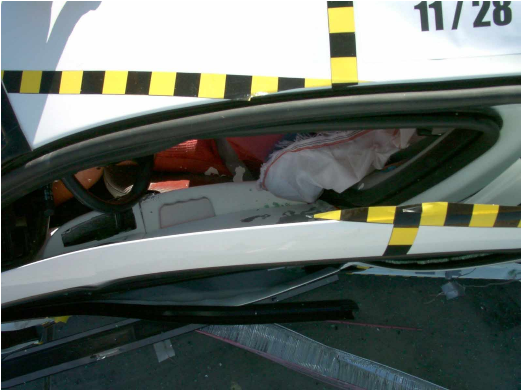
Figure A-22: Driver Dummy Clearance, Post-Test
