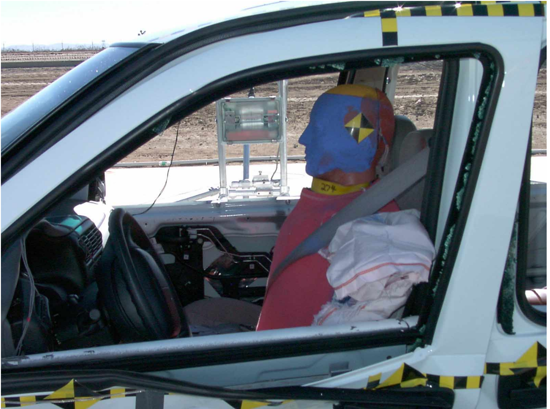
Figure A-20: Driver Dummy Left Side, Post-Test
