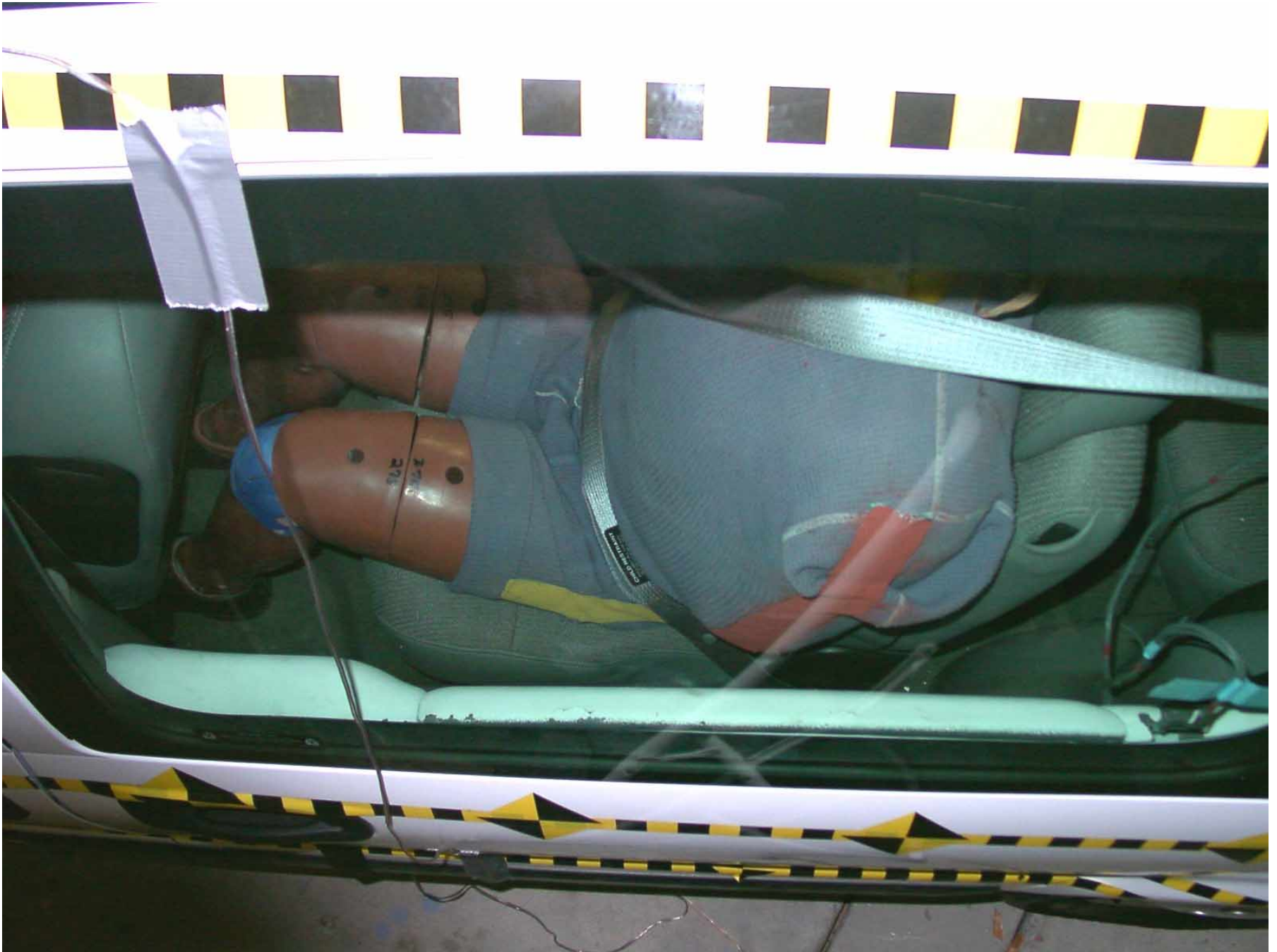
Figure A-30: Passenger Dummy Clearance, Pre-Test
