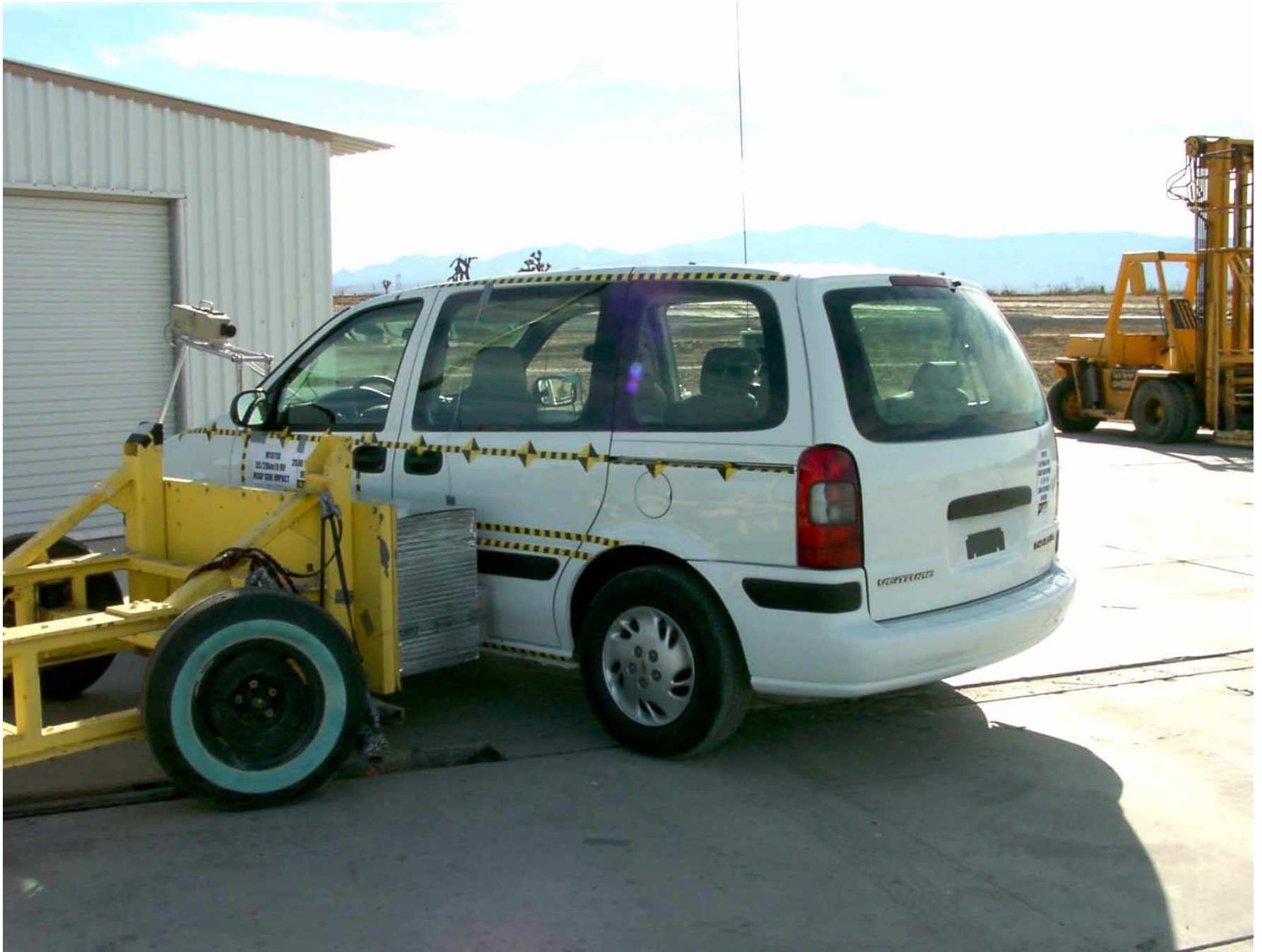
Figure A-15: MDB Right Side View at Impact Position, Pre-Test
