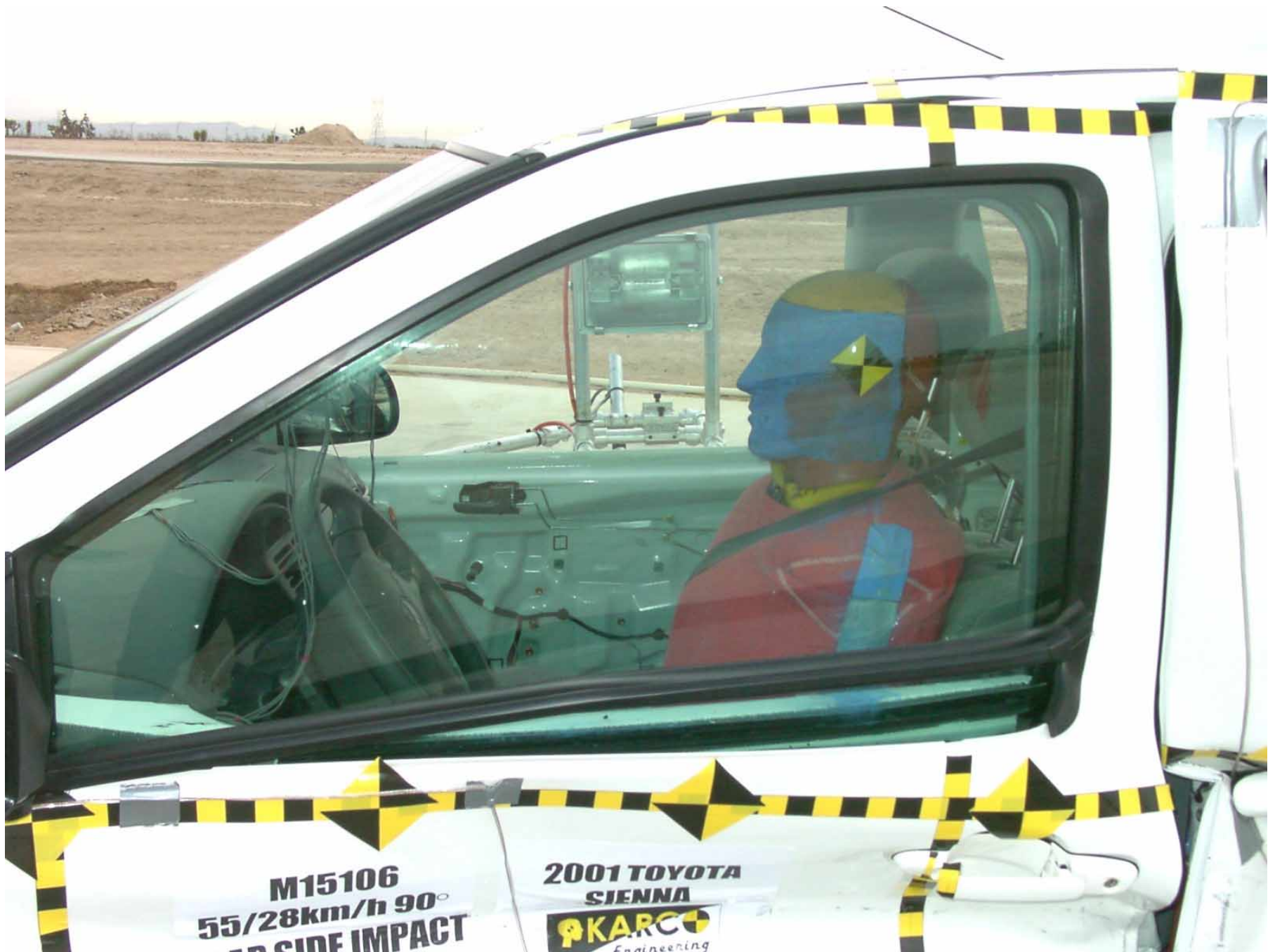
Figure A-20: Driver Dummy Left Side, Post-Test
