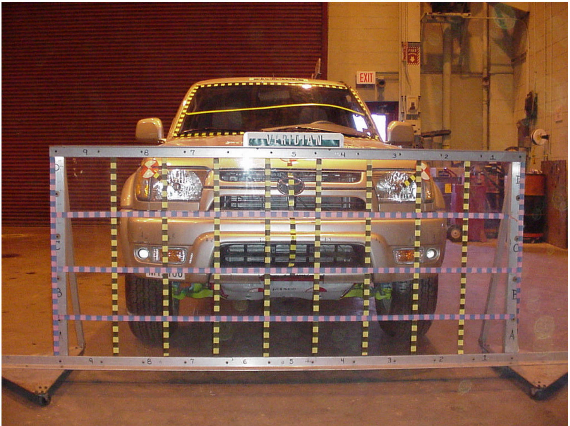
Figure A-1 LOAD CELL LOCATIONS
