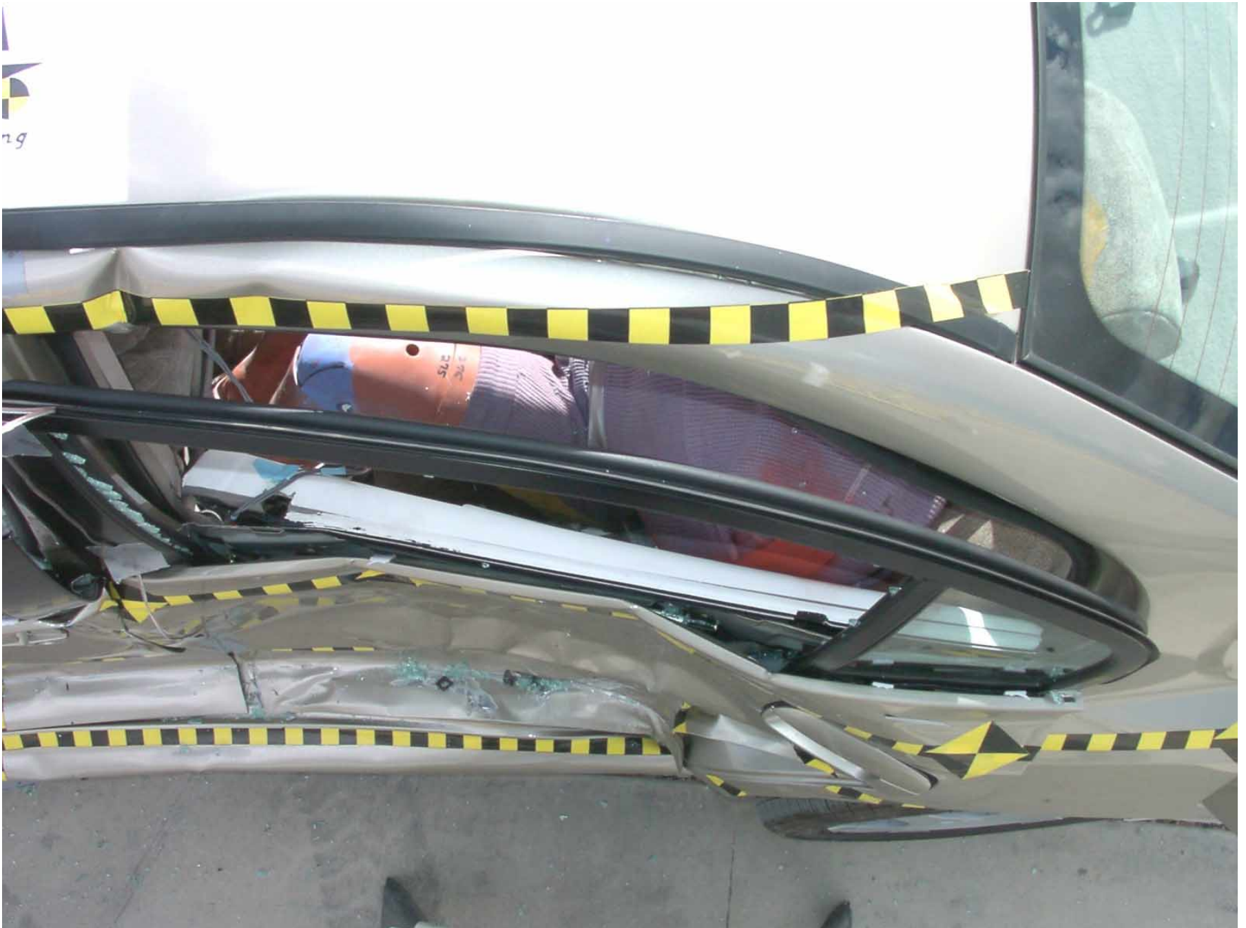
Figure A-31: Passenger Dummy Clearance, Post-Test
