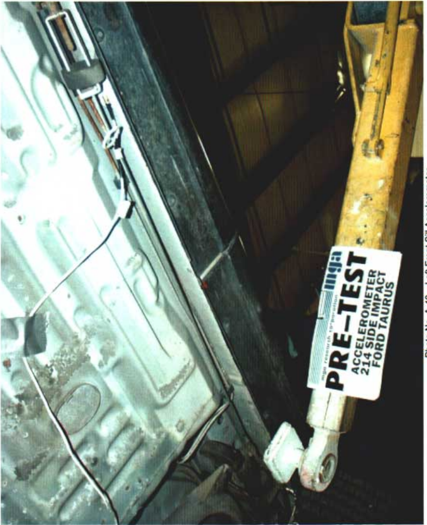
Photo No. A-40 - Left Front Sill Accelerometer
