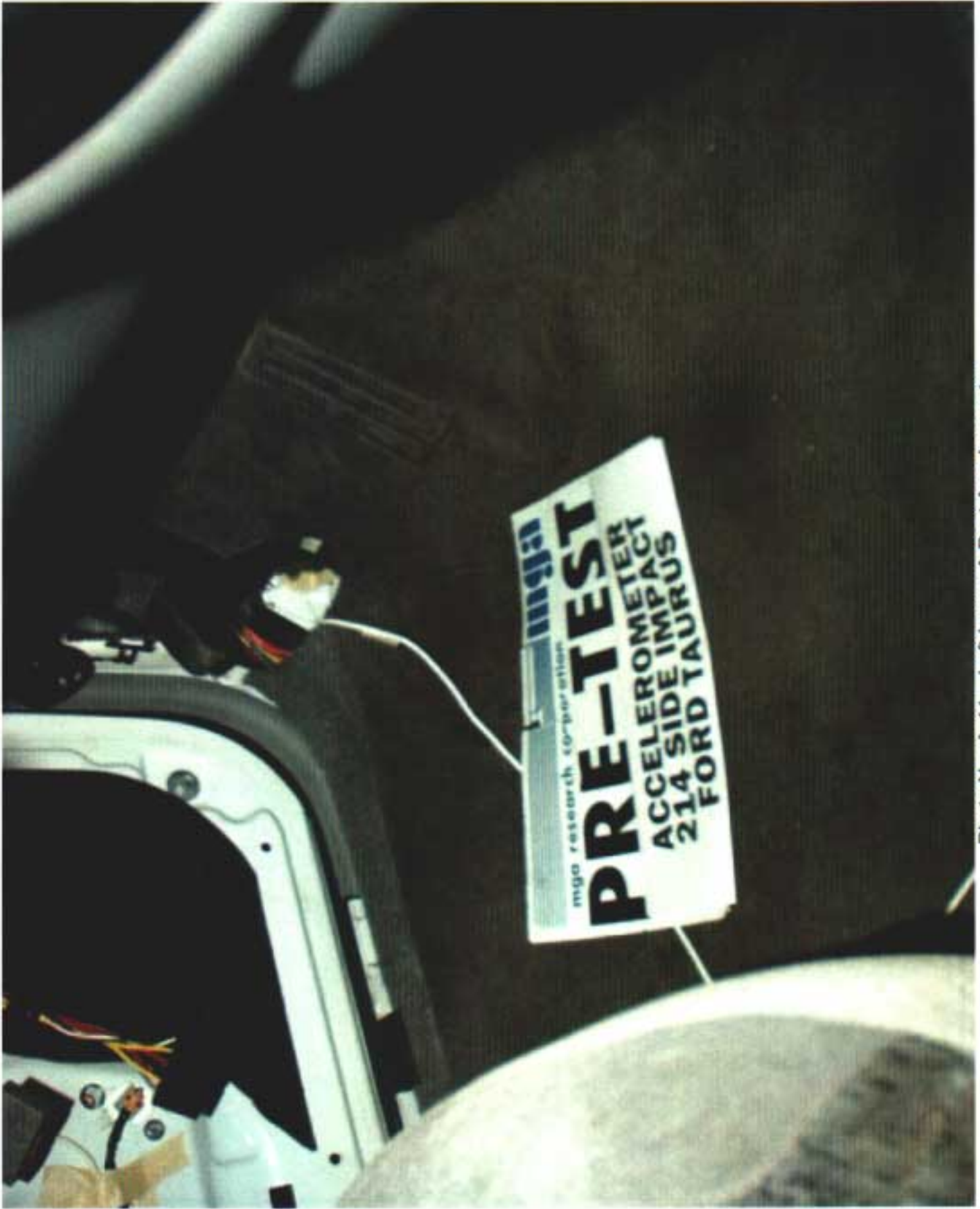
Photo No. A-44 - Left Lower A Post Accelerometer
