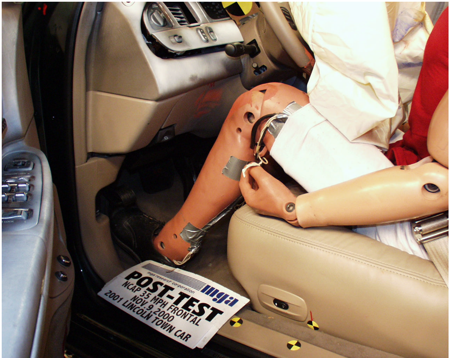
Photo No. A-27 - Post-Test Driver Dummy Knee Position
