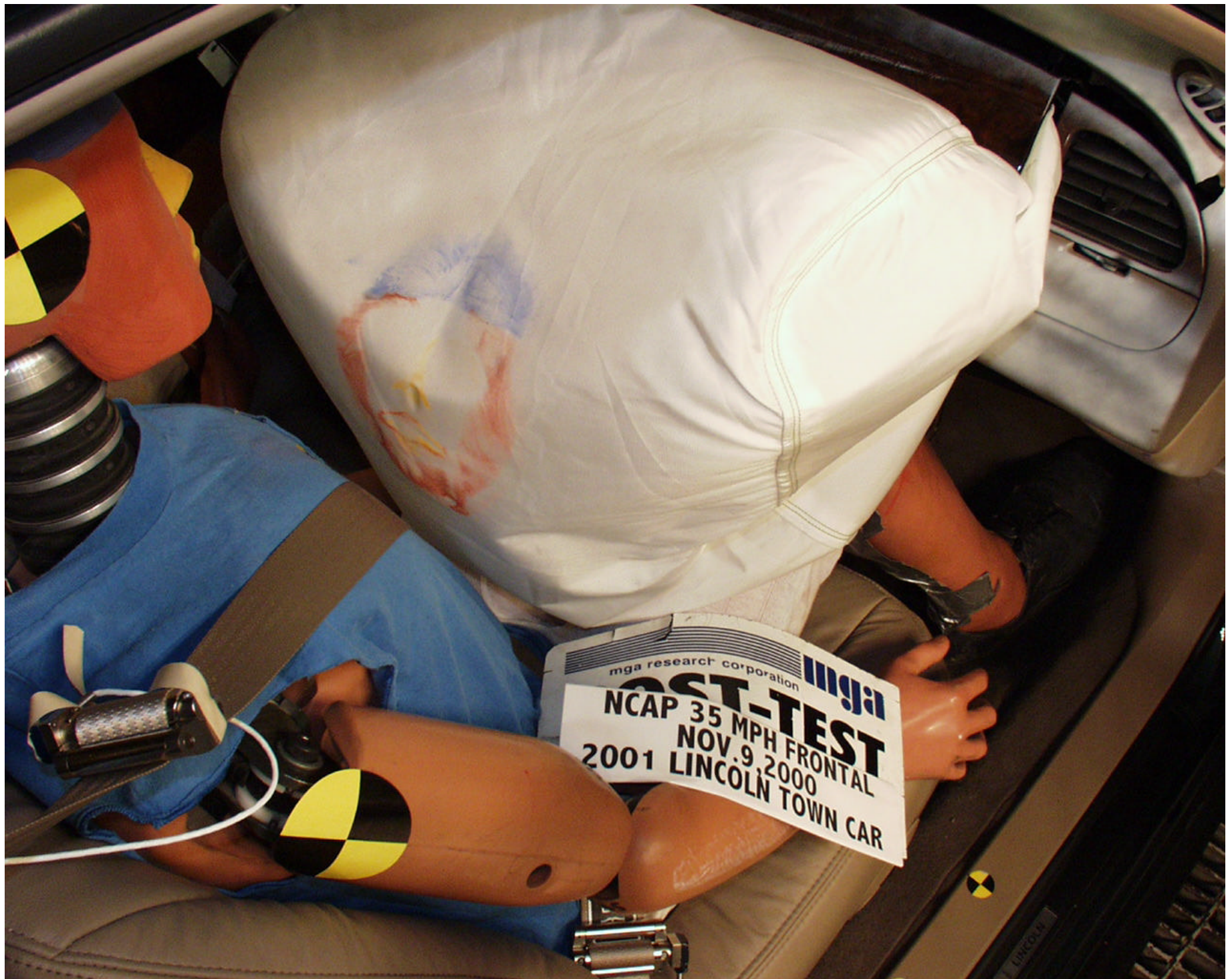
Photo No. A-40 - Post-Test Passenger Airbag Contact
