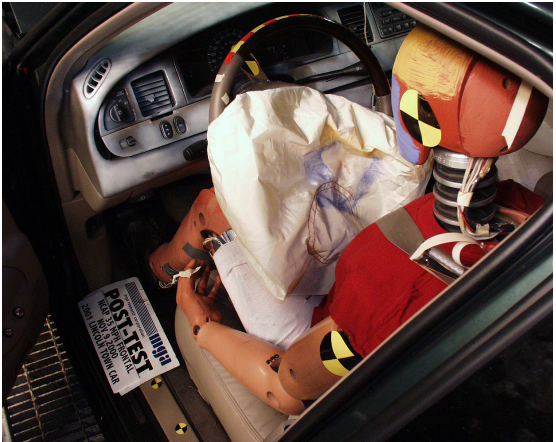
Photo No. A-28 - Post-Test Driver Airbag Contact
