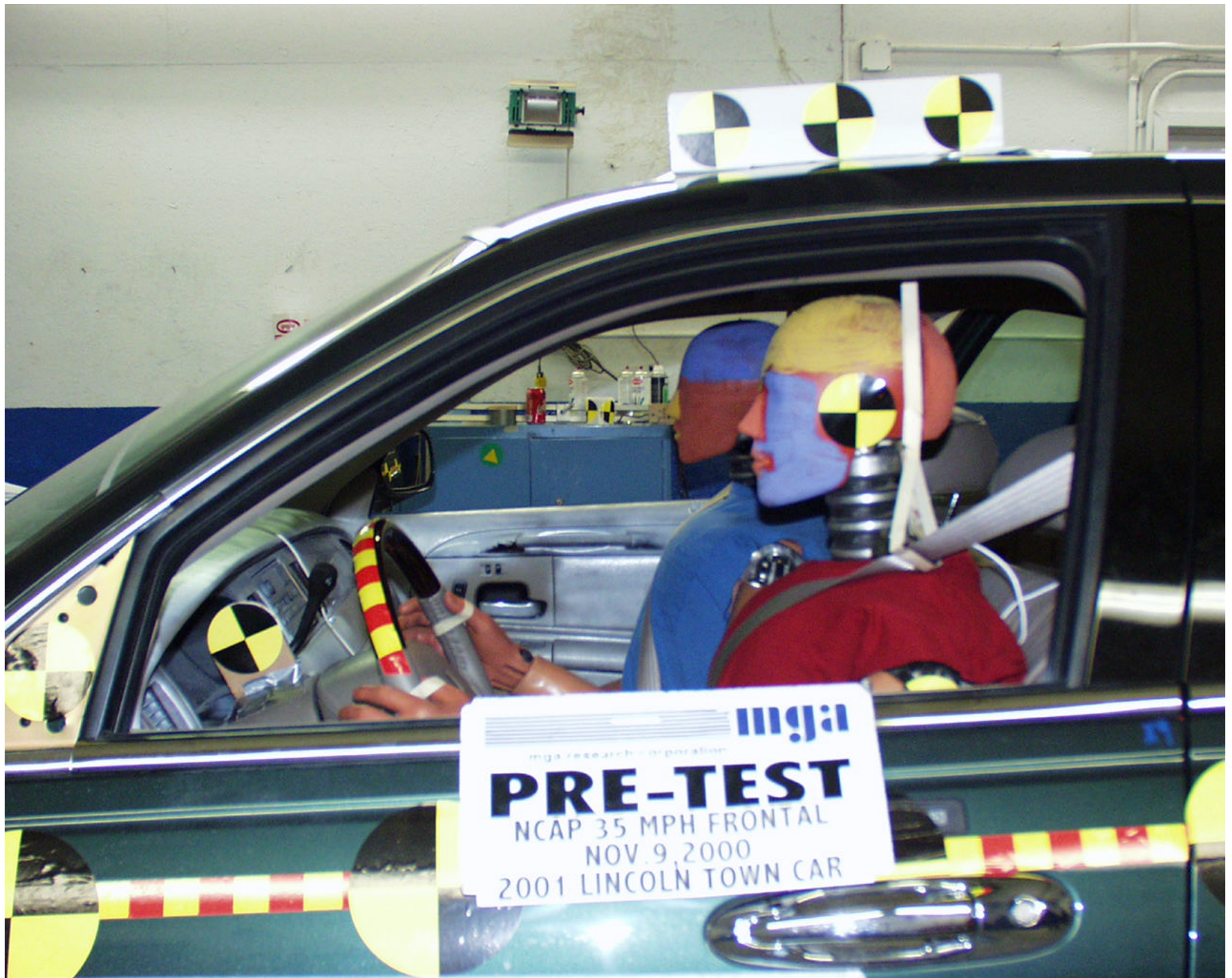
Photo No. A-20 - Pre-Test Driver Dummy Position Left Side View
