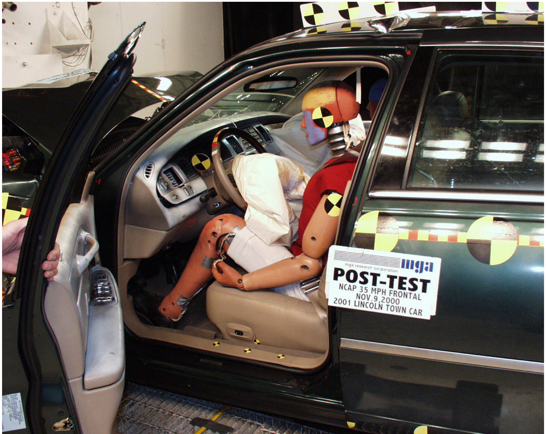
Photo No. A-23 - Post-Test Driver Dummy Position Left Side View (Door Open)
