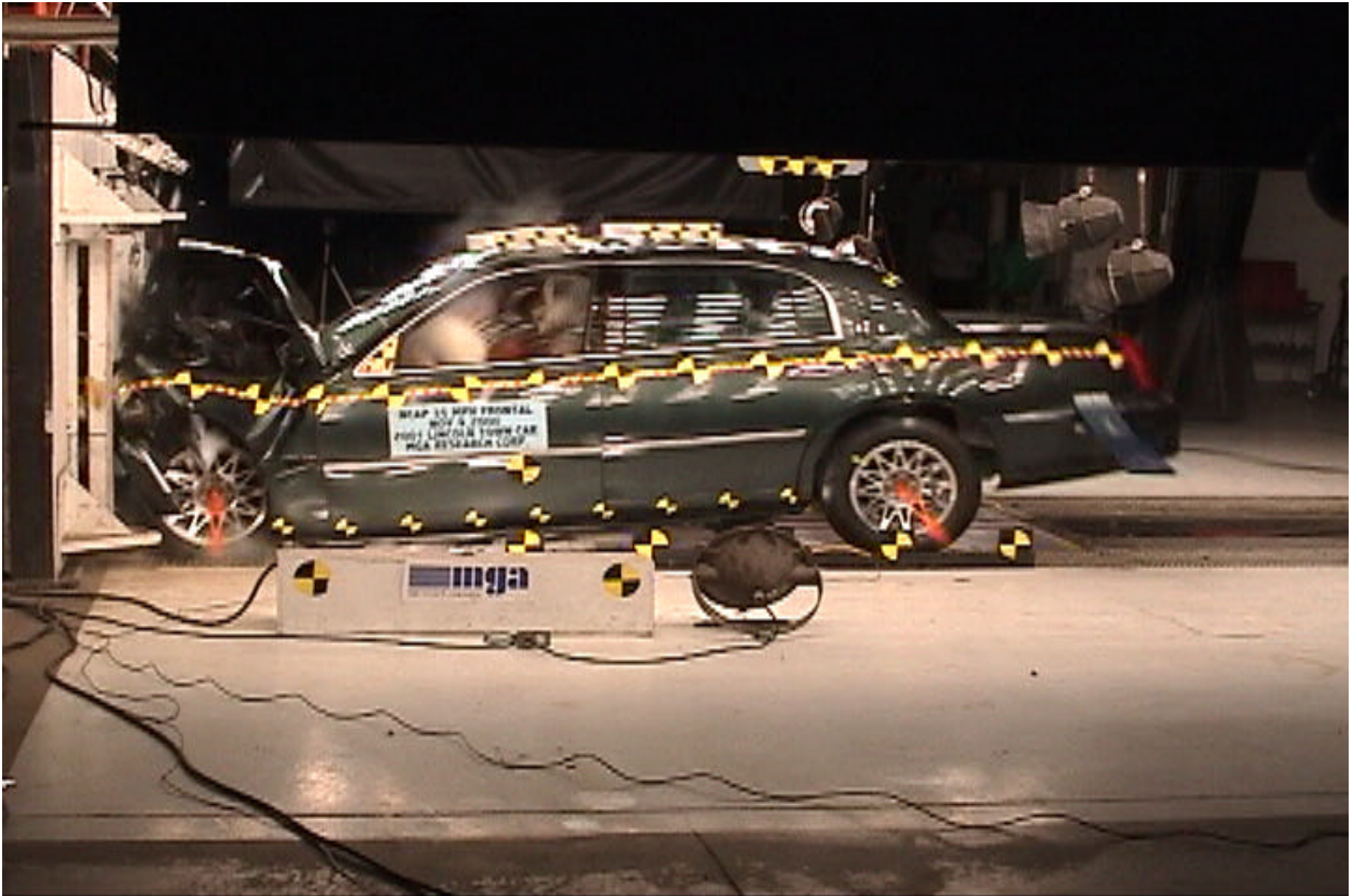
Photo No. A-44 - Vehicle Impact
