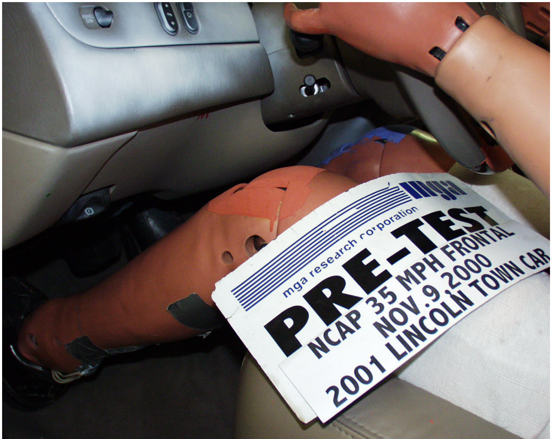
Photo No. A-26 - Pre-Test Driver Dummy Knee Position
