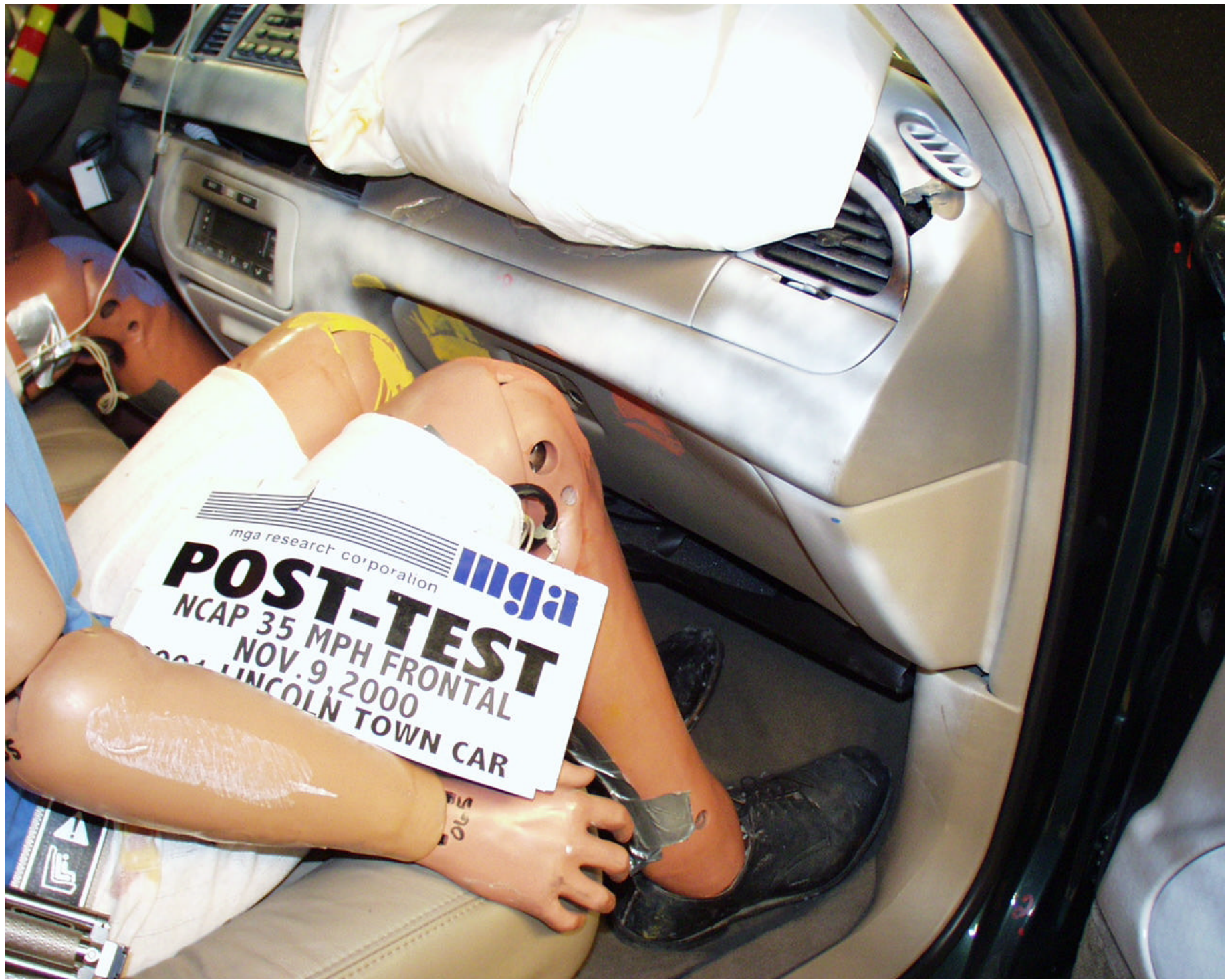
Photo No. A-39 - Post-Test Passenger Dummy Knee Position
