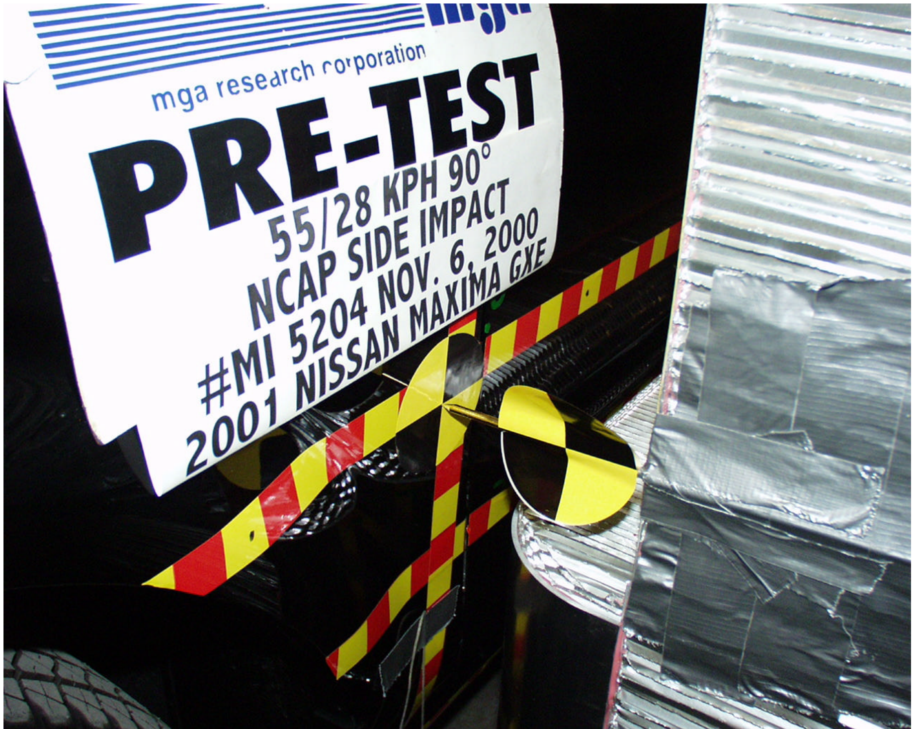
Photo No. A-36 - Pre-Test Left Front Impact Point on Vehicle
