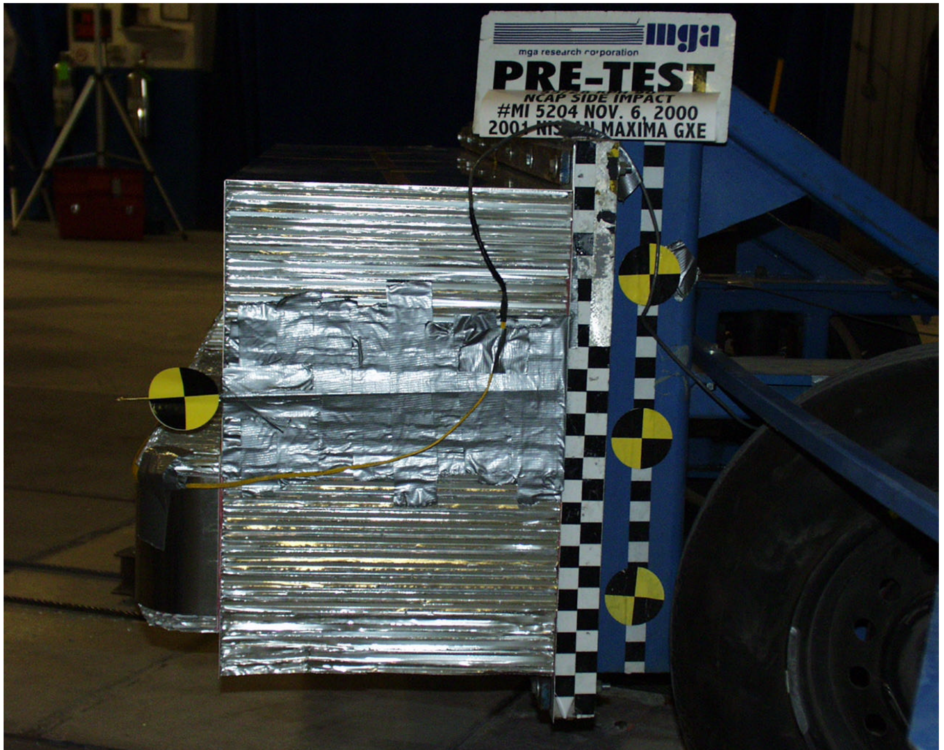
Photo No. A-16 - Pre-Test MDB Left Side View
