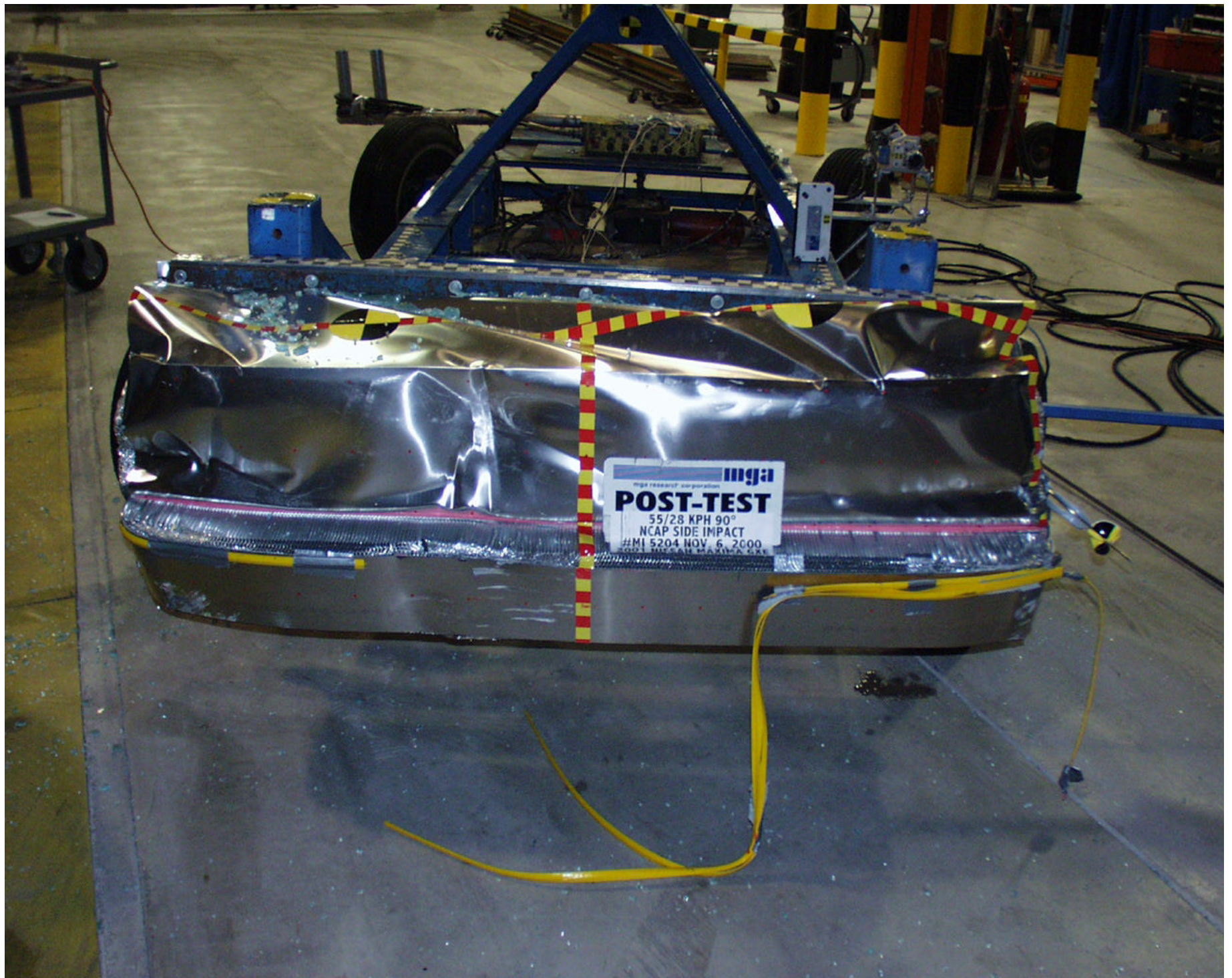
Photo No. A-13 - Post-Test MDB Front View
