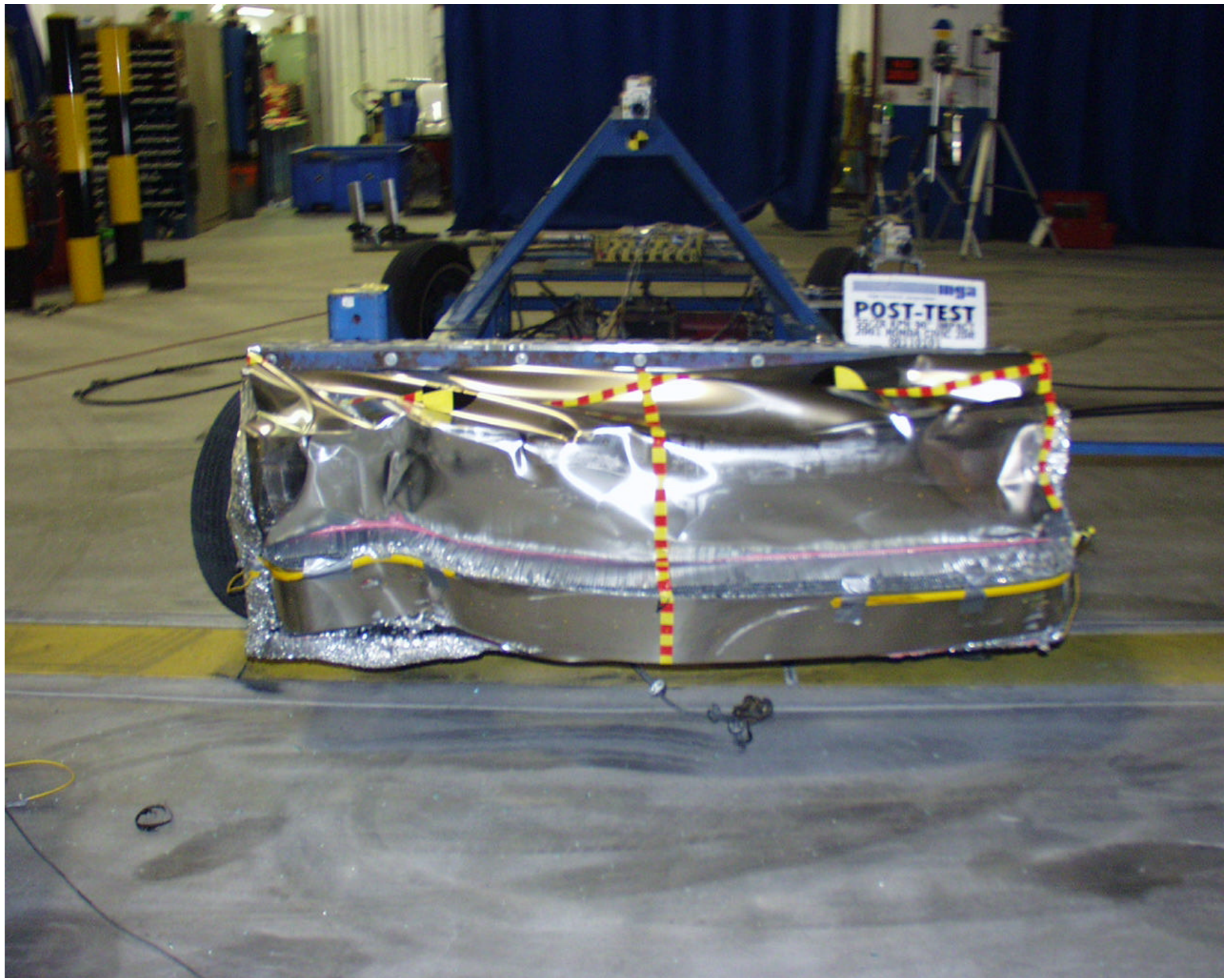
Photo No. A-12 - Post-Test MDB Front View
