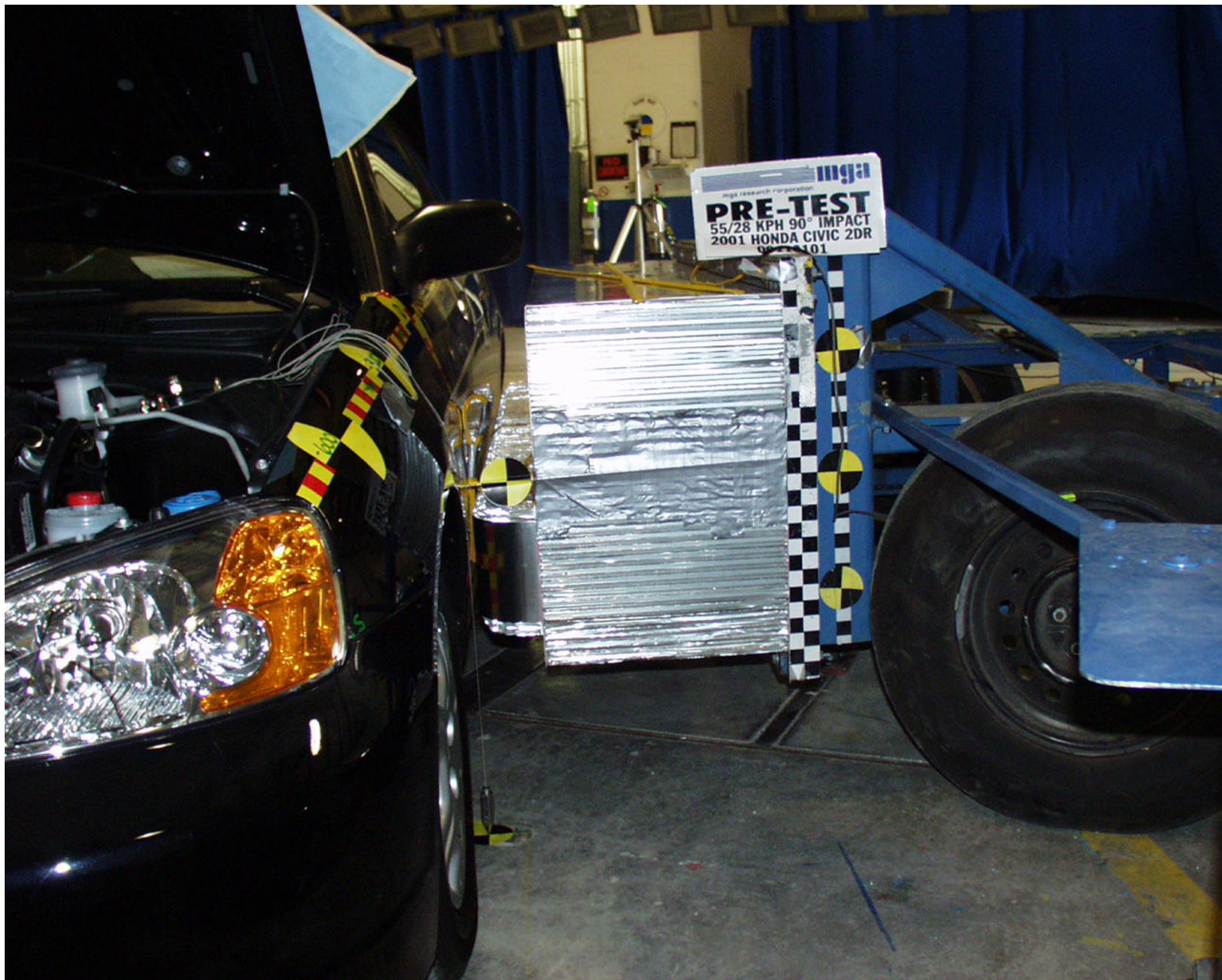
Photo No. A-7 - Pre-Test MDB Positioned Against Vehicle (left side)
