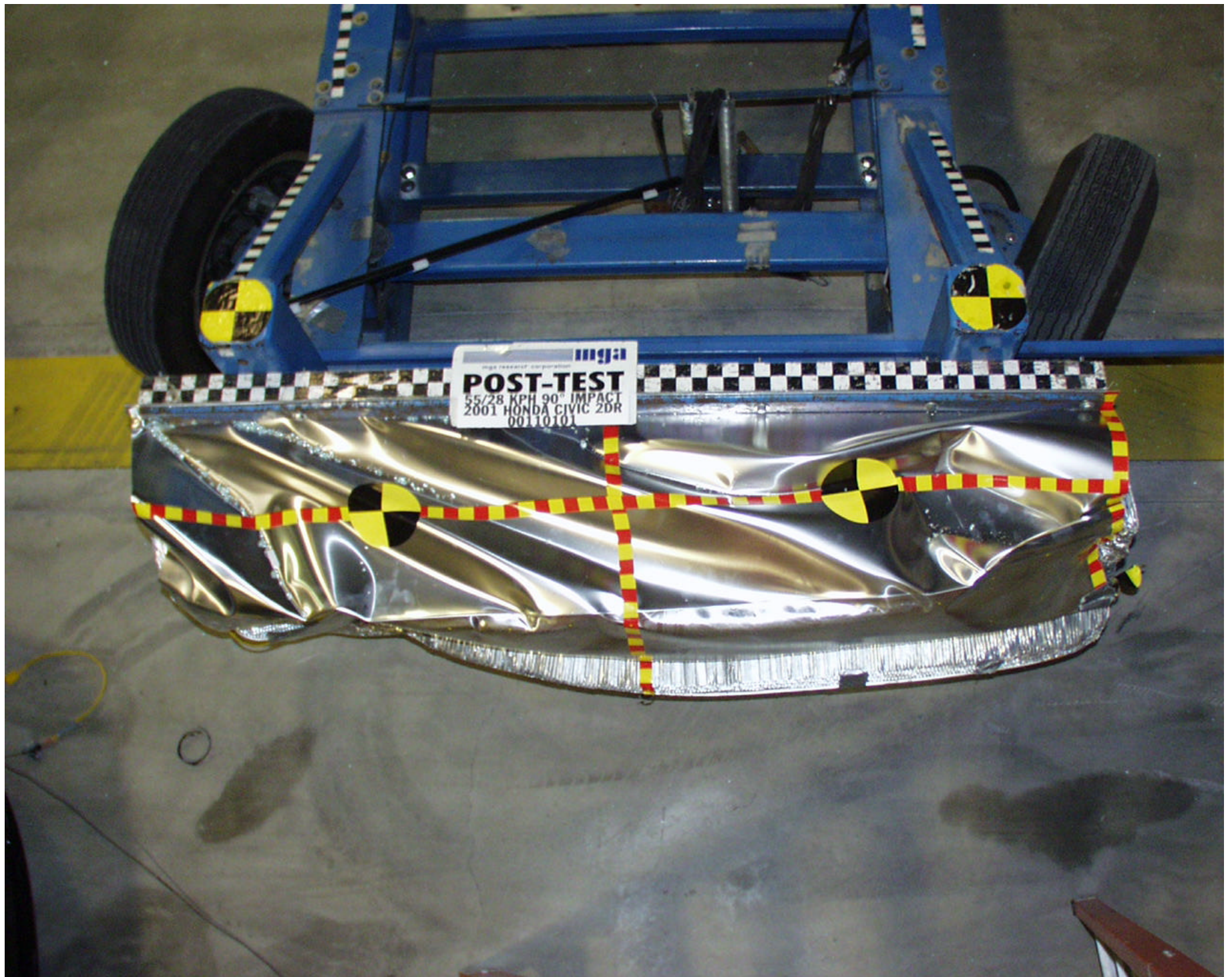
Photo No. A-10 - Post-Test MDB Top View
