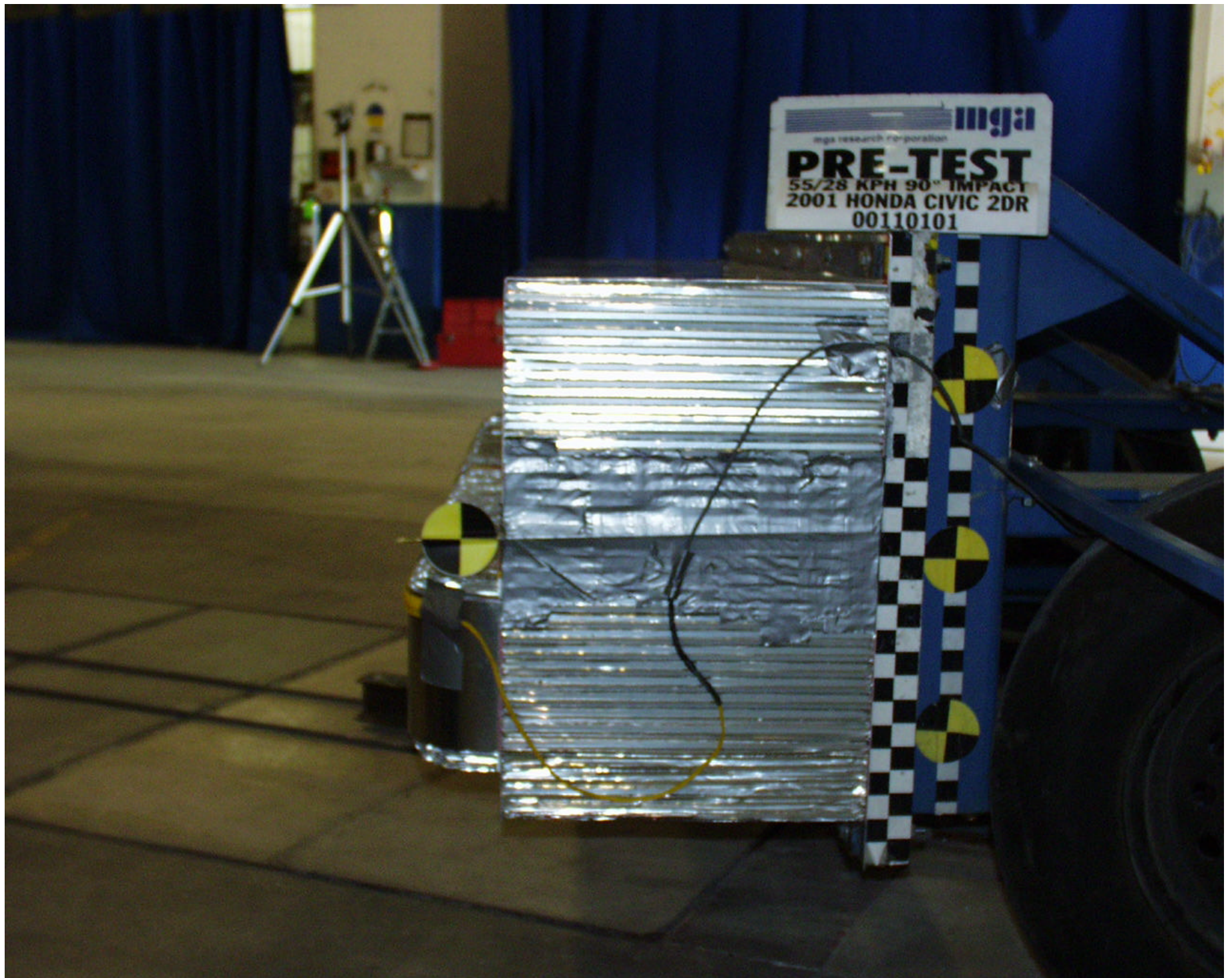
Photo No. A-15 - Pre-Test MDB Left Side View
