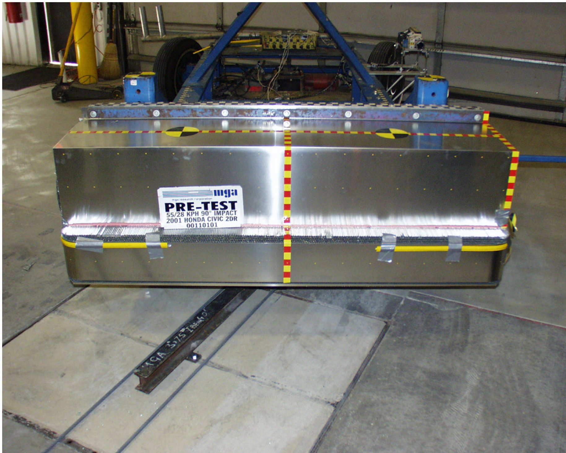
Photo No. A-11 - Pre-Test MDB Front View
