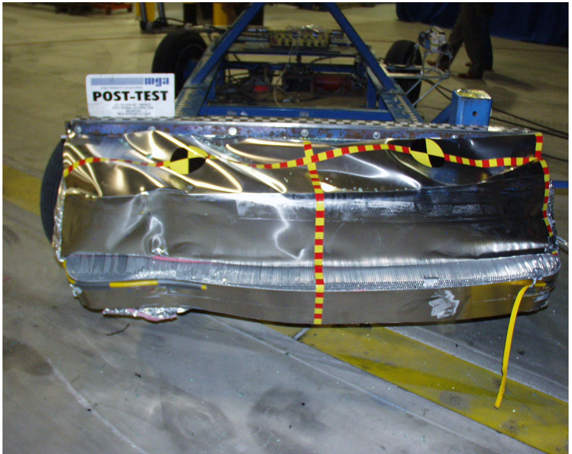
Photo No. A-8 - Post-Test MDB Front View
