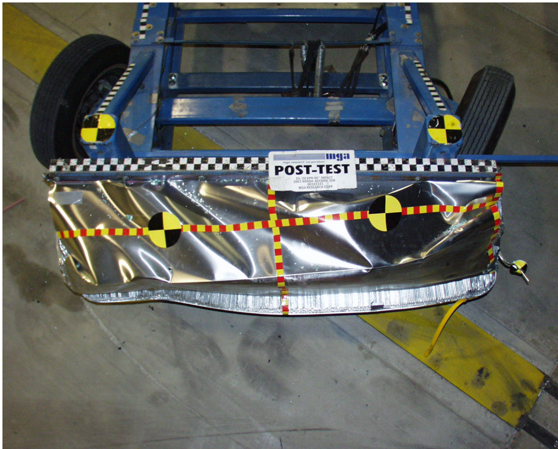
Photo No. A-7 - Post-Test MDB Top View
