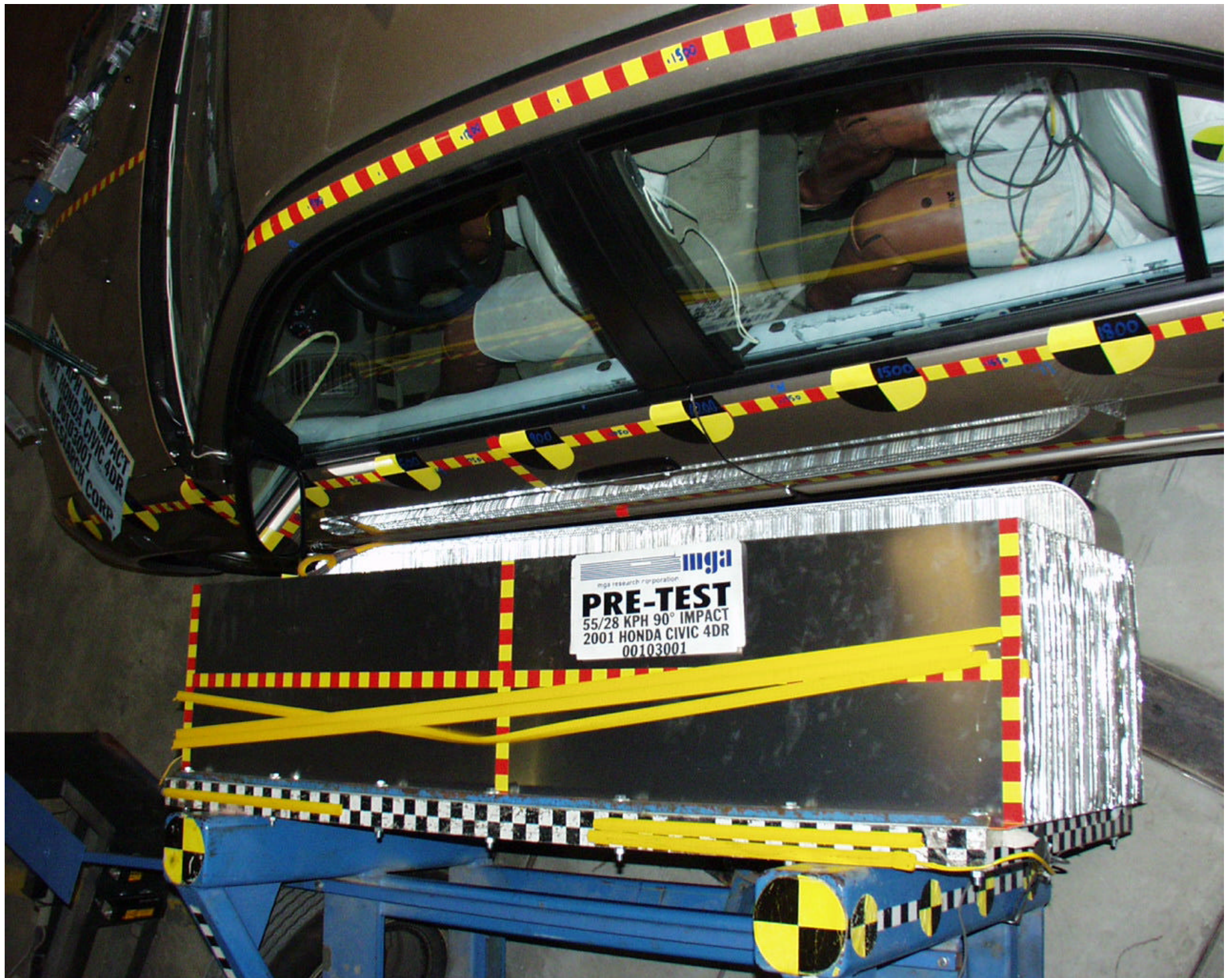
Photo No. A-9 - Pre-Test MDB Positioned Against Vehicle Overhead View
