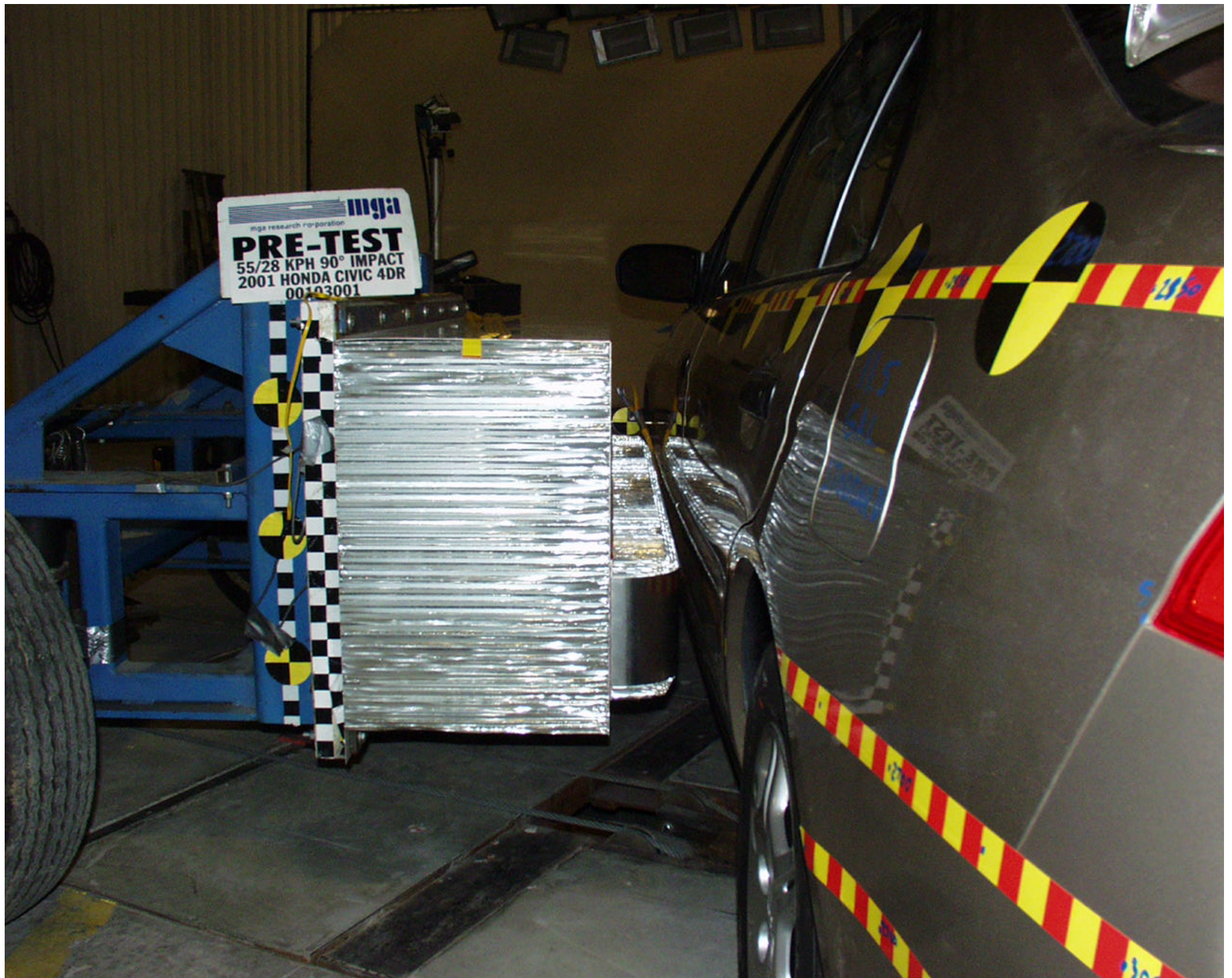
Photo No. A-8 - Pre-Test MDB Positioned Against Vehicle (right side)
