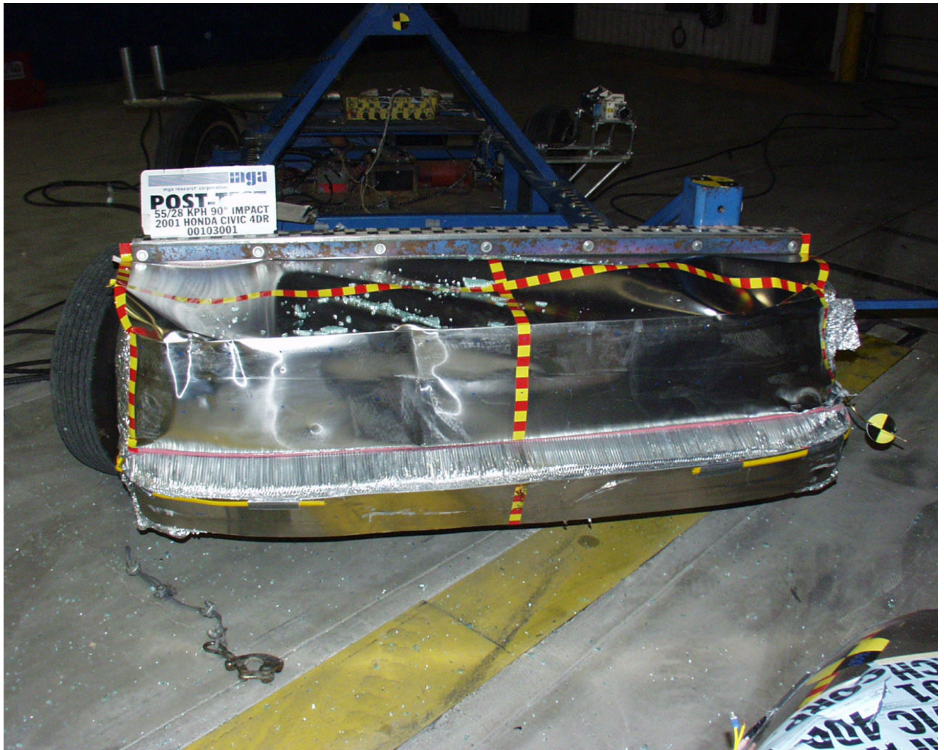
Photo No. A-15 - Post-Test MDB Front View
