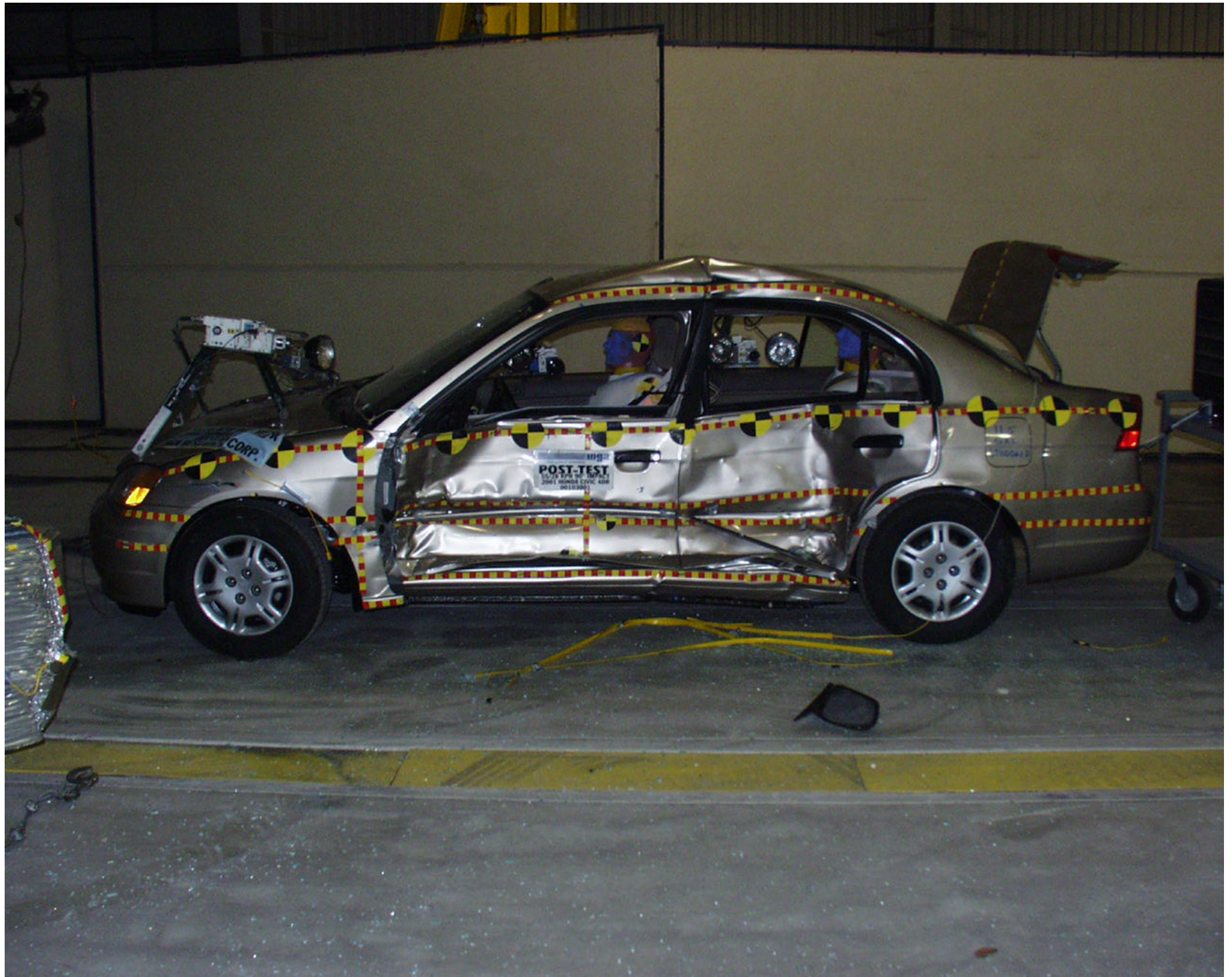
Photo No. A-6 - Post-Test Left Side View of Test Vehicle
