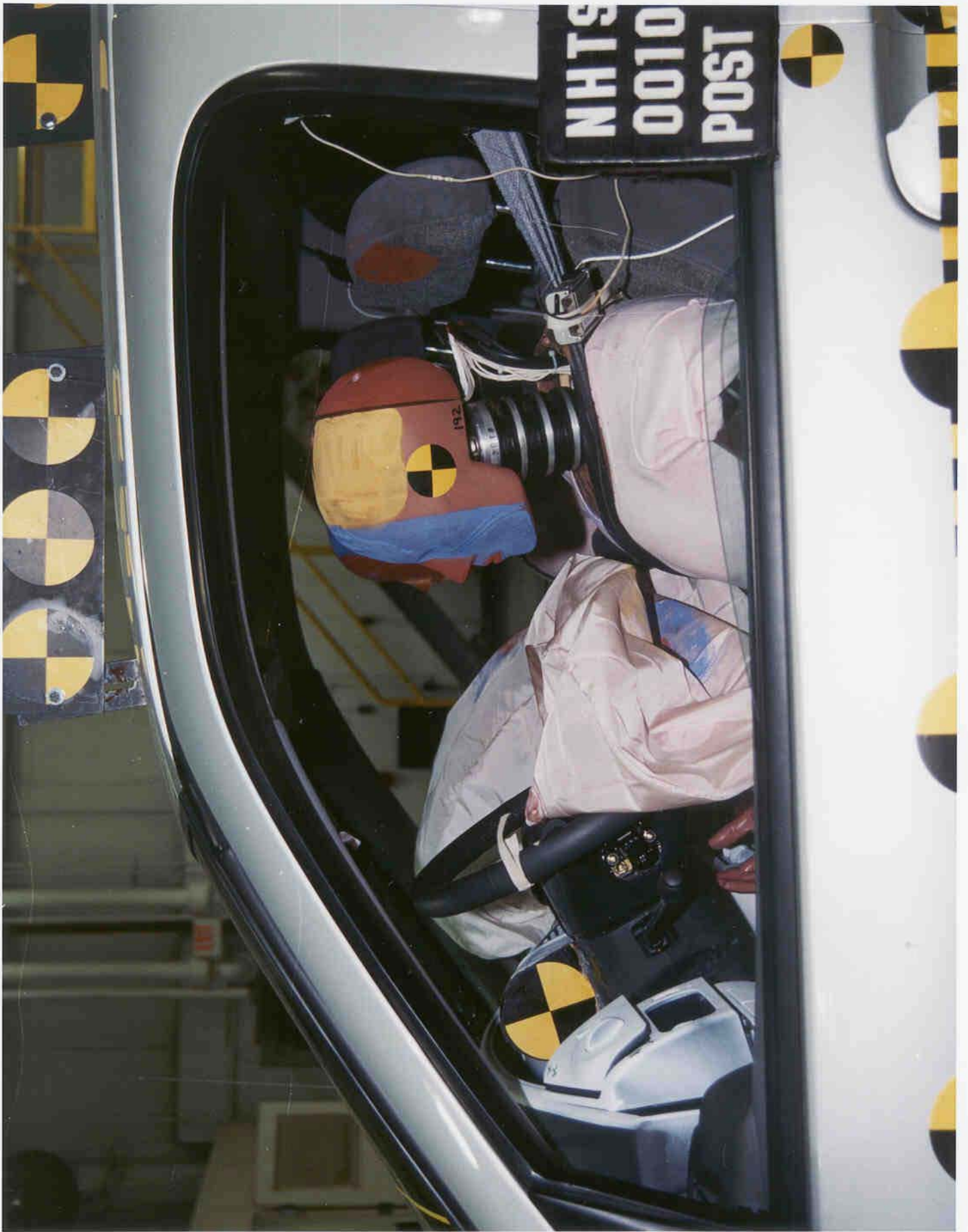
Figure A-35 Post-Test Driver Dummy Position - View 2
