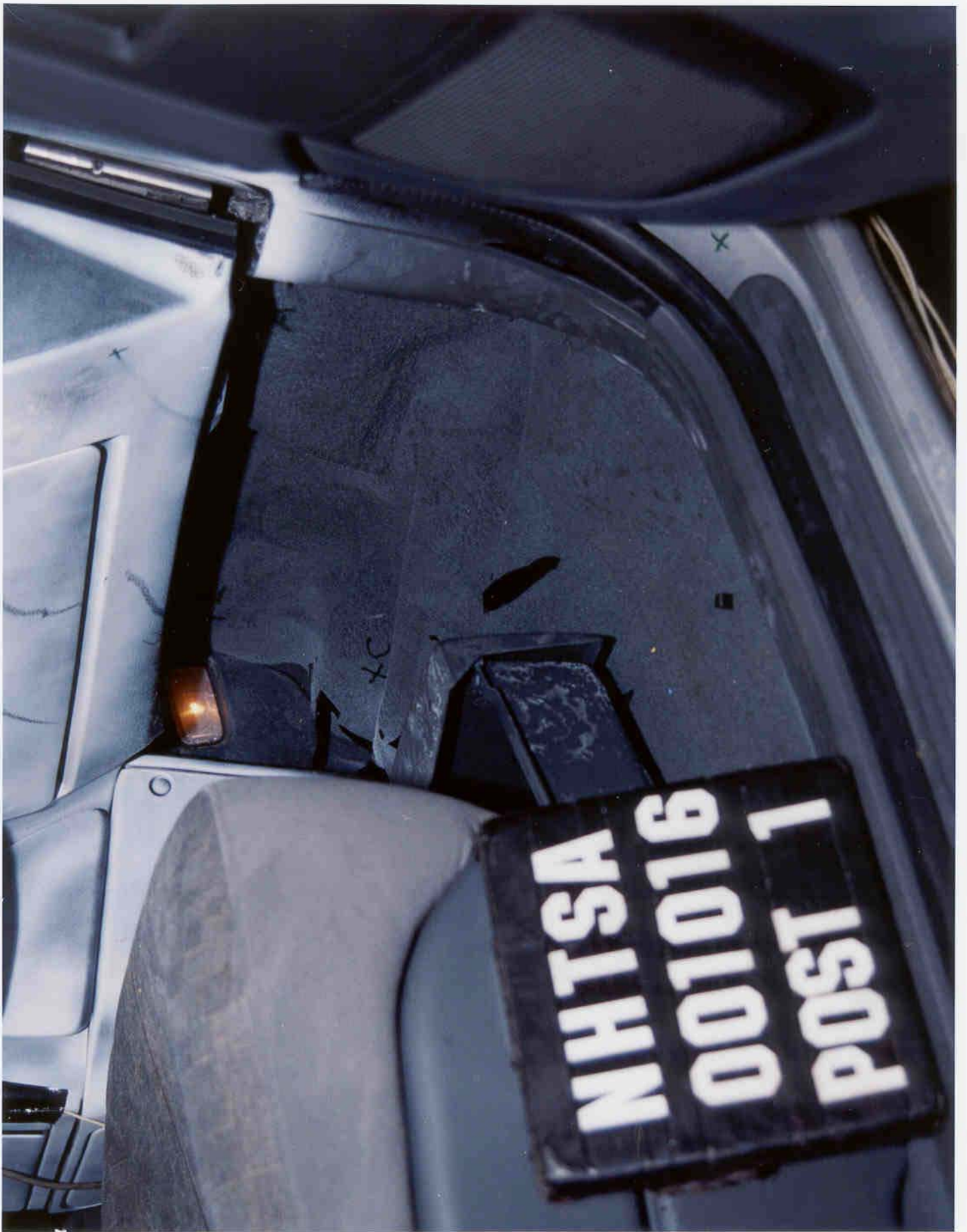
Figure A-61 Post-Test Passenger Floor Deformation View A-62
