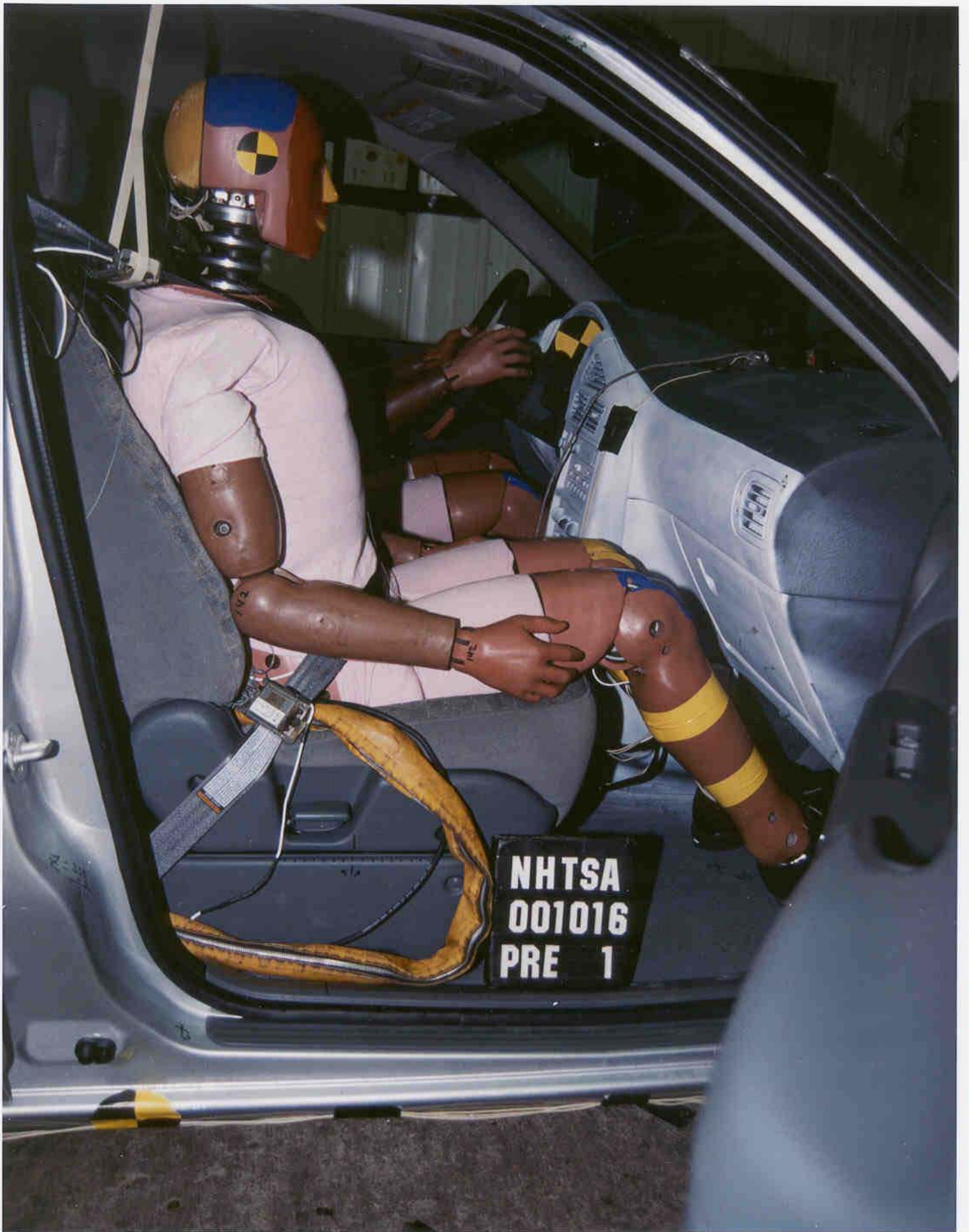
Figure A-44 Pre-Test Passenger Dummy & Vehicle Interior - View 1
