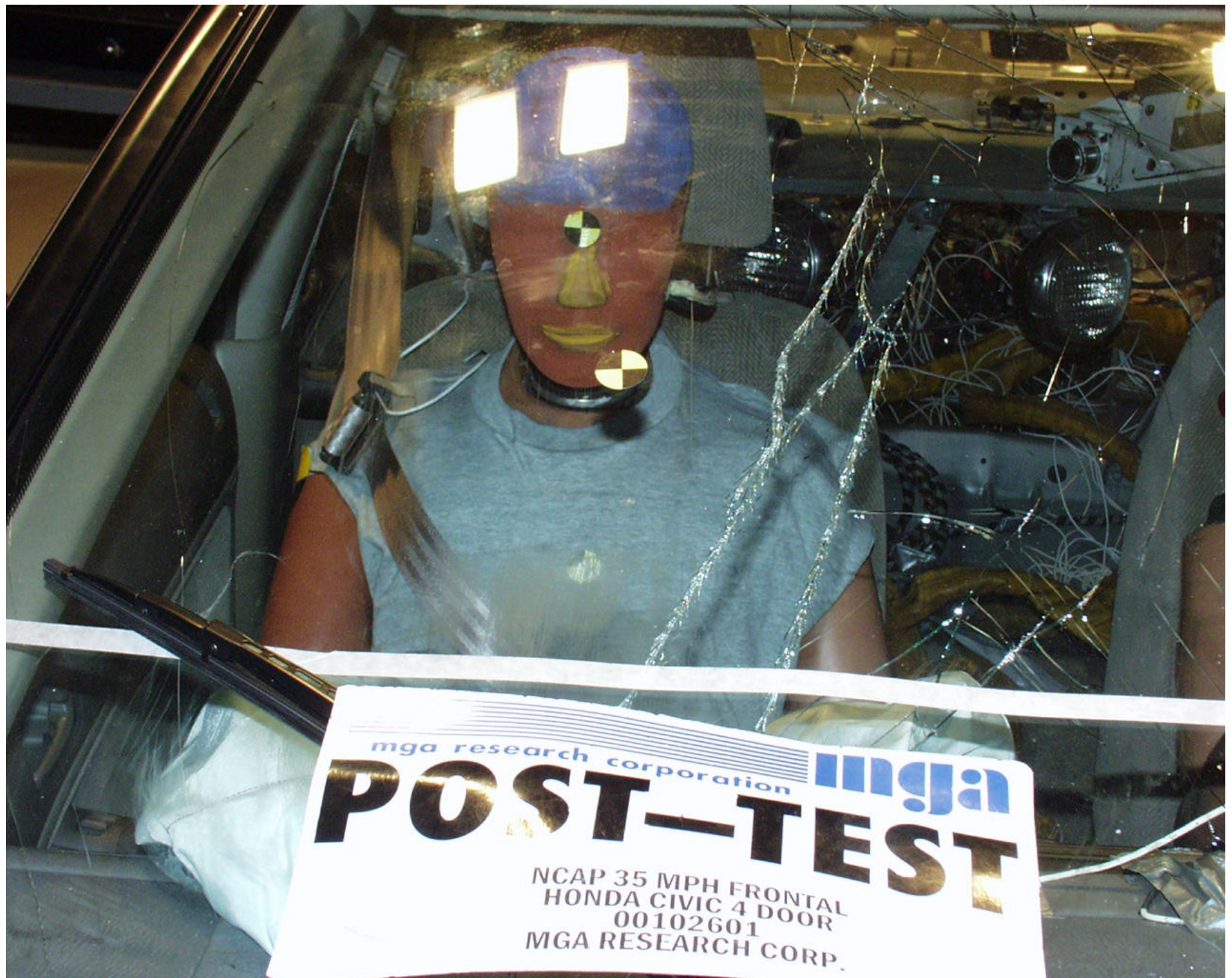
Photo No. A-46 - Post-Test Passenger Windshield View
