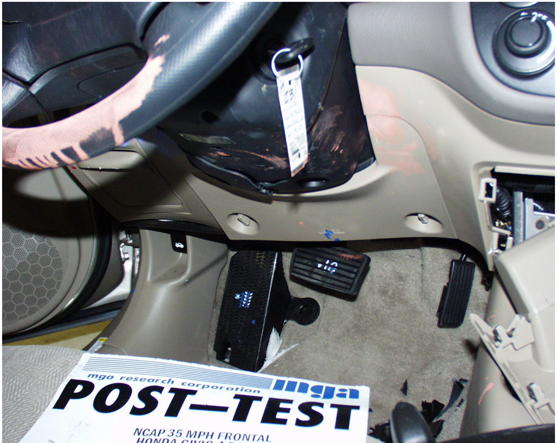
Photo No. A-32 - Post-Test Driver Knee Contact View
