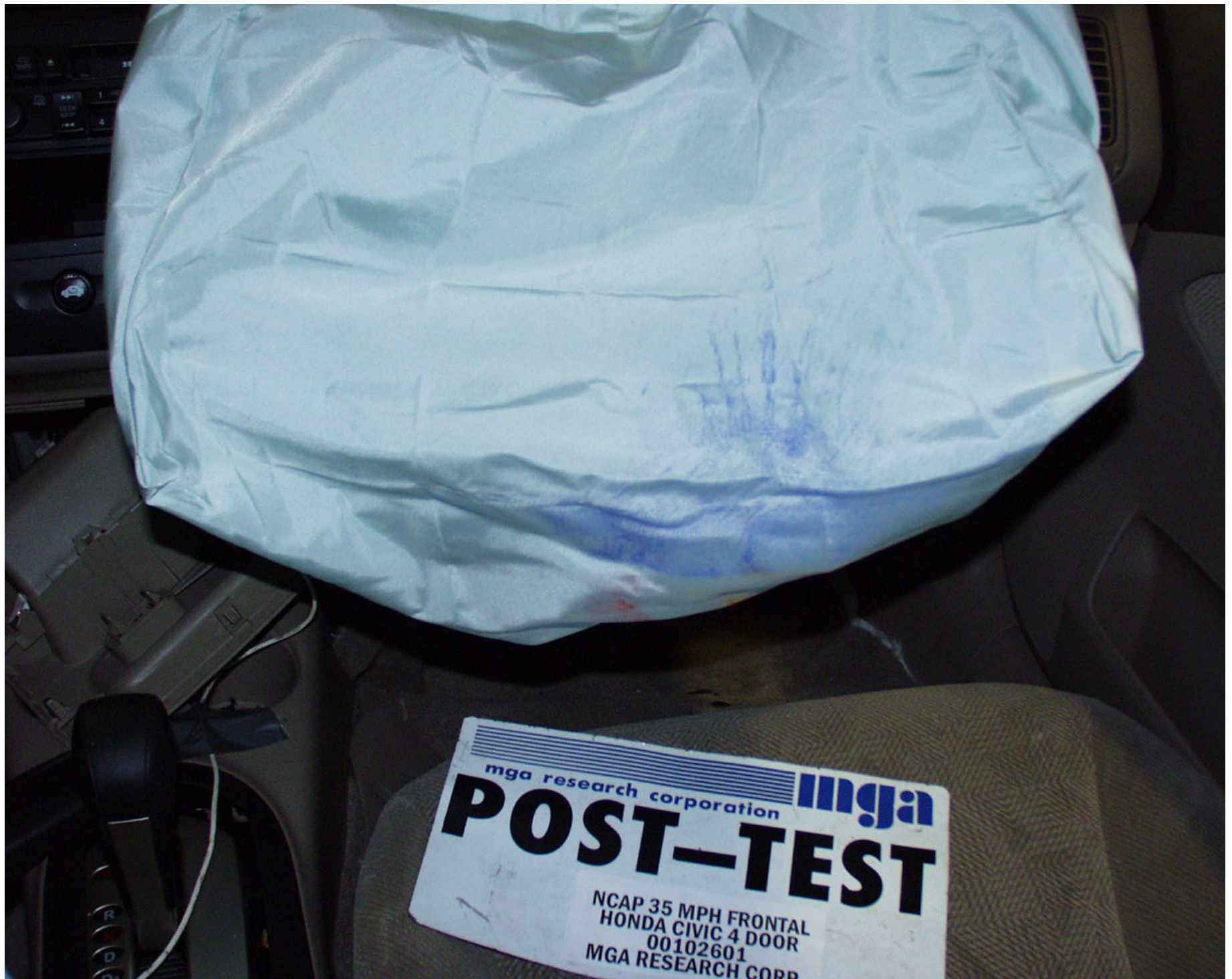
Photo No. A-43 - Post-Test Passenger Airbag Contact
