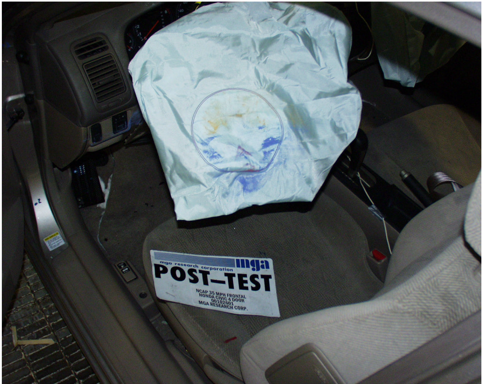
Photo No. A-30 - Post-Test Driver Airbag Contact
