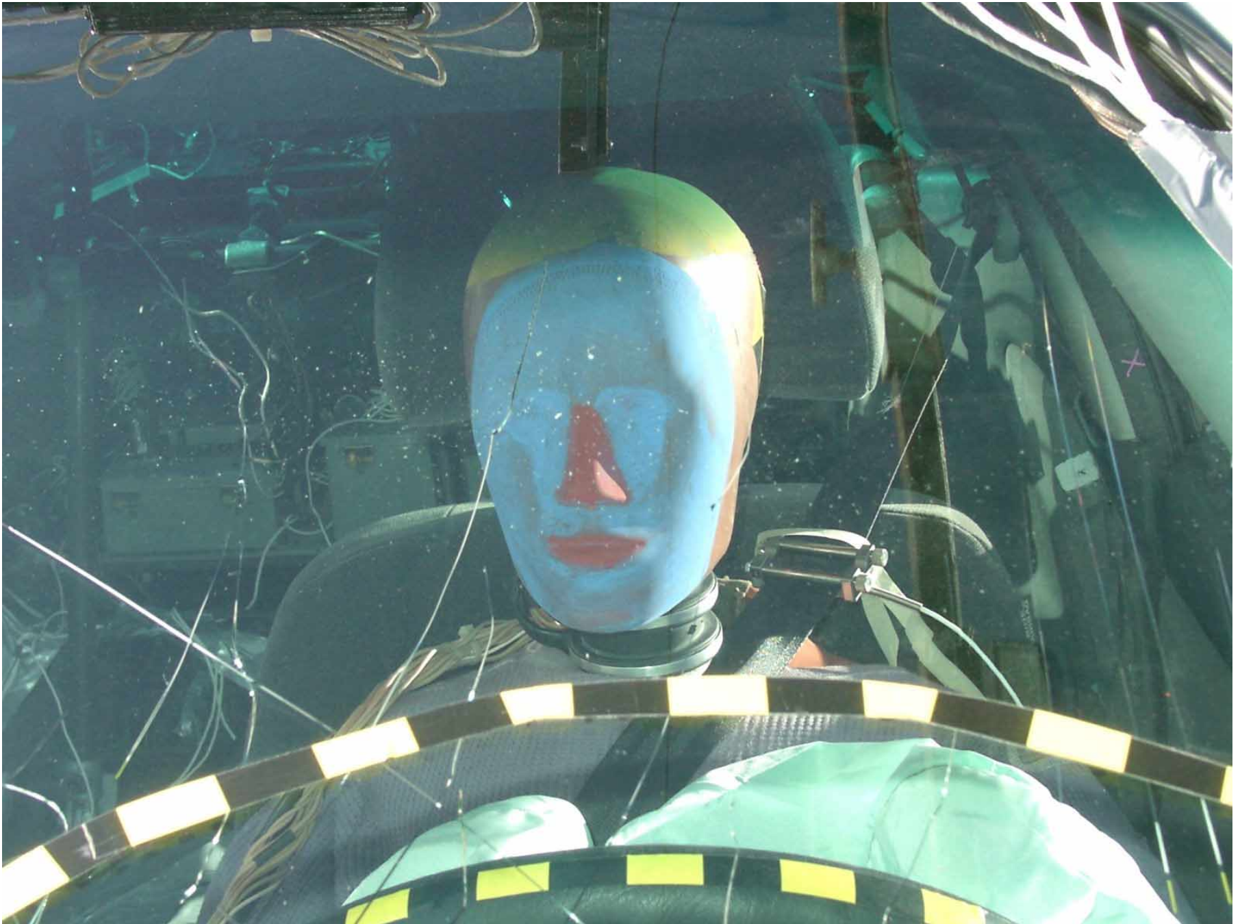
Figure A-26: Driver Dummy Front View, Post-Test
