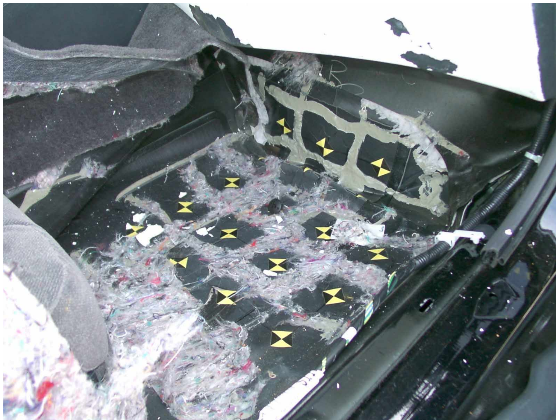
Figure A-52: Passenger Side Floor Pan, Post-Test
