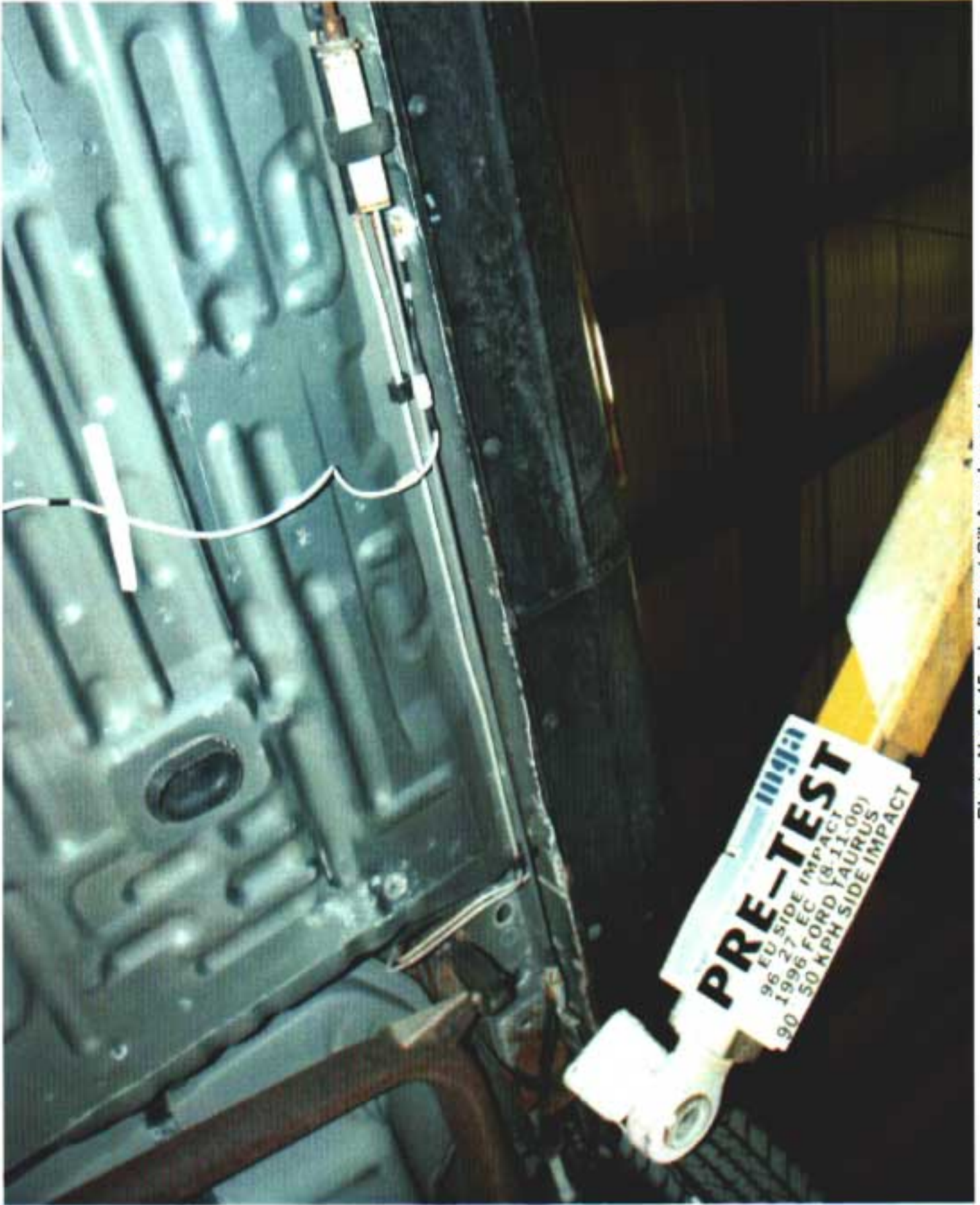
Photo No. A-45 – Left Front Sill Accelerometer
