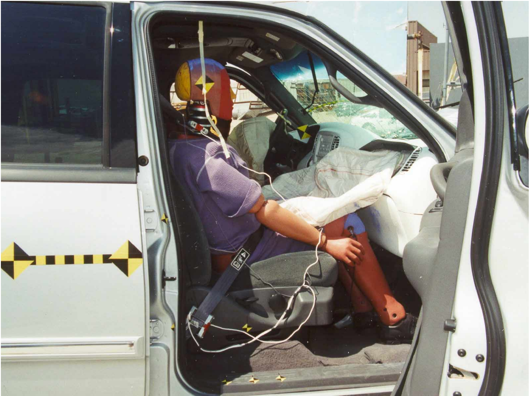
Figure A-48: Passenger Dummy 90° To Vehicle, Post-Test
