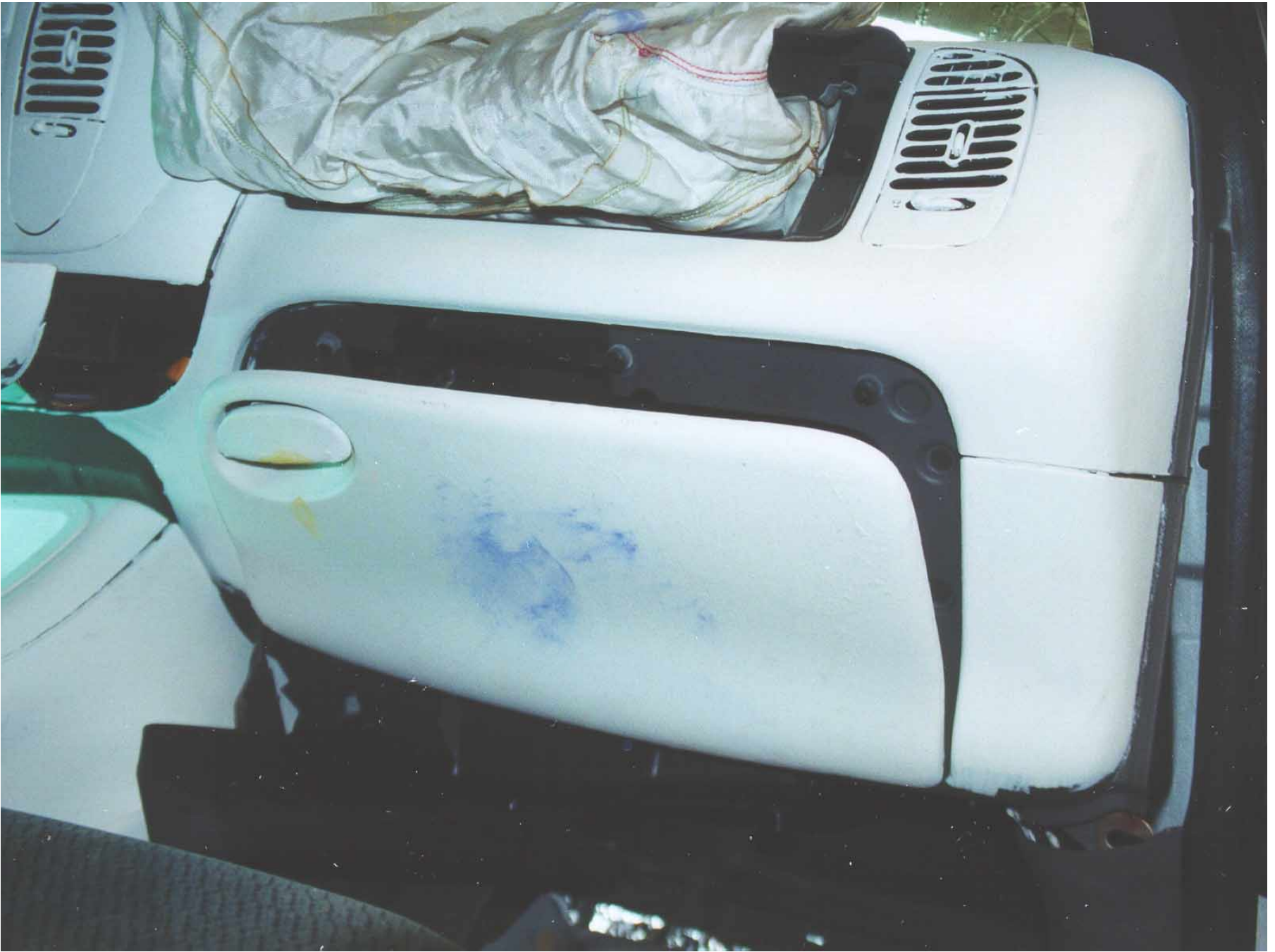
Figure A-54: Passenger Side Knee Bolster, Post-Test
