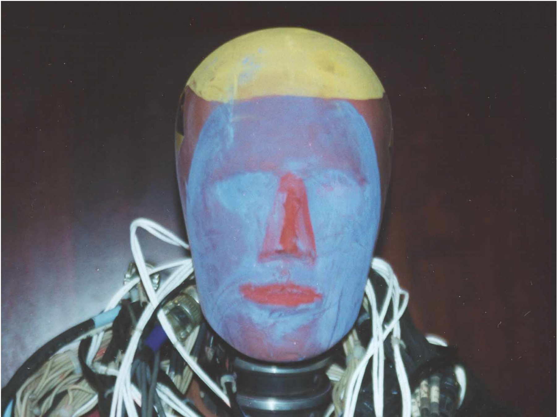
Figure A-41: Driver Dummy Head, Post-Test
