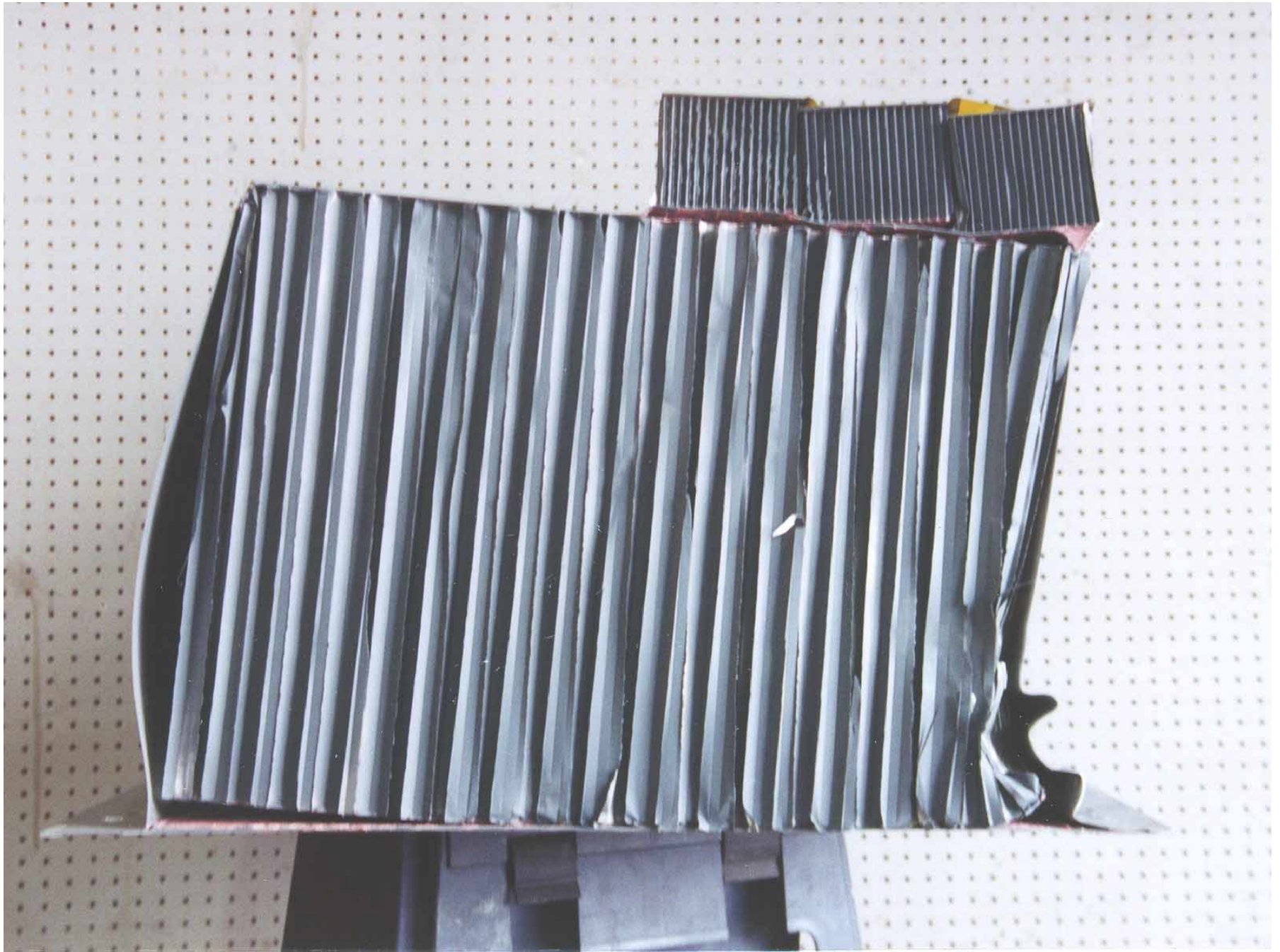
Figure A-62: Deformable Barrier Left Side, Post-Test
