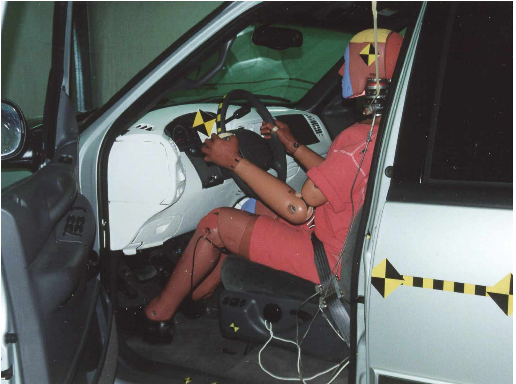
Figure A-31: Driver Dummy Door Open, Pre-Test
