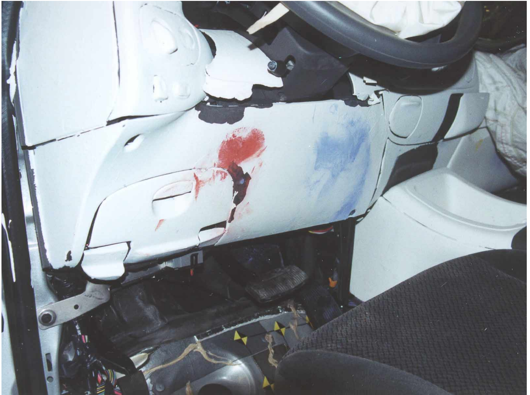
Figure A-40: Driver Side Knee Bolster, Post-Test
