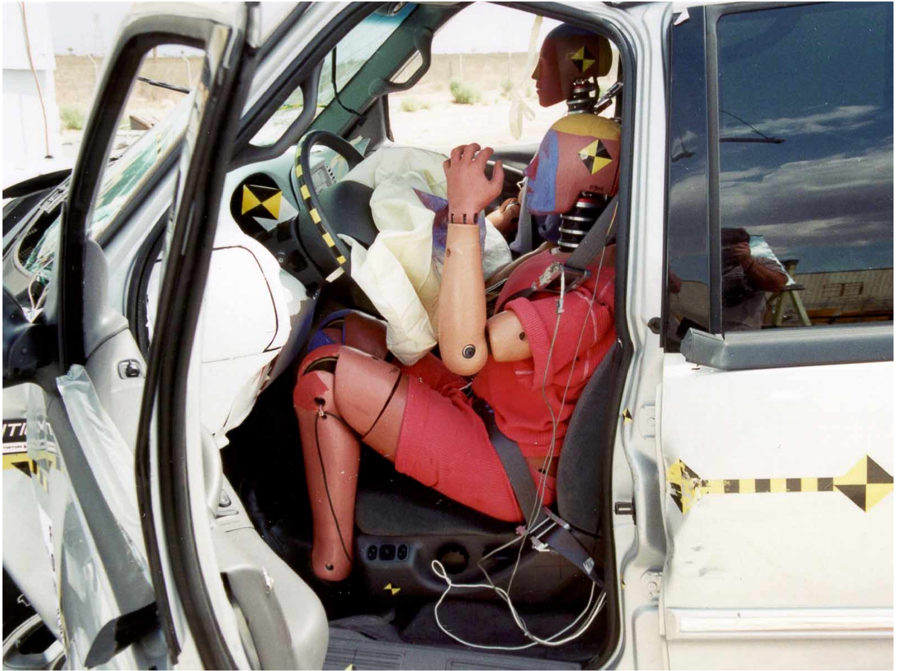
Figure A-34: Driver Dummy 90° To Vehicle, Post-Test
