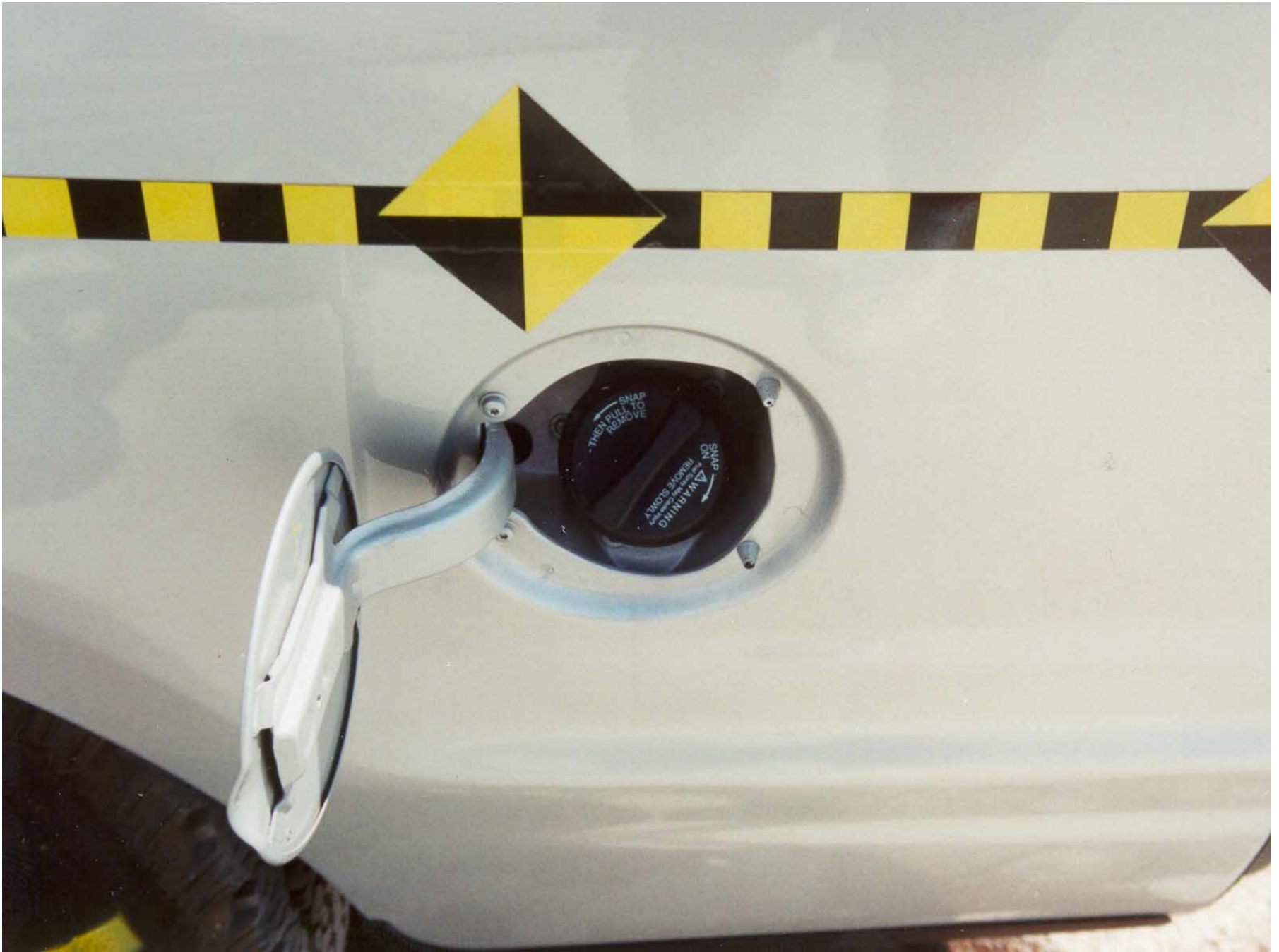
Figure A-20: Fuel Cap, Post-Test
