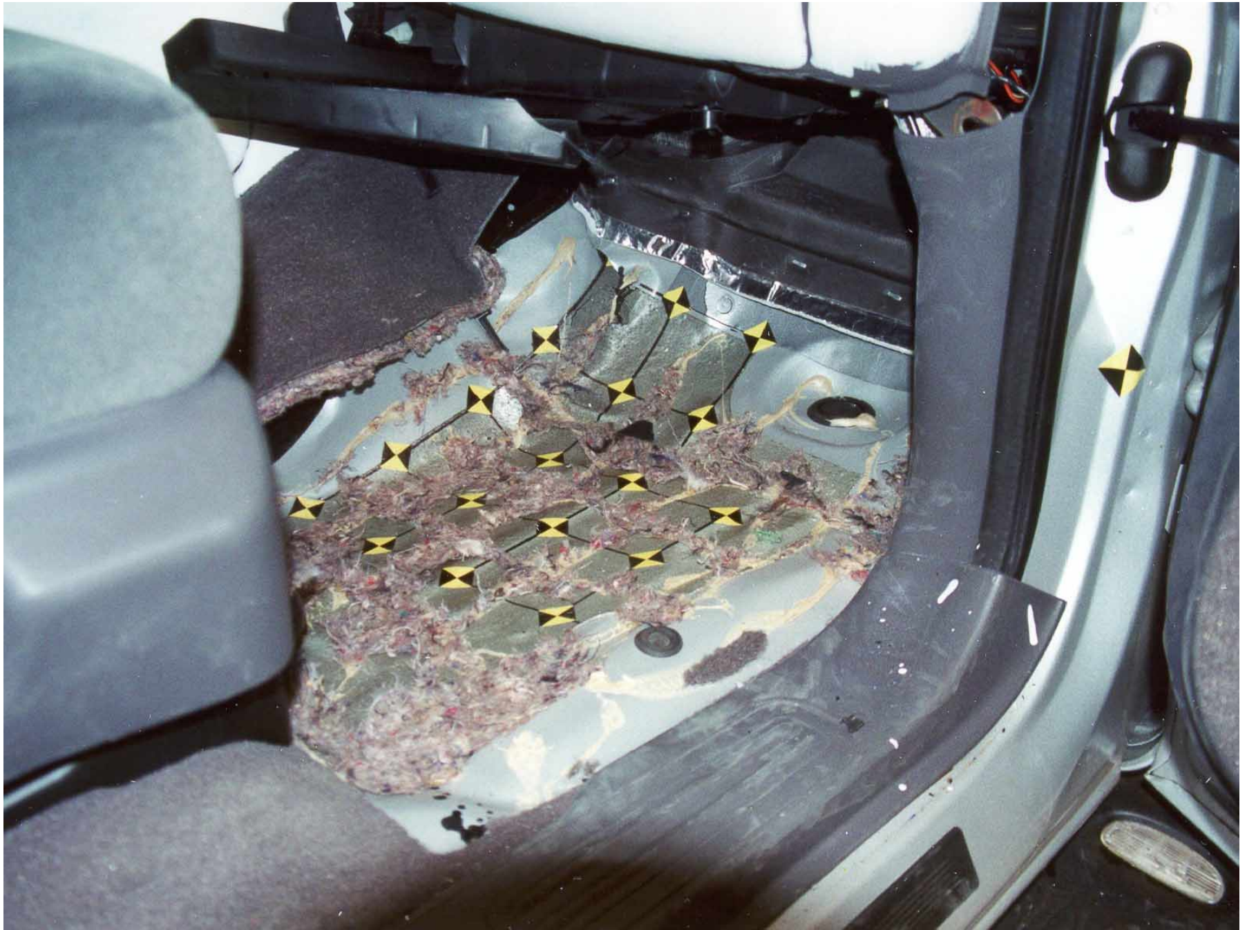
Figure A-52: Passenger Side Floor Pan, Post-Test
