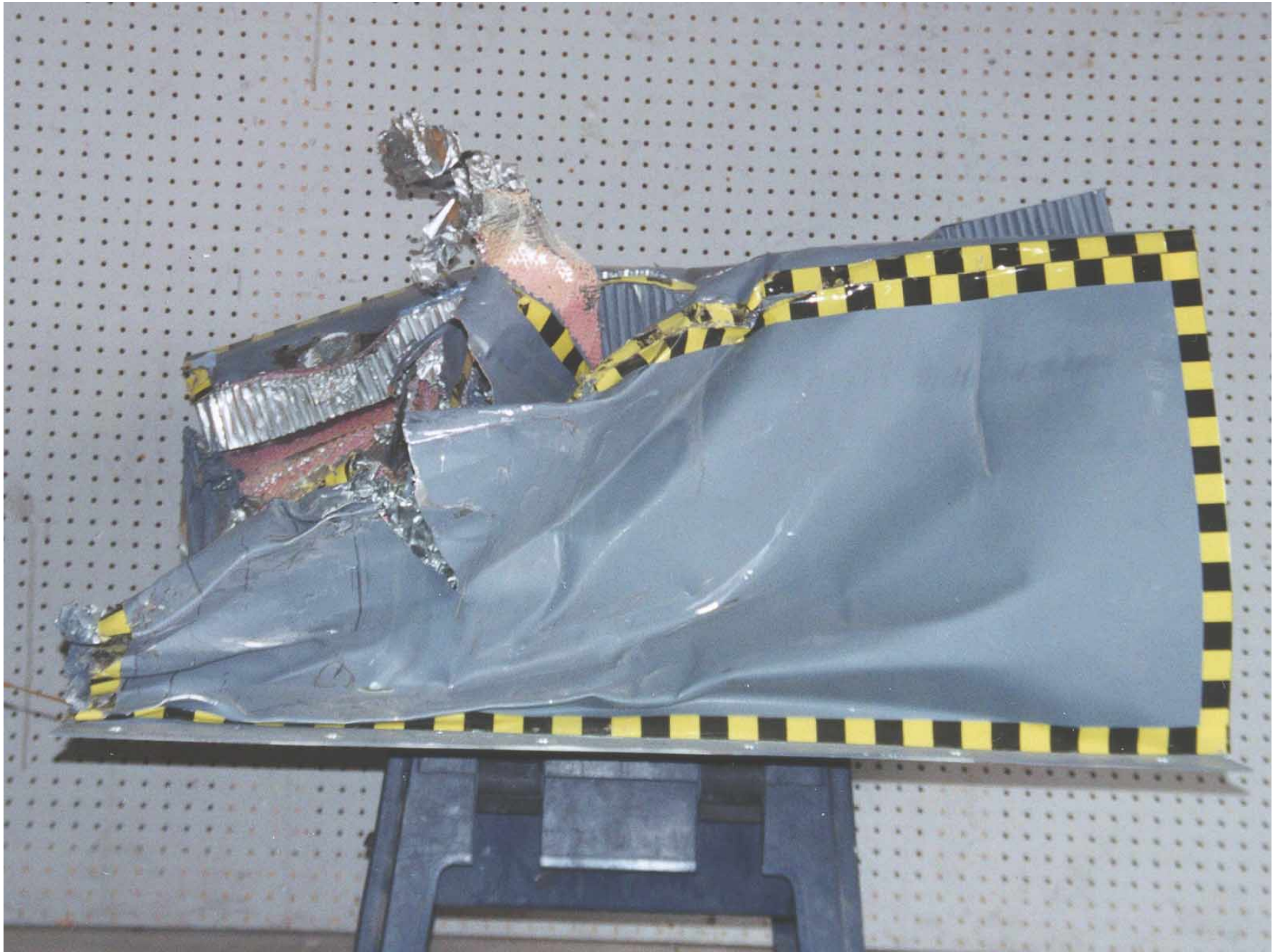
Figure A-66: Deformable Barrier Top, Post-Test
