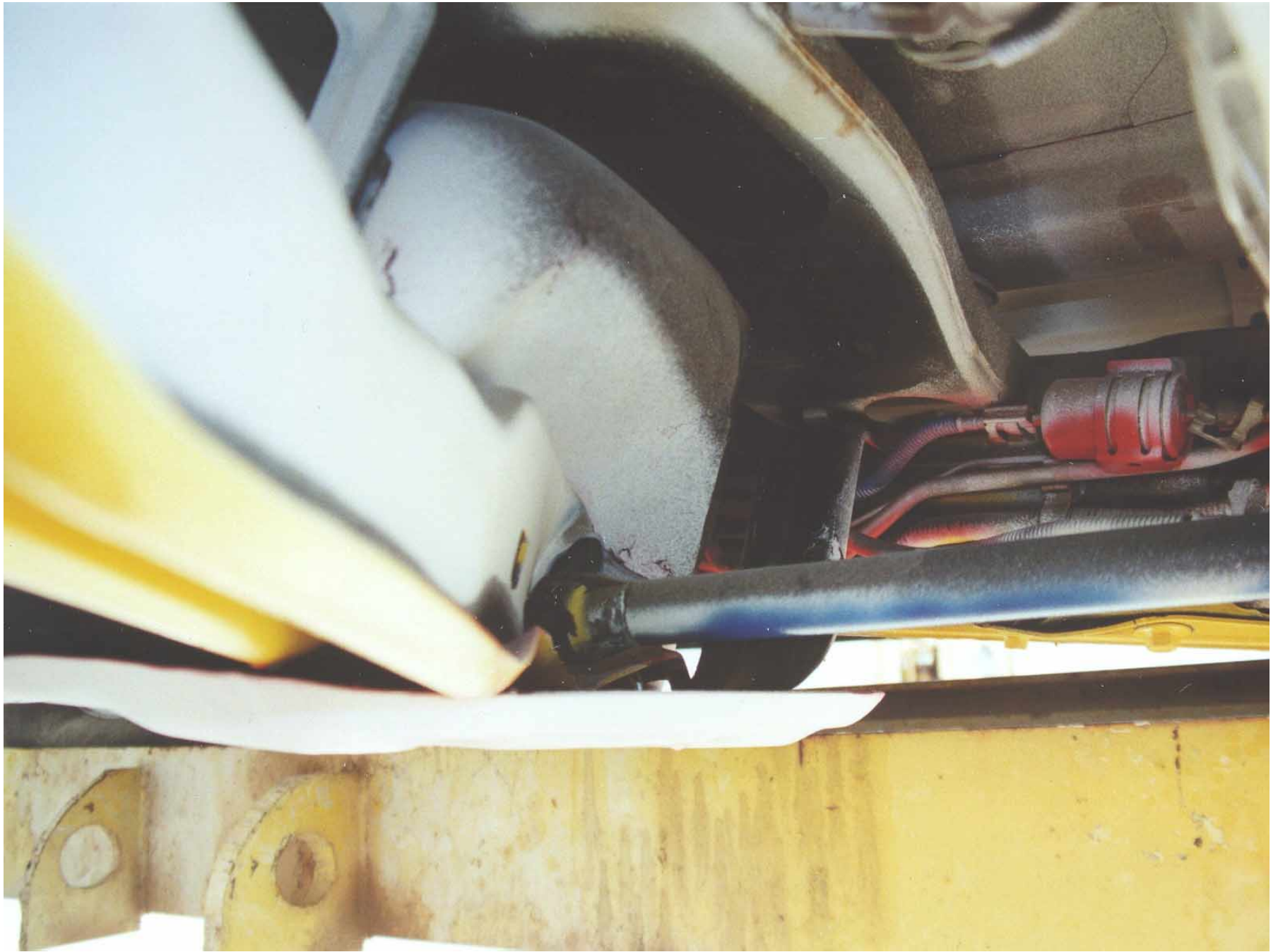
Figure A-69: Fuel Tank, Torsion Bar and Mount Intrusion Into Fuel Tank, Oblique View, Post-Test
