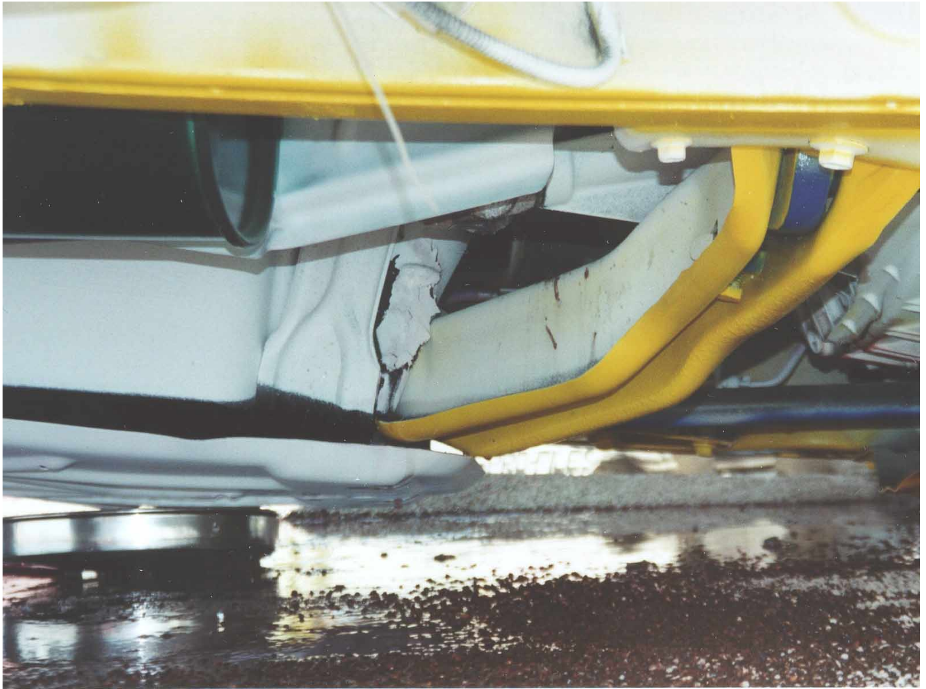
Figure A-68: Fuel Tank, Torsion Bar Mount to Fuel Tank Clearance, Side View, Post-Test
