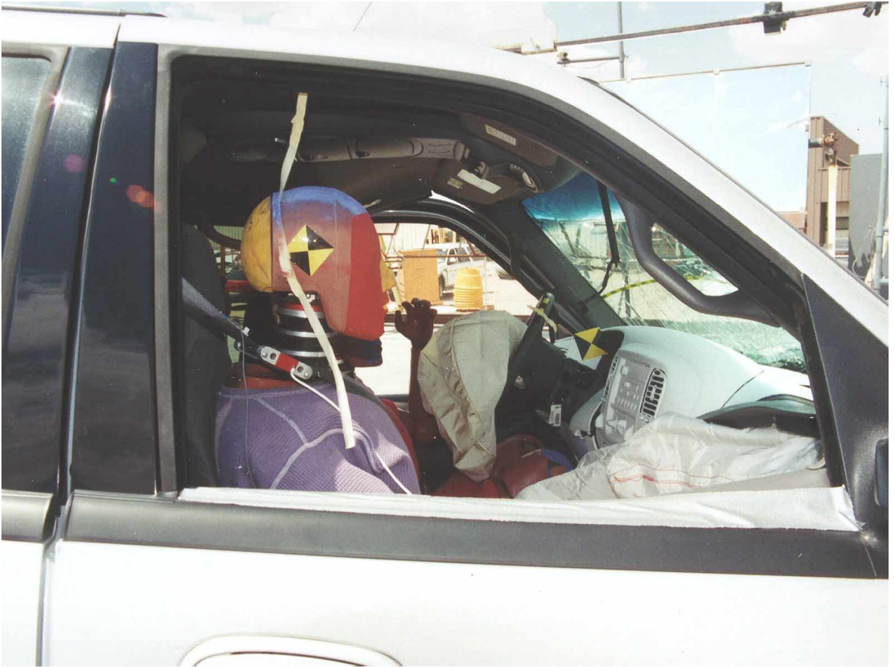
Figure A-44: Passenger Dummy Through Window, Post-Test
