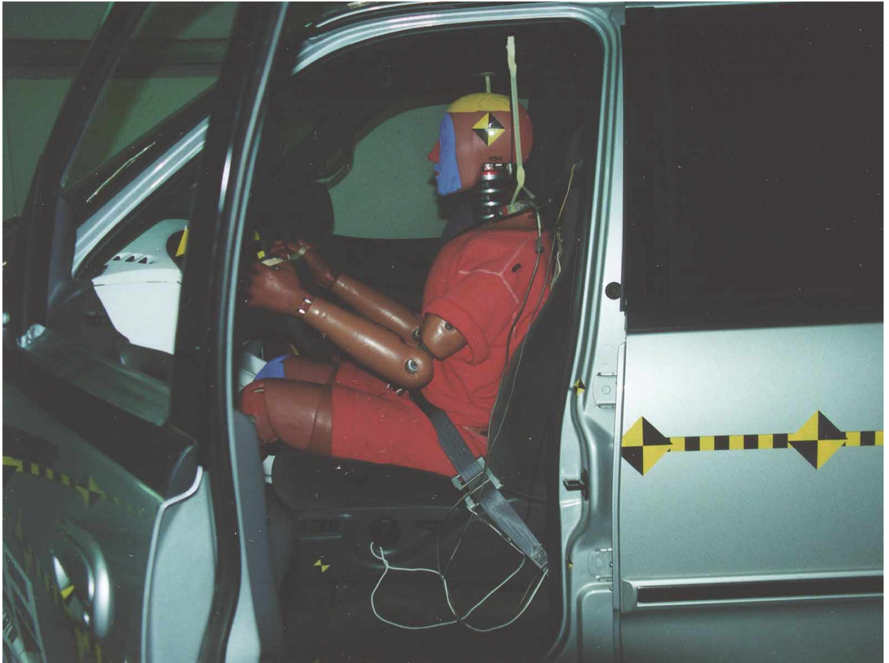
Figure A-33: Driver Dummy 90° To Vehicle, Pre-Test
