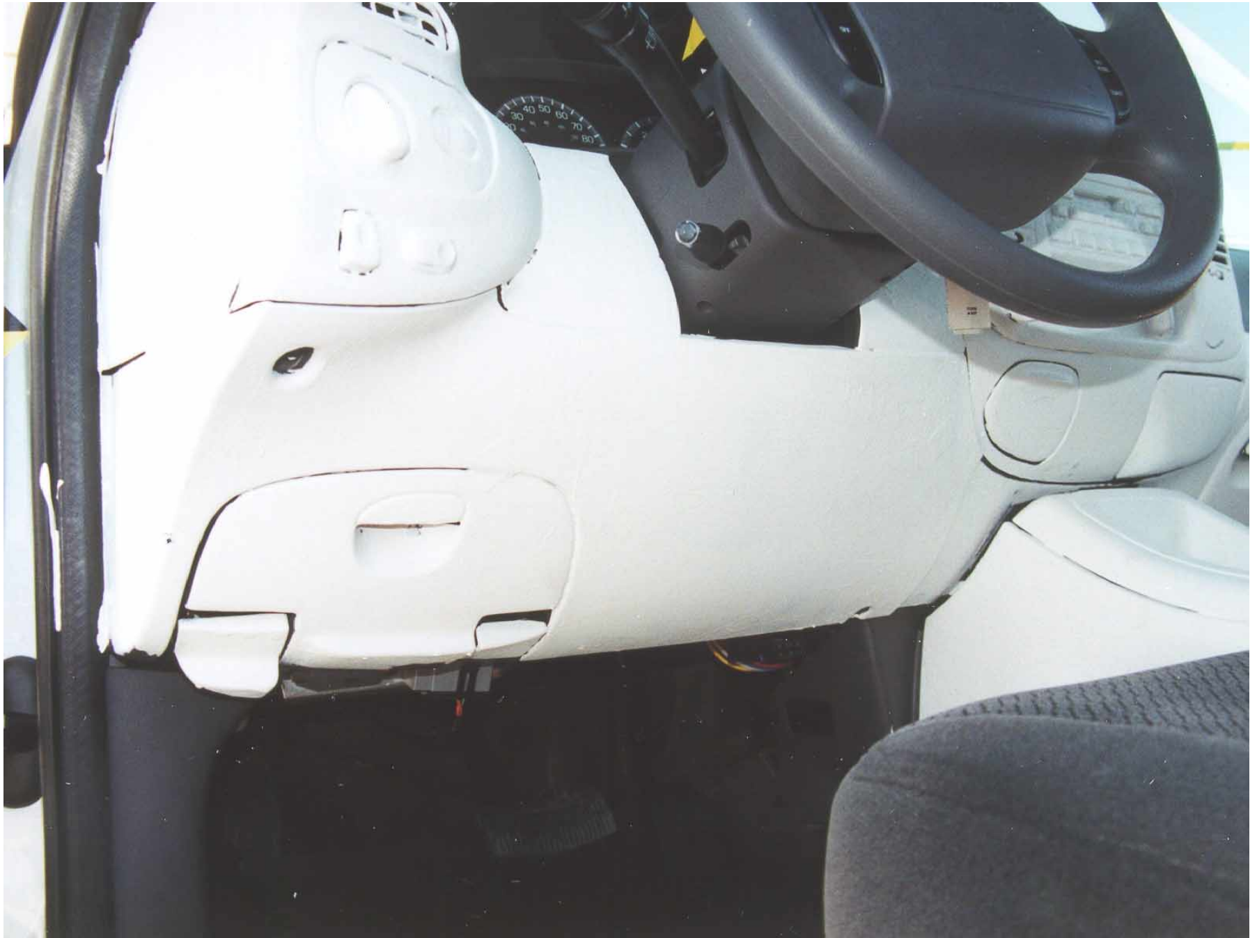
Figure A-39: Driver Side Knee Bolster, Pre-Test
