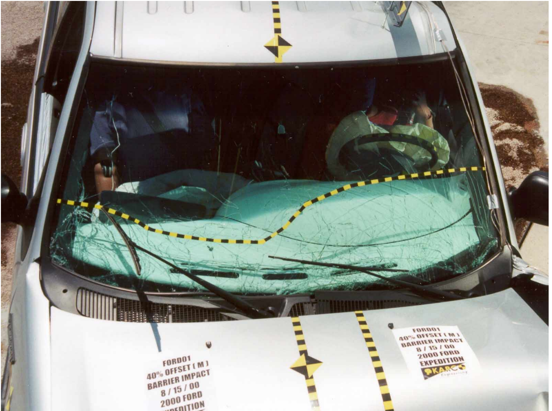
Figure A-16: Windshield, Post-Test
