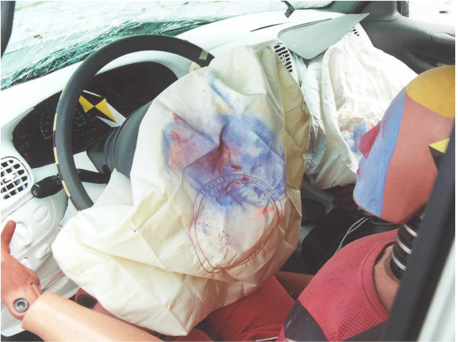
Figure A-42: Driver Dummy Head Contact, Post-Test
