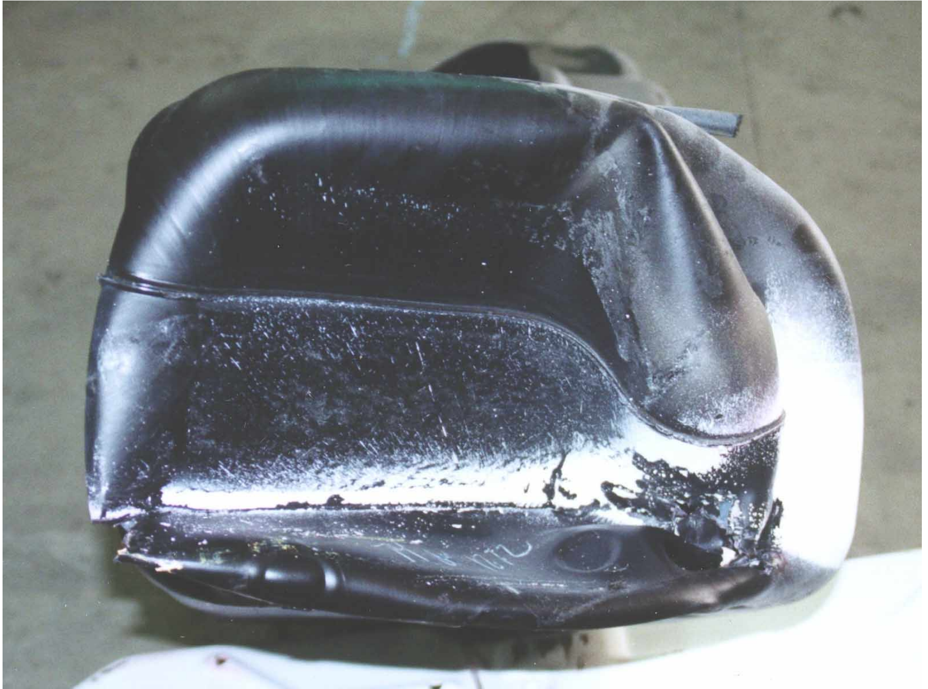
Figure A-71: Fuel Tank, Rupture Close-Up After Removal From Vehicle, Front View, Post-Test
