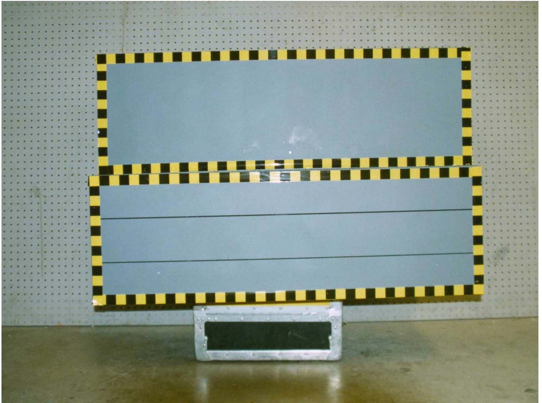
Figure A-59: Deformable Barrier Front, Pre-Test
