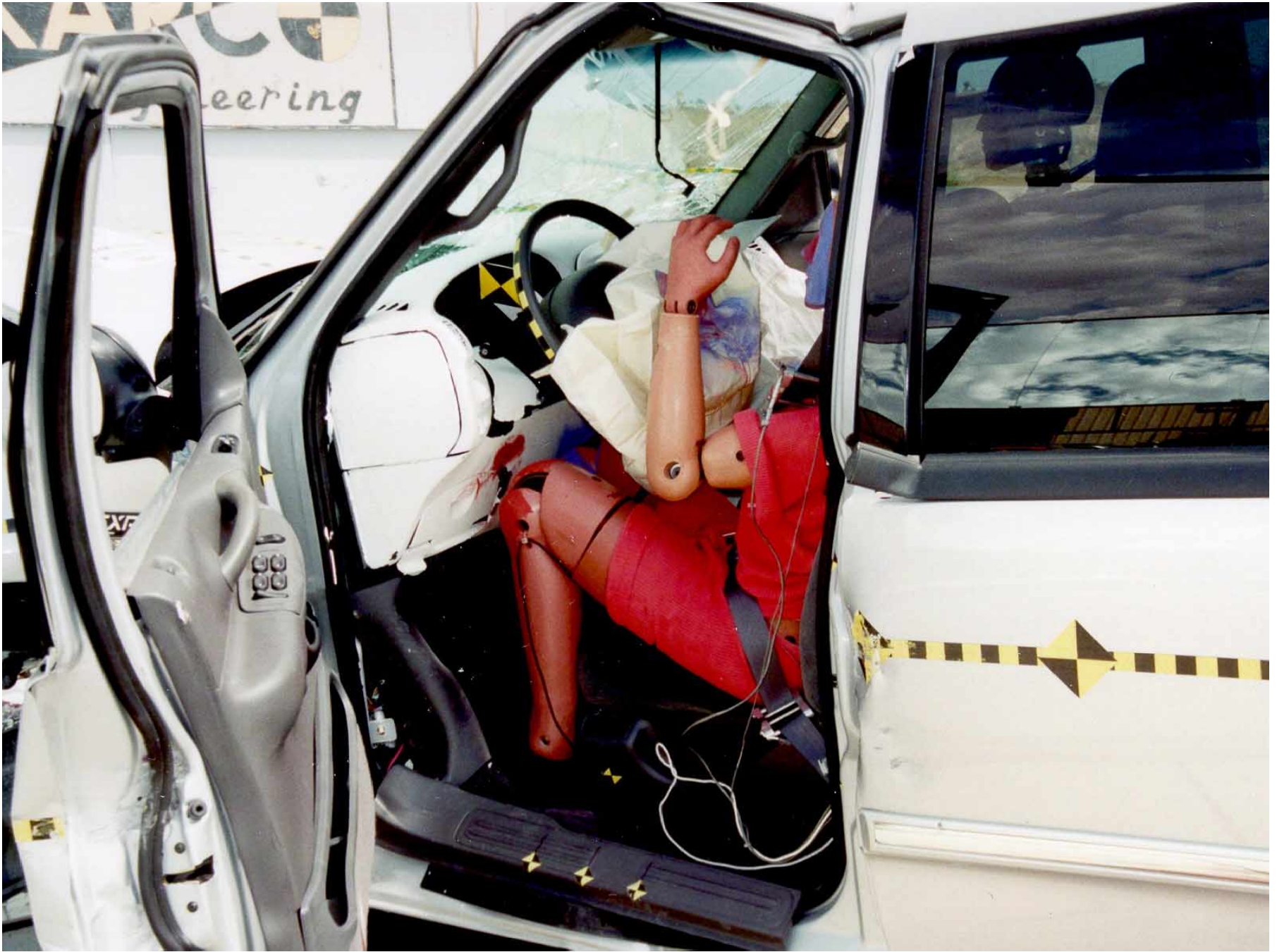
Figure A-32: Driver Dummy Door Open, Post-Test
