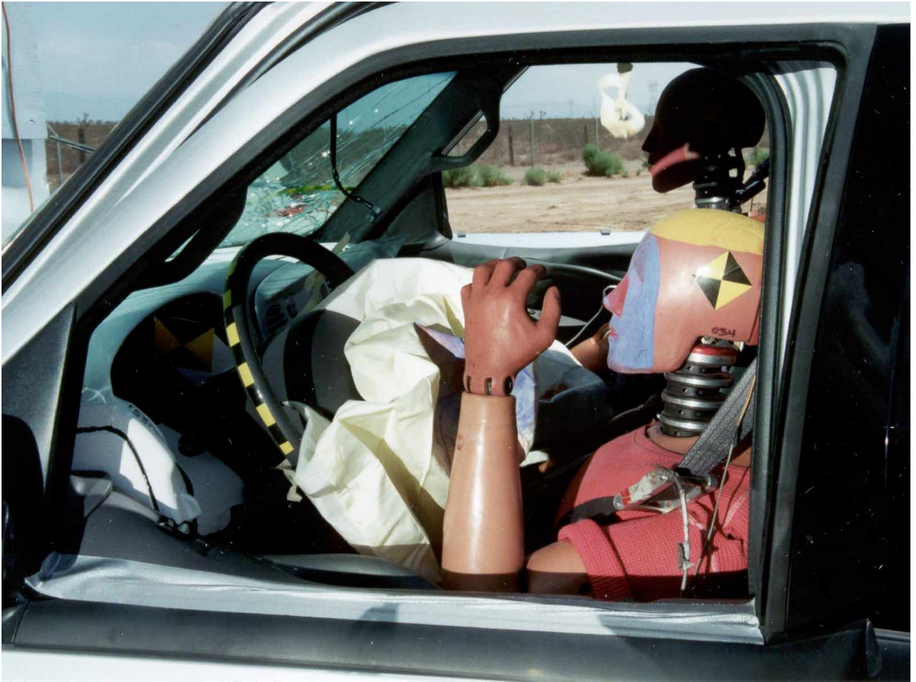
Figure A-30: Driver Dummy Through Window, Post-Test
