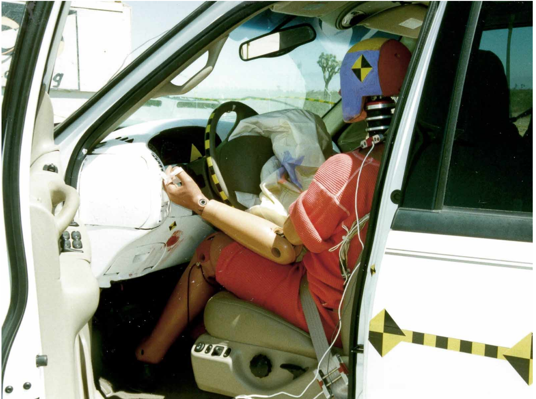
Figure A-32: Driver Dummy Door Open, Post-Test
