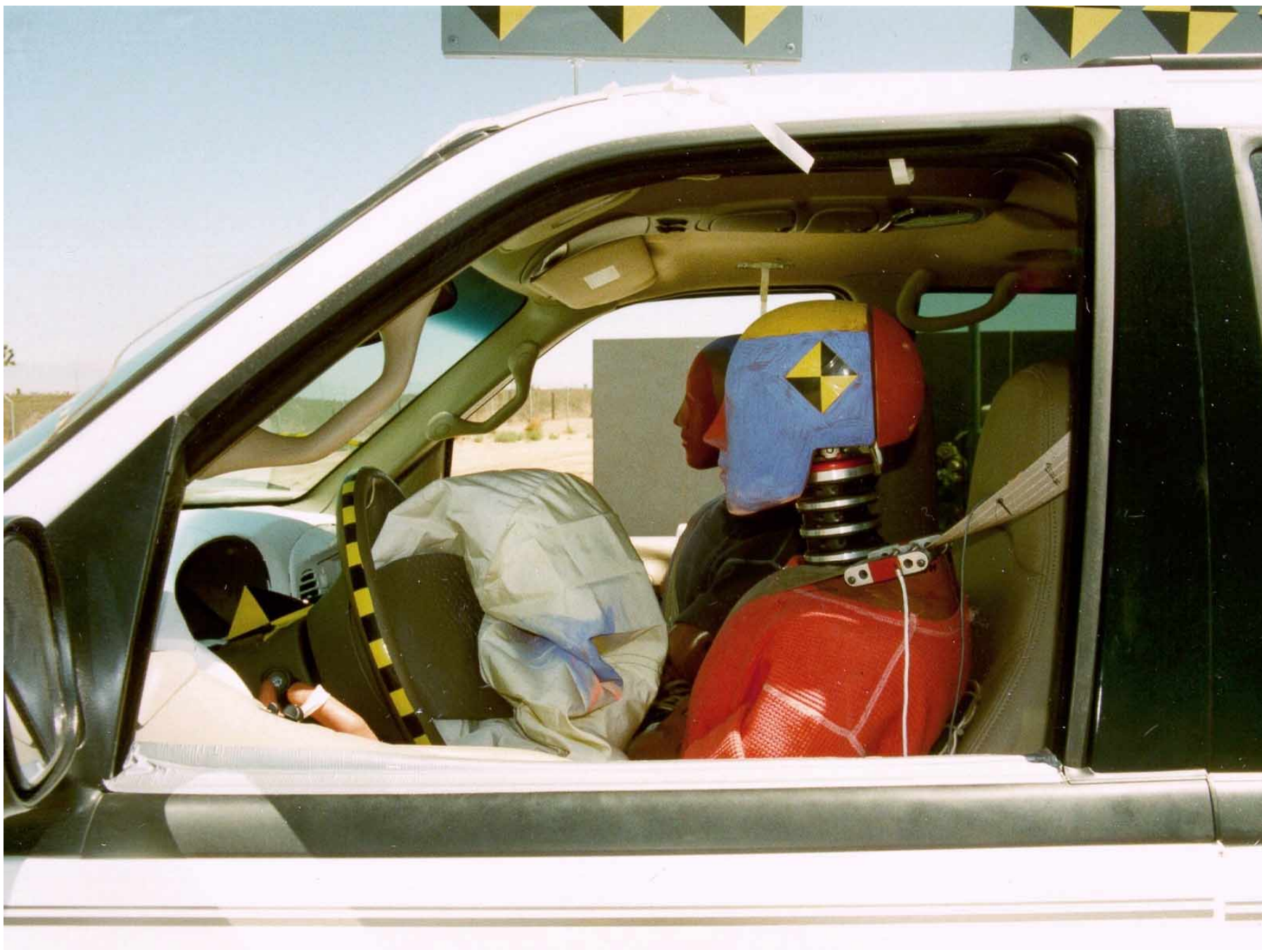
Figure A-30: Driver Dummy Through Window, Post-Test
