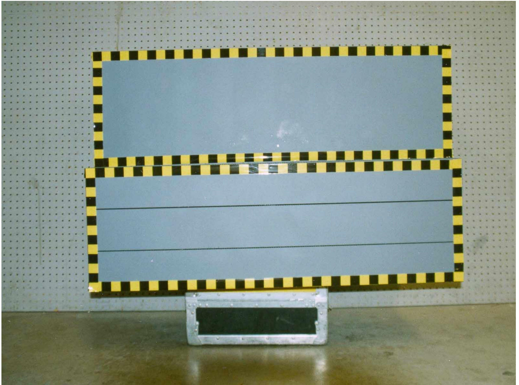
Figure A-58: Deformable Barrier Front, Pre-Test
