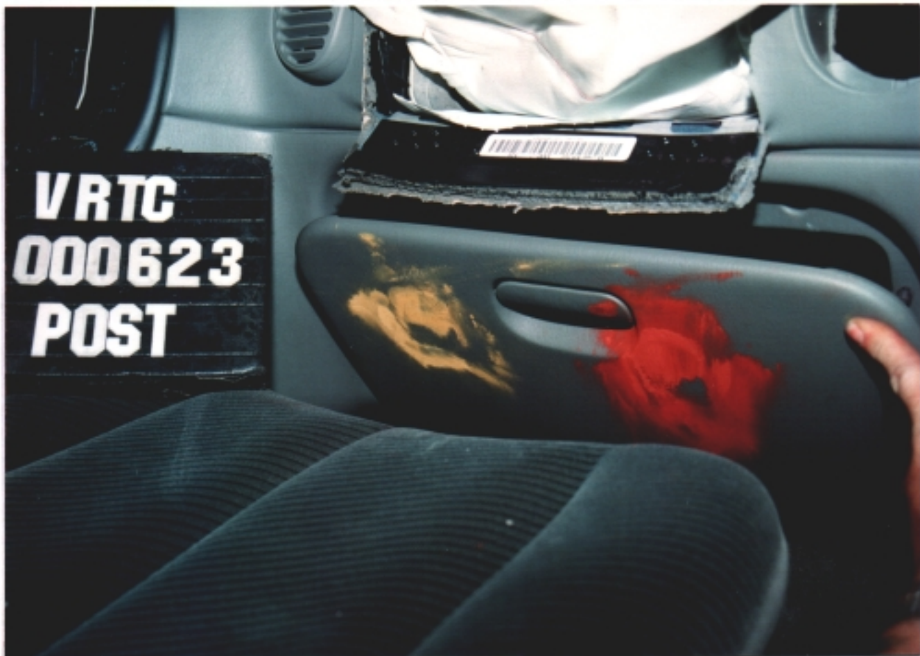
Figure A-107 Post-Test Bullet Vehicle Passenger Dummy Knee Contact - View 2
