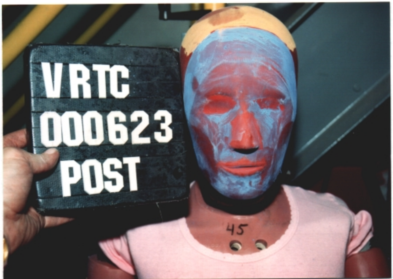
Figure A-90 Post-Test Bullet Vehicle Driver Dummy Head Contact - View 1
