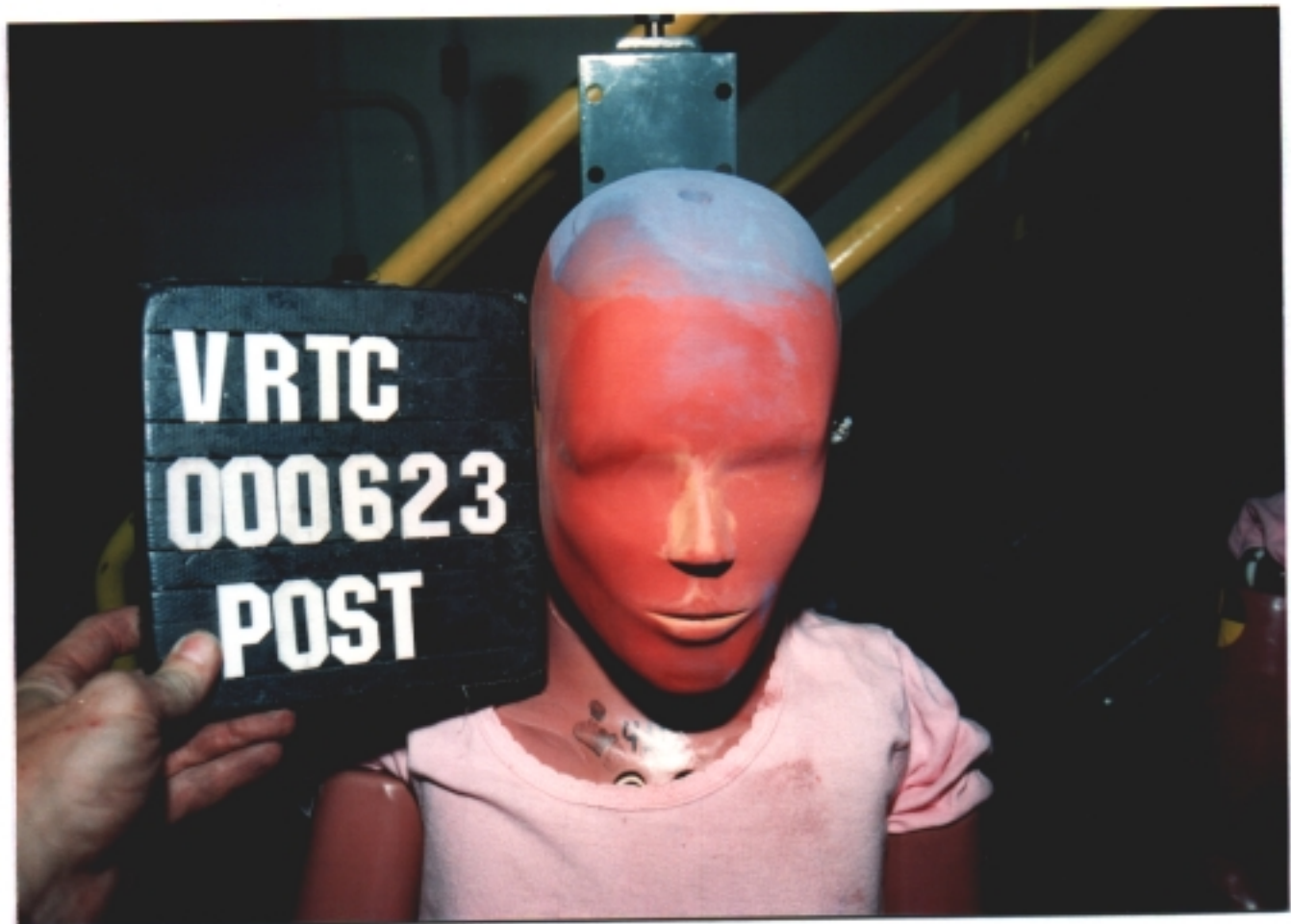
Figure A-104 Post-Test Bullet Vehicle Passenger Dummy Head Contact - View 1
