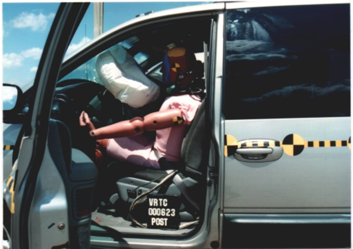
Figure A-86 Post-Test Bullet Vehicle Driver Dummy - View 2
