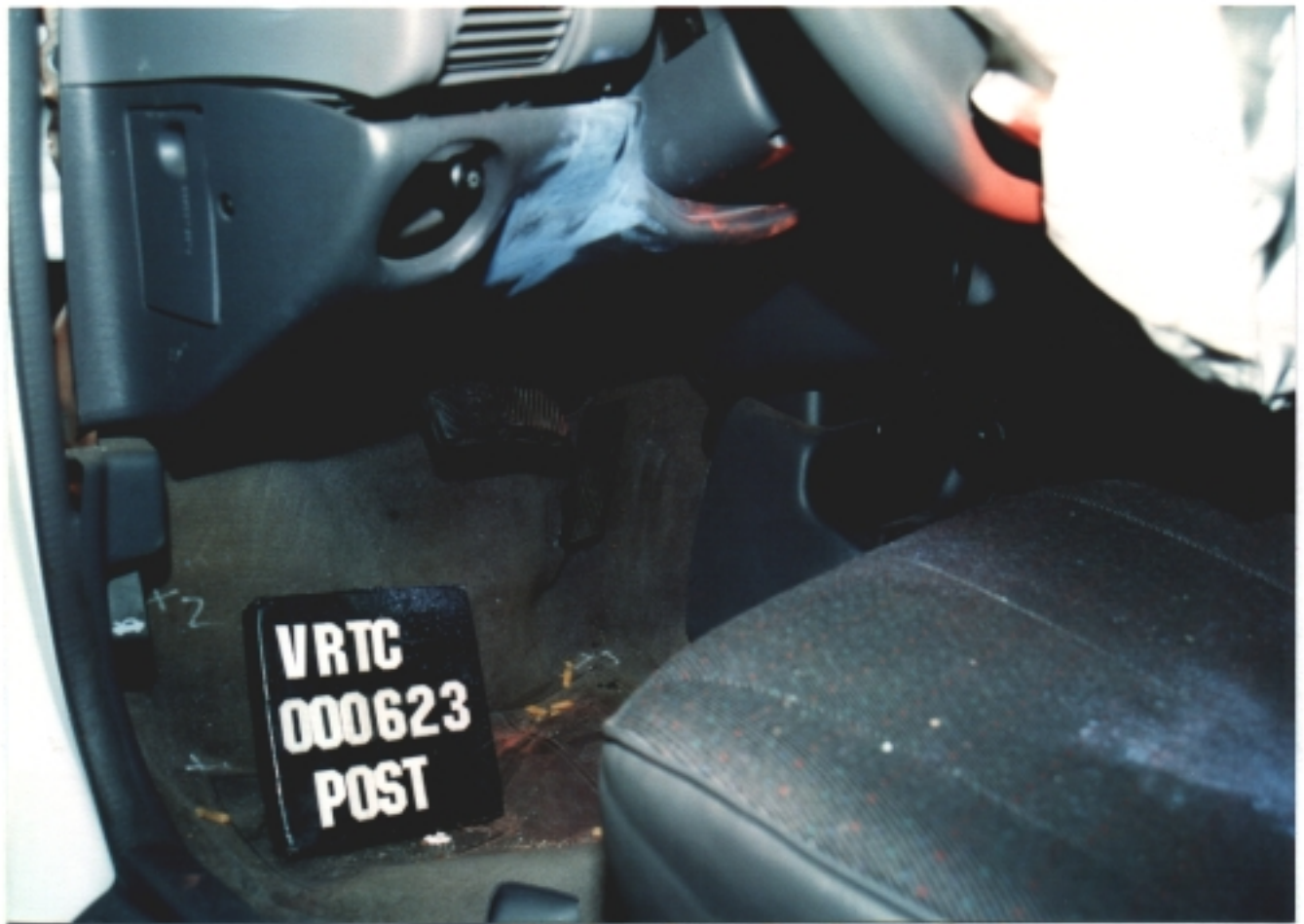
Figure A-46 Post-Test Target Vehicle Driver Dummy Knee Contact - View 2
