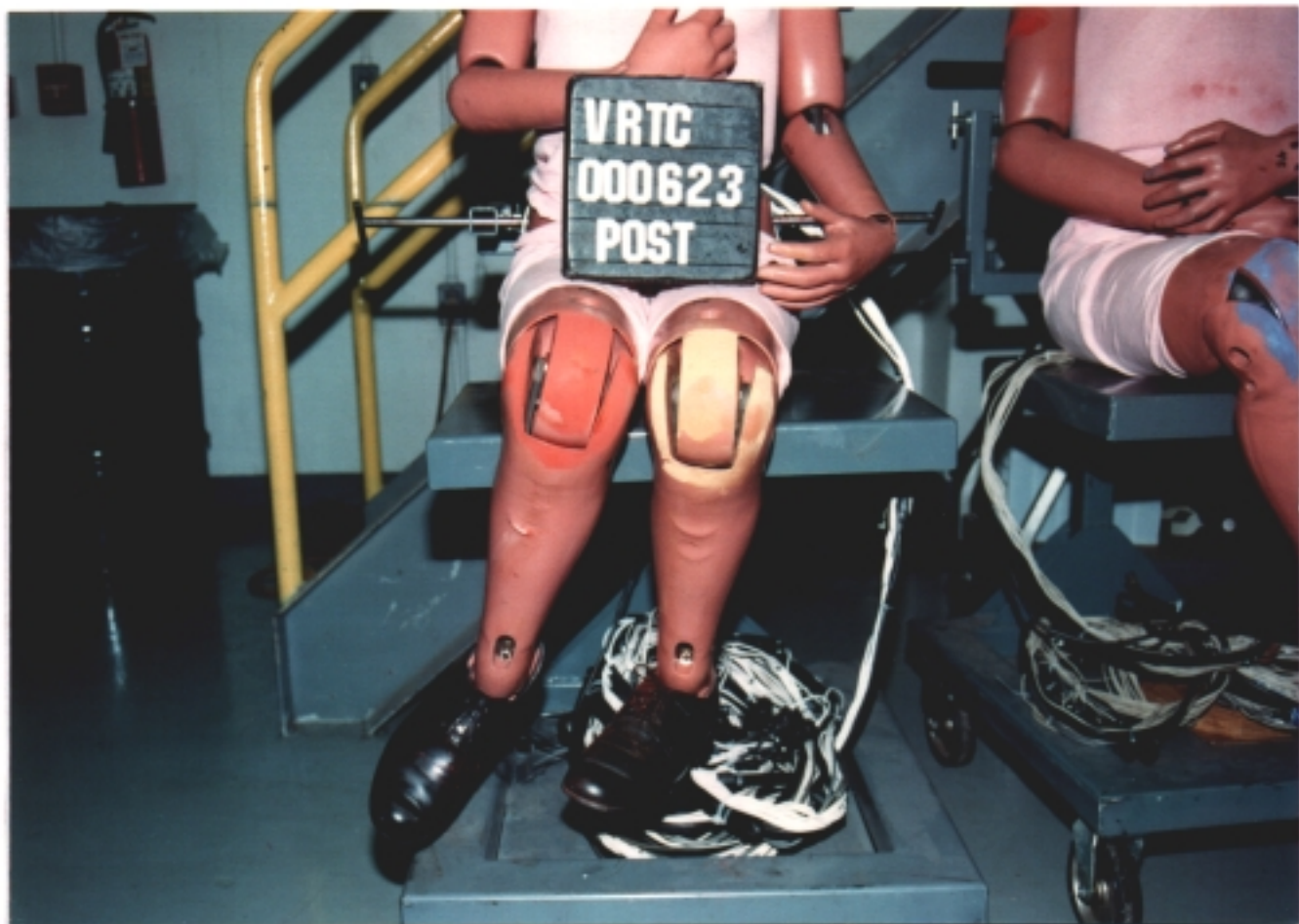
Figure A-106 Post-Test Bullet Vehicle Passenger Dummy Knee Contact - View 1
