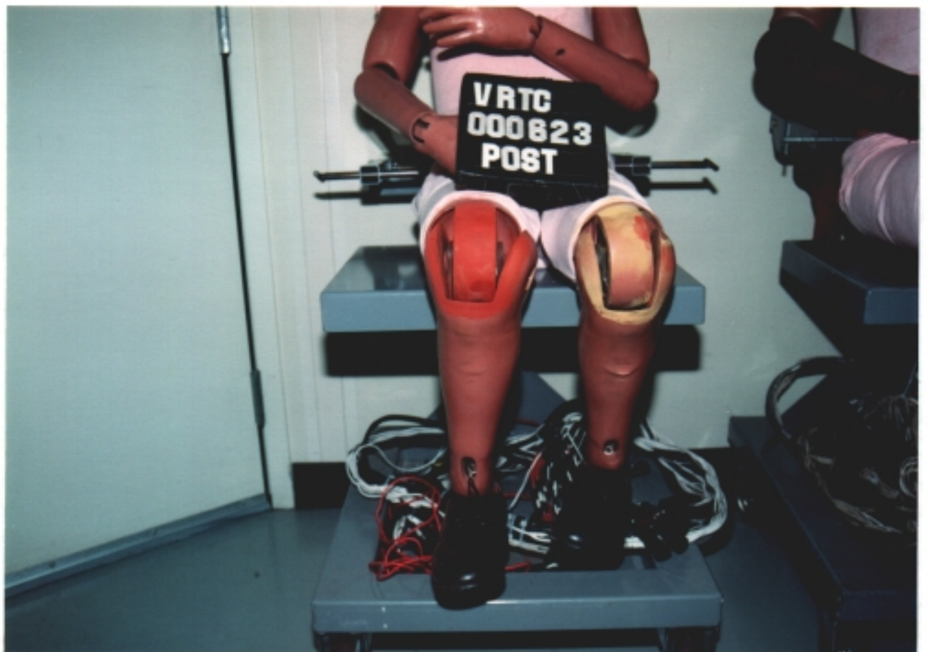
Figure A-58 Post-Test Target Vehicle Passenger Dummy Knee Contact - View 1
