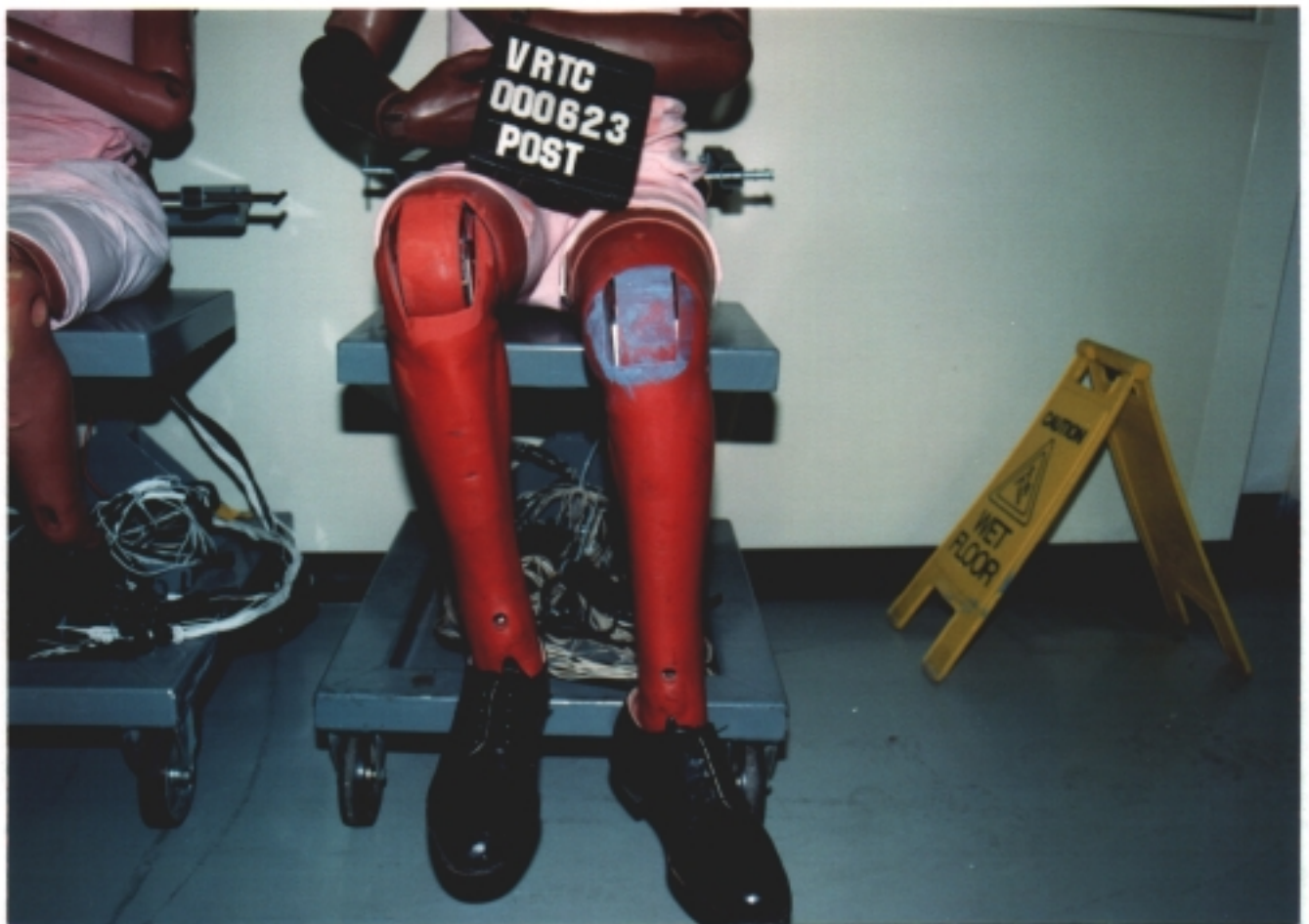
Figure A-45 Post-Test Target Vehicle Driver Dummy Knee Contact - View 1
