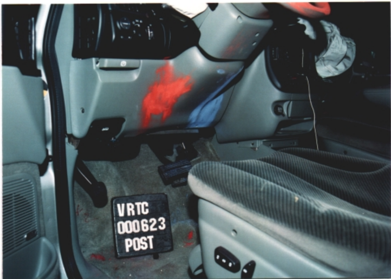
Figure A-94 Post-Test Bullet Vehicle Driver Dummy Knee Contact - View 2
