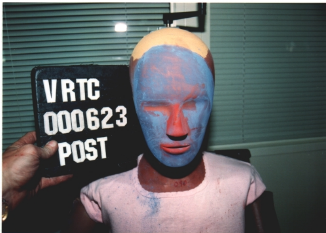
Figure A-42 Post-Test Target Vehicle Driver Dummy Contact View
