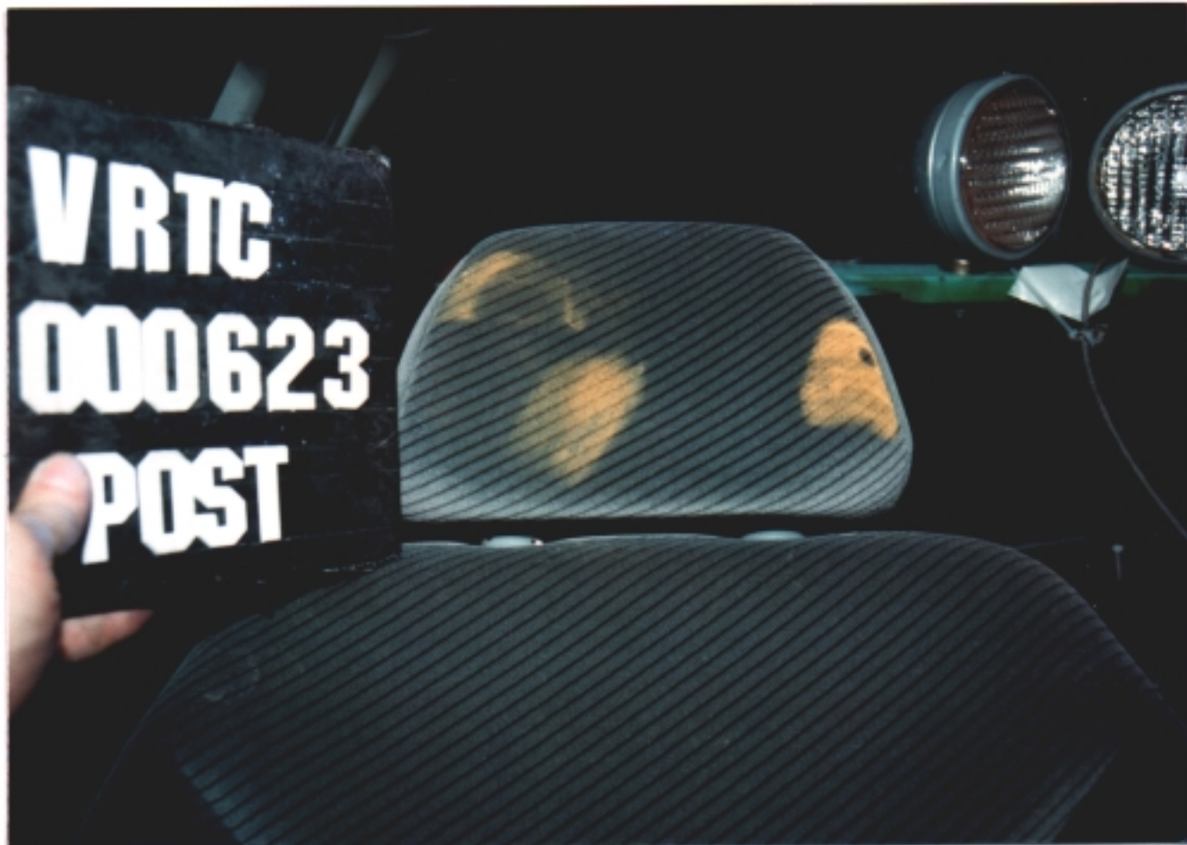
Figure A-105 Post-Test Bullet Vehicle Passenger Dummy Head Contact - View 2
