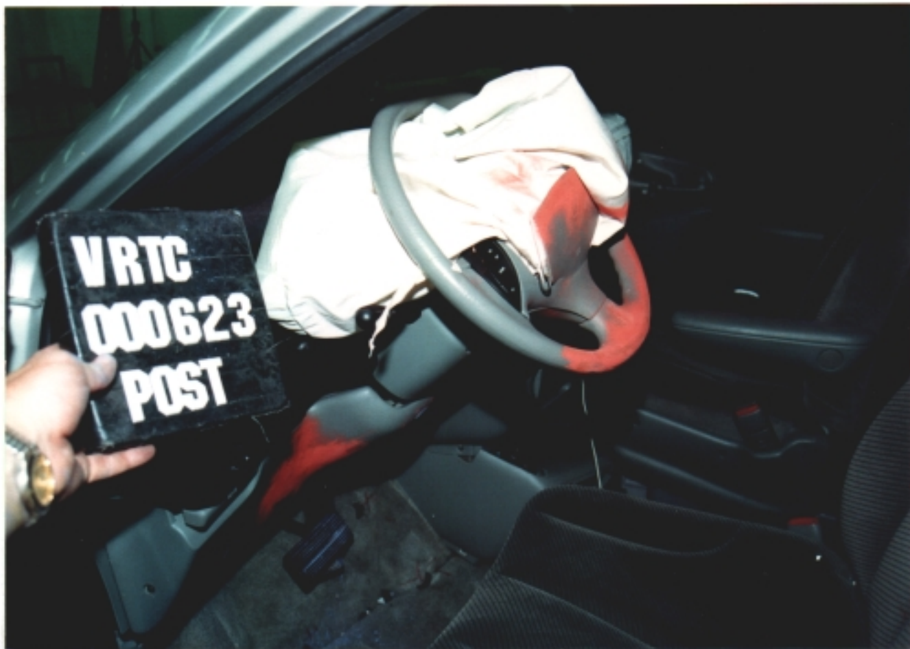
Figure A-96 Post-Test Bullet Vehicle Driver Dummy Abdomen Contact View
