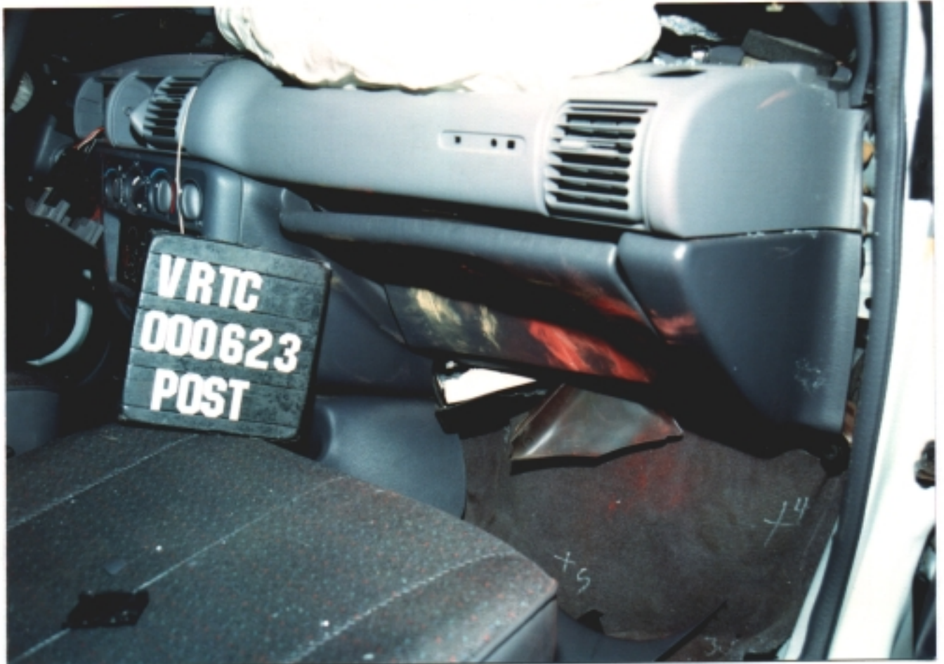
Figure A-59 Post-Test Target Vehicle Passenger Dummy Knee Contact - View 2
