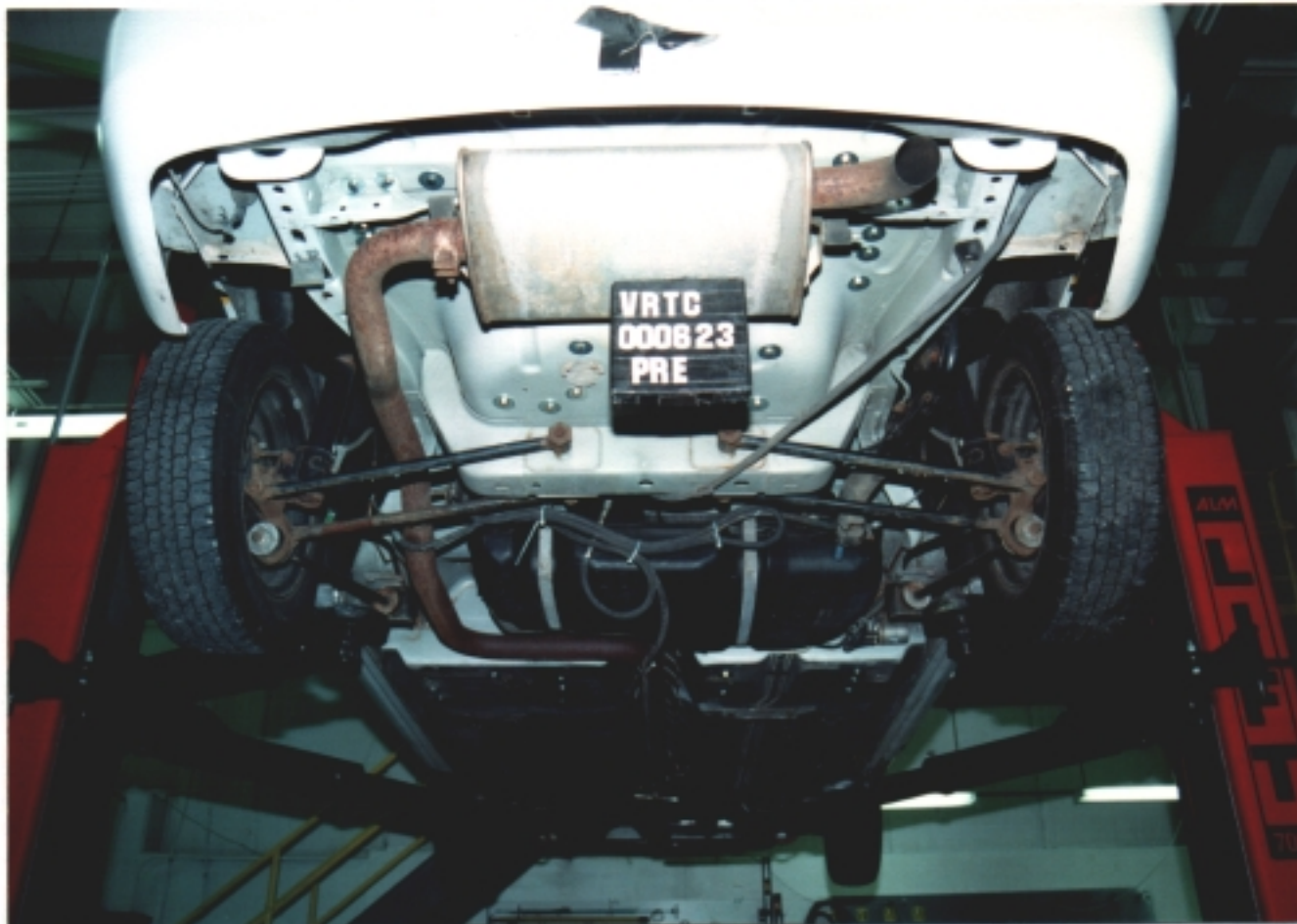
Figure A-27 Pre-Test Target Vehicle Rear Underbody View
