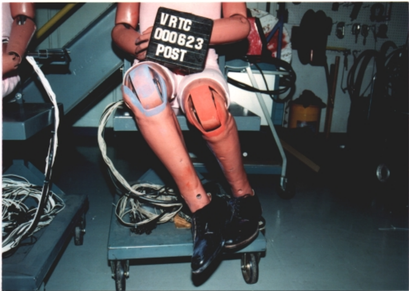
Figure A-93 Post-Test Bullet Vehicle Driver Dummy Knee Contact - View 1
