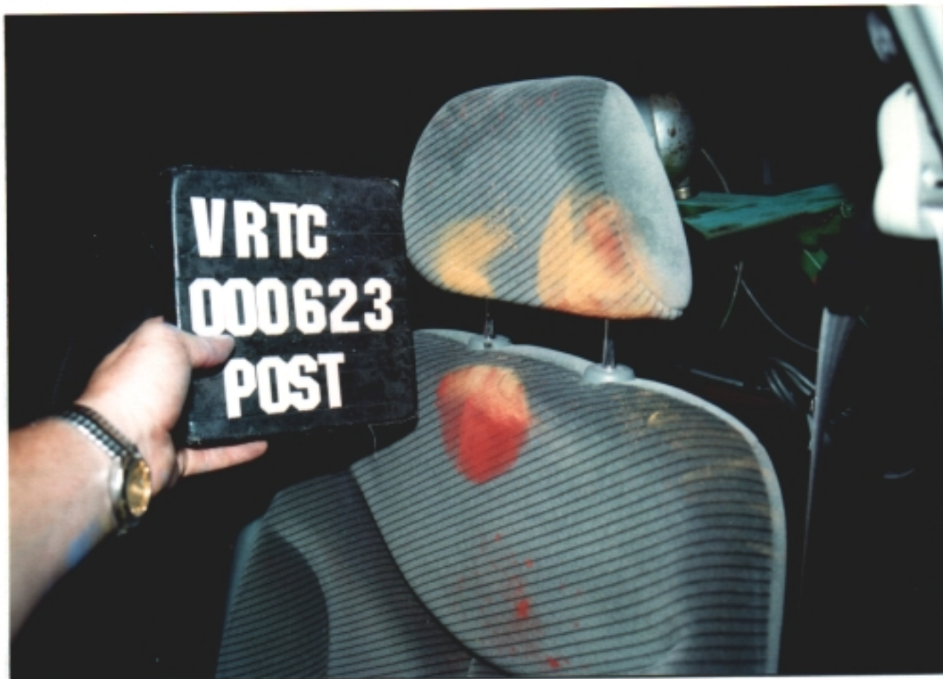
Figure A-92 Post-Test Bullet Vehicle Driver Dummy Head Contact - View 3
