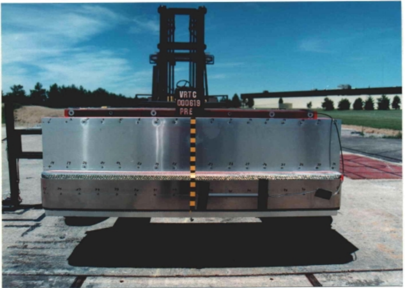
Figure A-30 Pre-Test Moving Deformable Barrier Front View
